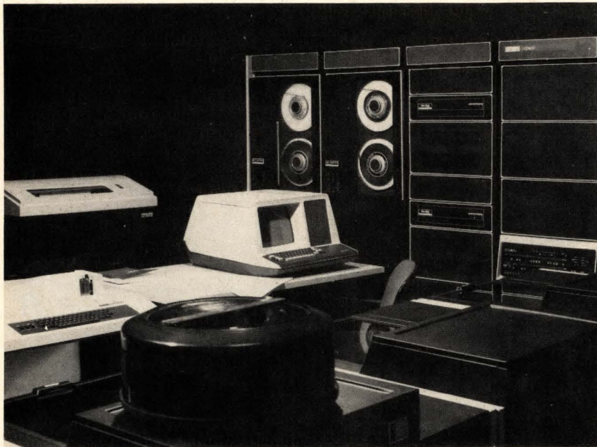
Speedier. DEC's PDP-11/70 minicomputer uses a special 32-bit internal data path to boost speed. Machine also features a cache memory and new high-speed digital controllers.
