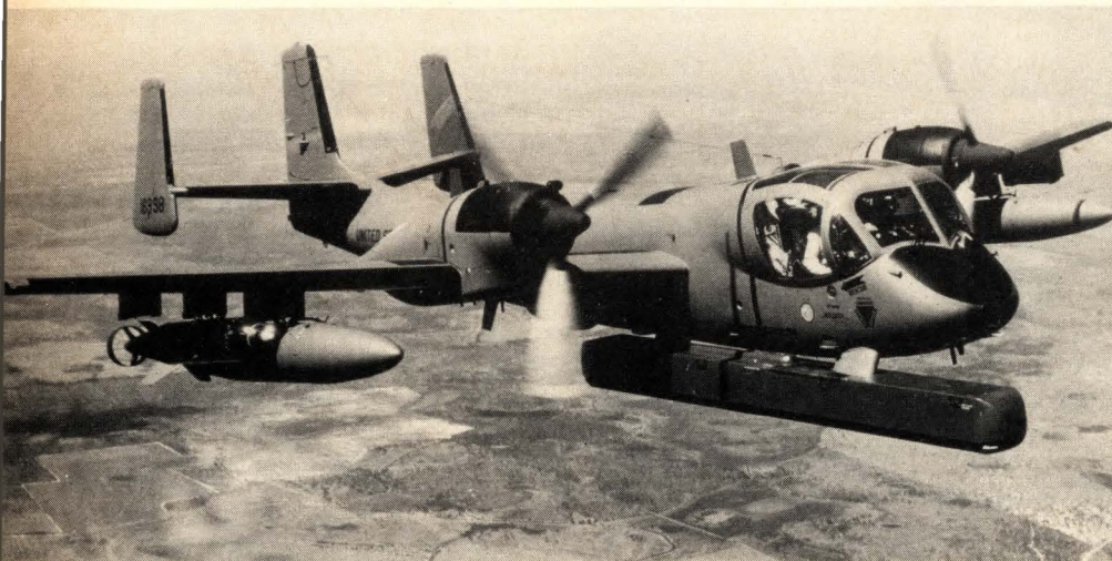
Data in a jiffy. Northrop Corp. transmission system sends data from side-looking radar, slung below Mohawk OV-1D fuselage, to the ground for processing while plane is in the air.
