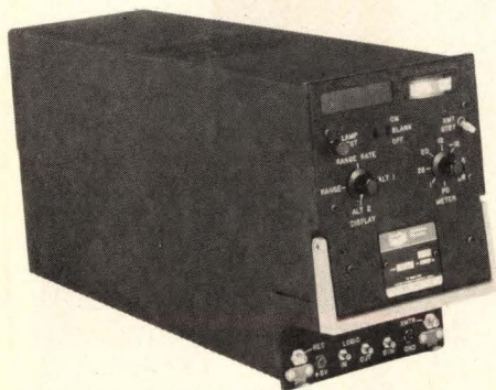
Hardware. Bendix airborne MLS package, above, is similar to one that would be needed for general aviation. At right is Hazeltine's prototype ground MLS system as it was laid out during tests being conducted at Wallops Island, Va.
