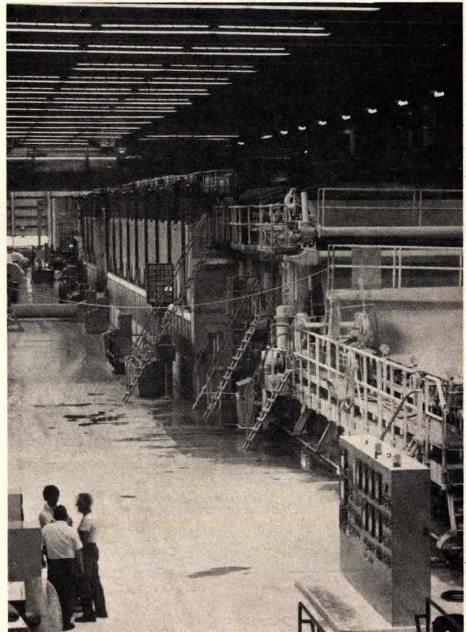
Computerized paper. In-line process measurement and control—which results in paper that runs closer to spec with less scrap and reduced consumption of expensive pulp—should do well this year.
