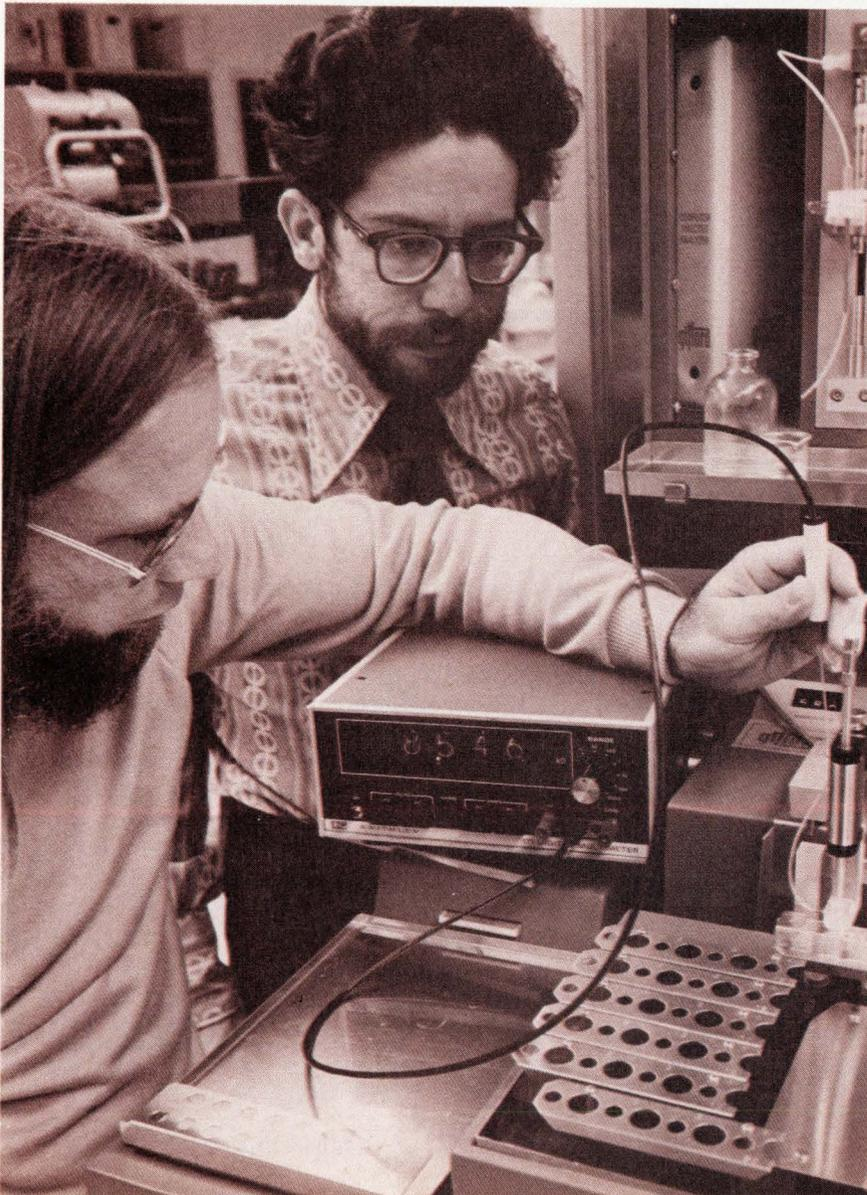
**Readout in action.** Author watches as Stephen Douglass of Gilford Instrument Laboratories uses an ac-dc digital multimeter and a precision thermistor probe to verify temperature control calibration in a computer-directed analyzer. The system performs analytical chemical analysis by measuring reaction rates and final light absorbancy, both of which are temperature-dependent.
