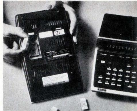
Sharp Electronics' model PC-1002 calculator is a scientific unit with four extra function keys that the user can define by plugging in the appropriate programmable read-only memory. With different PROMs, the functions of the special keys are changed, converting the calculator to any application the user needs.
