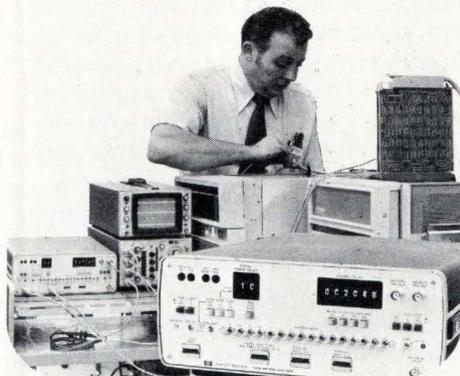
Troubleshooting a disc is a typical application for the new 1620A digital analyzer that scans parallel or serial bit patterns at rates up to 20 MHz.
