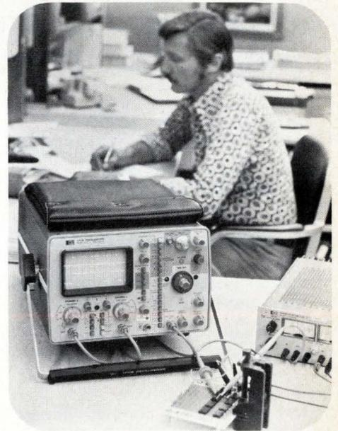
Accuracy and environmental specifications make either the 1710B scope (shown here) or the 1720A model equally suitable for bench use or field service.
