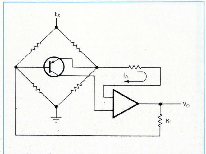
**2. Feedback.** Bridge circuit operates sensing transistor (a selected 2N2484) at a constant current so that its  $V_{BE}$  is a linear function of absolute temperature. Op amp is usually an LM-308.
