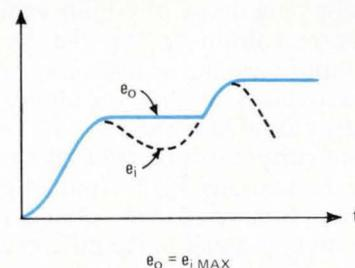
**1. Sample, then hold.** To store peak signal levels an op amp is connected in the manner of a voltage follower that supplies charging current to a capacitor. A rising voltage forward biases  $D_1$  to engender the voltage follower that impresses the increased level on  $C_H$ . A falling voltage reverse biases  $D_1$  so the voltage on  $C_H$  remains where it is.
