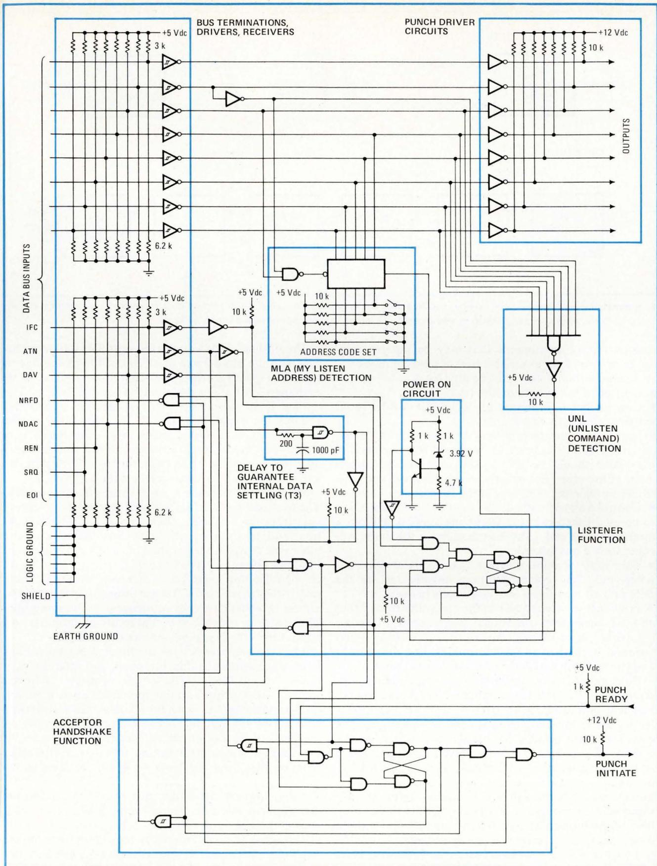
**7. Design.** Because of the simplicity of a tape-punch interface, standard TTL integrated circuits were chosen to implement the design. The class of devices that take digital data and convert it to some other form may make use of similar circuitry.
