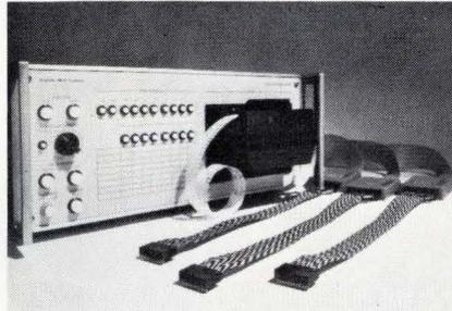
simulate the ROM's in your system. The ROM Simulator interconnects directly to your hardware by means of 16- or 24-pin DIP connectors. It will simulate any of the standard PROM's and ROM's available today. And with its 100ns access time, you can debug your system in real time.
