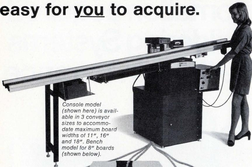
Console model (shown here) is available in 3 conveyor sizes to accommodate maximum board widths of 11", 16" and 18". Bench model for 8" boards (shown below).
