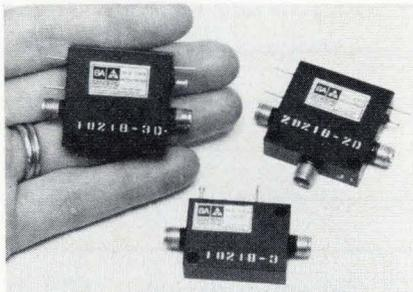
18 gigahertz yields greater than 50-dB isolation with 2.5-dB maximum loss, and it switches in less than 25 nanoseconds (50% TTL to 90% rf). Standard units handle up to 5 watts cw in a package 1.2 by 1.1 by 0.38 inch with SMA connectors. Series DS10000 and DS20000 diode switches are priced as low as \$195,
