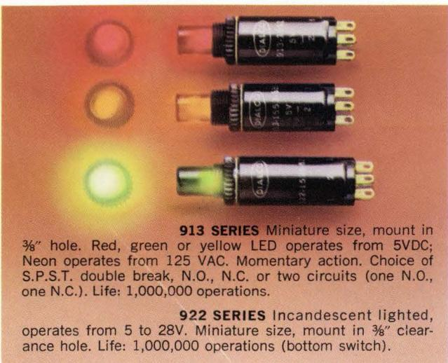
**913 SERIES** Miniature size, mount in 3/8" hole. Red, green or yellow LED operates from 5VDC; Neon operates from 125 VAC. Momentary action. Choice of S.P.S.T. double break, N.O., N.C. or two circuits (one N.O., one N.C.). Life: 1,000,000 operations.
