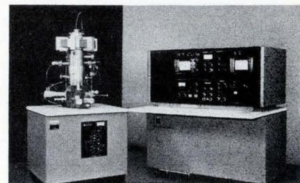
type specimen stage, and modular construction for easy addition of plug-in accessories. Twenty-six optional accessories are available, including a display unit for simultaneous dual magnification, a TV scanning device, and an energy-dispersive X-ray analyzer.
