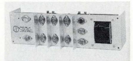
competitive models. Input is 105-125 v ac, 60 Hz. Line regulation is 0.01%, load regulation 0.02% and output ripple 1.5 mV, peak-to-peak maximum. Transient response is 30 microseconds for 50% load change. Other models at 12, 15, 24, and 28 v are available. Price is \$149.
