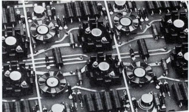
**Temperature matching at varying power levels** is easy with the wide variety of IERC dissipators. On this board problem was to keep TO-5s at approximately equal case temperatures although some were operated at 2.2 watts and others at 1 watt. Press-on Fan Tops costing pennies kept 1 watters at 55°C case rise above ambient while LP dissipators held 2.2-watt devices at nearly identical case temperatures. IERC Insulube® coating permits mounting LPs directly on printed circuit lines.
