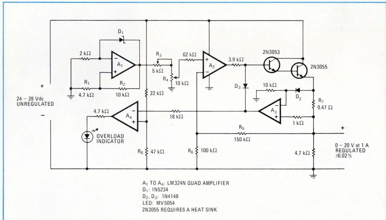
**Op amp regulator.** An unregulated 26-volt source becomes a 1-ampere 0-to-20-V supply regulated to within  $\pm 0.02\%$  by a simple quad operational amplifier. Input can vary between 24 V and 28 V, and quiescent current is less than 10 mA. A light-emitting diode gives an overload indication, the level of which depends on the value of resistor  $R_8$ . Single power Darlington can replace the two transistors.
