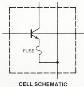
Our prices are low because Intel has always used Schottky and polysilicon technologies for high volume memory production. We fabricate the fuses with our standard silicon gate MOS process and make the rest of the PROM with our standard Schottky bipolar technology, also used for our compatible metal mask ROMs.
