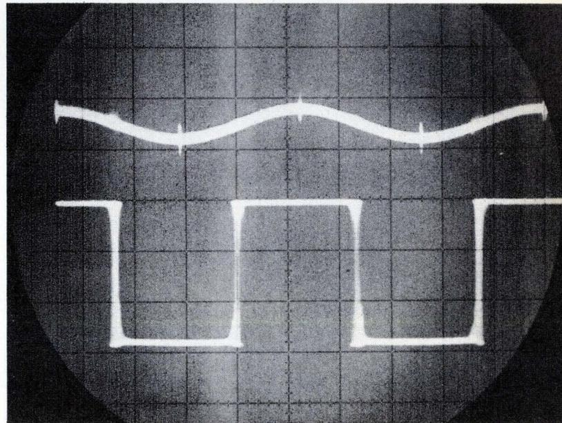
**3. Result.** In this trace, the horizontal scale is 200 microseconds per division. Vertical scales are 500 microvolts per division for input (top), and 5 volts per division for output.
