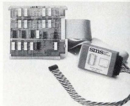
programs. These modules bring to 14 the number available to users of the simulator, called the model 1000A. The simulation options range from organizations of 256 by 4 bits to 1,024 by 4 bits and are priced from \$395 to \$795. The modules have a maximum access time of 100 ns. Microprogram-based systems are in the prototype stage.
