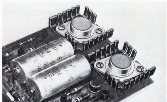
**Lower cost per unit** was result of replacing four TO-3s used in this 10-watt power supply with two TO-3s in UP3 dissipators. Dissipators allow two TO-3s to operate at 5 watts each with same 65°C case rise above ambient as four devices operated at 2.5 watts each. Low profile dissipators plus TO-3s were assembled in less space allotted to four transistors. New design saved money, improved reliability and eliminated troublesome charring of G-10 board.
