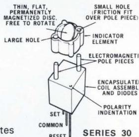
Ferranti-Packard's status indicators are light weight (Series 30, 0.17 oz (5 grams)) and are ideal for mounting on printed circuit boards and high density matrices.
