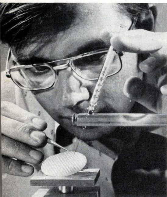
Conventional test equipment can determine whether an IC is functioning properly, but these tests may be of little value in determining exactly why and where an IC has failed. To solve this problem, scientists at the RCA Physical Electronics Research Laboratory in Princeton, N.J., say they have developed a nondestructive technique that enables both the electric fields and temperature distributions at the surface of an operating IC to be viewed through conventional optical microscopes.
