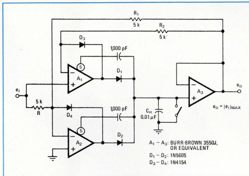
**6. Absolute magnitude.** A magnitude peak detector is put together in the fairly simplified combination of a positive peak detector and an inverting negative peak detector.  $A_1$  and  $A_3$  form the positive peak detector,  $A_2$  and  $A_3$  form the negative peak detector. The largest peak, either positive or negative, appears as output  $e_o$ .
