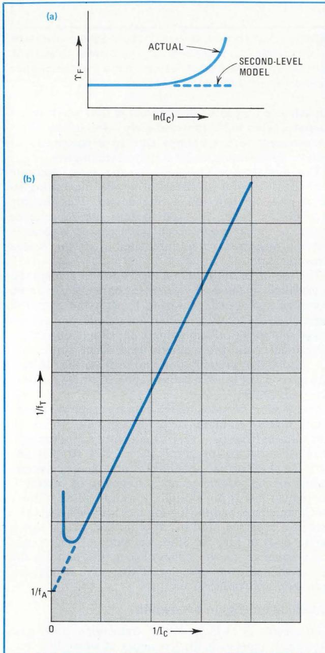
**7. Forward transit time.** For the second-level Ebers-Moll model, the total forward transit time,  $\tau_F$ , is assumed to be constant, although it does vary with collector current, as indicated in (a). Generally,  $\tau_F$  is computed from the measured value of the unity-gain bandwidth,  $f_T$ . But if there is no quasi-constant  $f_T$  region, an appropriate  $f_T$  value can be found graphically from a plot (b) of  $1/f_T$  vs  $1/I_C$ .
