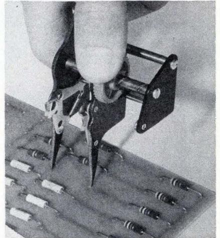
curately for insertion in printed-circuit boards. Function of the screw, which is permanently dry-lubricated for improved reliability, is smoother micrometer-type adjustment of bend spacing. Operating precision and efficiency are said to be increased. Standard features include strain relief between component and bend, replaceable plastic guides, and rigid hard anodized aluminum frame. The model N-300 costs \$32.50 and is available from stock.
