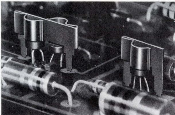
**Dissipators protect circuit** — Designer of this TV circuit made sure dissipators would stay when D-case devices needed replacing. He designed dissipators as a part of the circuit, making it impossible to fire the circuit without them. In addition to this circuit protection the dual "Universals" gave him some other benefits: excellent retention in shock/vibration environments, good heat sinking during solder operations, and they cost just pennies.
