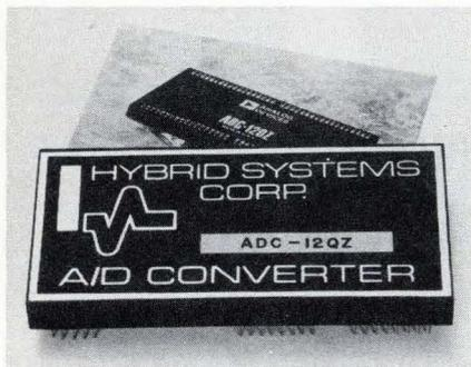
ferential nonlinearity temperature coefficient of  $\pm 2 \text{ ppm}/^\circ\text{C}$ . The model ADC-12QZ is intended to replace an a-d converter being supplied by Analog Devices of Norwood, Mass. The two devices are identical except for their differential nonlinearity temperature coefficient, which is lower for the Hybrid Systems unit.
