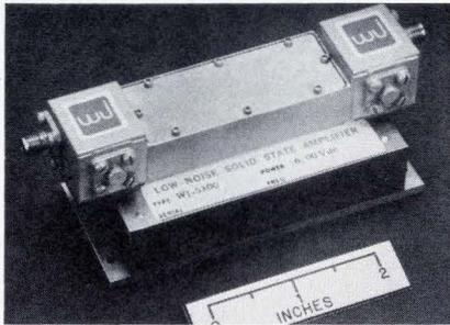
5300 series include: frequency of 7.25 or 8.4 gigahertz or 8 to 10 GHz, noise figure of 6.0 dB or 7.5 dB, small-signal gain of 30 dB or 27 dB, output power of +5 dBm or +6 dBm, and gain flatness of  $\pm 0.5$  dB or  $\pm 1$  dB.
