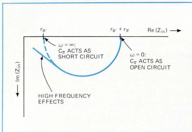
**2. For small-signal analyses.** The base resistance ( $r_{B'}$ ) of the second-level linear hybrid-model can be determined from a complex-impedance plot. As the signal frequency is varied, the real and imaginary parts of the input impedance of the base-emitter junction are measured. The intercepts of the resulting semicircle with the real axis yield the  $r_{B'}$  value, which can vary from ohms to kilohms.
