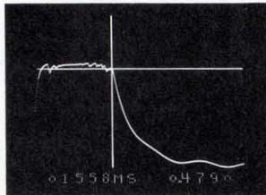
So you can closely inspect any particularly interesting portion of your signal the 1090 offers expansion of the stored waveform up to 64 times on both X and Y axes revealing selected detail of the 4096 x 12-bit word memory.
