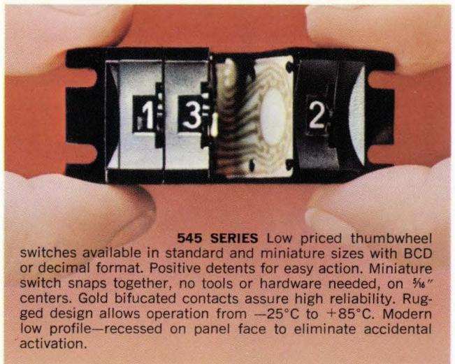
**545 SERIES** Low priced thumbwheel switches available in standard and miniature sizes with BCD or decimal format. Positive detents for easy action. Miniature switch snaps together, no tools or hardware needed, on 5/16" centers. Gold bifurcated contacts assure high reliability. Rugged design allows operation from -25°C to +85°C. Modern low profile—recessed on panel face to eliminate accidental activation.
