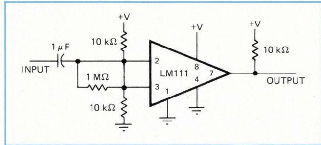
**1. Conventional.** Input offset limits the utility of the comparator when used as a clipper; it won't work with very small signals.
