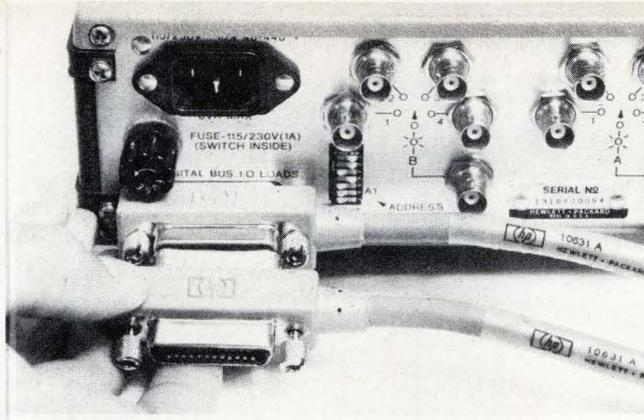
**2. Connector.** Cables used with the interface system have dual male-female connectors at each end so that they can be stacked, thus allowing more than one cable to be attached to any instrument. This permits either star or daisy-chain configurations.
