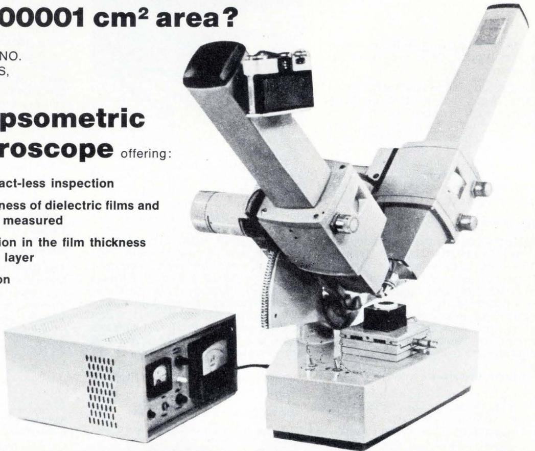
The LEM-2 is the first means to measure the thickness of dielectric films in mini-size "ports" in protective layers employed in planar techniques of production of integral circuits and individual semiconductor devices
