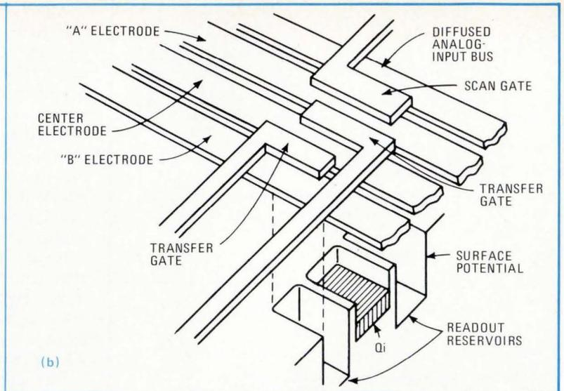
**5. Making a transfer.** In a charge-transfer device, readout of each charge sample is independently controlled by the voltage on the transfer gate of the cell. Readout is achieved when the gate voltage is sufficiently above a fixed threshold and when a signal proportional to the magnitude of the charge is induced by means of ac coupling in either "A" or "B" output circuit.
