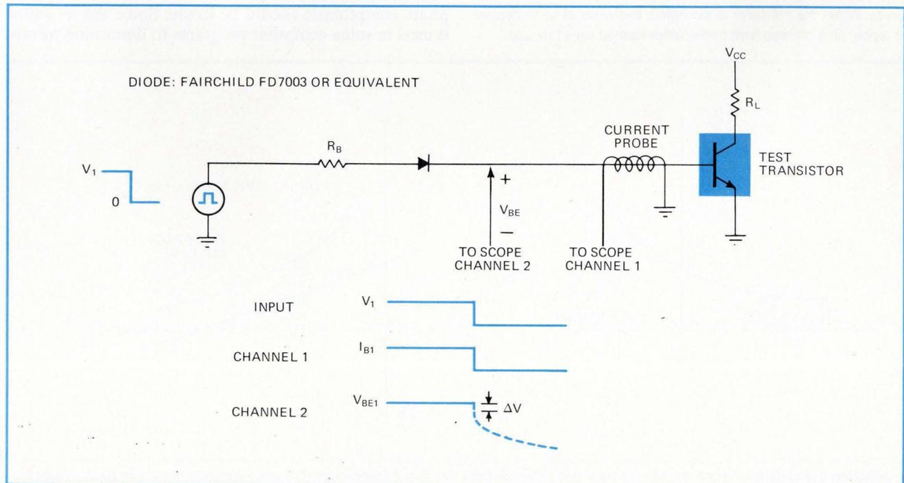
**3. For switching applications.** This pulse measurement scheme is best for determining base resistance  $r_{B'}$  when the transistor is to be used as a switching device. The voltage drop ( $\Delta V$ ) across  $r_{B'}$  is observed as the transistor turns off. Then:  $r_{B'} = \Delta V/I_{B1}$ .
