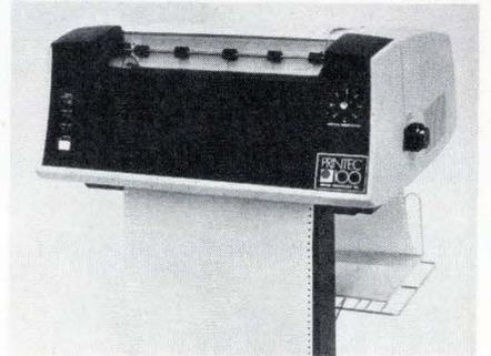
valuable in systems that combine CRT terminals and printers on one line. Since the interface contains a 1,024-character buffer, a Printec-100 can be printing a message while other terminals are being serviced by the computer. Price of the interface, complete with a Printec-100, is \$4,650.
