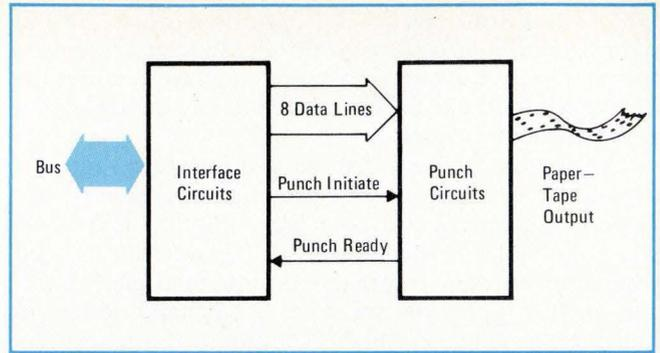
**6. Punch.** As shown by its block diagram, a tape punch can be partitioned into the punch circuits that will enable it to perform its functions as an instrument and the interface circuits that are necessary to connect it to the data bus.
