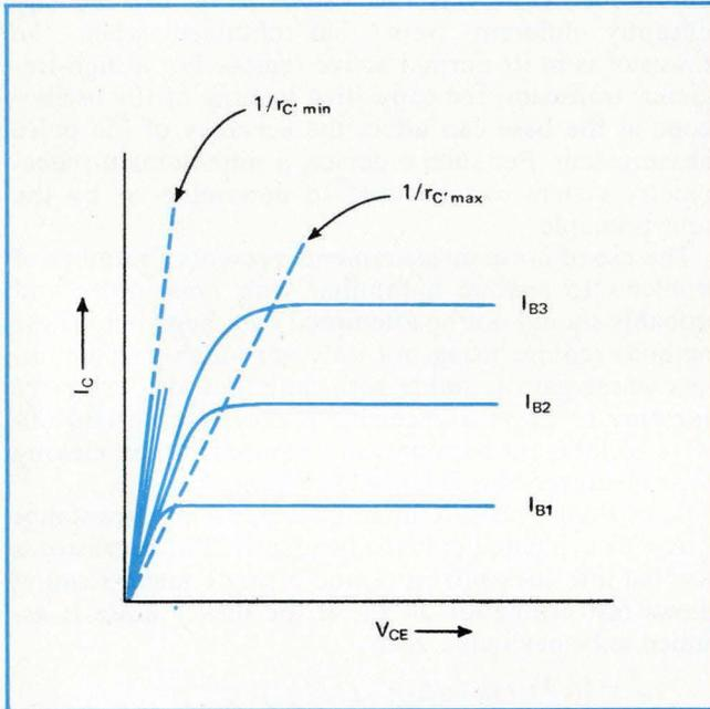
**4. Collector resistance.** The value of resistance  $r_C'$  can range from a few ohms to hundreds of ohms. It is measured by displaying the collector characteristics. In the normal active region,  $r_C'$  is the inverse slope of the dashed line ( $1/r_C'_{max}$ ) through the knees of the curves. When the transistor is saturated, the value of  $r_C'$  increases. Its upper limit is noted here by the other dashed line ( $1/r_C'_{min}$ ).
