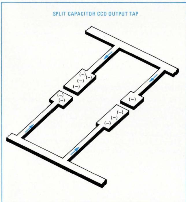
**3. Weighty.** The correct weighted output at each tap can be obtained by simply splitting the electrode at that position so that a fixed quantity of signal is detected. Summing all such taps produces the desired signal transformation.
