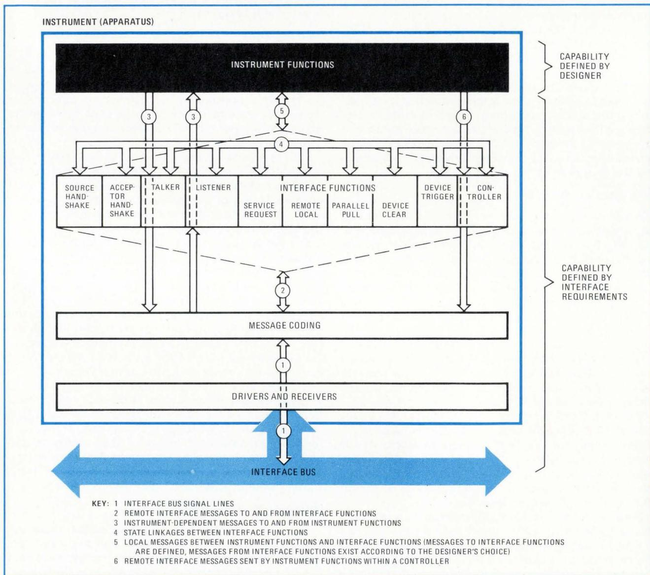
**4. Partition.** Instrument designs can be conceptualized as being partitioned into two areas: instrument functions and interface functions. But this division does not necessarily imply two separate physical layouts within the instrument.
