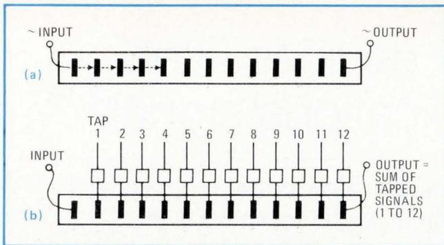
**2. The basic delay line.** A simple charge-transfer device (a) acts as a delay line when a signal is passed along from element to element and detected at the output. For signal processing, the a weighted signal is collected along the way (b) to form a summed output corresponding to a particular analog-signal transformation.
