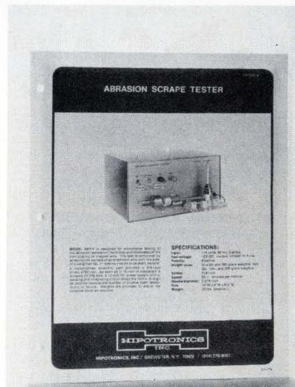
acceptance testing of the abrasion resistance (hardness and thickness) of the film coating on magnet wire is described in a technical bulletin available from Hipotronics Inc.,
