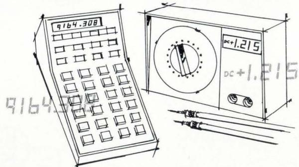
**Conclusion.** In the majority of display applications, MOS and C/MOS compatibility, reliability, flexibility and low power requirements are important considerations. No other display can match the liquid crystal display on these jobs. They could be the display of the future.
