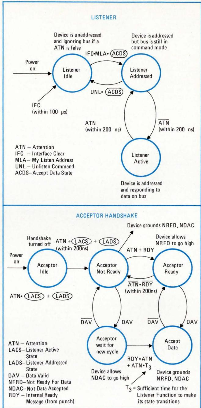
5. States. One way of looking at an instrument's interaction with the data bus is to use state diagrams like the two shown here for any listener tied to the bus (above) and for a listener in the process of receiving data and handshaking with a talker (below).
