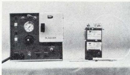
matograph. A worker wears only the first two items—the collector column on his collar, and the sample pump on his belt. After a period of time, the collector column is detached and placed in the flasher assembly, which is connected to the chromatograph. The flasher assembly heats the column and causes the collected sample to be passed through the chromatograph where it is analyzed in a matter of minutes.
