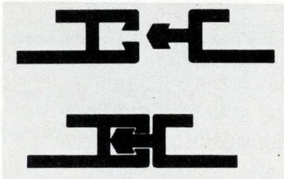
The tubing is supplied in flat, open form and can be wrapped around existing installations without re-wiring—an especially convenient feature when splices are required.
