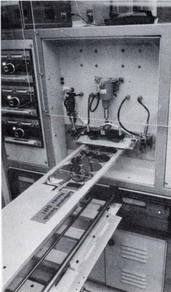
**5. Reactor.** The forklift inserts the boat into the epitaxial reactor. In production, any number of reactors can be loaded and unloaded by the forklift simply by extending the track, but Motorola expects that larger capacity models will become available within the next year—an arrangement that is better than the use of many small reactors.
