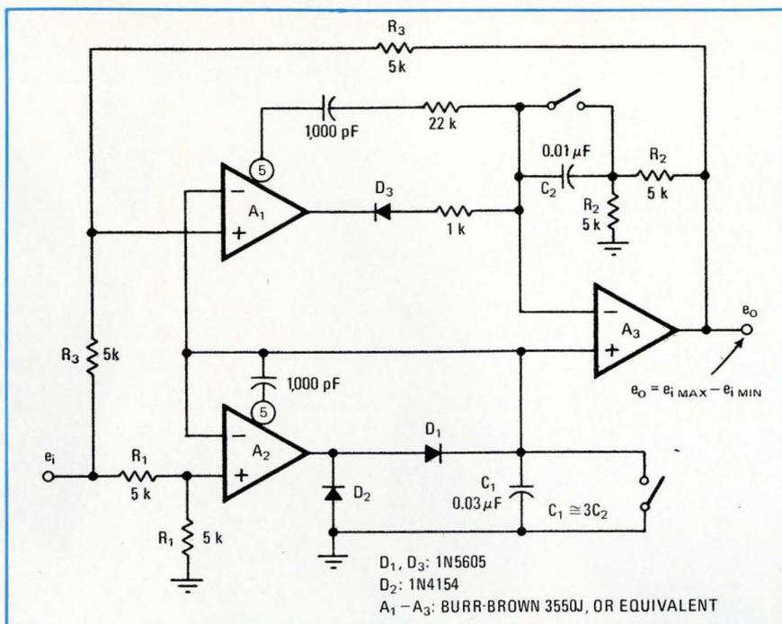
**5. Peak-to-peak.** A simplified peak-to-peak detector is formed by combining two simple peak detectors. A positive peak detector is formed by  $A_2$  and  $A_3$ , and a negative peak detector by  $A_1$  and  $A_3$ . Op amp  $A_3$  sums the peaks, positive and negative.
