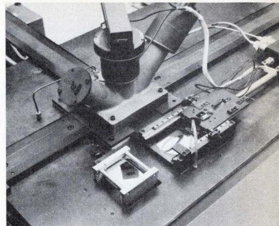
**3. Inspection.** From cleaner, wafers move individually to inspection, right. Defects reflect bright light to phototransistor sensors; defect data is recorded to help monitor cleaning operation. Defective wafers go back to cleaner, good ones move to next step.
