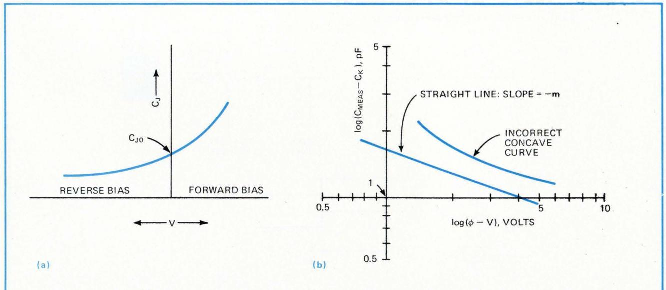
**5. Junction capacitances.** Both the emitter-base and collector-base junction capacitances ( $C_J$ ) are a function of their respective junction voltage ( $V$ ), as shown in (a). These two capacitances can be measured with a bridge, but the extra capacitance ( $C_K$ ), mainly caused by pin, stray, and pad capacitances, must be accounted for. A graphical method for reducing the measured capacitance ( $C_{MEAS}$ ) is given in (b).
