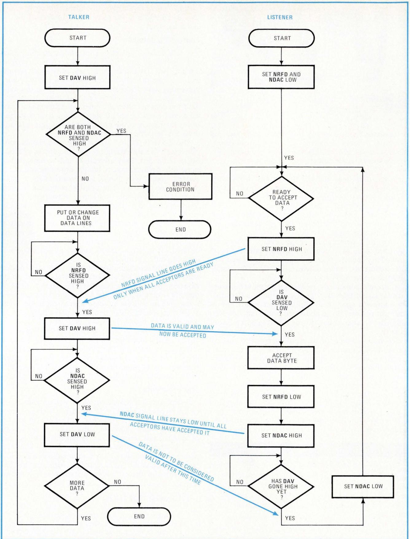
**3. Handshake.** To ensure that data is properly transferred, this handshaking procedure must be performed every time a talker sends data to a listener or listeners. The DAV line is controlled by the talker, NRFD and NDAC by the listeners.
