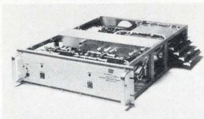
a 5-megahertz reference standard. The series of stabilizers provide discrete stabilization at frequencies from 1 to 40 gigahertz. With the automatic-lock option, these are suited for unattended or dedicated systems where maximum reliability is required.
