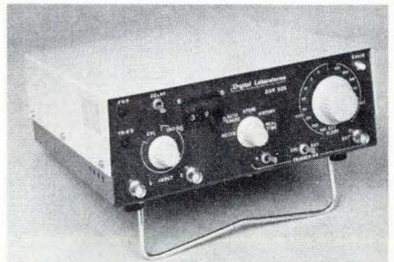
more expensive analyzers, the DSR-505 has adjustable "0" and "1" thresholds, can operate from its internal crystal-controlled clock or from an external timing signal, has a 10-MHz maximum sampling rate,
