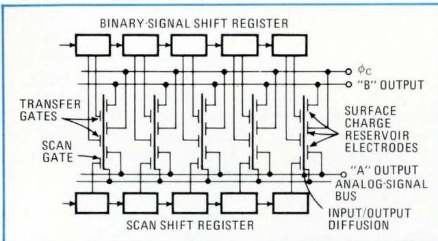
**6. Correlator.** In the CTD correlator chip, a binary reference word controls the polarity of the tap weight of a given charge sample. Two transfer gates control the direction of charge transfer. Charge samples assigned a positive weight are transferred toward one output line, while negative-weight samples go toward the other one.
