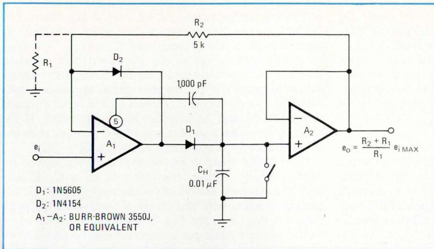
**3. Less error.** Improved output buffering, and peak detection gain greater than unity are achieved with an output voltage follower. The voltage follower replaces the FET buffer stage of the previous circuit, further reducing buffer error.
