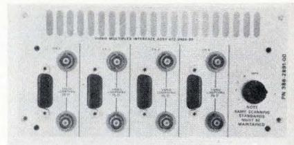
up to four standard composite signals, and from digital video signals of refreshed alphanumeric/graphic terminals. The unit allows the user to switch on any one of the four terminals for copying from a single one of them, and it also gives him the option of selecting a multiplex mode in which all four are copied in a four-channel queue. Price of the multiplexer, installed at the factory, is \$500. Price of the 4632 video hard-copy unit is \$3,395.
