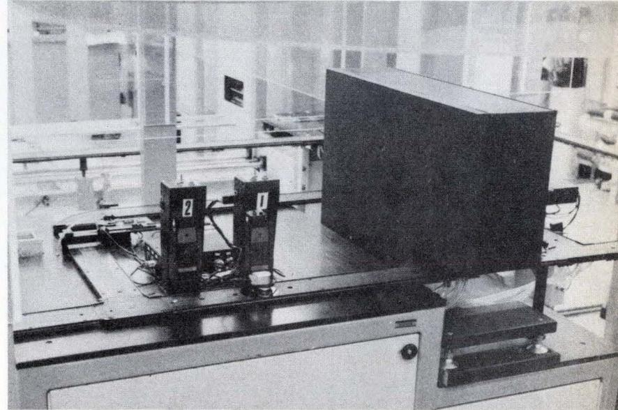
**6. Tests.** After leaving the warp detector, the wafers are visually inspected again. They then pass to stations that check the thickness and resistivity of the epitaxial layer. The units on left are four contact resistivity probes; at right is rapid-scan Michelson interferometer that checks thickness.
