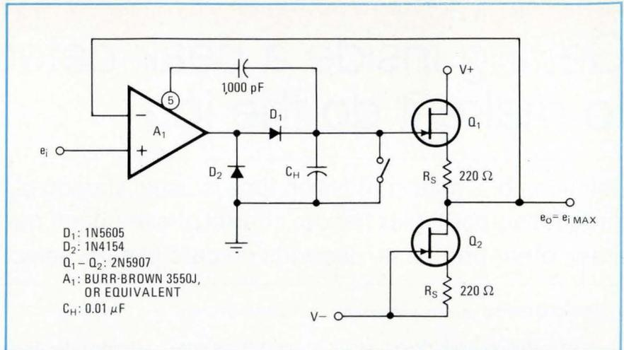
cant discharge between repetitive signal peaks, but will discharge the capacitor in the absence of signal.
