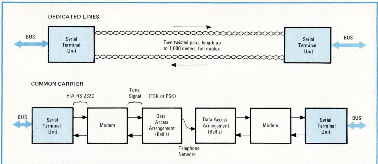
**8. Extension.** Serial terminal units may be used to extend the length of the data bus, either through dedicated lines or by common carrier. The units lower the cost of transmission by taking parallel data from the bus and converting it to serial form.
