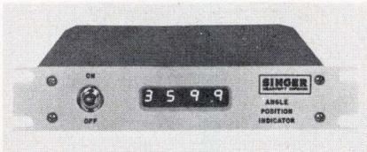
puts from 5 to 120 volts and from 50 to 1,000 hertz can be handled directly. The standard display ranges from 000.0 to 359.9°. Other special scales, such as  $\pm 180^\circ$ , are also available, as are BCD, binary or dc outputs.
