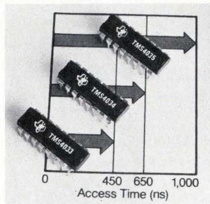
with the popular 2102-1, 2102-2, and 2102 RAMs, respectively, the TMS4033, TMS4034, and TMS4035 have respective access times of 450, 650, and 1,000 nanoseconds. Other features of the devices include full Series 74 TTL-compatibility, single 5-volt supply load, and three-state outputs for bus-driving capability. Delivery is from stock.
