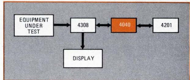
**Applications.** The 4040, with the 4308 ROM and the 4201 clock generator, could form a "smart" traffic controller (top), a preprocessor (middle), or a portable troubleshooter.
