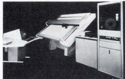
tem software allows the design engineer to make a preliminary drawing on a cathode-ray-tube display, look at the part from any angle, cross-hatch, zoom, rotate, window, insert fillets, add standard parts from a library, and define jigs and motions for numerically controlled tools. Data can also be formatted for design analysis and simulation.
