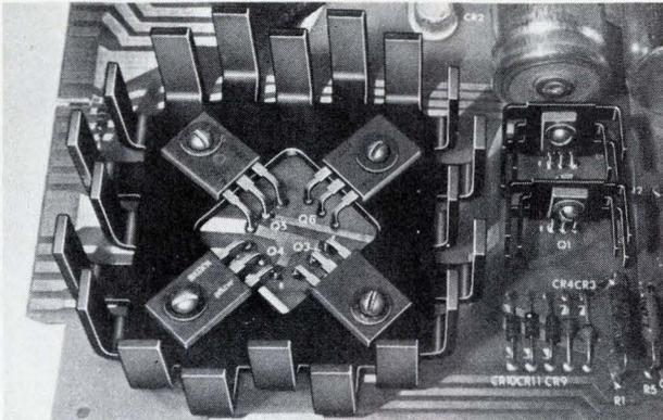
**Four times the power** from four power plastics took just one IERC dissipator. Bare transistors were capable of only 2 watts with 102°C substrate rise above ambient so designer used modified HP3 dissipator and got 8 watts from each at the same temperature rise. Or you could improve transistor life — roughly 7 times — by operating the devices at 2 watts and letting the same dissipator keep the substrate temperature rise to 32°.
