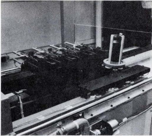
**2. Cleaner.** At this station, left, wafers are loaded in carriage. Modified LFE plasma cleaner then moves over the carriage to clean the wafers. LFE system is only commercial equipment in the entire Motorola epitaxial setup.
