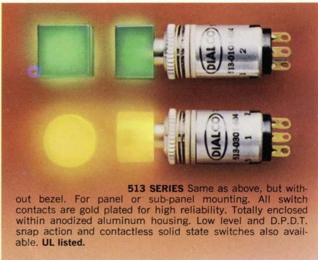
**513 SERIES** Same as above, but without bezel. For panel or sub-panel mounting. All switch contacts are gold plated for high reliability. Totally enclosed within anodized aluminum housing. Low level and D.P.D.T. snap action and contactless solid state switches also available. **UL listed.**
