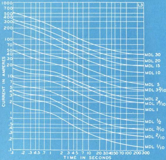
Time-current characteristics of BUSS® fast-acting fuses
