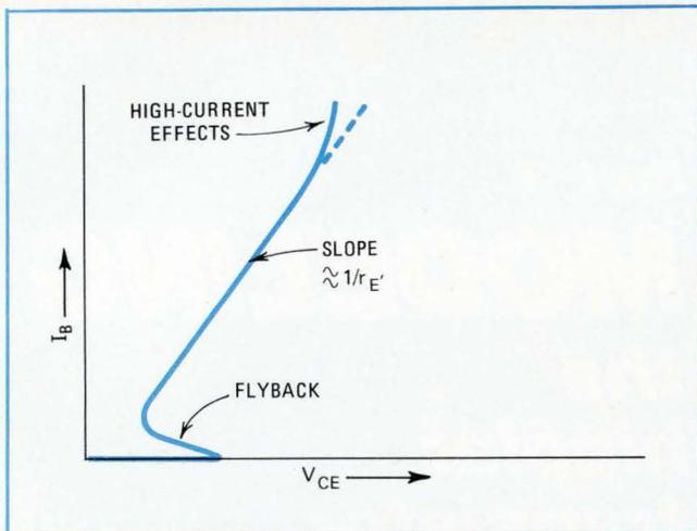
**1. Emitter resistance.** Constant value of emitter resistance ( $r_{E'}$ ) is obtained from a display of base current ( $I_B$ ) as a function of collector-emitter voltage ( $V_{CE}$ ). The  $r_{E'}$  value, typically around 1 ohm, is the inverse slope of this display at low currents.
