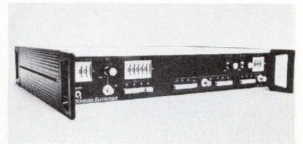
in the range from 0.001 hertz to 10 kilohertz and 40 time steps up to 100 kHz. Crystal-controlled frequency stability is  $10^{-6}$ /degree, resolution is  $10^{-5}$  of range, and signal linearity varies less than 0.5%. Price is \$995.
