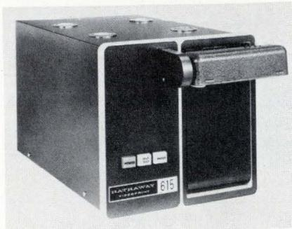
characters per second synchronously or asynchronously. The machine can link to computers, and the following logic levels or their complement are accepted: logic 1, +2.4 to +5 v and logic 0, 0.0 to +0.4 v.
