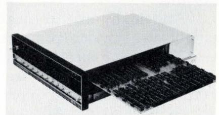
When used with a Nova 800, a 1,024 real-sample-time series can be transformed and the magnitude of the spectrum formed in 139 milliseconds. Time-domain signal-processing functions can be calculated at a rate of 2.8 microseconds per multiply-accumulate. Price is \$6,000.
