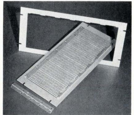
patible with standard 19- and 24-inch relay racks. The units are designated Swing Mount, and they can be used with boards, measuring 6.875 by 21.600 inches or 7.475 by 21.6000 in. in increments of 2.7 in. The frames are hinge-mounted and can be bolted to the rack.
