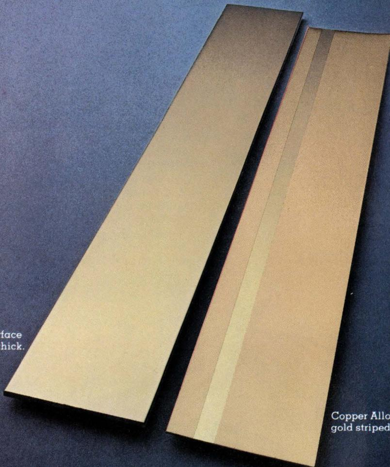
Copper Alloy 725, 3% of surface gold striped, 100 micro inches thick.
