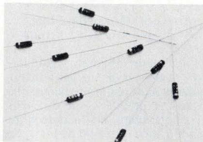
and inductance is rated at 2.5 nanohenries. The units are useful for applications in the uhf range. The hyperabrupt diodes also offer a Q of 400, measured at 50 MHz and 4 volts bias. Price is \$12 in 100-lots.
