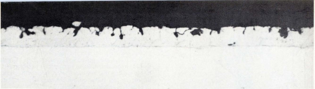
**2. Attacked.** One problem that tin plating can develop is the fretting corrosion shown here. The black tin-oxide inclusions, shown magnified 750 times, were driven deep into the tin plate by relative motion between this surface and an identical mating contact.
