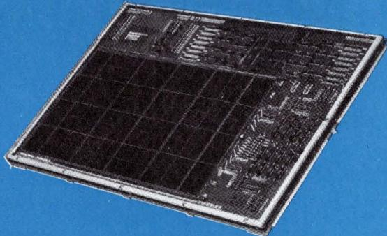
Basic module capacity of 32,768 words by 20 bits on a single card. Expandable to 64K, 128K, 256K or 512K by 10, 20 or 40 bits. Planar 3-D, 3-wire configuration measures 15 x 21.5 inches. Access time: 500 nanoseconds. Full cycle time: 1.2 microseconds. System options include: enclosures with printed circuit back panels, power supplies and test exerciser.
