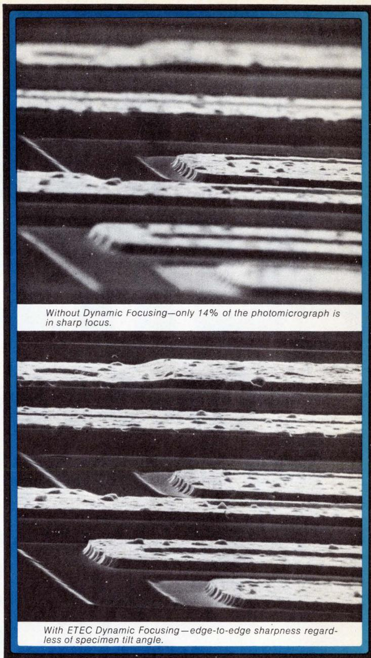
Without Dynamic Focusing—only 14% of the photomicrograph is in sharp focus.
