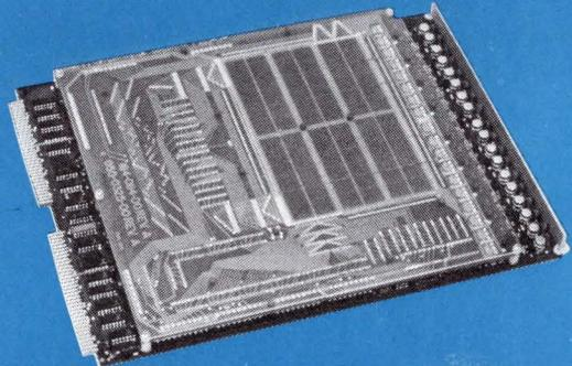
Basic module capacity of 8,192 words by 18 bits on a single card. Expandable to 32K, 64K or 128K by 9, 18 or 36 bits. Planar 3-D, 3-wire configuration measures 11.0 x 14.75 inches. Access time: 300 nanoseconds. Full cycle time: 650 nanoseconds. System options include: enclosures with printed circuit back panels, power supplies and test exerciser.
