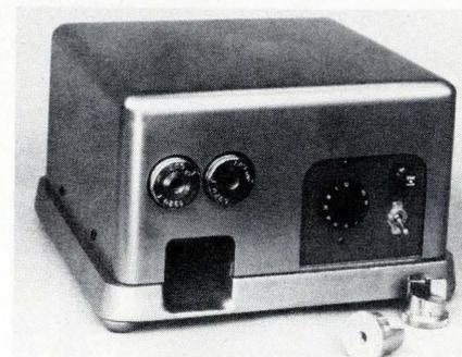
to 1,250 cables per hour, depending on the size of the cable. The trimming heads can be changed in less than 30 seconds to accommodate cable sizes, which can range up to 0.440 inch in outside diameter.
