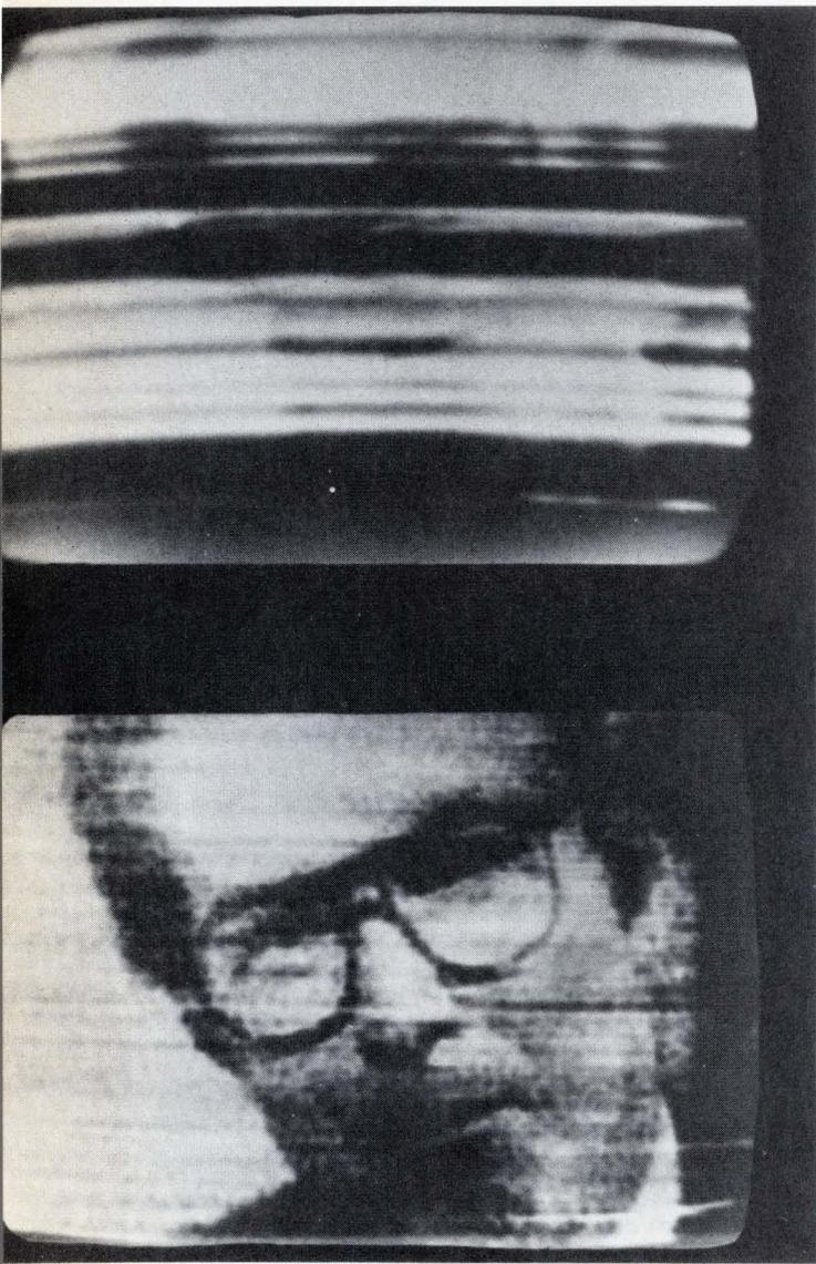
**1. Disk picture.** This TV picture is from the i/o Metrics video-disk system. The top is an unprocessed video signal and the bottom the video signal after clamping and a line-by-line AGC. Horizontal banding caused by encoding is not visible in normal viewing. The firm has negotiated with manufacturers to produce the system.
