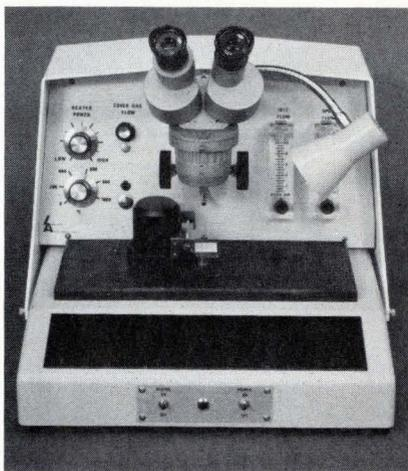
instead of the 5,000° hydrogen flames used in other spot bonders, eliminating water formation and leaching problems. With the HG720, an electrically heated, controlled stream of the hot gas is directed to the reverse side of the substrate, protecting the circuit side from solder-tip contamination, oxidation, and electrical transients, Price is \$1,300.
