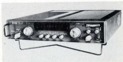
enced to a proportionally controlled master oscillator for a stability of  $\pm 1$  hertz at any frequency. Direct digital readout to the nearest hertz and tracked preselection are features of
