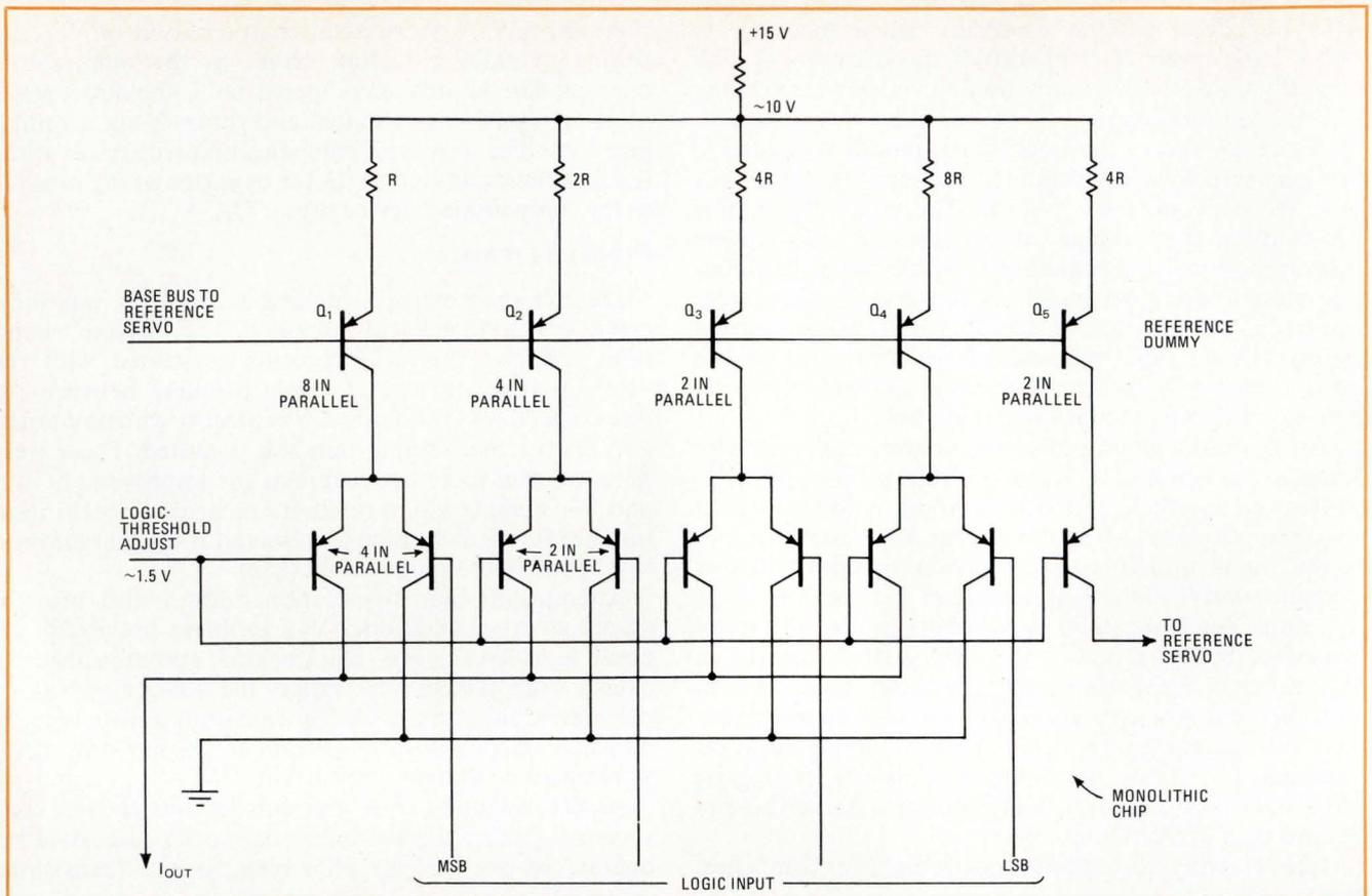
**6. Monolithic current-steering.** Current-source bit transistors  $Q_{1-4}$  operate continuously, while logic inputs switch currents from ground path to output line, thus avoiding thermal tails. Multiple transistors for each bit help assure base-emitter voltage-matching. A reference servo is also used in this circuit; it is not shown to minimize drawing complexity, but is similar to that in circuit of Fig. 5.
