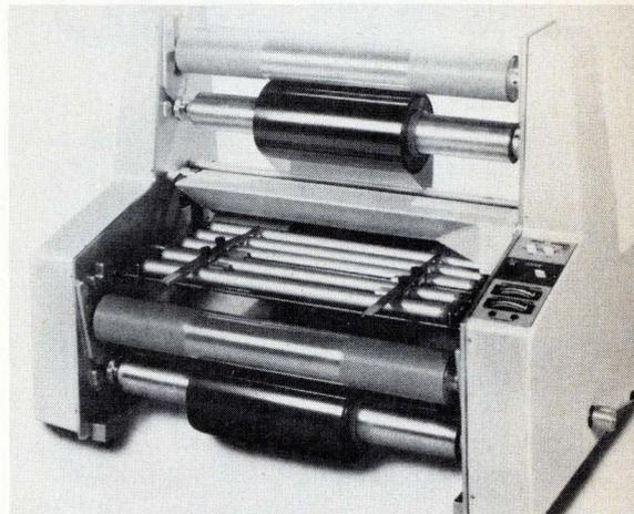
13 feet per minute. Normal working rate is 5 to 8 ft/min. By adding a 6-in. core adaptor, available as an option, 1,000-ft rolls of film can be accommodated.
