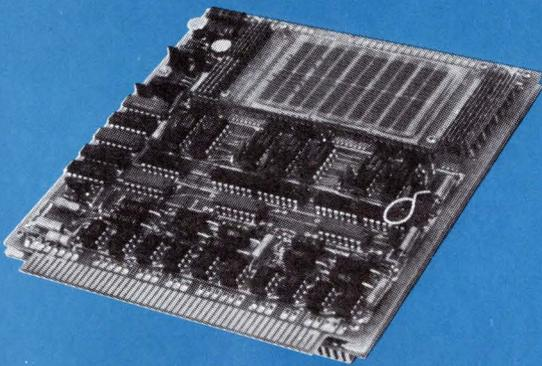
Capacity of 1,024 words by 10 bits on a single card. Planar 3-D, 4-wire configuration measures 6.0 x 6.4 inches. Expandable. Access time: 350 nanoseconds. Full cycle time: 1.0 usec.
