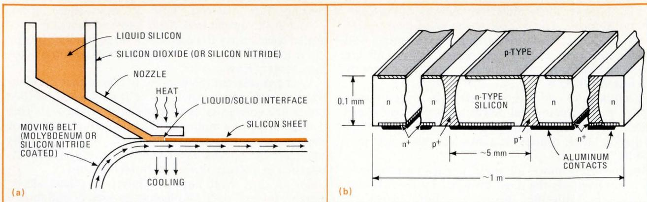
**4. Mass production.** The possibility of producing silicon in sheets at least a meter wide (left), is being considered by the University of Pennsylvania. Pn junctions could be diffused the length of the sheet, which could be processed sequentially at individual work stations.
