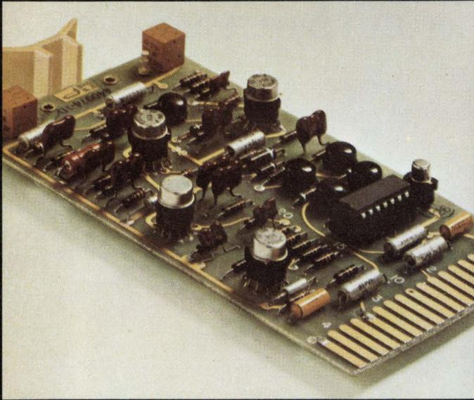
**level 1** Low-cost sockets for transistors in TO packages (above) allow easy replacement and service. ■ New IC sockets are end and side stackable for maximum single board density. Low profile design also allows maximum multi-board density.
