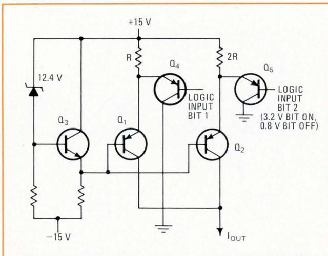
**3. Pnp-npn.** Replacing diodes of Fig. 2 with transistors eliminates diode storage times and thus raises speed, but this change does not affect problems of changing current gain and base-emitter voltages.
