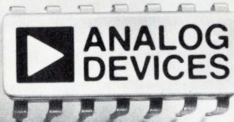
The first complete monolithic three-variable ( $V_0 = [V_{x1} - V_{x2}] [V_y] / V_z$ ) multiplier/divider. Perfect for rms-to-dc, AGC, vector summation. AD531.
