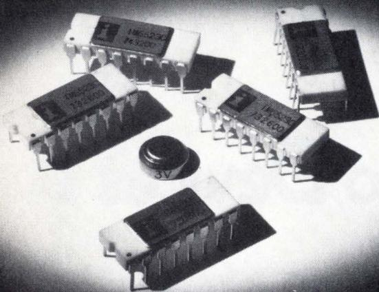
It's fully decoded and buffered, provides static asynchronous operation. Typical access time is 350 nanoseconds.
