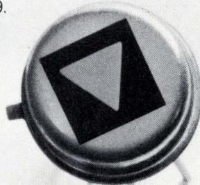
The first low drift ( $0.5\mu\text{V}/^\circ\text{C}$  max), low noise ( $0.6\mu\text{Vp-p}$  max) op amp with single-capacitor compensation and reasonable slewing rate. AD504.
