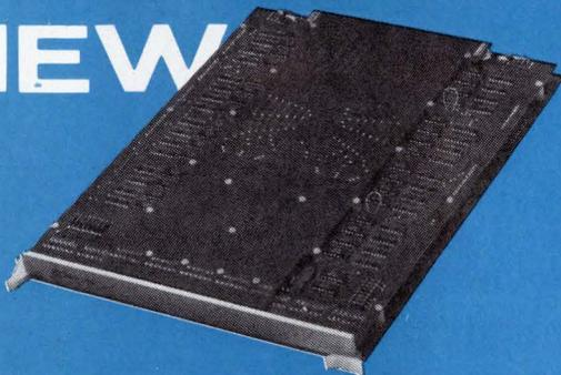
Basic module capacity of 16,384 words by 18 bits on a single card. Expandable to 64K, 128K or 128K by 9, 18 or 36 bits. Planar 3-D, 3-wire configuration measures 11.0 x 19.0 inches. Access time: 350 nanoseconds. Full cycle time: 750 nanoseconds. System options include: enclosures with printed circuit back panels, power supplies and test exerciser.
