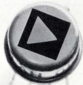
The first totally self-contained and internally trimmed monolithic multiplier,  $V_o = (V_{x1} \cdot V_{x2}) / (V_{y1} \cdot V_{y2}) / 10$ . AD532.
