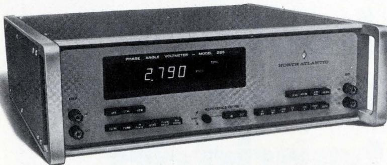
... This NEW DPAV provides complete analysis of complex AC waveforms at discrete frequencies and displays the results on a high readability 4½ digit display. Parameters measured are Total, Fundamental, In-Phase, and Quadrature voltage plus Phase Angle. Phase angle is displayed directly in degrees from 0° to 360° with a resolution of 0.1°.
