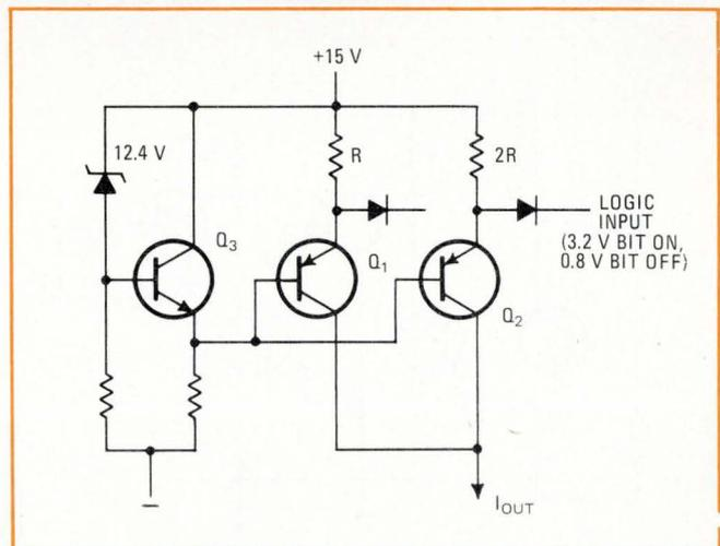
**2. Diode-pnp.** Nearly a mirror image of the circuit in Fig. 1, this circuit provides compatibility with TTL logic inputs, but it still shows the same deficiencies in compensating for changes in transistor-current gains and base-emitter voltages.
