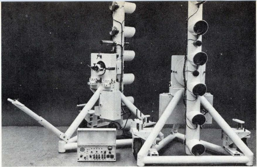
**Intruder detector.** Laser fence has six devices in vertical row. Their beams are picked up by optical receiver. Small instrument is local collector/display unit of the system.
