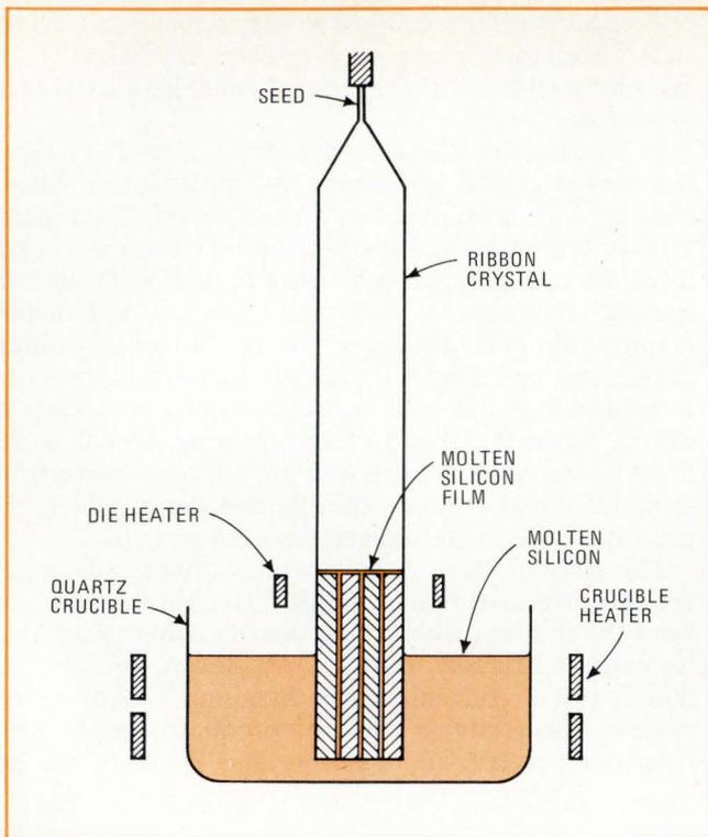
**5. Another way.** Ribbon-growing method at Tyco Laboratories entails pulling single-crystal silicon from melt through die. So far, inch-wide ribbons 18 inches long have been formed.
