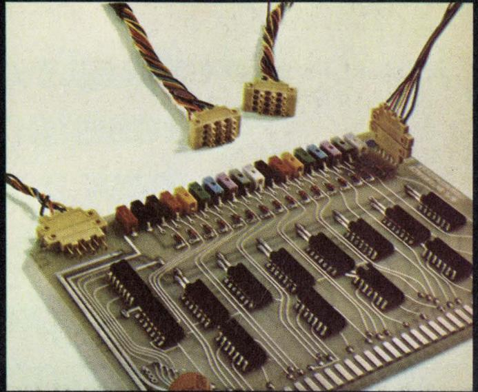
**level 4** Miniature contact (3 input, 3 output) hermaphroditic connectors can be snapped together to connect as many circuits as required. ■ Single finger-tip mounting of low cost connector saves assembly time. Available in UL Class SE-1 flammability rated material.
