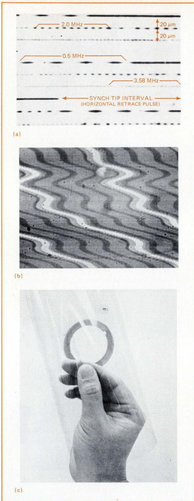
**4. Setting records.** Phase-contrast microphoto of the disk surface (a) shows the standard multiburst test video signal and the sync-tip interval (horizontal retrace pulse). At a lower magnification (b), it's possible to see the separate color bars and individual record tracks. One important advantage of the film disk (c) is that it can be handled without harming the recorded information.
