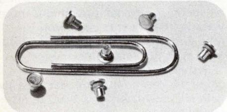
These developmental diodes have operating voltages from 100 to 143V, with operating current from 50 to 900 mA, depending upon frequency and power output.
