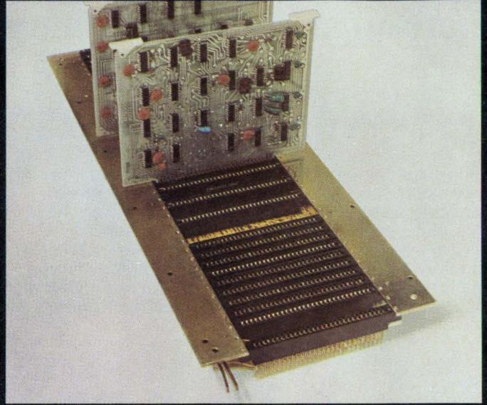
**level 2** Back panel edge board connectors with bifurcated contacts (above) can be wire wrapped or clip-terminated. ■ Bellows contact PC connectors (below) cut interconnection costs without sacrificing performance.
