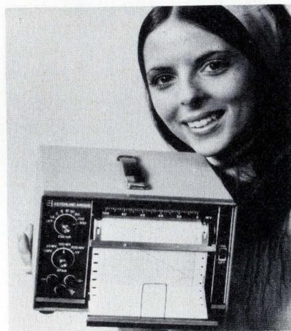
1 volt. Single range to 1 millivolt, single-speed thermocouple and thermistor ranges are optional. In addition, full-scale zero can be adjusted with a screwdriver, and the leads connect to the front or back. Price is \$349 or \$484, depending on the range.
