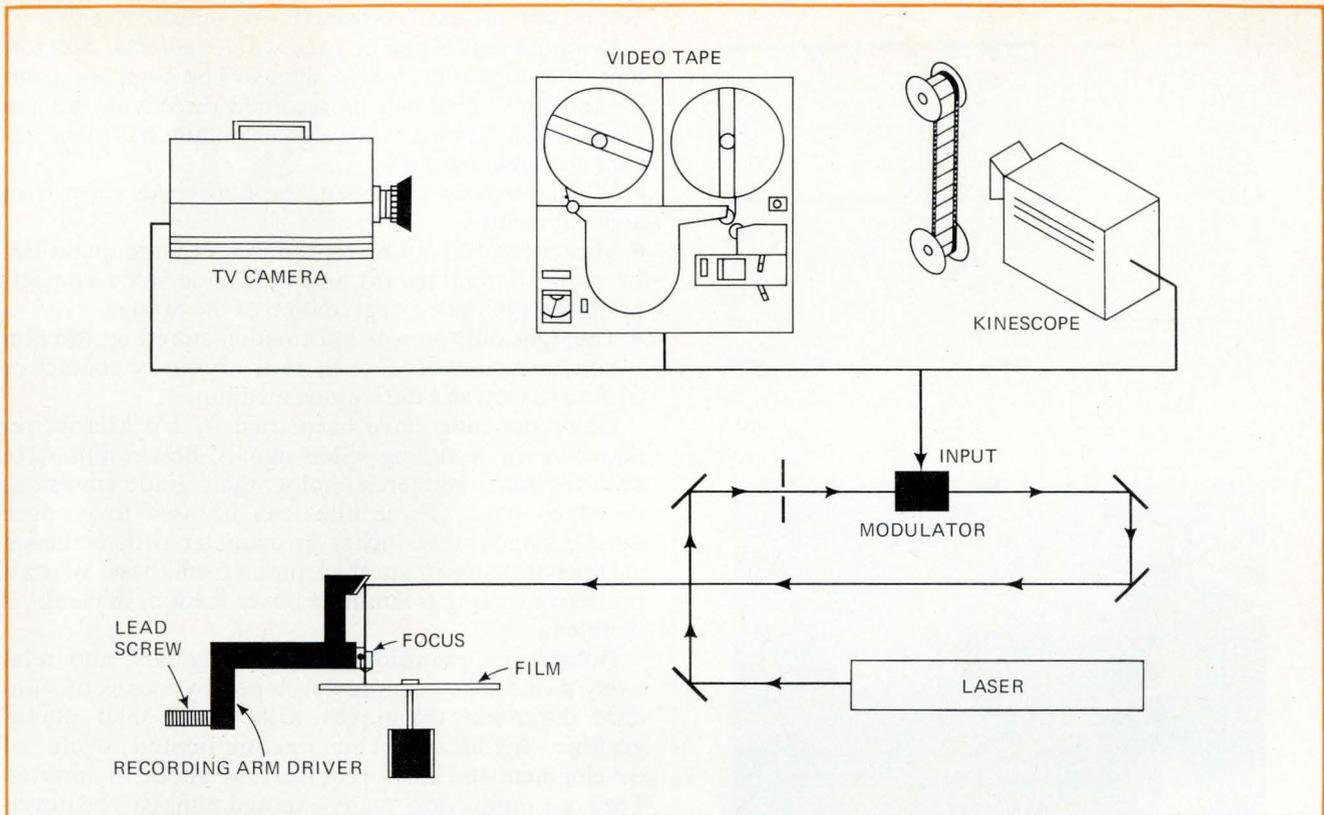
**2. Recording.** Any video medium, TV camera, tape, or kinescope, can be recorded on the film disk by using a helium-neon laser. The light beam, modulated with the video signal, is delivered to the turntable by mirrors aimed to pass through a focusing device.
