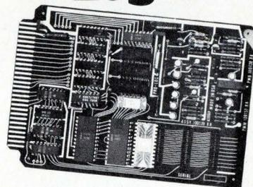
Our 4-bit microprocessor system can replace a rack full of your TTL chips. You'll save design time and production costs. No big redesign jobs for options or changes because the logic is stored in reprogrammable ROMs. Our programmed logic systems are available now, off the shelf.
