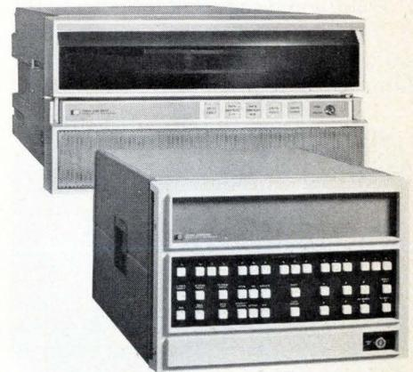
The 2123A OEM disc-based system has a data transfer rate of over a million 16-bit words per second.
