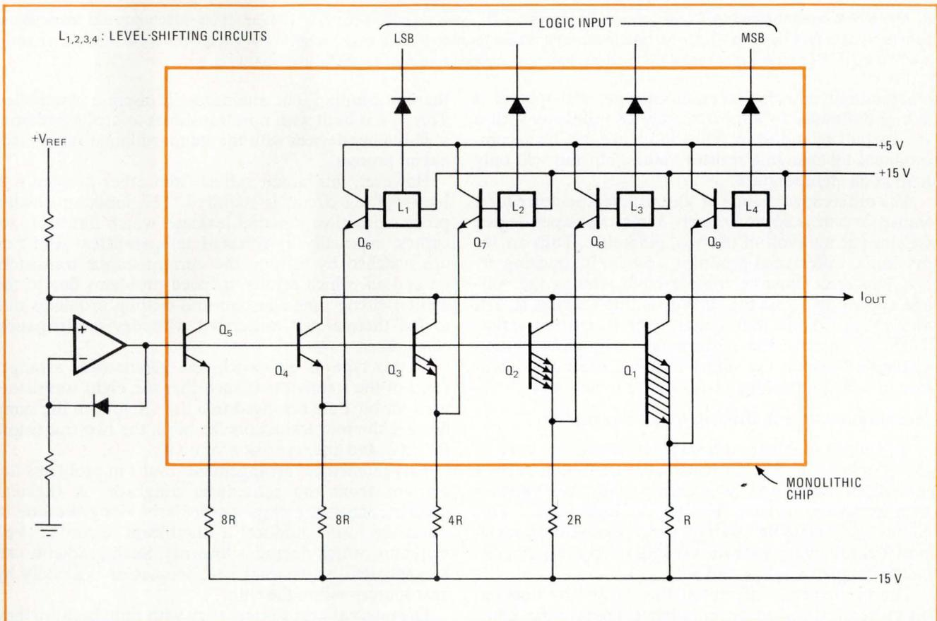
**5. Monolithic npn.** Paralleled transistors in the bit switches assure similar currents through each device and thus similar base-emitter voltages. However, use of npn transistors requires level-shifting circuits ( $L_{1-4}$ ) to work with TTL inputs. Also, switching is done directly on current-source transistors, which introduces thermal-stabilization problems (thermal tails), as in the discrete-component circuits.
