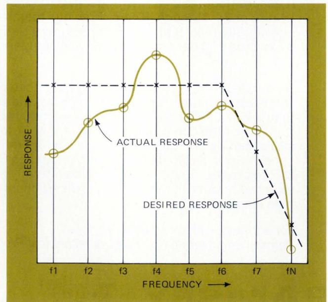
**1. The optimization process.** Magic optimizes a circuit design by minimizing a weighted error function that represents the difference between the desired response and the actual response. Optimization is done only at the frequencies specified by the user.
