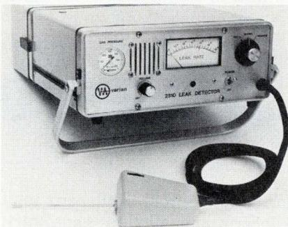
Bantam requires no tuning, calibration, or peaking when used in its search mode. Further, the new detector spans a six-decade range—from  $10^{-8}$  cc/s to  $10^{-2}$  cc/s—without any switching or other adjustment.
