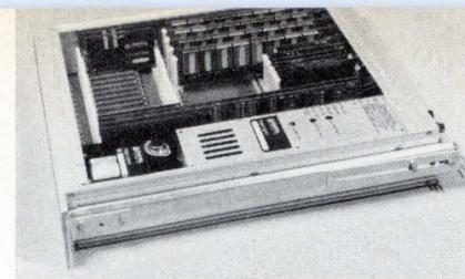
tors at a 50-kilohertz rate in about 1 ms. All 64 channels can be cycled every 5.5 ms, allowing for reed-switch signal-acquisition time, settling, and conversion. Both the controller and multiplexer are C-MOS devices, so power dissipation is low, about 70 watts from an ac line.
