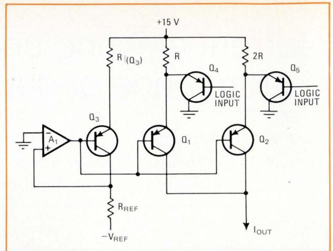
**4. Adding a reference servo.** Addition of an operational amplifier helps to compensate for changing current gain and base-emitter voltage. All bases are adjusted to maintain constant current through  $Q_3$ , and, if the transistors are matched, the currents through  $Q_1$  and  $Q_2$  are thus controlled by the operational amplifier.
