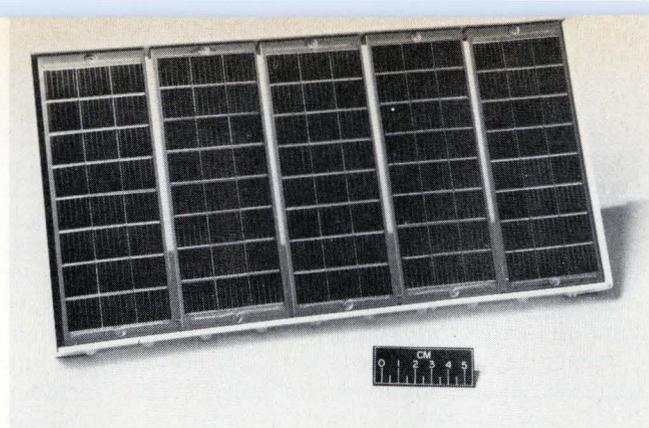
**2. Solar arrays.** Six 9 $\frac{1}{4}$ -by-18-inch modules are put (left) into a 50-watt (at peak) array from Solarex Corp. NASA's Lewis Research Center is experimenting with encapsulating space-type solar cells between sheets of plastic for structural strength and easy handling.
