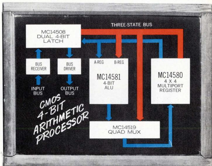
MC14581 performs 16 logical and 16 arithmetic operations. In the larger system, speed is maintained by adding the MC14582 Look-Ahead Carry Block for significant reduction of ripple-through delay.
