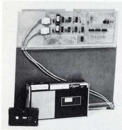
per is primarily a replacement for low-speed paper-tape input/output; it can load a 4,000-word Nova 1200 in less than 90 seconds. Price is \$500
