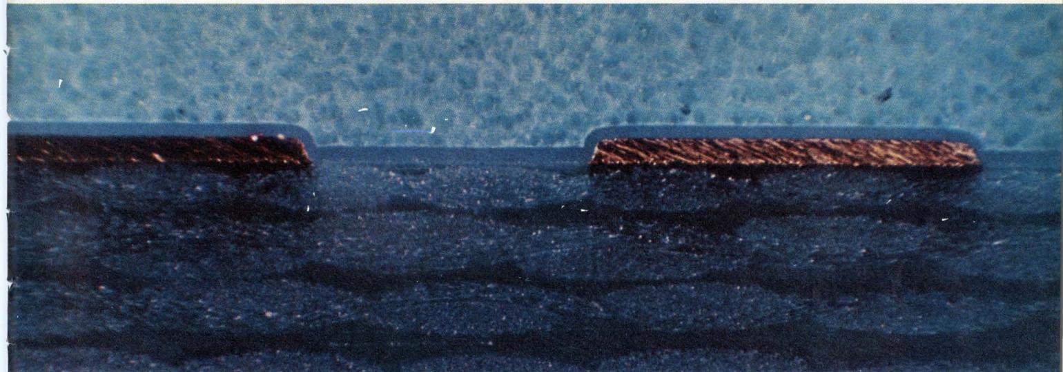
You are looking at magnified cross-sectional views of copper conductors on a circuit board . . . and why parylene protection brings the highest reliability to electronic circuitry.
