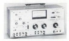
distortion in audio-frequency systems. The unit provides direct readings of the audio-frequency characteristics of passive or active components, such as amplifier transmission lines, networks, filters, transformers, and attenuators. The
