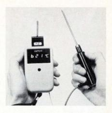
an analog-to-digital converter, MOS logic, and a small number of discrete items. There are three standard probes: chisel-end, flat-end, and a tube for holding liquids. The most likely use in electronics technology is in laboratories to check temperatures of heat sinks, transistor cans, and things like that. However, Ernest May, Kane-May managing director, expects to sell it for laboratory and production use throughout industry.
