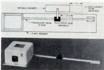
full scale. Several models are available, with displacement ranges of 0 to 12 inches and 0 to 60 in. Further, repeatability is better than 0.02%, and input is +15 volts at 250 milliamperes or -15 v at 25 mA.
