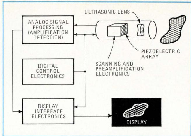
**5. Heart at work.** Cardiologists can study heart action with system that beams ultrasonic bursts into body, observes real-time echo.
