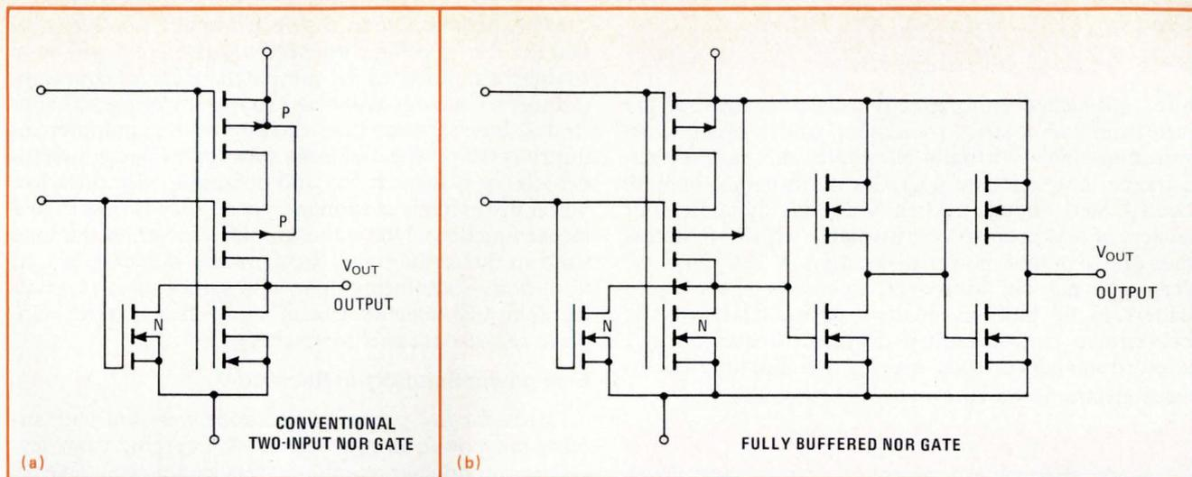
**7. Buffering C-MOS.** Fairchild's use of oxide isolation to build C-MOS circuits reduces gate area and makes room for a buffered gate structure. This improves noise immunity and output drive capabilities and eliminates delay sensitivities.
