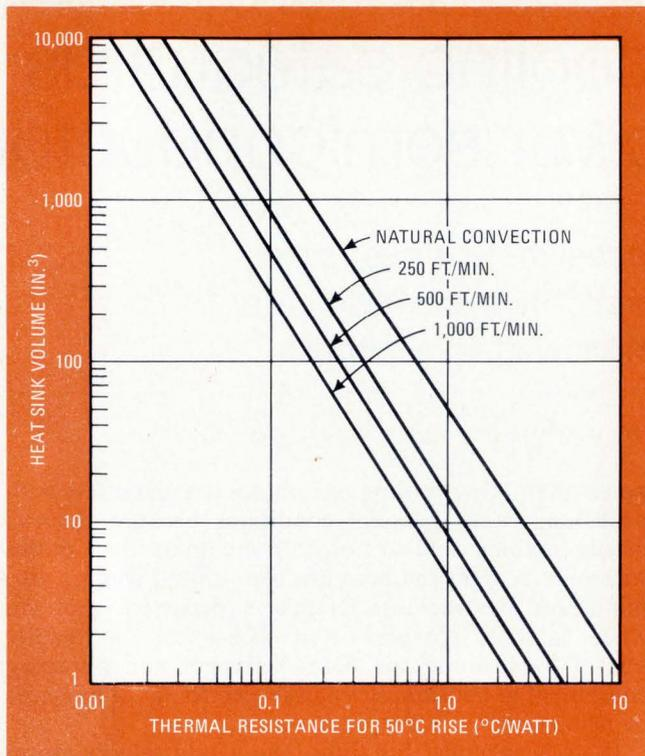
**1. Gobbling space.** The volume of an air-cooled sink grows enormously as a designer lowers the thermal resistance. These curves indicate the various sink volumes for cooling by natural convection and forced air. However, liquid-cooling requires much smaller sink volumes—desirable for compact electronic packaging.
