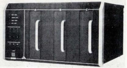
32 sectors per track, while rotation speed is 375 revolutions per minute, and single-track read-write time is 160 milliseconds. Access time is 10 ms for slewing-track, track-to-track positioning, and settling time at final track.
