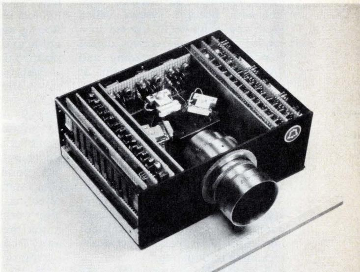
**Ring around a prism.** Bell Labs' CCD color camera of the Picturephone type has three CCD chips arranged around a prism to form the color images. Several other devices have been made using the three-level polysilicon approach.
