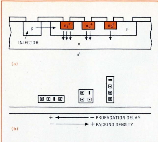
**14. Variable speed.** I<sup>2</sup>L has the virtue of operating at different speeds depending on device layout. Here collector 1, being closer to injector p, operates at higher speeds than collector 2 and collector 3 (a). The propagation and packing density rules are given in (b).
