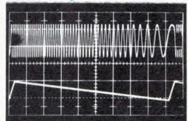
5. Sweep Up or Down the selected frequency range. Just select positive going ramp to sweep up, negative going ramp to sweep down.
