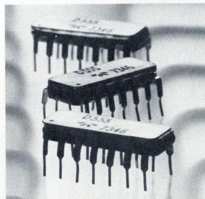
space, and reduces complexity in applications requiring two or more timer circuits. These include uses in sequential timing and synchronization, clock-pattern generation, and pulse modulation. The D555 can also be used in circuits for pulse shaping, frequency division, keyed oscillation, and other one-shot applications. Compatible with TTL,
