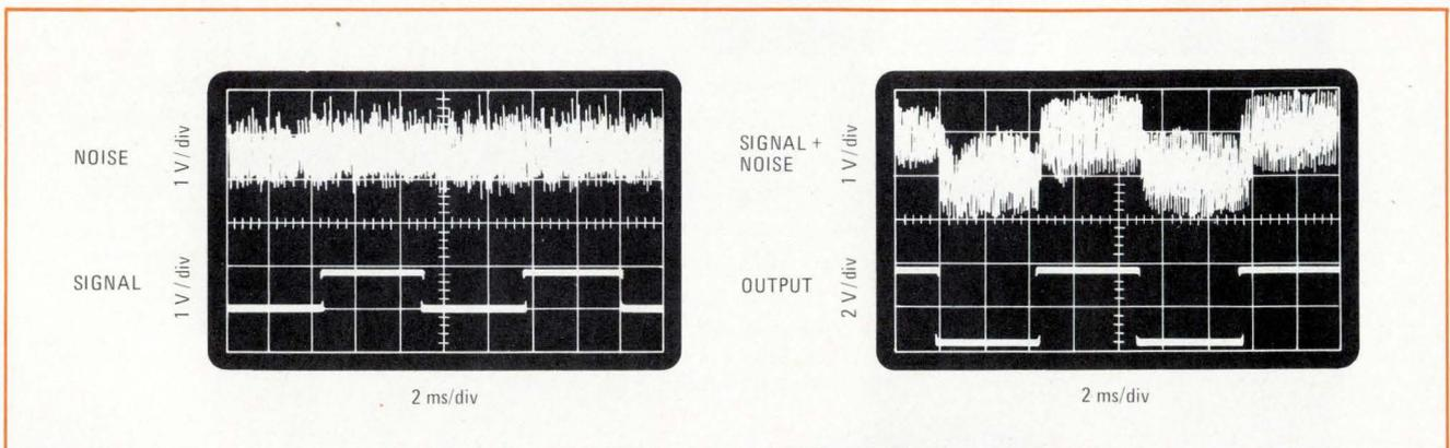
**Pulling the data out of the noise.** Adjustable-hysteresis voltage discriminator makes significant improvement in signal-to-noise ratios, as can be seen from the scope traces. The level of regenerative feedback of amplifier  $A_4$ , the voltage-discriminator stage, is adjusted to provide optimum noise immunity. The gain of amplifier  $A_1$  is controlled by transistor  $Q_1$ , which is operated as a voltage-variable resistor.
