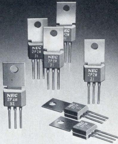
NEC's Models 2P05M, 2P1M, 2P2M, & 2P4M are P-gate all-diffused mold thyristors with an average on-state current of 2 Amps. ( $T_c = 54^\circ\text{C}$ ). Surface treatment of the pellets with glassivation technique guarantees a high degree of reliability.
