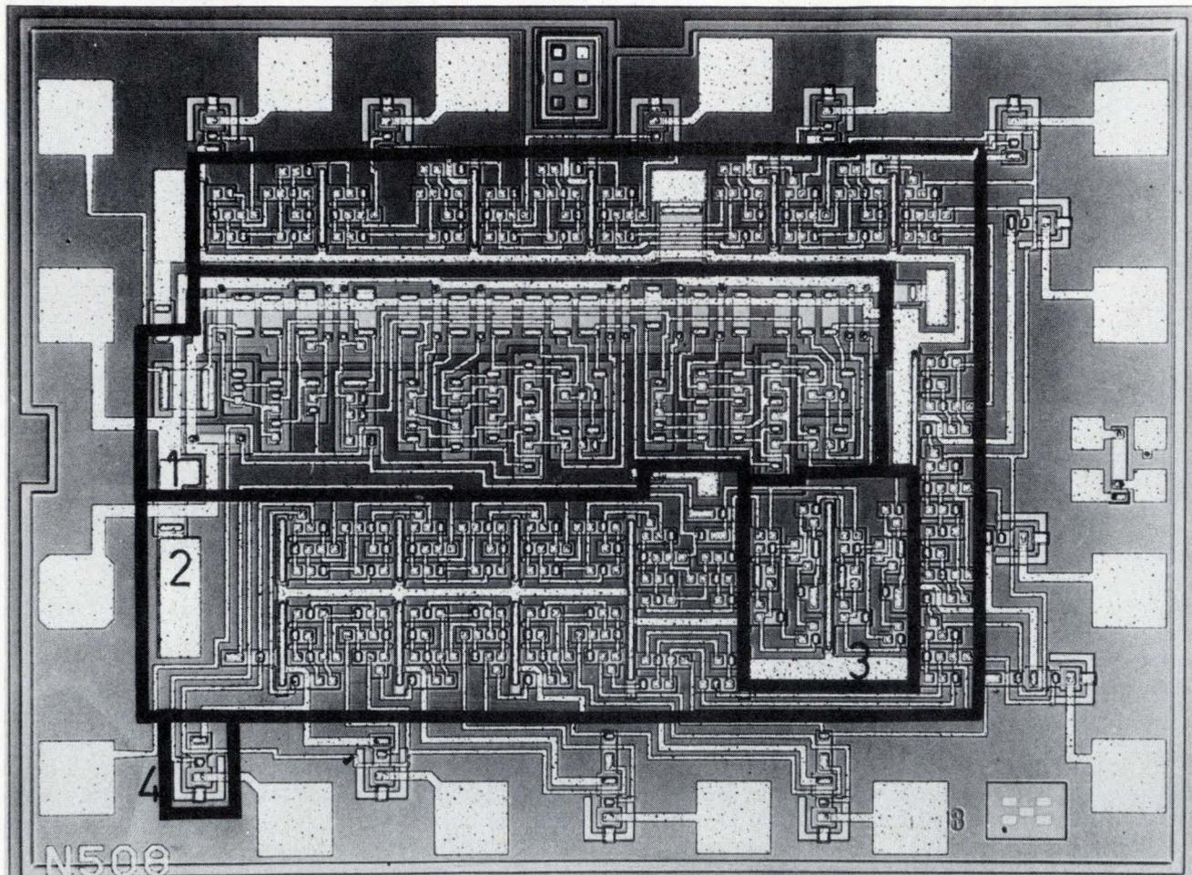
**16. Mixing it up.** In this  $2^{19}$  counter, the first two stages are built with MOS logic (region 1) and the remaining stages with  $I^2L$  (regions 2 and 3.) Note that the two  $I^2L$  flip-flops in region 3, with different layout rules from those of region 2, operate with different speeds.
