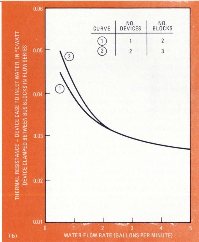
**Two stories.** Stacking two pressure-mounted devices, such as semiconductor rectifiers and thyristors, in a liquid-cooled assembly (a) is a compact technique for cooling kilowatt-level devices. Thermal resistance from the case to the coolant is low at low flow rates, and it diminishes little at flow rates above two gallons per minute (b). Adding the second device (curve 2) raises the thermal resistance a trifle (curve 1).
