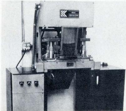
The company compares this operating rate to five conventional systems requiring 16 operators. The new system consists of an eight-ton hydraulic press and a progressive die containing a magazine with approximately 90 strips of devices, which are loaded into the press.
