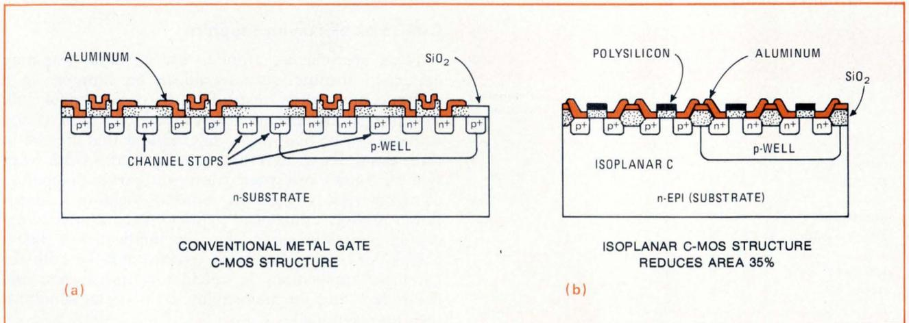
**9. Isolating C-MOS.** The active junctions that isolate devices in conventionally fabricated C-MOS (a) waste space. In Fairchild's oxide-isolated C-MOS structure, the heavily doped p<sup>+</sup> guard rings are eliminated, reducing area and the capacitance that degrades speed.
