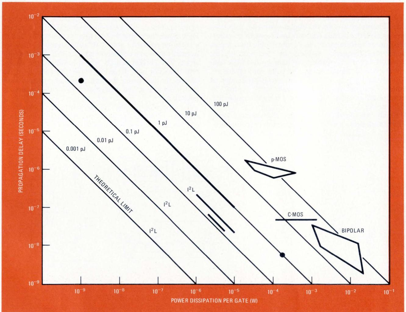
**13. Far out.** The performance of  $I^2L$  far exceeds that of other logic families, MOS or bipolar, because it can operate at nanowatts per gate in less than 10 nanoseconds per gate. The projected speed-power product is less than 0.1 picojoule (for today's TTL, it is 100 pJ).
