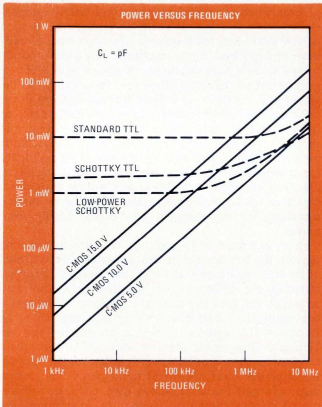
**6. Low power, low frequency.** At frequencies below 10 kHz, C-MOS can operate at dissipations of 10 microwatts per gate and is unbeatable by other logic families. But its power rates climb sharply at higher frequencies and above 100 kHz exceed those of TTL.
