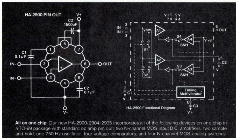
**All on one chip:** Our new HA-2900/2904/2905 incorporates all of the following devices on one chip in a TO-99 package with standard op amp pin-out: two N-channel MOS input D.C. amplifiers; two sample and hold; one  $750\text{ Hz}$  oscillator; four voltage comparators; and four N-channel MOS analog switches.
