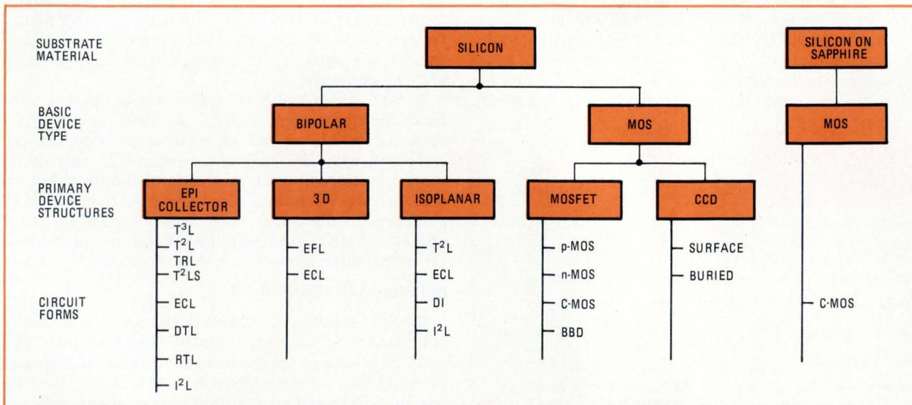
10. **Diversified technology.** Responsible for the growth in logic is an impressive array of processes. There are at least 13 bipolar LSI technologies using three distinct circuit approaches, and four to six MOS LSI techniques. The chart is modified from a TRW source.
