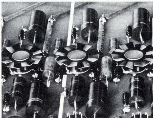
**Faster switching speeds** and lower junction temperatures at the same power levels without spending a bundle was called for after bread board testing of this circuit. Adding IERC Fan Top dissipators to the TO-5s held junction temperatures well below maximums and substantially improved rise and fall times. And the press-on Fan Tops cost just pennies.
