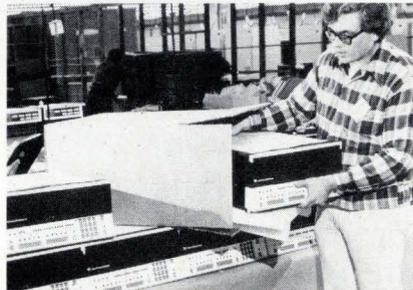
provided, and 32,768 words or 65,536 bytes are indirectly addressable. Numerous software packages are available. The type 2 is contained in a circuit-board case measuring 8.7 by 19.5 by 18.5 in.
