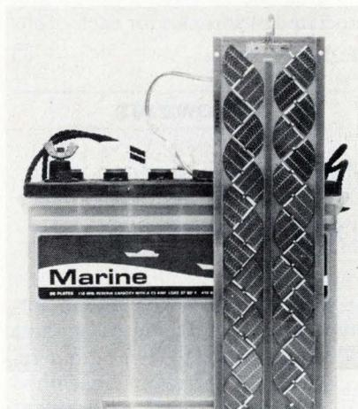
One key to making silicon cells available for such jobs is to get their costs down. Using proprietary design and fabrication tricks, Solarex has developed a cell with the surface electrode in patterns shaped like chevrons.
