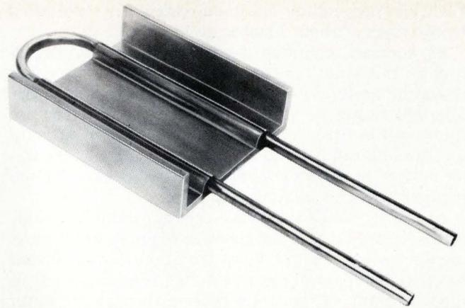
**5. Channel chiller.** This economical U-shaped aluminum plate, priced at \$16, can cool a small number of relatively high-power devices. Thermal resistance varies from about 0.25°C/W to 0.6°C/W, depending on spacing between devices and coolant-flow rate.
