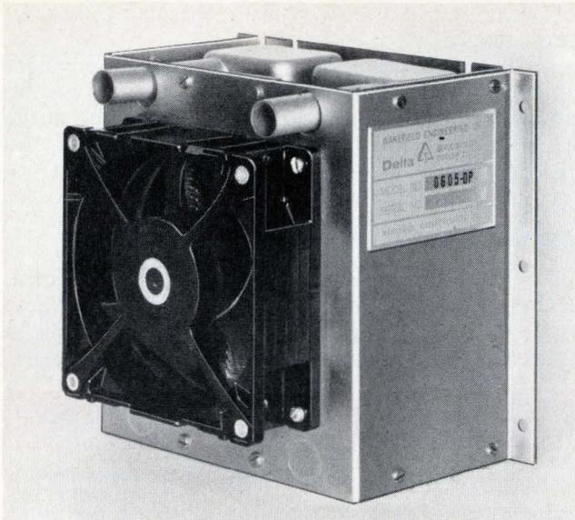
**7. Cool exchanger.** This double-pass heat exchanger transfers heat from the entering liquid to an air stream that is driven through the exchanger by a fan. The liquid enters and exits through the fittings above the fan. Raising the air and liquid-flow rates improves thermal performance. However, to minimize erosion and corrosion, liquid-flow rates through coolant lines should not exceed 10 feet per second.
