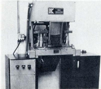
The company compares this operating rate to five conventional systems requiring 16 operators. The new system consists of an eight-ton hydraulic press and a progressive die containing a magazine with approximately 90 strips of devices, which are loaded into the press.
