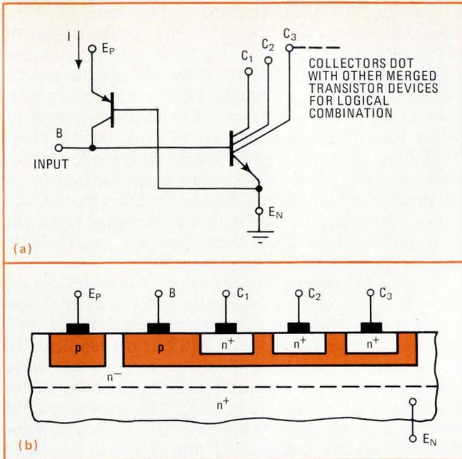
**11. Merging.** In the I<sup>2</sup>L structure, the gate is reduced to a single complementary transistor pair, one of which is a vertical npn transistor with multiple collectors (a). As shown in this IBM structure, on silicon it merges into the space of just one device (b).
