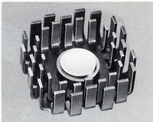
**Design-to-cost** criteria were missed in a touchy servo amplifier because 4 parallel devices required too much testing and matching. Designers went to single TO-6 cooled by nested HP1 and HP3 Staggered Finger dissipators. At 100°C case rise above ambient, the single TO-6 dissipates 36 watts, plenty for the application.
