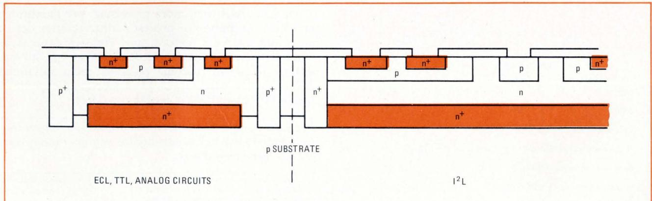
silicon-gate and I<sup>2</sup>L circuits. The results are singularly impressive. I<sup>2</sup>L needs less chip area of any of the MOS technologies, yet operates at bipolar performance levels.
