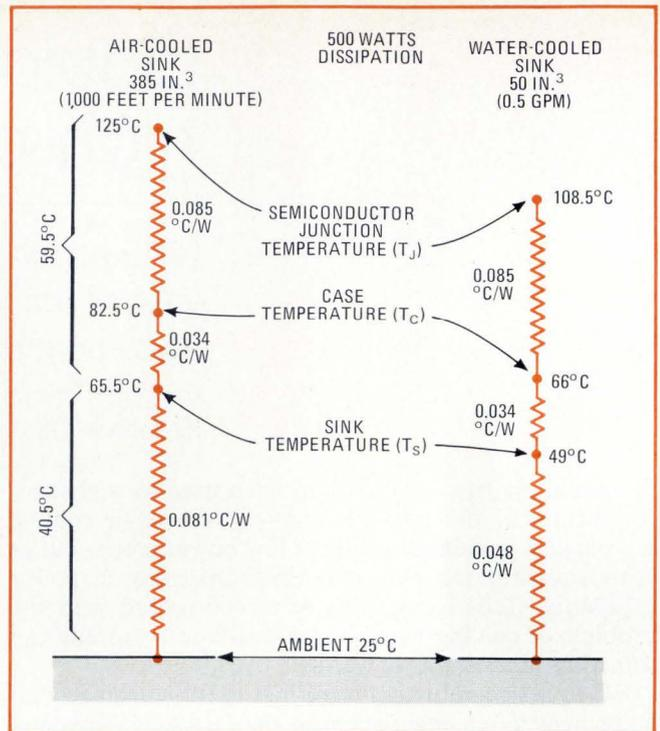
**2. Cool the junction.** Holding the semiconductor junction below a limiting temperature is crucial to thermal cooling—a key factor in long-term reliability. Here, circuit equivalents have been drawn for both an air- and a water-cooled sink dissipating 500 watts. The water-cooled system keeps the junction almost  $17^\circ\text{C}$  cooler and requires about one seventh the volume of the air-cooled sink.
