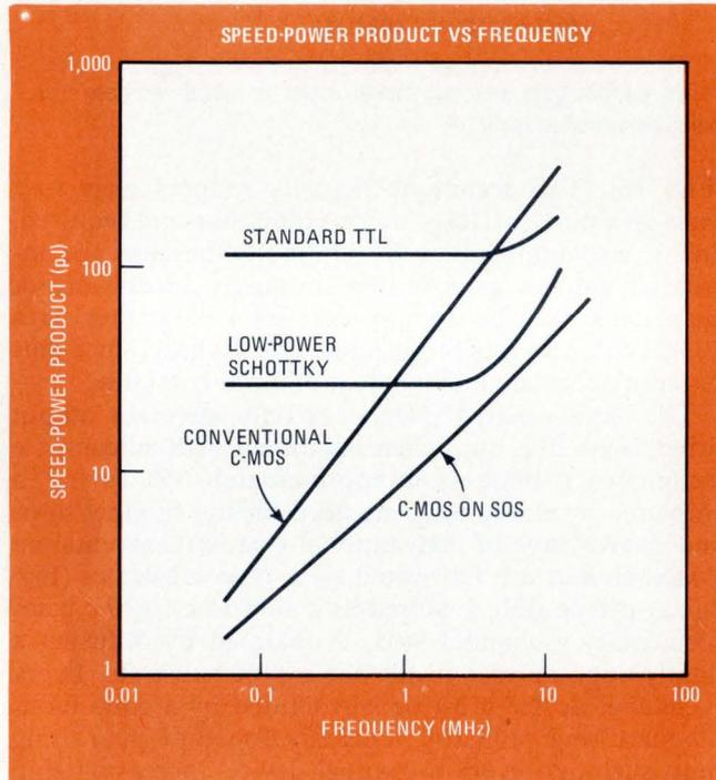
**8. Power struggle.** Low-power Schottky could take over some jobs from C-MOS. It operates at optimum speed-power tradeoffs for many applications, especially in the 100- to 500-kHz range, where it dissipates about twice the power of C-MOS but runs 10 times as fast.
