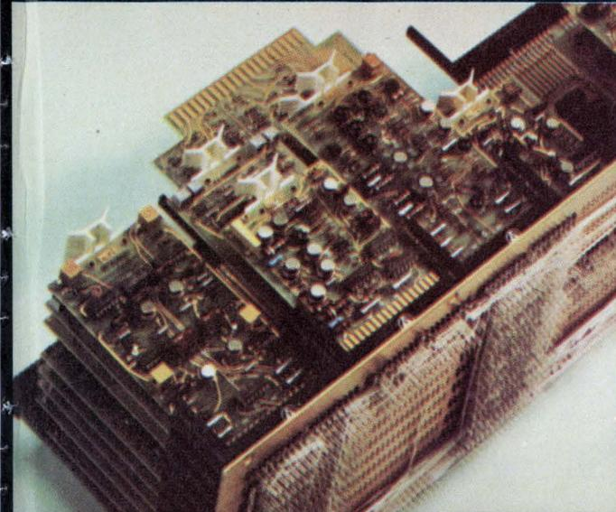
**level 3** Direct entry plate assembly offers modular packaging flexibility. Custom designed plates accommodate any size or style PC board with no tooling cost to you. Rectangular posts are true positioned for automatic wire-wrapping.
