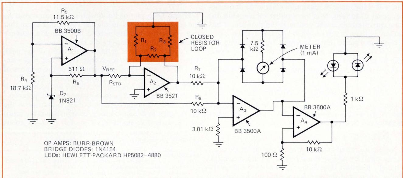
**Trimming circuit.** Individual resistors in closed resistor loop ( $R_1$ ,  $R_2$ , and  $R_3$ ) can be trimmed to desired value ( $R_{STD}$ ). The resistor to be trimmed ( $R_2$  in this case) is placed in the negative-feedback loop of amplifier  $A_2$ . When  $R_2 = R_{STD}$ , the milliammeter indicates a null, and both light-emitting diodes are dark. The LEDs show whether  $R_2$ 's resistance deviation is positive or negative with respect to the null.
