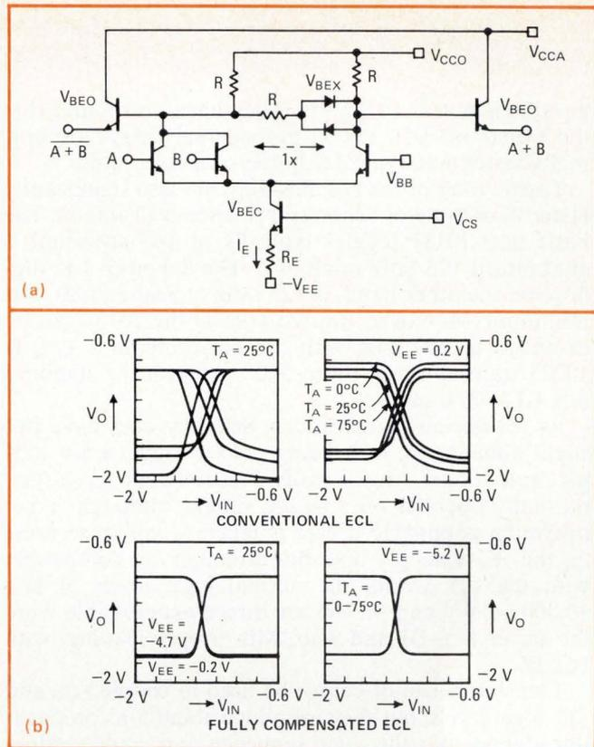
**3. Full compensation.** Fully compensated ECL circuits, the operation of which is not dependent on temperature and voltage changes, include a compensation network like the one shown in (a). This makes for a single switching characteristic (b).
