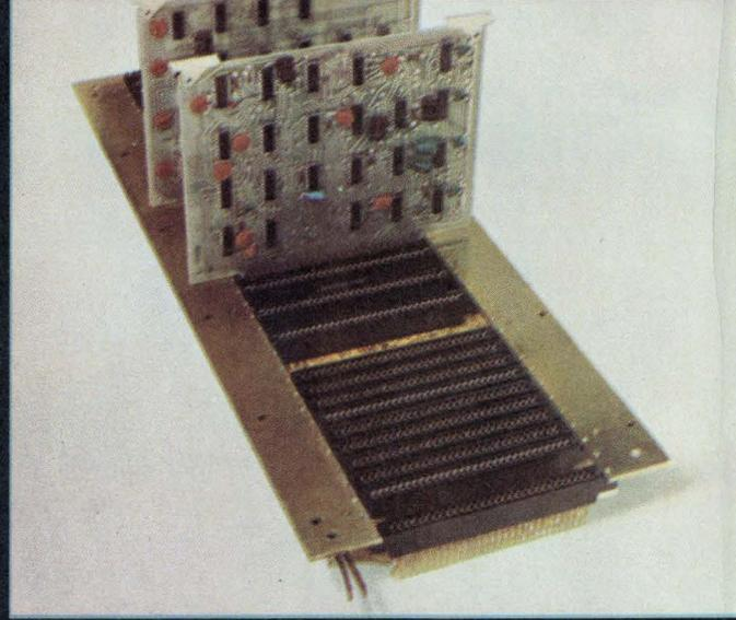
**level 2** Back panel edge board connectors with bifurcated contacts (above) can be wire wrapped or clip-terminated. ■ Bellows contact PC connectors (below) cut interconnection costs without sacrificing performance.
