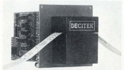
sensing system perform the reading. A stepping motor and dual-sprocket drive system transport the tape through the read head at asynchronous speeds up to 100 characters per second. The dual-sprocket drive eliminates tape skew and assures positive data registration.
