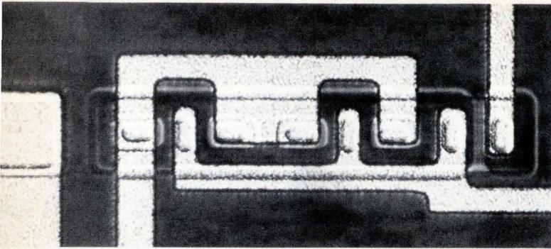
1. **New gate.** This I<sup>2</sup>L gate from IBM Boeblingen occupies space of one bipolar transistor, can operate at 0.1-pJ speed-power product.
