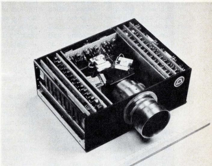
**Ring around a prism.** Bell Labs' CCD color camera of the Picturephone type has three CCD chips arranged around a prism to form the color images. Several other devices have been made using the three-level polysilicon approach.
