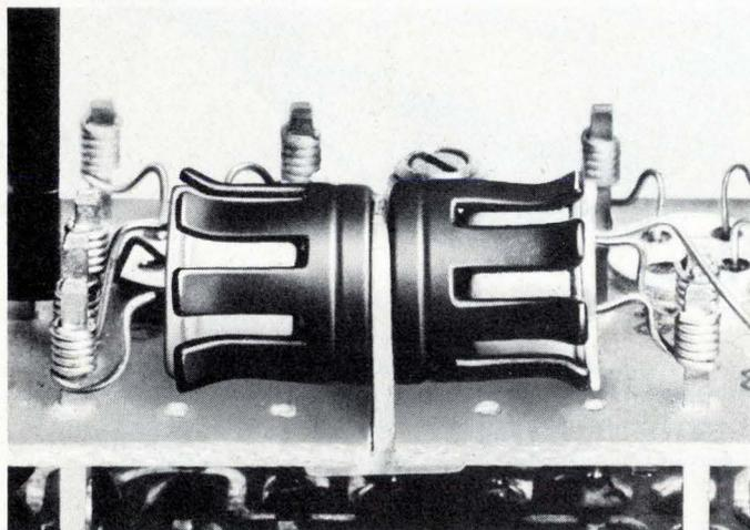
**Erratic flip-flop** in high-G environment posed problem until IERC Thermal Links came to the rescue. Thermal Links held the TO-5s firm, increased their thermal mass, and linked the two cases to a common heat sink. Resulting lowered junction temperature permitted more stable operation and higher reliability while thermal matching assured a balanced circuit.
