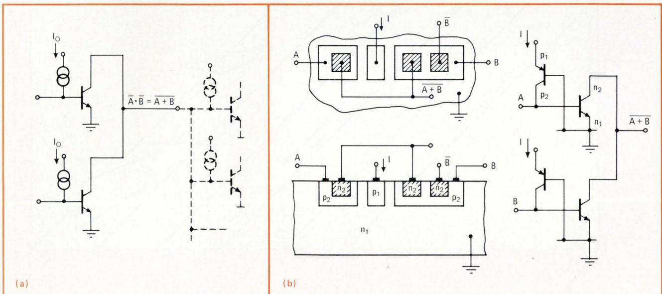
**12. Function.** Great space savings are made with I<sup>2</sup>L in implementing logic functions, like this NOR function, because all the emitters of all npn transistors are tied to a common substrate (a), and current is injected into the device, thus eliminating current-source resistors (b).
