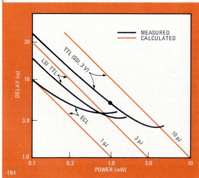
**4. Smaller, better.** Oxide isolation increases the density and speed of TTL and ECL circuits, especially when combined with ion implantation. Bell's OXIM transistor, with implanted base, emitter and collector (a), operates at very low speed-power levels (b).
