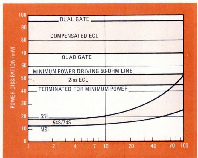
**2. Power tradeoff.** In the low and medium operating ranges, Schottky TTL operates at less power dissipation per gate than does ECL. But Schottky's power consumption goes up dramatically above 20 MHz, and in fact exceeds that of ECL at very high frequencies.
