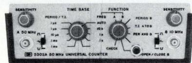
**5302A - Universal 50 MHz Counter Module:** 10 Hz to 50 MHz range. Automatic or manual gating. 100 nsec. time interval accuracy. Period, period average, ratio and totalize functions too. Input waveform selector. \$275.
