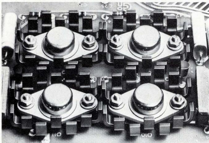
**More power, higher reliability** from the same TO-66s is a paradoxical requirement, but designer met it in this amplifier circuit with LB Series Staggered Finger dissipators. Nominal case rise above ambient of 90°C for bare case TO-66s permits 3 watts dissipation per device. Adding LBs doubled transistor life by giving 10°C temperature drop while increasing power to 5.5 watts per device.
