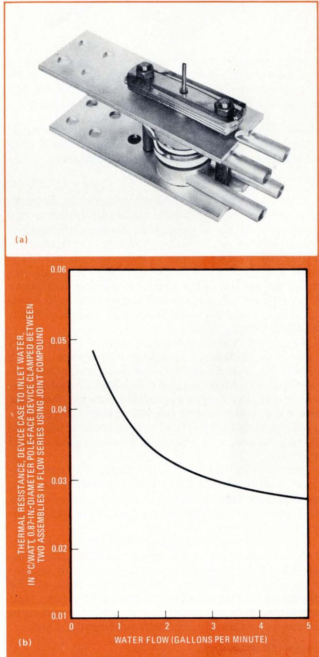
**3. Cool cooler.** The liquid-cooled solid-state copper blocks sandwiching the semiconductor device (a) provide two thermal paths (top and bottom) and dissipate 2 kilowatts. Clamp puts an 800- to 2,000-pound bite on the semiconductor device to assure a low thermal resistance—on the order of  $0.034^{\circ}\text{C}$  per watt at the interface (b).
