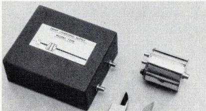
amplifier. Together, they provide a one-way data link with a range up to 20 miles. The transmitter handles 10,000 pulses per second, while the receiver has a wider, 15-megahertz bandwidth and can be used at higher data rates with cooled diode lasers or other sources.
