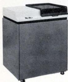
**Use one.** Either drive can be used separately for the storage and retrieval of up to 58 million bits, 7.25 million 8-bit bytes of data.
