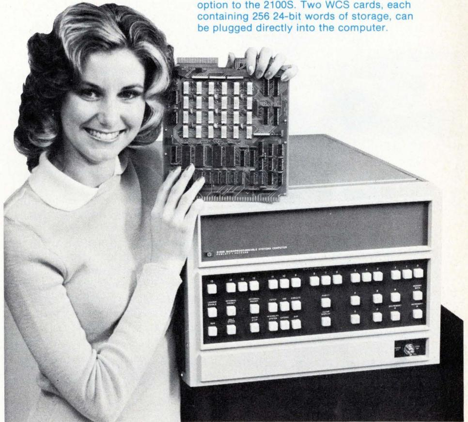
Now, HP offers a minicomputer with built-in "extras" including microprogramming. Extended arithmetic instructions, floating point hardware, dual-channel direct memory access, power fail interrupt, memory parity check, and memory protect—they're all built into the new 2100S computer. A programmable time base generator, communications control channel, and 16K words of 16-bit memory are also standard.
