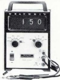
A compact, solid-state multimeter with digital readout — at a fantastic kit-form price. The new Heathkit IM-1202 has four overlapping ranges to measure voltages from 10 mV to 1000 V on DC (either polarity), 10 mV to 700 V rms on AC, 10 uA to 2.5A on AC or DC current. Five resistance ranges measure from 1 ohm to 2.5 megohms. Front panel polarity switch reverses inputs without changing leads. 6 lbs.
