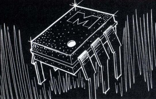
**INNOVATION NO. 3.** The Opto-Isolator. The idea of getting light-quick switching with isolation of  $10^{11}$  ohms has always been attractive. Only with light emitting diodes could it be possible in a small solid state DIP. And we've put them to work . . . Thanks to Monsanto this innovation is now in a lot of computer-to-peripheral and similar sockets.
