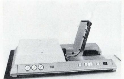
IC under test is observable during the handling cycle.
