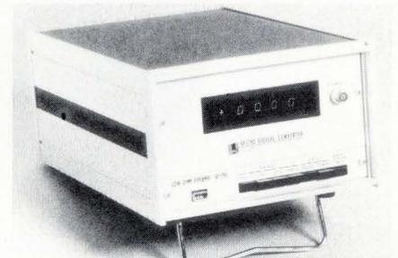
200 ohms. Measurements are displayed on a  $4\frac{1}{2}$ -digit light-emitting-diode readout, and operation may be in a single- or continuous-measurement mode. Ac noise rejection is better than 80 dB at 60 Hz. Test leads may have resistance to 5 ohms with no effect on accuracy.
