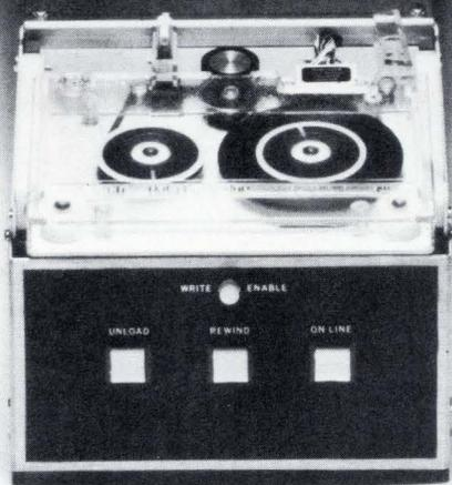
You know it—we know it. The only cassette around for years was great for rock 'n roll, but was definitely a loser—particularly of digital data. Now a new cartridge from 3M—one quarter inch and featuring an isoelastic drive system, has been incorporated into the first cartridge recorder designed solely for reliable data recording—the Kennedy Model 330.
