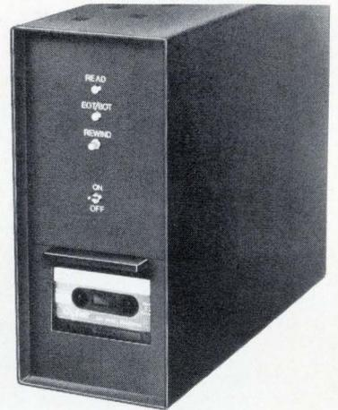
the drive system includes a controller and one bidirectional dual-differential capstan cassette transport with a speed of 6 inches per second. The system's packing density is 800 bits per inch with 8-bit characters. Read-write speed is 600 characters per second. Price is \$2,450.
