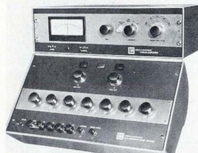
and inspection testing and includes a modified six-dial Wheatstone bridge, a linear amplifier, and a solid-state bridge power supply. The model 4271 is equipped with "low," "go," and "high-limit" lights, and provides 10 switch-selectable limit ranges. In addition to percentage
