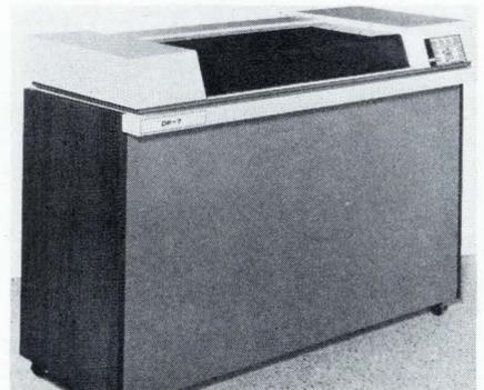
0.0025-inch increment size. The unit is available with up to three pens, available in colors, and automatically selectable. The pens provide a rectilinear trace.
