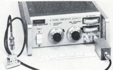
with one of 8 GHz, both putting out 5 milliwatts. The model 44066H covers 40 to 60 GHz; the model 44016H, 50 to 75 GHz; and the model 44076, 60 to 90 GHz. Price is \$1,000 for the power supply, and \$1,500 to \$3,275 each for the sources.
