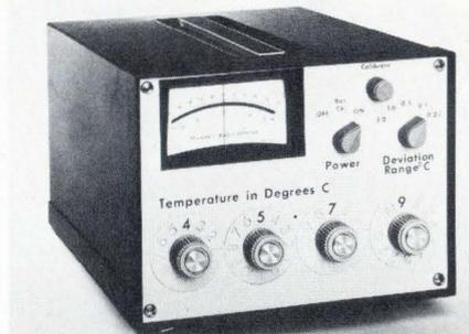
lution of 0.001°C, and long-term deviation from accuracy and stability is rated as  $\pm 0.01$ °C. The thermometer, designated model LD-1, provides a 60-hertz rejection ratio of 70
