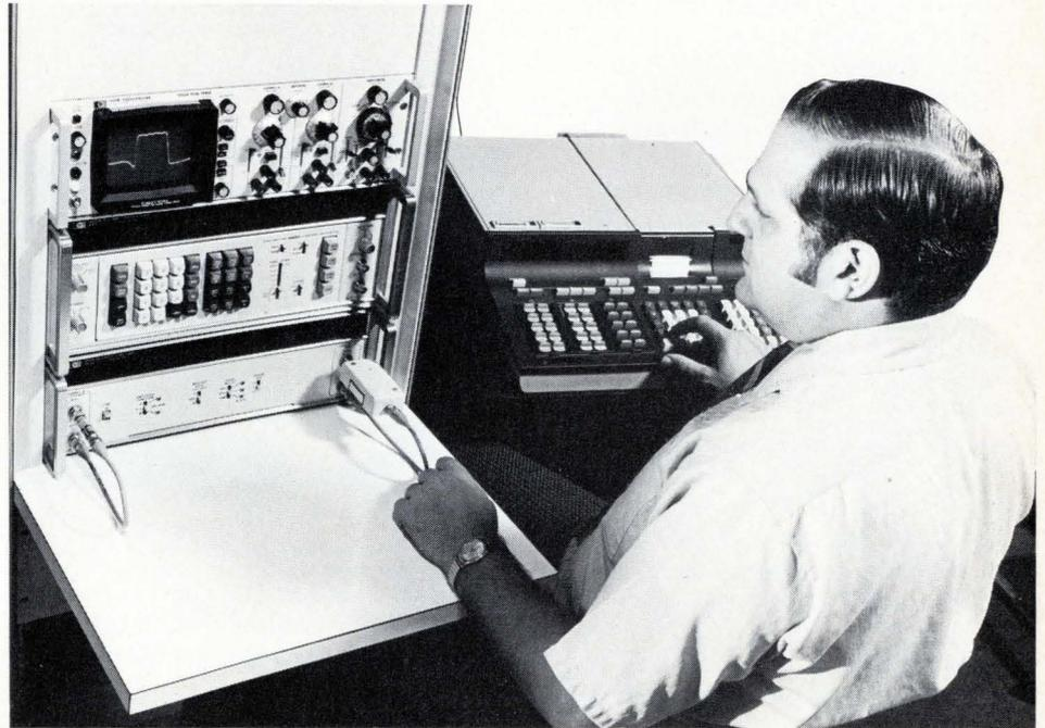
What happens when you combine a network analyzer with a calculator? You get automatic testing of gain, phase and group delay.
