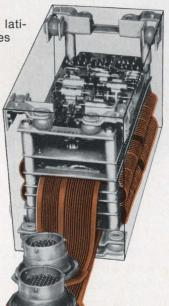
A unique 3-layer combination of flexible and rigid sections, the finished FLEXPRINT assembly in this airborne control system reduced volume 50%, with comparable savings in size and weight, installed faster and at lower cost. Wave soldering was made possible by careful material selection.
