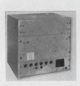
SSB transceiver CA-34 features automatic programming with simplified controls for ease of operation by nontechnical personnel. It is a 100-w unit developed as a multipurpose radio communications system for aviation ground stations. It will operate efficiently under temperature extremes from  $-30^{\circ}$  to  $+65^{\circ}$ C. Communication Associates Inc., 1208 Third Ave., New Hyde Park, N.Y. [387]
