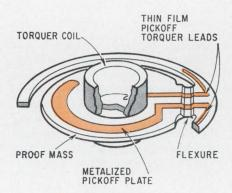
**One piece.** Proof mass, flexture and support are chemically milled from a single quartz blank.
