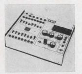
IC tester model 101 is a laboratory unit featuring two independent power supplies for collector supply voltage (V $_{\rm CC}$ ) and logic level "1". The two supplies are so designed that logic level "1" can be no higher than 0.5 v below V $_{\rm CC}$ . Range of the V $_{\rm CC}$  supply is 1 to 15.5 v and for logic level "1", 0.5 to 15 v. Price is \$275. AEI Instrument Co., 3691 Lee Road, Cleveland 44120. [361]
