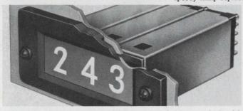
Series 875 Miniature, 24-position, rear-projection readout with .62" H x .62" W viewing area. Overall size just 1.39" H x .90" W x 3.095" D. Exceptional character brightness and clarity. Quick disconnect lamp assembly for easy replacement.
