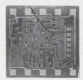
Differential preamplifier model  $\mu$ A727 is a monolithic linear circuit featuring input impedance of 300 megohms over a -55° to +125°C temperature range. Input offset voltage drift is 0.3 $\mu$  v/°C; input offset current drift, 2 pa/°C; input offset current, 2 na; long term drift, 5  $\mu$ v/wk. Fairchild Semiconductor, 313 Fairchild Drive, Mtn. View, Calif. 94041. **[439]**
