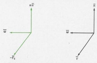
**Analogies.** Spring-restrained gyro's angular parameters, right, of torque,  $\tau$ , angular momentum, H, and angular velocity,  $\omega$ , have their counterparts of Coriolis force, F<sub>c</sub>, linear momentum, mV, and input angular rate,  $\omega$ , in the vibrating beam sensor, left.
