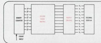
Why use ten logic gate packages to decode from binary to decimal for display read-out? Use only *two* RM-84 eight by five diode matrices. It makes no difference what weighted binary code you are working with, Radiation diode matrices can be easily customized to match.
