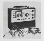
Tv alignment generator model 865 is capable of generating the familiar 10-bar gated rainbow, plus new single-bar and 3-bar test patterns. It provides a total of 9 patterns. The unit measures 4-7/8 x  $9\frac{1}{2}$  x  $5\frac{1}{4}$  in., weighs under 4 lbs. Featuring all transistorized circuitry, it is priced at \$189.95 less batteries. Amphenol Corp., 2875 S. 25th Ave., Broadview, III. 60153. **[401]**
