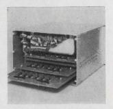
Compact, 8 K x 40 random access core memory series 500 has a 2  $\mu$ sec full cycle speed and features an 800 nsec access time. Only 19 x 11 x 5<sup>1</sup>/4 in., the memory contains 3 circuit module types. All modules and the memory stack are plug-in units that can be replaced quickly. The system is designed for commercial use. Sanders Associates Inc., 95 Canal St., Nashua, N.H. [381]
