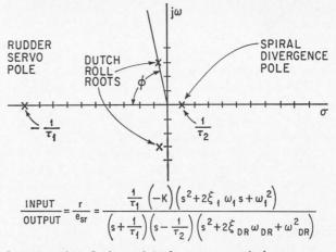
**Low damping.** S-plane plot of uncompensated yaw response of the Dutch roll channel shows that cosine  $\phi$  is low, indicating low damping ratio.
