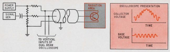
**Gain degradation.** A transistor biased by external resistors and a power supply is driven by a sine-wave generator. By dividing the collector voltage by the base voltage, an engineer can find the gain degradation of a transistor. How fast and to what degree the transistor recovers are determined from the amplitude of the collector waveform as a function of time.
