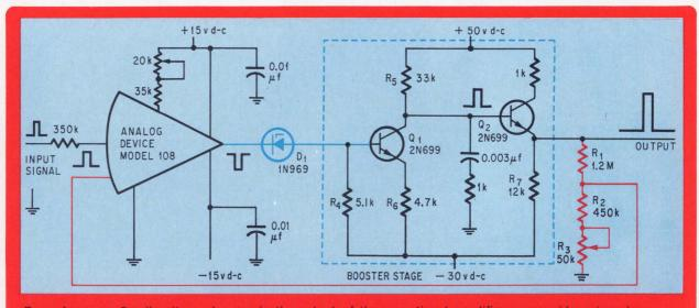
Zener leverage. Small voltage changes in the output of the operational amplifier cause wide swings in the collector voltage of  $Q_1$ , and thus in the emitter of  $Q_2$ . Resistor  $R_7$  gives the boosted voltage the capability of driving low-impedance inputs.
