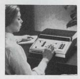
Electronic calculators series C3000 bring silent, instantaneous computing power to the desk top. The C3350, top model in a series of four, which can automatically extract a square root in less than 1/3 sec, features 2 independent core storage memories. Each memory provides 16 digit, 8 decimal storage capacity with minus total. Burroughs Corp., Detroit, Mich. 48232 [388]
