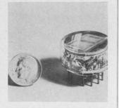
The Digivac readout tube has 7 triodes with a common anode and cathode sealed in a rugged glass envelope. The anode of each triode forms a segment about 8 mm x 1 mm which is covered with fluorescent material that ensures high visibility characters. Viewing distance is over 40 ft.; viewing angle, 150°. Tung-Sol Div., Wagner Electric Corp., 1 Summer Ave., Newark, N.J. [346]
