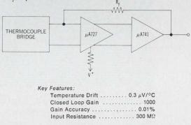
New Product #29 is the µA727 temperature-controlled differential preamp. It's held at a constant temperature by active internal regulator circuitry. As a result, it can provide:
