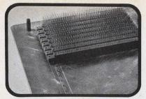
Alignment holes in HW Series connectors are polarized for fast, sure alignment.
