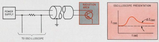
**Leakage current.** The collector-to-base junction is reversed biased by the power supply. By measuring the current flowing through the series resistor, an engineer can determine the magnitude of the leakage current,  $I_{OBO}$ , before, during, and after irradiation.
