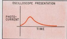
Plotting photocurrents. A balanced system prevents noise from masking the data. The proper choice of resistance optimizes the circuit and the power supplies back bias the collector-to-base junction. The amplitude of photocurrent is displayed on the oscilloscope as a function of time.
