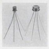
Small signal pnp and npn differential amplifier transistors will track over a wide temperature range with temperature coefficients as low as 3  $\mu\nu/^{\circ}$ C. They offer matched gains to within 3%, voltages up to 120 v, leakage less than 20 pa and low level gains typically 100. They come in TO-78 and TO-71 cases. Solitron Devices Inc., 1177 Blue Heron Blvd., Riviera Beach, Fla. [440]
