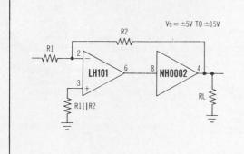
The NH0002 is something else. It has an output current of  $\pm 300$  mA into a load of  $50\Omega$ . The NH0002 buffer is useful in the loop in all your high current op amp applications. The price is \$20.00 in 100 to 999 quantities.
