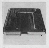
Ferrite memory core stack has a capability of 4,096 words with 16 or 18 bits/word and a fast 1.2 #sec cycle time. It was developed for small-scale, low-cost, computers intended for process control data terminal applications. It contains 65,536 individual 30-mil ferrite cores in the 16 bit/word configuration. Data-Ram Corp., Route 206, Princeton, N.J. 08540. [385]
