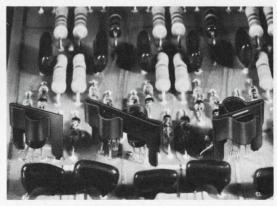
New "Universal" Spade Series for plastic transistors fits all D-case sizes. Spring clip allows for variation in case diameters. Excellent dissipation lets you boost operating power 33%. Both single and dual models as shown. IERC has heat dissipators for all popular epoxy and ceramic semiconductors.
