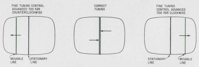
Visual fine tuning. This variation by Westinghouse on a basic AFT circuit presents an on-screen indication of the degree of mistuning by the spacing between movable and stationary lines.
