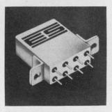
Military-type crystal can relay 79N is a low-cost, 2pdt dry circuit-to-3 amp unit that switches minimum current (100 ma to 0.5 amp) with the same reliability as dry circuit and load current. A new contact design permits the relay to meet a 100,000-cycle, no-failure test over its full range. Electronic Specialty Co., 19000 N.E. Sandy, Portland, Ore. 97200. [348]
