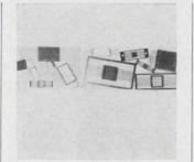
Flat Pak packages for IC's, discrete components and hybrid circuits are designed to meet critical military and industrial requirements. A wide variety of standard and special package sizes are available from 14 to 30 leads, from  $\frac{1}{4} \times \frac{3}{6}$  in. to 0.85 x 0.2 in. sizes. Units conform to MIL STD 705A. Space Ordnance Systems Inc., 25977 Sand Canyon Rd., Saugus, Calif. 91350. [343]
