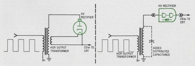
**High-voltage rectifiers.** By switching to the solid state design at the right, Motorola has eliminated the filament winding required in the flyback transformer of the vacuum-tube setup at left.
