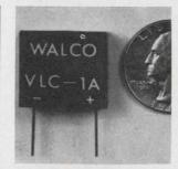
Solid state variable current limiters allow the user to obtain a continuously variable constant current with a ranging capability of 50 to 1. Current limiting capabilities are from 1  $\mu$ a to 50 ma with input ranges from 5 to 35 v. Level stability is an order of magnitude better than that of fixed current limiters. Wall Electronics Co., 3821 Commercial N.E., Albuquerque, N.M. [342]
