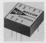
Low drift, FET input operational amplifier 1765 features high common mode rejection ratio, high power bandwidth, and high slew rate. It can be operated over a wide range of supply voltages and has an output swing of up to  $\pm 21$  v. Applications include control instrumentation and data logging. Melcor Electronics Corp., 1750 New Highway, Farmingdale, N.Y. [384]
