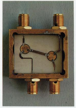
**Circulator.** This X-band, four-port circulator uses 20-mil thick alumina and handles 500 watts peak with an 0.8 db transmission loss and 0.4 db reception loss. The circuit provides 40 db isolation over a 25% bandwidth. Magnets are located below the ferrite disks, which are mounted in holes in the ceramic. The ceramic is 1 inch square. Thick-film techniques are used.
