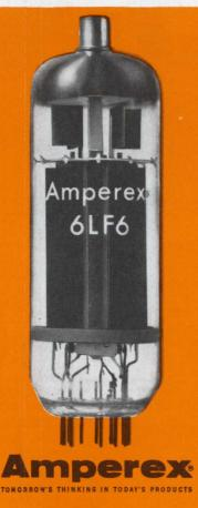
Two years ago we produced color TV's first—and only—low B+ anti-snivet tube, the 6KG6. Now we offer a 12-pin version of that unconventional device, the brand-new 6LF6 beam power pentode for use in horizontal deflection amplifiers. Like its 9-pin predecessor, the 6LF6 is built around the Amperex-developed "Cavi-trap" anode that prevents Barkhausen oscillations and eliminates snivets from color TV screens.
