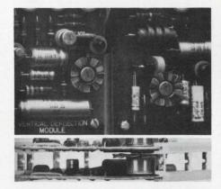
Fan Top Dissipators for TO-5 and TO-18 cases add almost nothing to board height. Don't need much room on the board either. Available for both metal and plastic cases. Spring fingers make installation simple. And Fan Tops cost just pennies.
