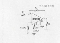
When we say high output current, we *mean* high. The output current on this, the NH0005, is  $\pm 50$ mA into a  $100\Omega$  load. The price in 100 to 999 quantities is \$45.00. And there's a commercial version, the NH0005C, priced at \$22.50.
