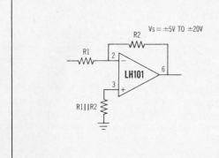
The LH101 is kin to the LM101. The essential difference is that all the required frequency compensation is *inside* the package. Current drain is low, even with the output saturated. There is no latch-up when common mode range is exceeded and there's continuous short circuit protection. Price for 100 to 999 is \$48.00. The commercial version LH201 is \$11.40.
