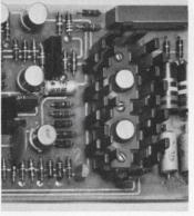
Help low-to-medium power transistors keep their cool with IERC's stagger-fingered LP's. Available in single or dual mounting for thermal mating of matched transistors. They fit both TO-5 and TO-18 cases.
