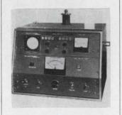
Corona test set model 4074 incorporates a Hypot with a 10 kv at 0.25 kva maximum continuously variable corona-free output. Output voltage crest factor is better than 5%. The corona detector consists of a scope with a verticle amplifier sensitivity of 3 mv/in. at max. gain. The 4074 is priced at \$2,250. Associated Research Inc., 3777 W. Belmont Ave., Chicago. [366]
