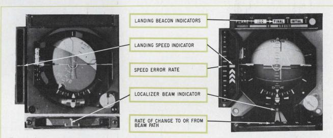
**Easy on the eyes.** Electroluminescent instrument panel (on right) is easier to read and supplies more information than conventional panel. Moving lights indicate landing beacon position and landing speed and their rate of change.
