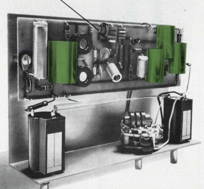
A typical part of the Primary Phase Angle Standard shown above with four capacitors of MYLAR (green).
