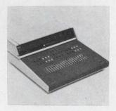
IC tester model 1740 provides parametric and functional operational measurements. Applications include incoming inspection, wafer sorting, and final inspection. The unit is capable of forcing voltages or currents and performing the measurements either go/no-go or readout, utilizing a front panel mounted dvm. Miracle-Hill Electronics, 320 Martin Ave., Santa Clara, Calif. [368]
