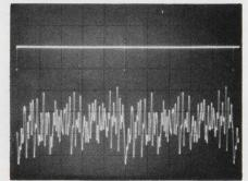
REPEATABLE Sweep time of oscilloscope, 0.2 millisec/cm; Noise Generator: sequence length, 1023; clock period, 1 µsec.
