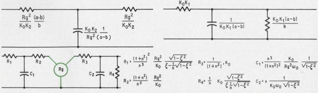
Active-filter design. Starting with a single gyrator flanked by two RC networks, the designer assumes the left one to be a T network. By synthesizing the over-all transfer function, he finds that the right network can be a series-parallel RC circuit. Values for all elements are shown on the drawing.
