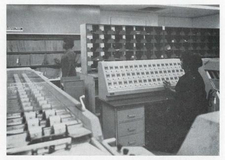
**Taking the high road.** After the analysts get through with a message, it is duplicated (the average is 125 copies; the outer limit is about 500) and each copy is placed in the proper mail receptacle by this Remington Rand Lektriever.
