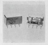
Welded half-size crystal can relay BR 26 features single-coil design and meets MIL-R-5757. Universal contacts permit operation from dry circuit to 2 amps with the same contact set, at coil voltages of 6, 12, and 26 v d-c. Max. operate/release time is 4 msec. Temperature range is -65° to +125°C. Babcock Electronics Corp., 3501 Harbor Blvd., Costa Mesa, Calif. **[345]**
