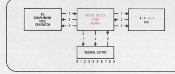
When one logic code must be converted to several other codes for processing, think diode matrices! Specify only *four* RM-84 diode matrices and form a 16 by 10 matrix array. Six conversions can be performed by this single bi-directional array...replacing approximately 80 logic elements.
