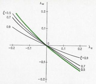
**Corner frequency vs.**  $R_g$ . Colored line represents data obtained from design example 1. Second method's response in black, is superior for stability of corner frequency.
