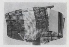
**Back to back.** Telefunken's upcoming air traffic control radar uses a pair of reflectors, each  $29\frac{1}{2}$  by  $48\frac{1}{2}$  feet. Waveguides aren't mounted on this unit, a model for wind-tunnel tests.
