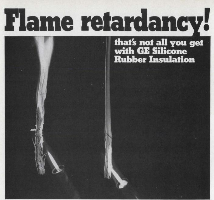
New ultra-tough SE-9090 braidless wire and cable insulation (right) doesn't support combustion like conventional insulation. It's shown here passing the UL vertical flame test. SE-9090 has both outstanding insulation resistance and dielectric strength.
