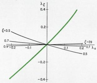
**Damping ratio vs.**  $\mathbf{R}_{g}$ . Data obtained from design method 2, shown in black, is superior to that obtained from method 1, in color, for a specified damping ratio.
