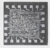
MOS FET JK flip-flop logic circuit element type HRM1306 features AND gates forming the J and K inputs, together with a clocked preset function and a direct reset function. It operates at frequencies ranging from d-c to 500 khz and at power dissipations of less than 30 mw. Price is \$21.50 in lots of 1 to 99. Hughes Aircraft Co., 500 Superior Ave., Newport Beach, Calif. [442]
