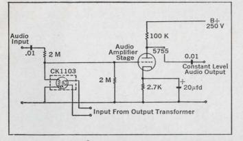
**1. Use the Raysistor**<sup>®</sup> as a simple remote or automatic volume control in SSB suppressed carrier receivers. Feeding part of the audio output into the control light source varies the resistance of the Raysistor's photocell, making it usable in place of a normal volume control.
