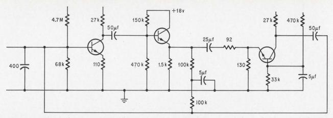
**Practical gyrator.** Three transistors are used to form this this gyrator circuit. Gyration resistance is 118 ohms, and remains constant within a frequency range of nearly 3 decades. Entire network behaves as a passive device and neither consumes or adds signal energy. In the transmitting direction the circuit has a maximum insertion loss of 1.5 db; isolating direction 60 db.
