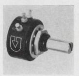
Precision pot model 1090-1001 offers advantages in applications involving high signal frequencies and need to minimize noise during adjustment. Specs include max. capacitance of 1.5  $\mu$ f, max. inductance of 0.15  $\mu$ h, total resistance of 1,088 ohms  $\pm$ 10%. Linearity is 1%, temperature coefficient  $\pm$ 20 ppm/°C. Digilog Electronics Corp., 701—3rd Ave. North, Seattle 98109. [344]
