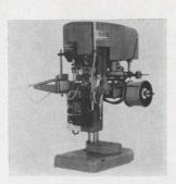
Coil-winding machine BV4-G is a carousel-type unit designed to wind electrical coils without forms at production rates from 160 to 1,920 coils per hr depending on coil design and size. Lead ends are automatically tinned. Low voltage electric heat is applied to the rotating tinning bath with electronic temperature control. Leesona Corp., 131 West St., Danbury, Conn. 06810. [424]
