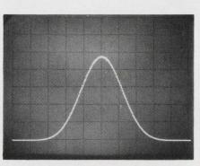
The Hewlett-Packard 3722A Noise Generator now lets you harness noise so that it becomes a defined and calibrated input to your system. It allows you to synthesize and reproduce at will noise signals of constant noise power with a probability density function (pdf) in the classical Gaussian construction. This unique new instrument uses computer techniques to synthesize noise patterns of selectable length that are thoroughly defined and repeatable.
