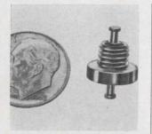
EMC/RFI filters series 75000, for use in low voltage circuits, combine high capacitance-low voltage ceramic capacitors and high current inductors in a sealed device. Measuring 0.400 in. diameter x 0.370 or 0.100 in. body length, units have max. d-c resistance at 25°C of 0.11 or 0.01 ohm, respectively. Electro Materials Corp., 11620 Sorrento Valley Rd., San Diego, Calif. [341]
