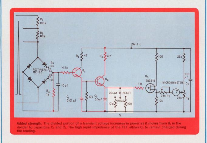
tion of the microammeter's needle. The needle remains deflected as long as switch  $S_1$  is in the hold position. A fast or slow return of the needle to zero is achieved by switching to either the reset or decay positions.
