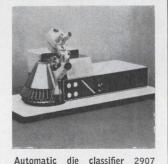
Automatic one classifier 2907 tests devices ranging from 0.020 to 0.125 in, round or square, at the rate of 3600 per hr. It features a vacuum feed device which deposits the devices gently in the test position. Vacuum is generated internally and controlled by valves to prevent them from sticking or scattering. Hughes Aircraft Co., 500 Superior Ave., Newport Beach, Calif. **[426]**
