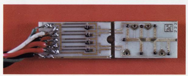
**Phase shifter.** A Ku-band, four-bit phase shifter, measuring only 0.220 by 1 inch, has two 20-mil alumina boards mounted on a supporting plate—one board for the thick-film phase shifter, and the other for the thin-film driver for the p-i-n diodes. The diodes are located at ends of various length impedance stubs, which act as transformers to translate the diode reactance to achieve the desired phase shift. The power level is 100 watts peak.
