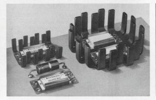
Cool off microcircuit devices with a choice of four new dissipator/retainers. Example: with natural convection, a typical microcircuit device dissipates 1.8 watts with case temperature rise of 103°C. Add IERC's model LBOC2-61B and retainer and you dissipate 5 watts with the same case mount package to conduction plane.
