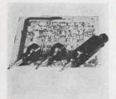
Air operated cut and bend tool BP-1 Bend Eze features interchangeable heads, which meet the circuit board at either 20, 30, or 45°. The quill has a max. o-d of 3/16 in. diameter. The tool will take an existing component wire, cut it off, and lay it flat to the circuit board to military specifications. Price is \$99.50. Henry Mann Co., Box 37, Cornwells Heights, Pa. 19020. [421]
