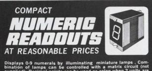
Displays 0-9 numerals by illuminating miniature lamps. Combination of lamps can be controlled with a matrix circuit (not supplied). Decimal points can be used as colon when 2 units are placed together. Indicator provides high illumination with a low voltage and current. Colored filters available. 6 & 12V. Figures 25/32" high. 20,000 hr. bulb life.
