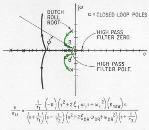
**Higher damping.** Root locus plot with rate sensor in the damping loop shows paths (arrows) taken by poles as loop gain goes from zero to infinity.
