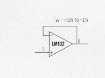
The LM102 voltage follower is the first monolithic amplifier that has combined low input current with high speed. Slew rate is  $10V/\mu$ s. The maximum input current is an incredible 10nA. Input currents better than 10nA at 125°C are guaranteed. The price: \$30.00 each in 100 to 999 quantities. The -25°C to +85°C LM202 is priced at \$12.00, LM302 commercial at \$5.40.
