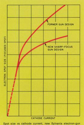
mount vs previous mount. Tests have shown that spot diameter of new gun is  $10-20^{\circ}/_{0}$  smaller at currents above 300  $\mu$ a...a very definite advantage in spot blooming at high brightness in a color scene.
