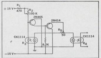
2. As a remotely controlled linear potentiometer. The Raysistor can be used as a remotely controlled linear potentiometer when used in the circuit shown above. Here the Raysistor forms a voltage divider between the positive and negative voltages.
