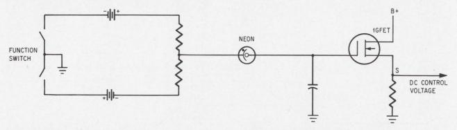
**Remote control circuit.** Continuously variable functions are handled by a "memory" module developed by Motorola. The neon lamp serves to isolate the timing elements from external circuitry when a function switch is open.
