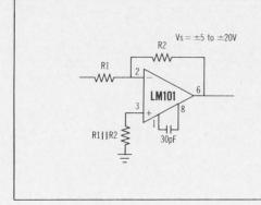
Old faithful LM101 is both general purpose and no-sweat in operation. It's short-circuit proof and has a large differential input voltage allowance. Moreover, frequency compensation is simple, and there is no latch-up problem. The price is \$40.00 in 100 to 999 quantities. (There is also a commercial version, the LM201, priced at \$8.80.)
