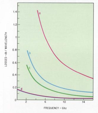
Lower loss. Because of alumina's high resistivity, its losses are low—lower than those in silicon. Curve "a" indicates the dielectric loss in 1,000 ohm-cm silicon, 10-mils thick; curve "b" shows dielectric and conductor losses for 5,000 ohm-cm silicon, 10 mils thick; "c" is dielectric loss for 5,000 ohm-cm silicon, 10 mils thick. Curve "d" represents dielectric and conductor loss in alumina that is 20 mils thick.
