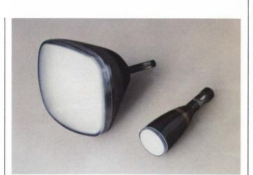
21" SC-4876 and 5" SC-4689 are typical of the range of multicolor tube types that can be made. Each is capable of displaying alphanumeric or analog information in 4 or more colors simultaneously, using a single gun.
