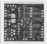
Monolithic active filter IC WML-5, a true linear MOS device, consists of 3 differential amplifiers in a 70 x 90 mil chip. It is a basic building block that can be used for more complex functions. For example, a 4-pole pair band pass filter could have relative bandwidth from less than 1% to over 100%. Western Microwave Laboratories, 1045 DiGlulio St., Santa Clara, Calif. [437]
