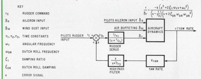
**Damper system.** Beam sensor is placed in feedback loop in Dutch roll damper system to sense yaw rate, help keep aircraft on an even keel. Simplified transfer functions of each element are indicated.
