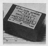
Active high-pass filter networks series HPB4 features the 4-pole Butterworth gain and phase frequency response characteristic. Attenuation over the operating temperature range of  $-40^{\circ}$  to  $+71^{\circ}$  C is 3 $\pm$ 0.5 db at cutoff frequency and 24 $\pm$ 2 db at onehalf cutoff frequency. Standard cutoff frequencies are from 1 to 1,000 hz. Linear Networks Co., Box 1103, Bozeman, Mont. [383]
