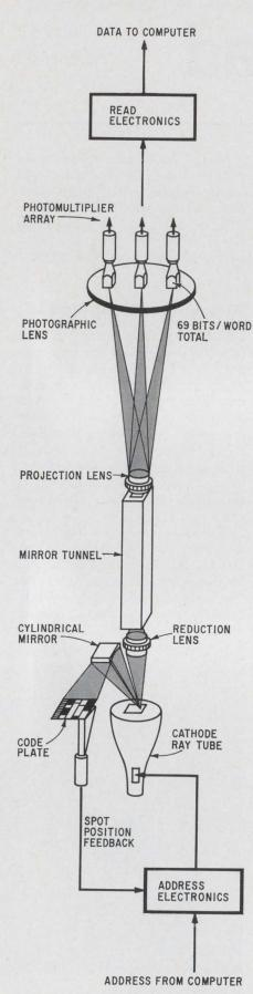
Kaleidoscopic. Tunnel of mirrors that multiplies crt spot is basis of optical read-only memory.
