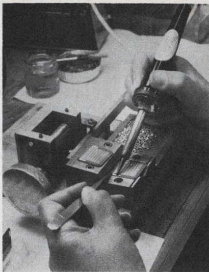
Cool. Low-temperature solder is used to wire ferrite memories.
