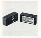
Arc accuracy of 30 seconds is attainable with a series of Scott-T transformers. The miniature toroidal devices convert 3-phase synchro inputs to 2-phase resolver outputs. Line-to-line input voltage is 11.8 v, rms output voltage 5 v. Operating frequency is 400 hz; temperature range is -55° to 125°C. Price is \$70 for single units. Magnetico Inc., 6 Richter Court, East Northport, N.Y. [345]
