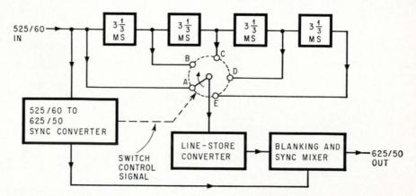
**Slight delay.** Five-position switch and four delay lines in cascade are key to BBC's television-standard converter.
