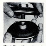
"Doorbell" rectifier module series UG has ratings up to 8.25 amps in air and 10 amps in oil, and from 2.5 kv to 10 kv. Modules are vacuum encapsulated with highthermal-conductivity filled epoxy for voidless construction and corona-free operation. Each module has threaded connectors for stacking up to 600 kv. Delivery takes 2 weeks. Unitrode Corp., 580 Pleasant St., Watertown, Mass. [437]
