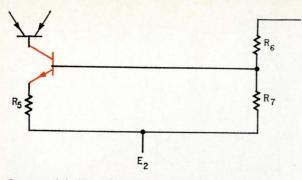
**Current sink.** Use of constant current source in place of large resistor in the common-emitter circuit improves common-mode rejection and simplifies monolithic fabrication.
