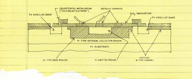
\*Field Relief Electrode — Patent #3,302,076 Annular Structure — Patent #3,309,245 and #3,309,246
