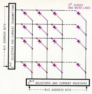
**Diode matrix.** In conventional design, one transmitter and one receiver send current through a single word line. The diodes block parallel paths through adjacent wires for any given transmitter-receiver combination. Matrix is used to minimize the number of components, thus holding down costs. Diodes and word lines are in color.
