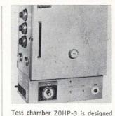
to provide stable life-test temperature conditions for in-chamber parameter measurements of semiconductor and axial-lead components mounted to p-c boards. It provides for life-test temperature environments from 100° to 400°F with a stability of  $\pm 0.25^\circ$ F, utilizing a laminar air flow. Associated Testing Laboratories Inc., 200 Rt. 46, Wayne, N.J. [423]
