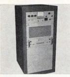
Frequencies from below 200 khz to above 220 Mhz are amplified linearly more than 50 db to power levels up to 400 watts by the M404A laboratory amplifier. No tuning is needed. Applications include communications systems, rfi tests, antenna research programs, and nuclear magnetic resonance work. Instruments for Industry Inc., 151 Toledo St., Farmingdale, N.Y. 11735. [381]
