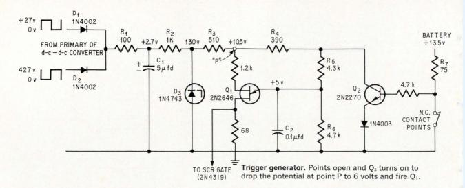
used elsewhere in the system, which is rectified by diodes  $D_1$  and  $D_2$ , filtered with network  $R_1$ ,  $C_1$ , and  $R_2$  and regulated to 13 volts with diode  $D_3$ . Sufficient current, supplied from the battery through  $R_7$ , assures reliable contact.
