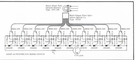
MRD300 combined with 2N4198 ELF\* SCR (600 V) gives total  $t_{on}$  of 300 ns. Single light source coupled by multiple-output fiber optic bundle transmits light to photo transistors. Fast  $t_{on}$  is accompanied by gate isolation advantage.
