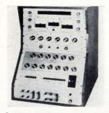
Guildline 9930 d-c current comparator potentiometer features a 7-figure readout without critical resistors. Linearity is 0.05 ppm over full range, and long term drift less than 0.1 ppm per year. The unit's resolution is only 1 part in 2 x  $10^7$  of full scale, and standard cell dial resolution is 0.1 ppm. Cost is \$7,890. Hallmark Standards Inc., 145 Library Lane, Mamaroneck, N.Y. [361]
