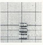
Molded chokes come in 3 types. Models 3710-1 through -7 cover inductances from 47 to 150  $\mu$ h in a 0.250 x 0.560-in. package. Q values range from 18 to 75. Models 3711-1 through -5 cover 180 to 390  $\mu$ h, are 0.310 x 0.560in. with 80 to 75 Q's. The 3712-1 through -5 cover 470 to 1.000  $\mu$ h and are 0.375 x 0.625 in. Cambridge Thermionic Corp., 445 Concord Ave., Cambridge, Mass. [348]
