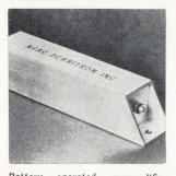
Battery - operated preamplifier series PA uses a noise-canceling circuit and features an rms-integrated broadband noise level below 10  $\mu$ v. Input impedance is 1,000 megohms; frequency range, 0.2 hz to 100 khz. Models are available in fixed gains of 0, 10, 20, 40, and 60 db, and variable gains of 0 to 20 and 20 to 40 db. Agac-Derritron Inc., 600 N. Henry St., Alexandria, Va. [385]
