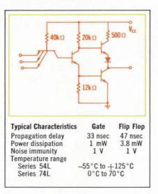
At 1mW per gate, Series 54L/ 74L circuits offer a ten-fold power savings...yet are approximately twice as fast as other circuits with similar power dissipation.
