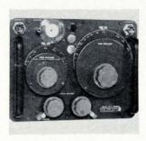
Impedance bridge 1606-B, adaptable to coaxial connectors, measures in the 400-khz to 60-Mhz range. Resistance range of the bridge is 0 to 1,000 ohms, and reactance range is  $\pm$  5,000 ohms at 1 Mhz. At other frequencies the reactance reading must be divided by the frequency in megahertz. Price is \$1,050. General Radio Co., West Concord, Mass. 01781. [375]
