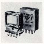
Military relay type PF has contact ratings up to 10 amps, with operate and release time of 7 msec max. Initial circuit resistance is 10 milliohms max., 20 milliohms max. after more than 100,000 operations at 10 amps, 28 v d-c. Unit operates from  $-65^{\circ}$  to  $+125^{\circ}$ C, withstands vibration of 20 g at 10 to 2,000 cps. C.P. Clare & Co., 3101 Pratt Blvd., Chicago. [353]
