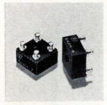
Miniature single-phase bridge rectifier assemblies with ratings up to 2,500 piv mount to p-c boards with one screw; terminals are silver-plated brass for easy soldering. Devices offer piv's of 1,500, 2,000, or 2,500 at current ratings of 1.2, 0.8, or 0.6 amps respectively. Price is \$3.27 each in lots of 1,000. Sarkes Tarzian Inc., 415 N. College Ave., Bloomington, Ind. **[3501**
