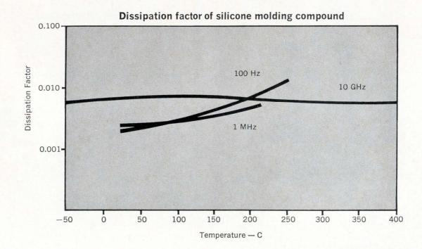
Why the big swing to silicone molded devices? . . . Electrically stable materials over a wide range of temperatures from low to high frequencies—as shown graphically above. Silicone molded packages do not limit the design or performance of high frequency semiconductor devices. Design characteristics will not drift due to changing electrical properties of the molded package.
