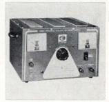
Heavy-duty, solid state supplies series PSR-500 deliver continuously variable 500-w outputs with regulation of line or load to less than 1%, no load to full load. Ripple is less than 1% at max. rated current. Three models are available: 2-32 v d-c, 0-15 amps; 2-55 v d-c, 0-10 amps; and 2-125 v d-c, 0-5 amps. Electro Products Laboratories Inc., 6125 Howard St., Chicago. [388]
