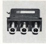
A remote coaxial switch, with 10° cycles minimum lifetime, is a spdt unit with a range of d-c to 12.4 Ghz. Isolation is 60 db minimum over entire range. Insertion losses as low as 0.3 db from d-c to 7 Ghz and 0.6 db from 7 to 12.4 Ghz are claimed. SR-2 series switches are available with N, TNC, BNC, or RSM connectors. RLC Electronics Inc., 25 Martin Pl., Port Chester, N.Y. **[404]**
