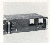
Frequency converter CRS-150A converts 50 or 60 hz single-phase input power to precision, low-distortion 400 hz single-phase output. It delivers 150 v-a, with continuous duty in ambients of  $-20^{\circ}$  to + 60°C. Its sine-wave output has less than 1% total harmonic distortion. Frequency regulation is  $\pm 0.25\%$ . CML Inc., 350 Leland Ave., Plainfield, N.J. 07062. [372]
