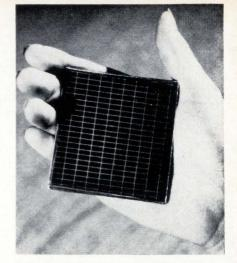
Substitute. Ceramic solar cells replace silicon at lower cost.
