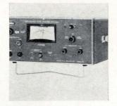
Automatic transfer standard model ATS is a true rms to d-c converter that makes a measurement in 10 seconds for frequencies from 2 hz to 10 Mhz. Accuracies are: 0.1% for a-c signals up to 1,000 v and to 20 khz; 0.02% up to 500 v and to 50 khz; 0.05% up to 16 v and to 1 Mhz; 0.5% up to 8 v and 10 Mhz. Singer Co., 915 Pembroke St., Bridgeport, Conn. [370]
