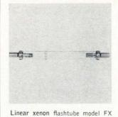
81-4 has a 4-in. arc length. The 10 x 12 mm quartz device handles an energy input of 3,000 joules per flash with a pulse duration of 1.4 msec. Units can be used in environments ranging from ocean depths to outer space. Applications include laser stimulation, medical research, and satellite flashers. EG&G Inc., 160 Brookline Ave., Boston. Mass. [346]
