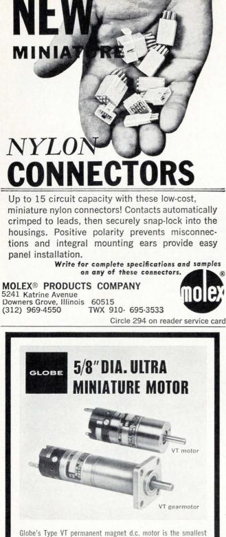
Globe's Type VT permanent magnet d.c. motor is the smallest **standardized** power motor we know about. Fourteen standard armature windings are available for 3 to 50 v.d.c., with no-load speeds from 5,000 to 22,000 rpm. You can apply this miniaturized unit for continuous duty ratings up to 1-1/2 watts, and for starting torques up to 1.0 oz. in. Unit is 5/8'' in diameter by 1-5/8'' long; weight is 1.5 ounces.
