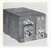
A uhf/f-m transmitter for aerospace telemetry applications delivers 20 w minimum at S-band frequencies in the 2.2- to 2.3-Ghz range. The 3620-01 withstands 55 g shock, 20 g sine-wave vibration, and 30 g acceleration environments. Center frequency stability is within  $\pm$ 0.003% under all environmental conditions. Electro-Mechanical Research Inc., Box 3041, Sarasota, Fla. **[401]**
