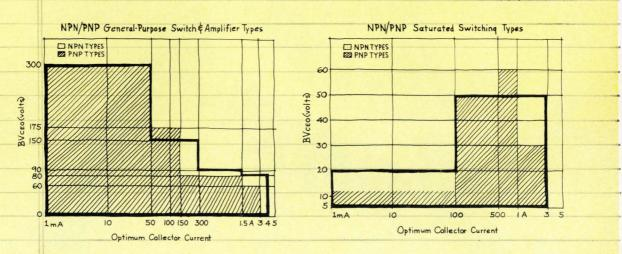
No matter what your application, chances are Motorola has a Silicon Annular transistor to fit it. The charts above are indicative of the broad voltage and current ranges covered. All are fabricated using the Annular Process, Field Relief Electrode or both. Result: State-of-the-art devices -- free of failure due to surface or bulk defects!\*
