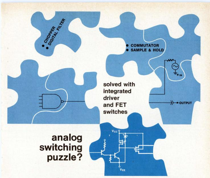
Analog switching got you puzzled? Here's the answer — an integrated circuit with drivers and FET switches all in one package. Drive the input with almost any integrated logic — only 0.8 volt swing is required. The output FET with ON resistance as low as 80 ohms and leakage less than 1 nA can switch plus or minus 20 volt signals.
