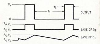
**Output waveforms.** When the potential at the base of  $Q_1$  reaches  $\frac{2}{3}$  Vs,  $Q_1$  turns on,  $Q_2$  turns off, and the output drops to ground, completing the pulse.
