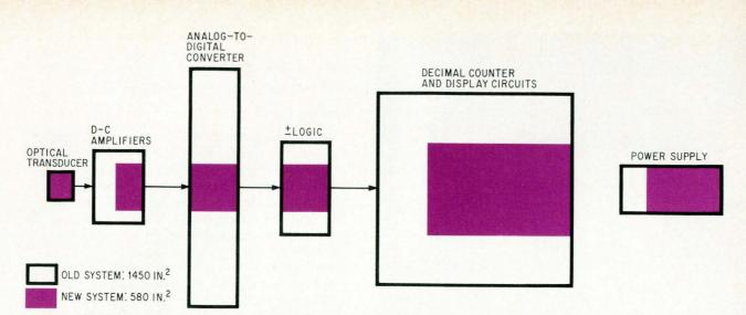
Space saver. Picomm II requires only about 40% of the area needed in the discrete component system.
