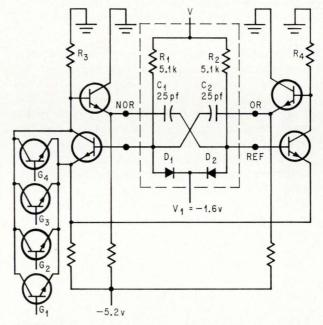
Astable. In the gated astable multivibrator, variable supply voltage V as well as circuit components control the oscillation frequency. Components outside the dashed box are included in the IC chip, a Motorola MC-301.
