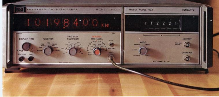
AVAILABLE PLUG-INS: TWO FREQUENCY CONVERTERS (50 MHz TO 500 MHz, 100 MHz TO 3 GHz); PRESCALER (dc TO 1 GHz); PRESET UNIT (20 Hz TO BEYOND 10 MHz); VIDEO AMPLIFIER (1 mV SENSITIVITY, 10 Hz TO 200 MHz); TIME INTERVAL UNIT (100 ns RESOLUTION); NON-COMMITTED PLUG-IN.
