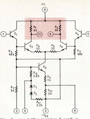
Video. Presence of diffused resistors,  $R_1$  and  $R_2$ , in collector legs of the amplifier marks video-type IC.
