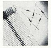
Metal alloy film resistor MAL-20 is a  $\frac{1}{2}$  watt (70°C) semiprecision device for use in color-tv, computers, and industrial instrumentation. It has temperature coefficients of 100 and 150 ppm/°C, and resistance tolerances of 2 and 5%. The unit meets or exceeds requirements of MIL-R-22684. It is epoxy coated and stamped and color-coded. Mallory Controls Co., Frankfort, Ind. [343]
