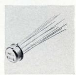
Hybrid IC, d-c wideband amplifier HX610 is offered in a 10-lead T0-5 can. It has built in by-pass capacitors and needs no external components when used as an amplifier with a voltage gain of 26 db. Maximum output voltage swing with no load is 20 v peakto-peak to 8 Mhz, derating to 2.5 v p-p at 100 Mhz. Halex Inc., 139 Maryland St., El Segundo, Calif. [443]
