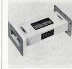
A line of waveguide isolators is based on a patented design that eliminates the external magnet. Series covers 5,925-7,125 Mhz frequency range. Units have 20, 30, or 40 db isolations with maximum losses of 0.5 to 0.8 db. Bilateral vswr is 1.15 maximum. Devices can be furnished with magnetic shielding. E&M Laboratories, 7419 Greenbush Ave., North Hollywood, Calif. [402]
