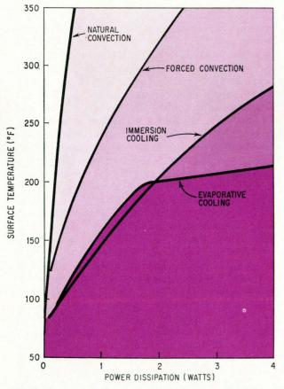
**Tradeoff curves.** Quick comparisons between alternate cooling techniques can be made with families of curves. Efficiency rises and size decreases from left to right in this comparison of methods for cooling TO-5 packages.
