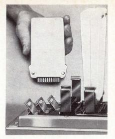
No mistake. Modules and the rails they plug into are engineered to prevent installation mistakes.
