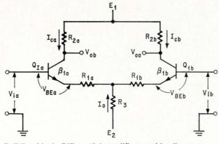
**Building block.** Differential amplifier provides linear IC's with balance (symmetry) and application versatility.
