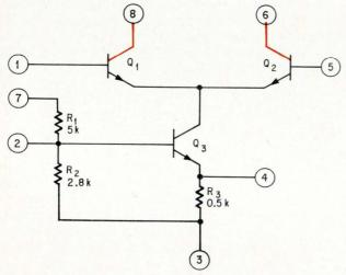
**Narrowband.** Uncommitted collectors of transistor elements  $Q_1$  and  $Q_2$  typify the narrowband differential amplifier.
