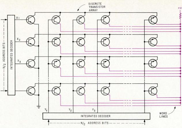
**Common connection.** A positive signal at  $X_1$  forward- biases the first current-sink transistor. This provides a ground connection for the top row of transistor AND gates. A positive signal at  $Y_1$  permits current to pass through only the first gate. Thus line 1 is selected. The word lines are in color.
