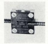
Pressure sensor PSF100A senses level changes in liquids, granular powder semisolids, equivalent to  $^{1/2}$  in. or less of water column or pressure/vacuum and differential in the same range. It is virtually insensitive to shock, vibration, and acceleration. It is 1  $\times$  1  $\times$  11/32 in., and weighs less than 10 grams. Fairchild Camera & Instrument Corp., 225 Park Ave., Hicksville, N.Y. **[367]**
