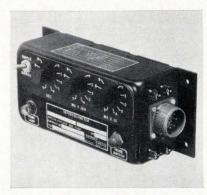
The unit shown above, for example, is programmable in both time and mode. We make others where the sequence, too, can be programmed from the face of the unit. You can select the time interval, with 5% accuracy, from 100 miliseconds to 9.99 seconds, in 0.01 second increments. They are simple to operate, and extremely reliable.
