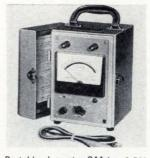
Portable ohmmeter 244 has 0.5% accuracy at center scale. It makes direct readings of resistances from 0.05 to 50,000 ohms. It is calibrated in 4 ranges: 0 to 50, 0 to 500, 0 to 5,000, and 0 to 50,000 ohms. Accuracy is assured by a built-in standard that compensates for battery condition and lead resistance. Associated Research Inc., 3777 W. Belmont Ave., Chicago. [363]
