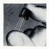
Plastic complementary silicon transistors rated at 360 mw with a maximum operating junction temperature of 150°C can be used to replace the standard 2N2222 series. The TD100 meets MIL-S-19500/255E, with a noise figure of 0.5 db and a minimum gain of 100 at 10 µa. Base-toemitter voltage is matched within 2.5 mv. Sprague Electric Co., North Adams, Mass. [440]
