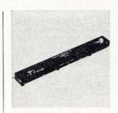
An ultralinear variable magnetostrictive delay line provides continuously variable delays from 2 to 35  $\mu$ sec at frequencies up to 2 Mhz. Unit operates in temperatures from -40° to 85°C and survives shocks of 600 g. Delay is varied by a shaft; normal performance is 167 ns/turn with linearity to better than 0.25%. Digital Devices Inc., 200 Michael Dr., Syosset, N.Y. [351]
