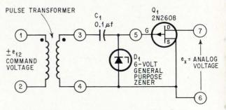
Switching action. Voltage at point 5 is either 6 or zero volts, turning  $Q_1$  off or on, respectively.
