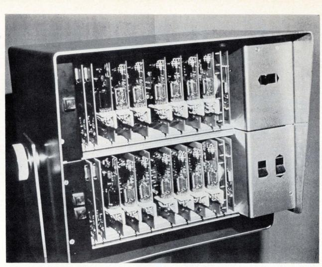
Inside look. With front panel removed, each circuit board with its numercial readout tube can be seen.
