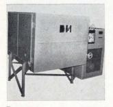
Temperature heating rate of  $-100^{\circ}$ F to  $200^{\circ}$ F in 2 hours and cooling rate of  $200^{\circ}$ F to  $-100^{\circ}$ F in 1 hour are featured in an environmental Thermaline vibration chamber that is insulated with nonsetting, nonhygroscipic Fiberglas/Foamglas. Control is maintained to within  $\pm 3^{\circ}$ F. Environmental Engineering Division, Bethlehem Corp., 225 W. 2 St., Bethlehem, Pa. L4251
