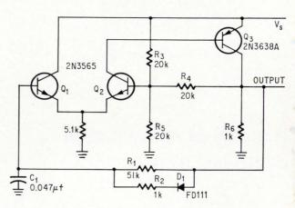
**Nonsymmetrical multivibrator.** Capacitor  $C_1$  is charged through  $D_1$  and  $R_2$  until  $C_1$ 's potential reaches  $\frac{2}{3}$   $V_s$ .
