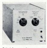
Suited for swept frequency measurements, model 1008 a-c/d-c converter has a 70-db dynamic range, a frequency response from 5 hz to 5 Mhz, and a 300-µv sensitivity. It is applicable for audio and video measurements such as those encountered by telephone companies and filter manufacturers. Pacific Measurements Inc., 940 Industrial Ave., Palo Alto, Calif. [366]
