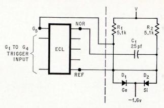
**Monostable.** By rewiring the astable multivibrator a monostable circuit results with fewer components. Circuit to the right of the dashed line represents discrete component addition to the ECL.
