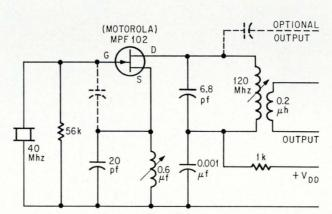
Active element. Use of FET simplifies crystal loading in oscillator-multiplier design. Values shown are suitable for fundamental operation at 40 Mhz, tripling to 120 Mhz.
