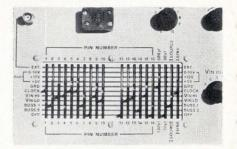
**Programer.** Operator sets up test conditions with contacts that are pushed by hand over printed circuit program boards.
