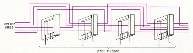
**Transformer memory.** In this word-per-line organization, current through any one word wire generates a voltage pulse in the sense wires of those ferrite cores that the word wire passes through. The cores are U-shaped with ferrite caps to complete the flux path.
