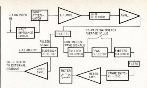
**Two detection paths.** Pulsed input signals are measured with slide-back detector. Either the peak or average value of continuous-wave signals can be measured in second detection circuit.
