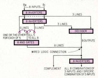
**Selector gate module.** Plugging jumpers into different positions enables this circuit to be used with memories as large as 256 by 256 bits.
