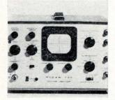
Dynamic flutter analyzer 720 provides precise analysis and measurement of tape recorder flutter. The built-in oscilloscope identifies and measures all flutter-contributing components from 0.2 hz to 10 khz. The analyzer includes a crystal-controlled reference-frequency oscillator. Both sine- and square-wave outputs are provided. Vidar Corp., 77 Ortega Ave., Mountain View, Calif. [369]
