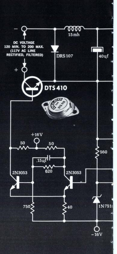
Application of Delco high voltage silicon power transistors
