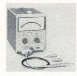
H-f probe 11096A converts d-c voltmeters into a-c instruments that measure signals from 100 khz to 500 Mhz. Accuracy in this range is better than 1 db. Input impedance is 4 megohms shunted by 2 pf. The probe works with analog or digital voltmeters that have input resistances of 10 megohms ±10%. Price is \$45. Hewlett-Packard Co., 1501 Page Mill Rd., Palo Alto, Calif. [371]
