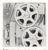
Bidirectional reader/spooler model RRS-502B features a 500-characters/sec reader and a 50-in./ sec spooler equipped with  $101_{2-}$ in. diameter reels. Panel height is 21 in. Price is \$3,580 in small quantities, with discounts for higher quantities. Delivery is 10 weeks. Remex Electronics Division, Ex-Cell-0 Corp., 5250 W. El Segundo Blvd., Hawthorne, Calif. 90250. **[382]**
