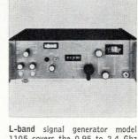
1105 covers the 0.95 to 2.4 Ghz range. The manufacturer's Unidial control system provides singleband continuous tuning with digital frequency indication accurate to  $\pm 0.5\%$ . Frequency stability is 0.0008% per volt change in line voltage and 0.005% per°C change in ambient temperature. Polarad Electronic Instruments Inc., 34-02 Queens Blvd., L.I.C., N.Y. **[407]**
