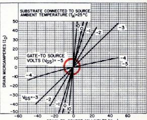
DRAIN-TO-SOURCE MILLIVOLTS (VDS)
