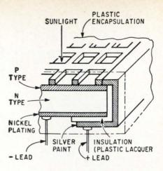
grains of cadmium sulfide are converted to copper sulphide, while the inner portion remains unconverted.
