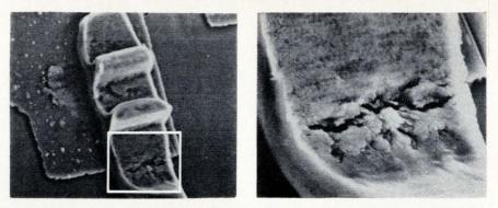
**Flaw.** Scanning electron miscroscope at 1,000  $\times$  magnification (left) and 3,500  $\times$  discloses fault in gold lead ultrasonically bonded to gold pad. This fault would not be detectable by optical methods.
