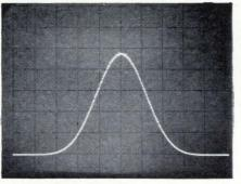
EXCELLENT GAUSSIAN DISTRIBUTION Using HP 5400A Multi-Channel Pulse Height Analyzer, ±250 mw; 1024 channels; Noise Generator: sequence length, 1,048,575; Clock period, 3.33 µsec.
