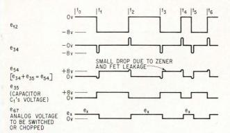
**Waveforms.** Negative steps in command voltage  $e_{12}$  turn the FET off and positive steps turn it on to pass the analog signals.
