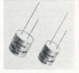
Plastic-cased electrolytic tubular capacitors with epoxy end sealing are designed for p-c transistor circuitry and miniature electronic assemblies. Type EKA units come in 11 different models with capacitance values from 5 to 250  $\mu$ f; and in 3 sizes, the largest being  $15\%2 x^{31/64}$  in. D-c voltage ratings include 3, 6, 10, 15, 25, 35, and 70. Aerovox Corp., New Bedford, Mass. [344]
