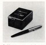
Stabil-ac is a 14-oz d-c/a-c inverter that provides 400-hz output with ripple-free, low-noise characteristics. It is used with airborne, synchronous servo equipment. Frequency stability is  $\pm 0.25\%$ . Adjustable output ( $\pm 1\%$ ) compensates for mechanical tolerances in users' equipment. Price is \$375 in quantities of 1 to 9. MIL Associates Inc., Dracut Rd., Hudson, N.H. [**283**]
