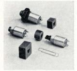
Designed for fast computer circuits, switches are moisture-proof and have less than 1 µs contact bounce after transfer. B5200 and BW5200 series are rated at 3 amps resistive, 1 amp inductive, and 1 amp lamp-load at 28 v dc or 120v a-c. They are available in 3 circuit arrangements with 18 mounting styles. Controls Co. of America, 1420 Delmar Drive, Folcroft, Penn. [341]
