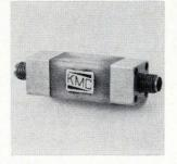
Miniature d-c block, model 754, has a capacitance in series with both the center and outer conductors preventing a flow of d-c current while permitting an uninterrupted flow of r-f power. Typical specifications at 6 Ghz include a vswr of 1.20 max; insertion loss, 0.25 db max; impedance, 50 ohms; and d-c voltage, 100 v. Kevlin Manufacturing Co., 24 Conn St., Woburn, Mass. **[406]**
