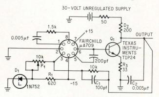
**IC-regulated.** Power-supply regulator is built with an IC operational amplifier and a transistor. Output resistance is 0.05 ohms, ripple and noise less than 1 mv.
