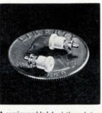
A semiassembled feed-through terminal is for installation in a 0.040-in.  $\pm$ 0.02-in.-thick chassis, mounting in a 0.136-in. hole. Designated FT-2-SM-1200, the terminal's 0.040-in. diameter gold-plated brass lug extends 0.100 in. above and below the Teflon bushing. The unit handles 5.5 amps and can be used from 65° to 200°C. Sealectro Corp., 225 Hoyt St., Mamaroneck, N.Y. [342]
