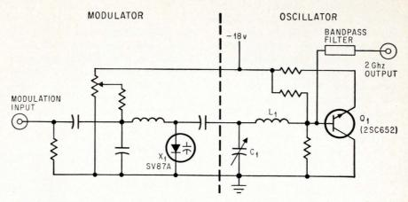
**Do-it-yourself doubler.** Nonlinear collector-to-base capacitance of transistor multiplies basic frequency to 2 Ghz in simplified oscillator for microwave repeater transmitter.
