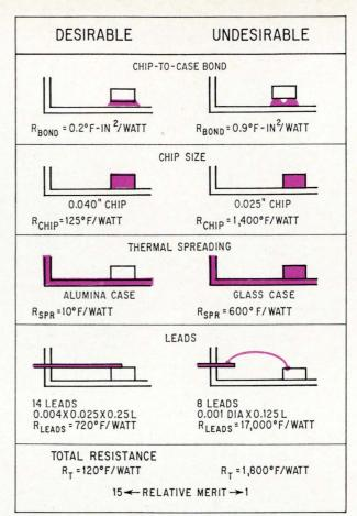
**Package problems.** Thermal characteristics of integrated circuit flatpacks can vary as much as 15:1 because of differences in construction, processes, materials, and dimensions. In each illustration, color shows the part responsible for the thermal resistance value given.
