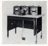
Model 1400 console enables the welding of insulated tape cable to itself or to connector terminals without prestripping the insulation. It includes 2 a-c power supplies, 1 d-c supply, an a-c/d-c controller, and a weld head with 4 electrodes (2 above and 2 below the items being welded). Copperto-copper welds take  $\frac{1}{2}$  sec. Wells Electronics Inc., 1701 S. Main St., South Bend, Ind. [424]
