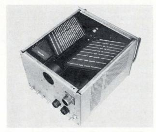
**Chevron.** Air stream cools more efficiently when circuit cards are placed at  $120^{\circ}$  angle rather than the usual  $90^{\circ}$ .
