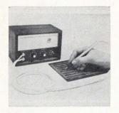
Pulsemeter soldering system features pencil-type holder and miniature parallel-gap electrodes. Both time and current can be preset to control heat delivered. Time settings range from 0.1 to 1.0 sec; current settings, from 10 to 35 amps. Uses include IC flatpack soldering, and thin- and thick-film soldering. Development Associates Controls, 725 Reddick Ave., Santa Barbara, Calif. [421]
