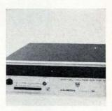
**Programable**, digital volt-ratio meters series 6600 handle 1,000 samples per sec. Accuracy is within  $\pm 0.01\%$  of full scale  $\pm 0.017\%$  of reading for 6 months over a temperature range of 10° to 40°C. With the optional millivolt preamp accessory, the 6600 automatically ranges from  $\pm 10.999$ mv to  $\pm 1099.9$  v d-c full scale. Lear Siegler Inc., 1152 Morena Blvd., San Diego, Calif. [376]
