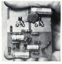
Hand made. Collector lead is connected to area of copper in a circuit developed to test the power dissipation of the TIS90.
