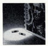
A resistor 0.040 in. in diameter and 0.130 in. long operates from 1 x 10<sup>8</sup> to 1 x 10<sup>12</sup> ohms with a tolerance of  $\pm 25$ %. It handles temperatures to 100°C and with a compatible epoxy can be readily encapsulated. The ends of the resistor serve as terminals for direct soldering to terminal board and circuit component connections. Pyrofilm Resistor Co., 3 Saddle Rd., Cedar Knolls, N.J. [355]
