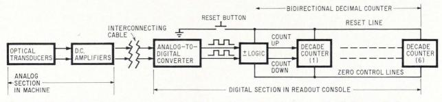
**System design.** Both the horizontal x- and y-axis of the machine sense probe movement with linear optical transducers and convert signals to digital form. The z-axis uses rotary position encoder to save space.
