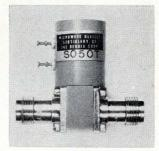
Shutter switch model SO50T operates from 2.4 to 11 Ghz with a vswr of less than 1.30. Insertion loss is under 0.4 db, and isolation exceeds 30 db in the normally open position at 11 Ghz. Switching time is 0.01 sec, operating life greater than 100,000 cycles. The switch weighs 3 oz, is  $15/8 \times 3/4 \times 17/8$  in. Bendix Micro-wave Devices Inc., Farmington, Conn. 06032. **[408]**
