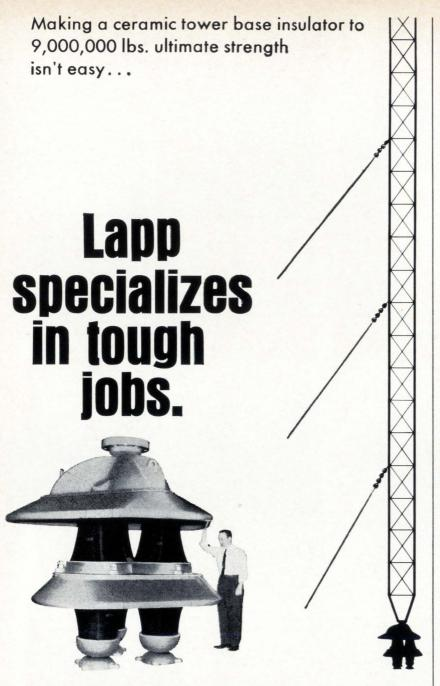
That was one of our toughest. But, Lapp has designed and built hundreds of tower insulators. They range downward to 80,000 lbs. ultimate strength. In fact, Lapp insulators support most of the world's larger radio towers, both selfsupporting and guyed masts.
