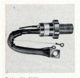
Series NL-C180 are silicon controlled rectifiers with voltage ratings from 100 to 1,300 v. Devices are all-diffused, shortedemitter types with 235 amp rating. Minimum dv/dt rating is 200 v/ $\mu$ sec; maximum di/dt ratings, up to 100 amps/ $\mu$ sec. Peak on-voltage is 1.8 v. Hard solder construction yields low thermal fatigue. National Electronics Inc., Geneva, III. [436]
