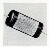
Current-regulating diodes with working currents from 0.22 to 4.7 ma come in a 32-device series. The 1N5283 through 1N5314 are field effect diodes that provide constant currents independent of voltage. Devices offer a peak operating voltage of 100 v, 600 mw power dissipation. Prices are from \$4.90 for 100 units. Motorola Semiconductor Products Inc. Phoenix, Ariz [439]
