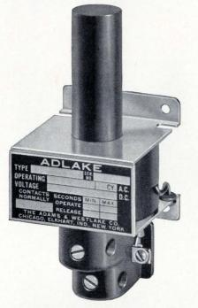
Varying ambient temperatures have little or no effect on Adlake Mercury Displacement Time Delay relays. From the graphic illustrations, ambient temperatures up to  $200^{\circ}$  F or down to  $-37.8^{\circ}$  F (freezing point of mercury), the change in timing is less than 10%.
