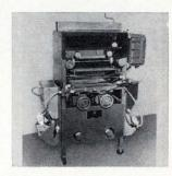
Roller coater for applying thinfilm photoresist materials to p-c boards has a double-pumping system for automatic cleanup, ground rolls, dial indicators for thickness adjustment, and separate drive systems for doctor roll and coating roll. Coater operates at any speed from 3 to 9 ft per minute. The unit will accept boards up to 1 in. thick. Union Tool Corp., Warsaw, Ind. [428]
