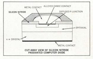
Superior electrical characteristics are now combined with this built-in reliability in General Instrument's line of high-speed silicon nitrided diodes in miniature DO-35 or DO-7 packages for computer applications.
