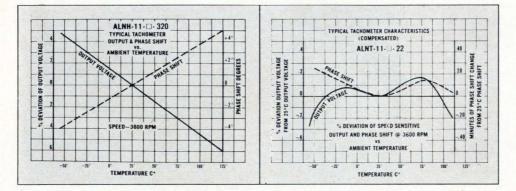
In precision computing applications using integrating tachometers, variations in output characteristics with temperature must be held to a minimum. To obtain the required performance, Clifton, Division of Litton Industries employs temperature compensation.
