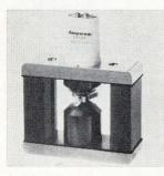
A rising sun magnetron that delivers 5-nsec pulses of 95-Ghz energy at 10 kw has a 3.2-mm wavelength output. Output figure of the DX287 lies in the center of an atmospheric window where the attenuation is much lower than that at other frequencies in the mm region. Duty cycle of 0.0002 allows repetition rates to 40 khz. Amperex Electronic Corp., Hicksville, N.Y. [405]
