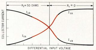
Shaping. Emitter degeneration, introduced by placing a
