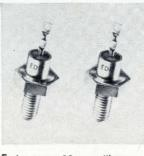
Fast recovery 12-amp silicon rectifiers designated JAN 1N3889 through 1N3893 meet MIL-S-19500/304(EL) specs. The series is for high-reliability military equipment using high-frequency sine wave, square wave or pulsed inputs. Applications include inverters, modulators, converters, and accelerators. Electronic Devices Inc., 21 Gray Oaks Av., Yonkers, N.Y. 10710. [442]
