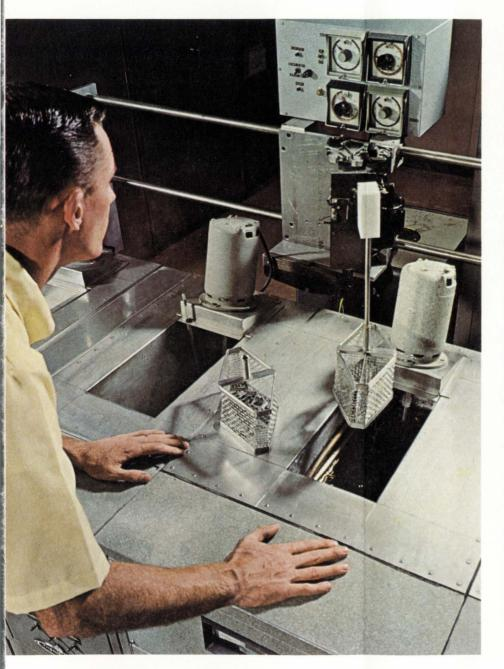
Recently-completed reliability tests, such as the one for temperature-cycling shown here, have proved the ruggedness and durability of TI's plastic dual-in-line package for integrated circuits. Now you can take advantage of reduced initial costs – plus big savings in handling, assembly and testing – without compromising essential reliability.
