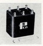
An interstage pulse transformer— 1 cu in. in volume and weighing 75 grams—operates up to 50,000 ft, withstands thermal shock and h-f vibration to 50 g, and environmental temperature from  $-54^{\circ}$ to  $+110^{\circ}$ C. With a working voltage of 10 kv d-c, it has a 1:1 turns ratio, a 0.05-#sec rise time, and meets MIL specs. PCA Electronics Inc., 16799 Schoenborn St., Sepulveda, Calif. [352]
