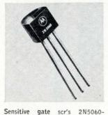
2N5063 are rated at 800 ma (forward current rms) with voltage ranges from 30 to 150 v in a TO-92 Unibloc plastic package. Gate current requirement is 200 µa. Uses are in fractional h-p motor controls, sensing and detection circuits. Prices range from 51 to 85 cents (100 and up). Motorola Semiconductor Products Inc., Box 13408, Phoenix, Ariz. [441]
