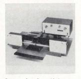
Pantograph reflow-soldering system RS-334 consists of a power supply, 2 reflow-soldering heads, a pantograph p-c board positioning mechanism, and an IC loading/ placement fixture. It positions an IC on its mounting board and solders as many as 14 leads at once. Each soldering head has interchangeable electrode-tip configurations and sizes. Sippican Corp., Mattapoisett, Mass. **[422]**
