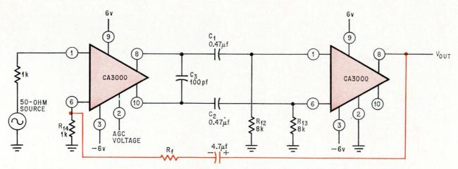
**Cascade.** Feedback amplifier using two video-type differential amplifying IC's and RC-coupling network. Besides providing 62 db of gain, subsystem has automatic gain control capability.
