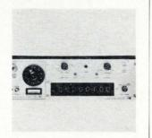
Frequency counter 5247M counts directly from 10 hz up through the communications bands to 135 Mhz. With frequency converter plug-ins, the range can be extended to 18 Ghz. The instrument has a time-base oscillator with short-term stability of better than  $5 \times 10^{-11}$  rms for a 1-sec averaging period. Price is \$3,000. Hewlett-Packard Co., 1501 Page Mill Rd., Palo Alto, Calif. [374]
