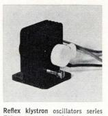
EM-1149 are useful as pump tubes for parametric amplifiers. The 5,000-hr warranty tubes, operating from 12 to 18 Ghz, are available in 2 versions. One offers an output of 1 w over a 500-Mhz tuning range; the other, 1.5 w over a 100-Mhz range. The 7oz tube mounts in any position. Varian Associates, 611 Hansen Way, Palo Alto, Calif, **[403**]
