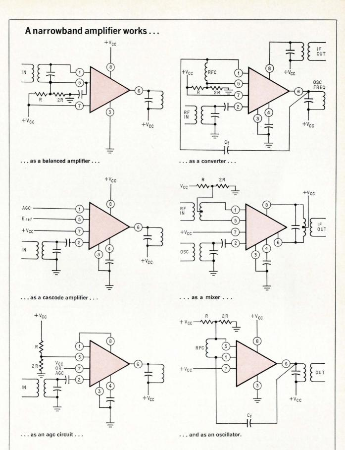
**Broad base.** The application versatility of the narrowband differential amplifier is largely due to its uncommited collector arrangement. Relatively few changes are required in terms of the lead pins used; designers merely alter the external network connected to the IC to meet various applications. The unit shown here is the CA3020, popularly known as the universal IC.
