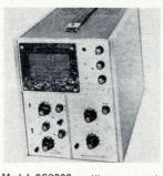
Model OS2000 oscilloscope, made by Xetex Electronics, England, has 20-Mhz bandwidth with sensitivity of 10 mv/cm. There is a choice of single- or dual-trace and highgain differential amplifiers, and standard or delayed-sweep time bases. Signal delay of 200 nsec ensures that the leading edge of an acceptable waveform is clearly visible. Alban Electronics, 111 Cedar Lane, Englewood, N.J. [373]
