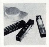
Reed relay series 325-12-1A measures 1.4 x 0.25 in. sq. with 0.1-in. pin spacing for standard p-c layout techniques. Direct p-c mounting eliminates changes in reed characteristics caused by cutting and bending of axial-lead types. The spst contacts switch in less than 1 msec, and are rated at 4 v-a into a resistive load. Self-Organizing Systems Inc., Box 9918, Dallas. [356]
