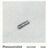
Photocontrolled resistor type 5082-4510 uses a cadmium-sulfoselenide photocell for stability in a changing temperature environment. Photocell resistance, when illuminated, changes typically by a factor of 1.5 with a variation in temperature from 25° to 65°C. Units cost \$8 each in small quantitles, and \$6.80 for 10 to 99. Hewlett-Packard Co., 1501 Page Mill Rd., Palo Alto, Calif. [438]
