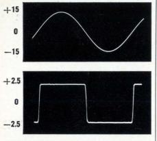
SIMULTANEOUS SINE AND SQUARE-WAVE outputs pack real power (up to ½ watt into 50 ohms). Photos show open circuit output voltages at 1 MHz.
