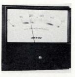
The Centurion line of electrical meters has easy-to-read scales, recessed glass window to minimize marring, and glare-free scale illumination. D-c current sensitivities are available from 5  $\mu$ a through 50 amps with self-contained shunts. D-c voltage sensitivities are from 3 mv through 500 v with self-contained multipliers. Beede Electrical Instrument Co., Penacook, N.H. [362]
