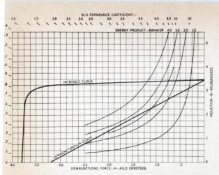
With a coercive force of 3200 oersteds, Indox 7 has a higher resistance to demagnetization than any commercially available magnetic material except costly platinumcobalt. It also has a high peak energy product and high intrinsic coercive force.
