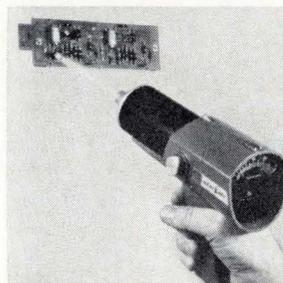
Heat-Spy model HS-8 handles selective noncontact temperature measurement of small components. The exact target area is defined by a light beam which enables the operator to aim at objects 0.1 to 0.4 in. in diameter. The instrument is available in 4 models covering 60° to 1,000°F. Its accuracy is  $\pm 2\%$ . William Wahl Corp., 1001 Colorado Ave., Santa Monica, Calif. [374]
