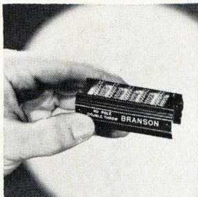
A 40-pole, double-throw relay package has 2-amp, 28 v d-c resistive contacts. The SR package eases replacement of individual switching units, eliminating the need to replace the complete unit. The sealed relays operate in a -65° to +125°C range, withstand 50 g shock for 11 msec, 20 g vibration from 10 to 2,000 hz. Branson Corp., Vanderhoof Ave., Denville, N.J. [350]
