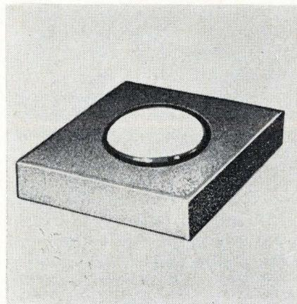
**Contact.** White dot on diode chip is junction contact.
