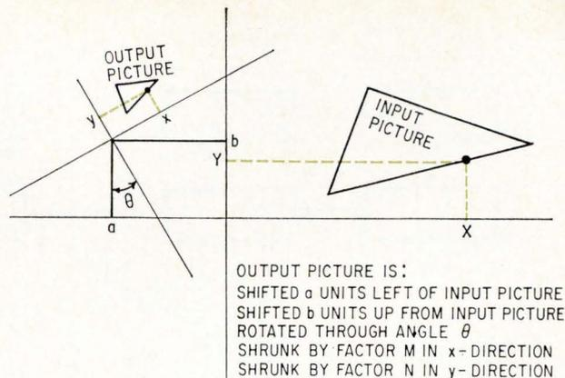
**Shifting output picture.** Limits on horizontal and vertical movement are those of the scan; angle of rotation is unlimited. The size can be increased or decreased. The transformation equations are derived from the quantities in this diagram.
