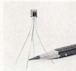
Silicon planar npn Darlington transistors 2N2723-4-5 are 2 transistor chips mounted in either a 3- or 4-lead TO-18 package. Characteristics include  $h_{FE}$  within 10%,  $V_{BE}$  matched within 30 mv, and temperature tracking within 100  $\mu v/^{\circ}C$ . Applications are constant-current supplies and voltage comparators. Solitron Devices Inc., 1177 Blue Heron Blvd., Riviera Beach, Fla. [439]
