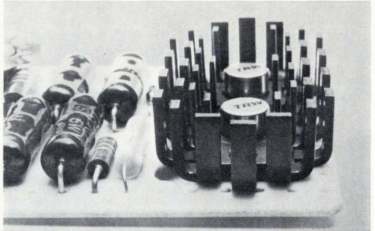
Fan-top dissipators for TO-5 and TO-18 cases drop temperatures dramatically; cost just pennies. T-shape adds almost nothing to board height; allows components to snuggle close to transistors. Spring fingers provide fast, press-on installation.
