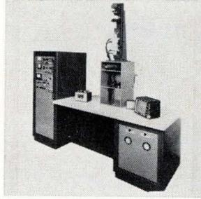
Resistor trimming is performed by an automatic laser system suitable to production use. Safety to the operator or persons in close proximity is assured by light-tight seals and safety interlocks. The system has been tested for 100,000 discharges and operates continuously at rates up to 1 pps. Prices start at \$17,500. Space-rays Inc., Northwest Industrial Park, Burlington, Mass. [423]
