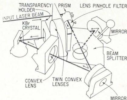
**Crystal set.** Diagram shows how light travels among prototype components set up in photo at left to record analog data such as photos or drawings. After exposure, a joy stick is used to lift the beam splitter out of optical path, and the crystal can be viewed from the rear. In this early model, the stepping motor for the KBr crystal holder is below the table.
