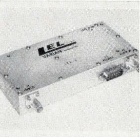
Logarithmic amplifier ITL-5, for microwave receivers, provides a log video output with a 70-db input dynamic range. Video output is proportional, within  $\pm 2$  db, to the log of the input from -60 to +10 dbm. The unit is available at 30- or 60-Mhz center frequency, 4- or 8-Mhz bandwidth. It operates in a 50-ohm i-f system. Price is \$325. LEL Division, Varian Associates, Akron St., Copiague, N.Y. [405]
