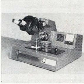
Ultrasonic die bonder DU-6 attaches dice to devices ranging from large stud packages to small headers or flatpacks. Ultrasonic energy is supplied by a 10-watt 40-khz generator. The dice are picked up by vacuum and a slide with the heater column holding the work is moved rapidly into place for bonding. Axion Corp., 6 Commerce Park, Danbury, Conn. [422]
