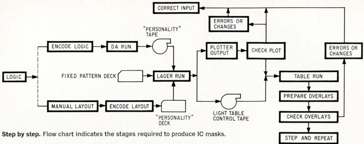
Step by step. Flow chart indicates the stages required to produce IC masks.
