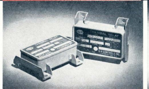
The PT Series relays provide the most precise performance available in thermal relays. Meet the exacting military requirements for reliability under extreme operating environments. **Features:**  $\pm 5\%$  tolerance over a temp. range of  $-55^{\circ}\text{C}$  to  $+125^{\circ}\text{C}$ ; 2000 Hz vibration; 50g shock; time delays, 3 to 180 sec.; heater voltages, 6.3, 28 and 115V AC or DC.
