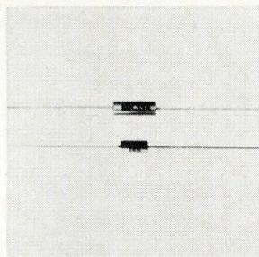
Molded metal film resistors conforming to MIL-R-10509E come in 2 types. The MR-31 and MR-39 have wattage ratings of 0.1 and 0.125 respectively. Units have a ceramic core on which a metal film is deposited. End caps make contact with the resistive film. Tinned copper leads are resistance welded to the end caps. Mepco Inc., Columbia Road, Morristown, N.J. [354]
