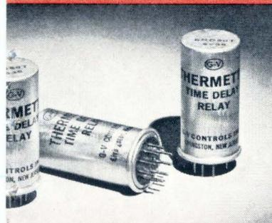
Each enclosed thermal time delay is shatter proof and shatter proof — designed for industrial applications requiring reliable operation and long life. **Features:** temp. compensated; time delays, 2 to 180 sec.; heater voltage, 6.3, 26, and 115V. AC or DC; contacts, SPST, NO or NC.
