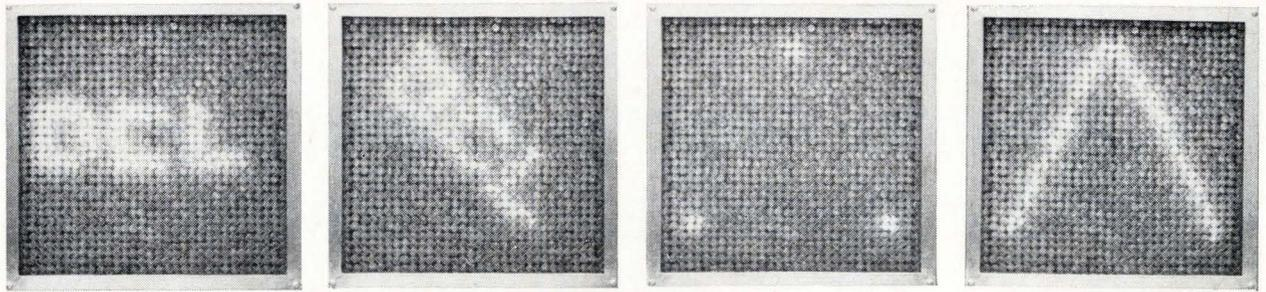
**Alphanumeric display.** Normal and rotated positions are at left. Other photos show how Paramatrix can fill in large gaps in an input picture.
