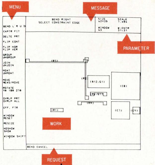
Screen areas. Five basic sections of the screen used by the designer to develop an IC layout.
