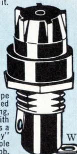
Fuseholder only  $1\frac{5}{8}$  inches long, extends just  $\frac{29}{64}$  inch behind front of panel. Takes  $\frac{1}{4} \times 1\frac{1}{4}$  inch fuses. Holder rated at 15 ampere for any voltage up to 250.
