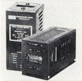
A universal dual-output power supply named Unitwin-164 meets MIL-E-5272 and related specs. It provides 2 voltage outputs adjustable between 0 and 25 v at 0.750-amp capacity for each section. Regulation is better than  $\pm 0.005\%$  or 1 mv for line and load. Output impedance is 0.0032 ohm or less to 1 khz. Power/Mate Corp., 163 Clay St., Hackensack, N.J. 07601. [381]
