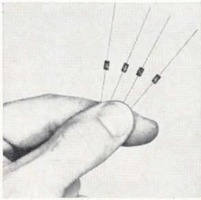
Subminiature ceramic tubular capacitors series CT07 are rated at 50 v d-c over a temperature range of  $-55^{\circ}$  to  $+125^{\circ}$  C. Capacitance values are from 10 to 10,000 pf in tolerances of  $\pm 10\%$  and  $\pm 20\%$ . The capacitors exceed the requirements of MIL-C-11015. They measure 0.165 x 0.095 in. Gulton Industries Inc., 212 Durham Ave., Metuchen, N.J. [341]
