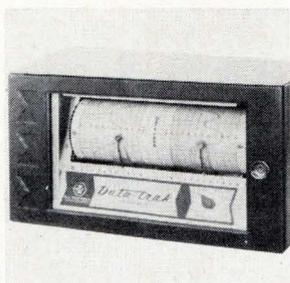
Data-Trak 5110-2P is an electrostatic curve follower with 2 curve-sensing probes which track the individual x and y coordinate data plotted on a Mylar chart. A precision pot is servocoupled to each probe to translate graphical data to equivalent electrical outputs. The unit is suited to any process requiring 2 synchronized and programmed signals. Research Inc., Box 6164, Minneapolis. [369]
