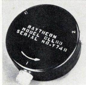
Coaxial L-band circulator model CLL-83 operates at 1.2 to 1.4 Ghz. It has a maximum vswr of 1.20, maximum insertion loss of 0.3 db, and minimum isolation of 20 db. The unit has a Y package configuration. It can also be supplied with 1 port terminated for isolator uses. The circulator is 3 $\frac{1}{8}$  in. in diameter, 1 $\frac{1}{2}$  in. thick. Raytheon Co., 130 Second Ave., Waltham, Mass. [407]
