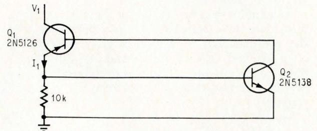
**Triggering.** Current  $I_1$  flows in the direction indicated after the reverse-biased base-emitter junction of  $Q_1$  breaks down.
