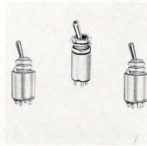
Rfi-shielded toggle switches attenuate conduction and radiation in the 0.14- to 200-Mhz range. They are suitable for radiation-free airborne electronic equipment conforming to MIL-I-26600. Series TR2100, 2150, and 3100 have an operating torque of 20 in.-oz max. Prices start at \$7.56. Control Switch Division, Controls Co. of America, 1420 Delmar Dr., Folcroft, Pa. [343]
