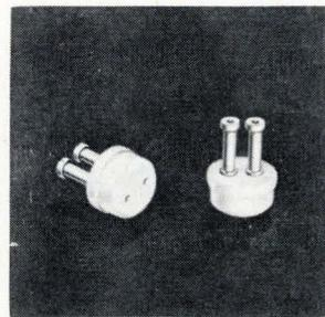
Two-pin, feed-through terminal FT-MC-300 features tubular lugs mounted in a single Teflon bushing suited for multiconnection applications in compact assemblies. Component leads come up from beneath the chassis, through holes in the lugs, and are then soldered in place. Circuit wiring can be attached to the outer lugs. Sealectro Corp., 225 Hoyt St., Mamaroneck, N.Y. 10543. [347]
