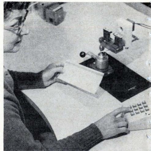
**Dialing trouble.** Western Electric is computerizing its testing of crystals. Information is entered through a touch-tone dial system.
