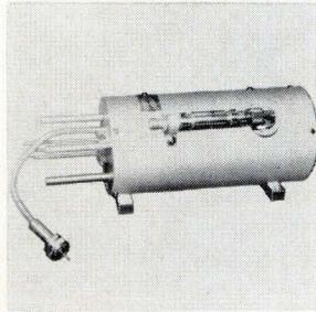
Class C pulse-cavity oscillator 11005 is a 2.5-kw unit that is tuned manually and covers 410 to 460 Mhz. Applications include drone control circuitry and a h-f test source. The unit is rated at 35% efficiency and has a duty cycle of 0.00015. Maximum input vswr is 2:1. Dimensions are 11 $\frac{1}{16}$  x 3 $\frac{1}{2}$  in. Microwave Cavity Laboratories Inc., 10 N. Beach Ave., LaGrange, Ill. [402]
