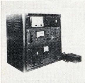
Magnetic stabilizer model MS-10 fully charges and stabilizes metallic alloy magnets up to ¼ lb with a stabilization accuracy within 2%. It is capable of up to 1,000 charging cycles per hour. It is available in 115-v or 230-v models with single pushbutton or foot pedal operation. Instrumentation Division, Thomas & Skinner Inc., 1120 E. 23d St., Indianapolis, 46207. [361]
