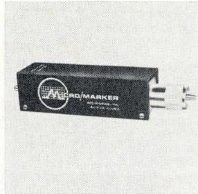
The Micro/marker is a crystal controlled, time-mark generator. The battery-powered unit provides a harmonic output of approximately 1 v peak-to-peak with an output impedance of 50 ohms. Stability is better than  $\pm 0.01\%$  from 0° to +60°C. The unit is packaged in a 1¼ x 1¼ x 4½ in. aluminum case. Price is \$59.50. Accutronics Inc., 12 South Island, Batavia, Ill. [367]
