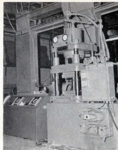
Press. Resin is cured in the mold.
