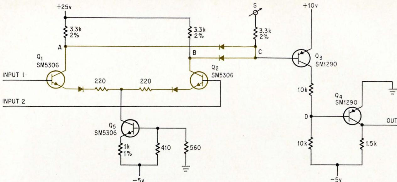
**Comparator circuit.** A binary 1 output appears when the two inputs are equal within a sensitivity margin determined by the setting at S. The circuit portion in color does the actual comparing. Point C follows the lower of the two collector voltages A and B, depending on which transistor is conducting more heavily.
