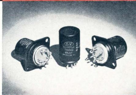
The LT Series relays provide hi-level performance in a subminiature hermetically sealed housing — space saving without loss of performance. Meets military standards. **Features:** height above mounting panel 40% of standard relays (7 pin flange mount); time delays, 2 to 75 sec.; operating temp.,  $-65^{\circ}\text{C}$  to  $\pm 85^{\circ}\text{C}$ ; operating voltages, 6.3 to 115V AC or DC.
