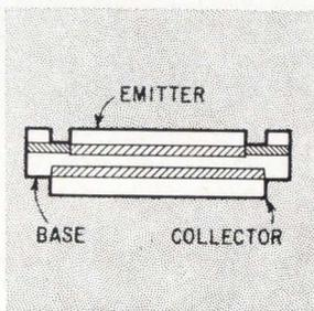
Utilizing the ADE (alloy diffused epitaxial) construction process, the MP2200A-2400A germanium transistors are suited for core driving, power conversion, and high-voltage switching where high power handling capability (80 to 120 v minimum at 8 amps) is needed. Prices range from \$2.25 to \$2.60. Motorola Semiconductor Products Inc., P.O. Box 995, Phoenix, Ariz. 85001. [442]
