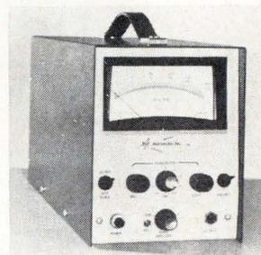
Portable strain gauge and transducer indicator model 1-115SI is an input conditioning module with integral power supply, amplifier, and meter readout. It accepts inputs from 1, 2, and 4 active arm bridges using input wiring up to 8 wires, plus shield. Accuracy is  $\pm 0.5\%$  full scale in 4 ranges to 20 mv. Price is \$475. B&F Instruments Inc., Cornwells Heights, Pa. 19020. [372]
