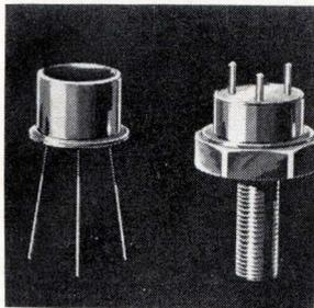
Silicon npn transistors A200/A201/A202 serve as class C r-f amplifiers. Power output is 1w, 7 w, and 12 w; gain is 10 db, 6 db, and 6 db, respectively. The inherently fail-safe units are intended for use in 12 v, battery-operated 175 Mhz mobile communication systems. Semiconductor and Receiving Tube Division, Amperex Electronic Corp., Slatersville, R.I. 02876. [436]
