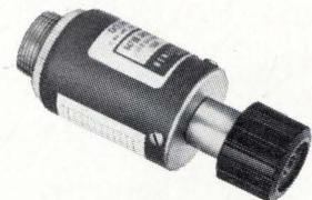
Coaxial thermistor mount for HP 431C Power Meter measures power in coax from 10 MHz to 18 GHz. Features low swr over entire range, zeroing holds for all measurement impedance, and units are temperature compensated for low drift. Mount efficiency data provided for highest measurement accuracy. Unit has Type N male connector (optionally available with 7 mm APC-7 connector). Model 8478B, \$275.
