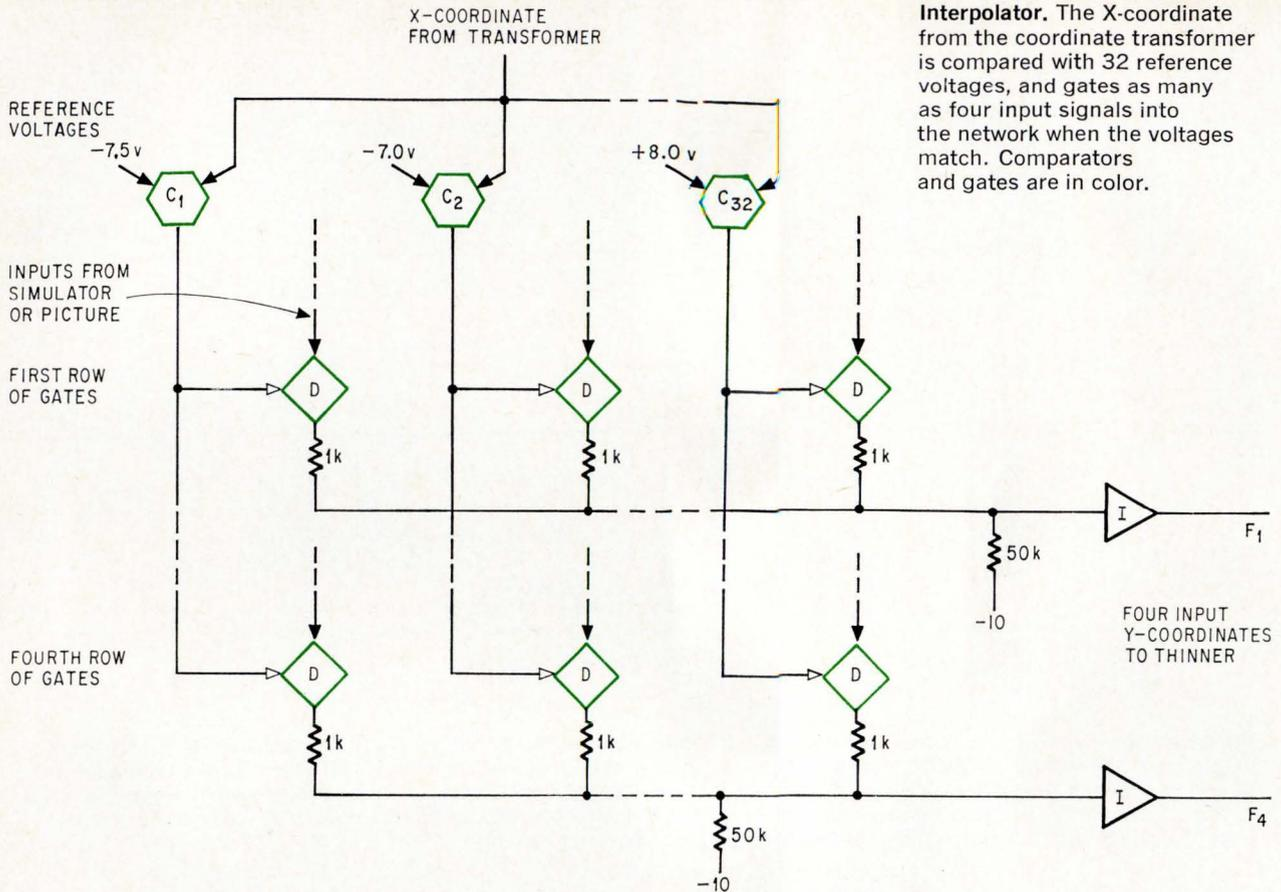
**Interpolator.** The X-coordinate from the coordinate transformer is compared with 32 reference voltages, and gates as many as four input signals into the network when the voltages match. Comparators and gates are in color.
