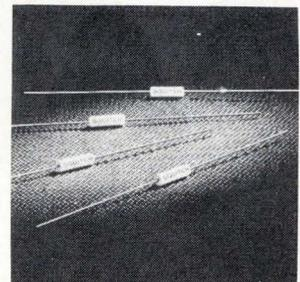
A radiation-hard squib firing switch withstands nondestructive testing. Called Squitches, the 2-terminal devices are made of Ovonic amorphous semiconductor materials encapsulated in standard DO-7 glass envelopes. Blocking resistance is over 1 megohm in the off-condition, switching speed, less than 1 nsec. Energy Conversion Devices Inc., 1675 W. Maple Rd. Troy, Mich. 48084. [443]
