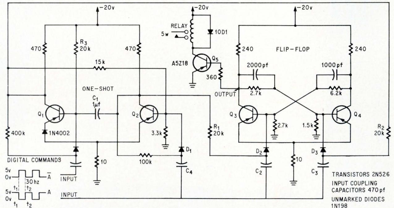
**Operating sequence.** Leading edge of  $\bar{A}$  at  $t_1$  triggers the one shot to start the timing. If the command pulse is short,  $Q_2$  turns on and fires the relay.
