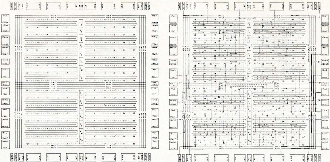
**Mask layout.** Both placement and wiring are laid out at left to indicate a final circuit scheme. Horizontal rows of dots indicate the vertical wiring positions; three solid lines between these rows indicate dual NOR circuits. By adding metal and diffused lines, the designer defines his final layout. Rectangles represent inputs to the circuit.
