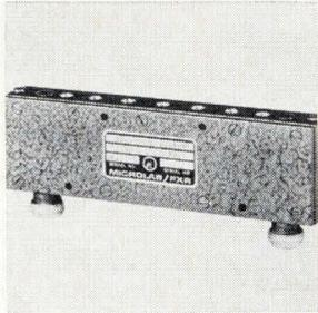
Coaxial bandpass filter model BK-51FN, covering 2.2 to 2.3 Ghz, is useful in telemetry receivers and down-converters. It offers high rejection-band characteristics—50 db at 2.04 and 2.46 Ghz—with 80 db image rejection. Insertion loss is 0.5 db, and vswr is 1.5 max. Price is \$275. The unit is available from stock. Microlab/FXR, 10 Microlab Rd., Livingston, N.J. 07039. [406]
