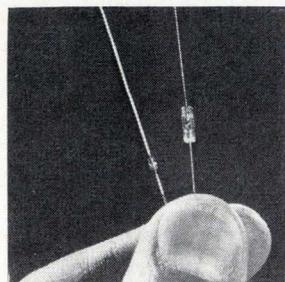
Mini-Mono, whiskerless glass diodes 1N5315 and 1N5316 are less than 1/8th of the standard subminiature DO-7 glass package. Minimum breakdown voltage at 10  $\mu a$  is 100 v. Forward voltage drop at 10 ma is 0.650 and 0.690 v minimum for the 5315 and 5316. Reverse current at 50 v is 50 na. Continental Device Corp., 12515 Chadron Ave., Hawthorne, Calif. 90250. [441]
