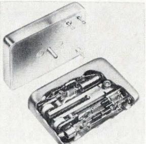
Tuning-fork oscillator LCG-2 is offered in discrete frequencies from 400 to 8,000 hz. Accuracy is 0.050% at 25°C. Output voltage at nominal d-c input is 6 v peak-to-peak 50% clipped sine-wave into 6,000 ohms through an external d-c blocking capacitor. D-c input voltage is 12 v at 3.33 ma. Price is under \$32. Philamon Laboratories Inc., 90 Hopper St., Westbury, N.Y. 11590. [385]
