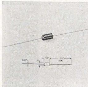
Axial-lead silicon rectifiers rated at 2 amps have a surge rating of 200 amps. Piv ratings range from 50 to 1,200. The devices are 0.2 in. in diameter and 0.38 in. long with a transfer molded, void-free body. They replace 3/16-in. stud units and eliminate heat sinks. Price of a typical unit—the MIBO (200v)—is 64 cents each. Electronic Devices Inc., 21 Gray Oaks Avenue, Yonkers, N.Y. [437]
