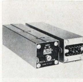
Amplifier model 2227A is a 15-pin device for voice frequency repeater systems. The low-frequency response may be adjusted for a flat characteristic or a roll-off at 200 hz. The unit has an input-output impedance of 600/1,200 ohms and operates on either 48 to 52 or 24 to 26 v d-c. Altec Lansing Division, LTV Ling Altec Inc., 1515 S. Manchester Ave., Anaheim, Calif. [383]
