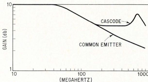
**Resonant peak.** Unlike the single common-emitter stage, whose frequency response is fairly flat, the cascode amplifier has a resonant peak. A variable capacitor,  $C_1$ , controls peak position. When  $C_1$  is increased, the resonance is shifted to a lower frequency and a higher amplitude. This circuit has an 18-db gain and a 550-Mhz bandwidth.
