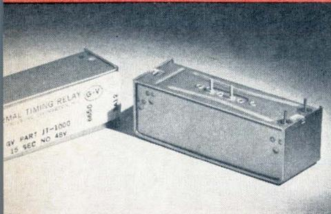
This series is the only thermal relay designed to be mounted directly on pc boards without need for sockets or sockets. This design conserves space, reduces weight, allows greater packaging densities. **Features:** time delays, 2 to 180 sec.; contact types, SPST, NO or NC; heater voltages, 6.3 to 115V AC or DC; temperature compensated; operating in any position.
