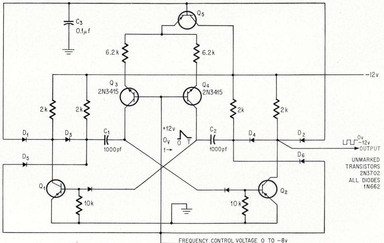
**Astable multivibrator.** Frequency control voltage is applied to the bases of  $Q_3$  and  $Q_4$  and the cathodes of  $D_3$  and  $D_4$  to increase the multivibrator's controllable frequency range by 50%.
