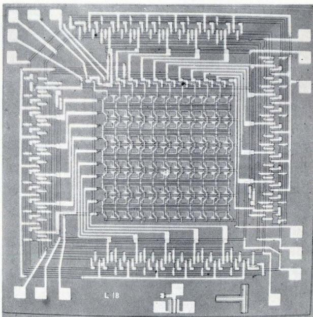
**Ultracomplex array.** More than 600 elements are crammed into the Plessey Co.'s linear array, including a 10-by-10 matrix of photodiodes and scores of MOS-transistor amplifiers. MOS input impedance levels approximate those of optoelectronic units, whereas bipolar impedances are orders of magnitude lower.
