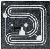
The TIXS67 is a p-channel silicon enhancement-mode field-effect transistor. It is the first such device to be encapsulated in plastic.
