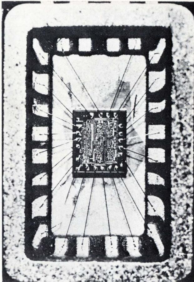
**MOS analog array.** Chip containing 230 MOS-transistor elements, General Instrument Corp.'s digital differential analyzer, performs such linear jobs as function generation and analog computing.
