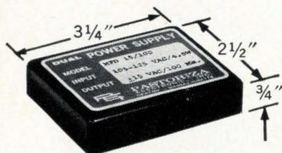
**MODEL MPD 15/100** is designed for use with operational amplifiers, instruments and systems. It provides  $\pm 15$  VDC @ 100 Ma output from 110 VAC input, in a package only  $\frac{3}{4}$ " high including the power transformer. MPD 15/100 represents the first significant step in power supply miniaturization. The systems designer can now take full advantage of the comparable reductions in his circuits brought about by hybrid techniques.
