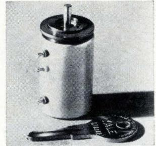
Ten-turn precision pot 2110 meets MIL-R-12934E, RR1000. It is servomounted, 7/8 in. in diameter, wirewound, and offers ±0.25% independent linearity. Available in resistance values from 100 to 50,000 ohms, the units give more than 20,000 cycles of rotational life. They withstand 15 g shock. Amphenol Controls Div., Amphenol Corp., 120 S. Main St., Janesville, Wis. [348]
