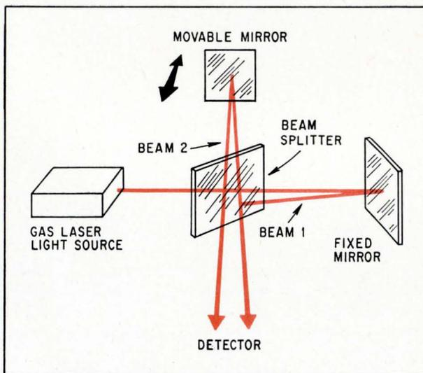
**Michelson interferometer.** Light beam from gas laser is split, reflected from fixed and movable mirrors and then recombined at photo detector.
