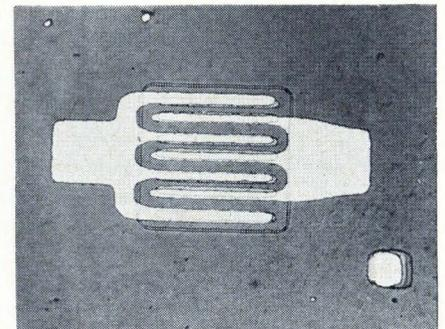
**Wave maker.** A rearrangement of internal geometries permits the L-187 to put out 100 mw at 2 Ghz.
