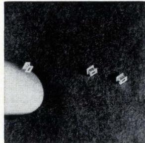
Custom-molded bobbins hold coils of fine wire for pots and similar devices. Typical dimensions are: length, 0.073±0.001 in.; flange outside diameter, 0.073±0.001 x 0.106±0.002 in.; core inside diameter, 0.062±0.001 x 0.031±0.001 in. Units offer low moisture absorption and high insulating capacity. Thermotech Industries Inc., 3328 Gorham Ave., St. Louis Park, Minn. [346]
