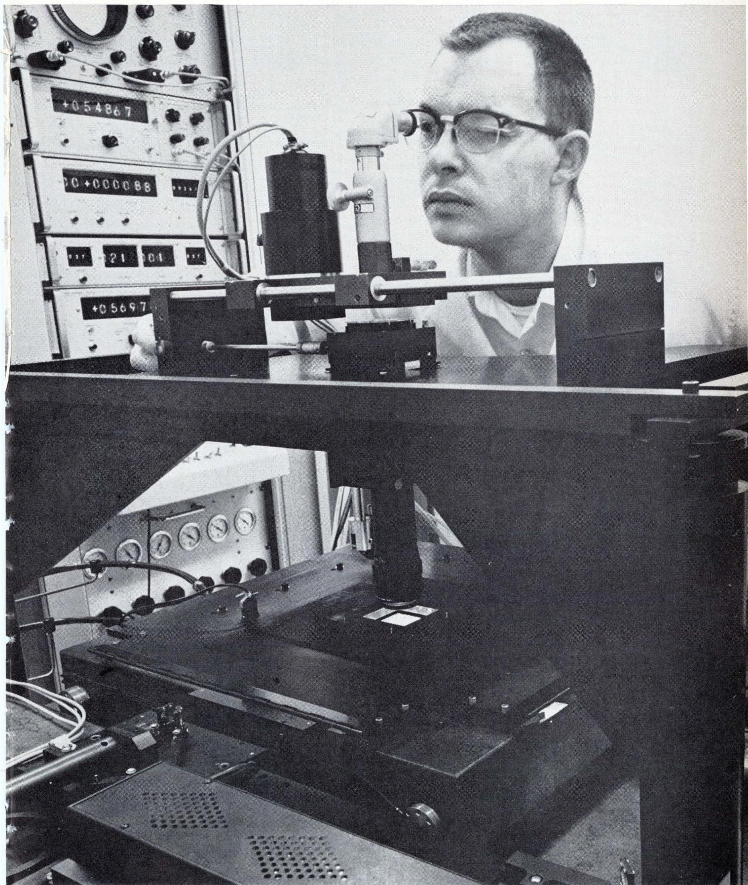
**Focusing.** D. M. Cross focuses the mask master onto the plane of the photographic plate before the xenon flash lamp, to the left of the focusing microscope, is moved into position. Helium-neon laser is in the foreground.
