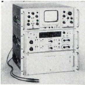
Type S-3100 time measurement system features digital programming, measurement speeds greater than 100/sec, and programable vertical and horizontal sampling units. It consists of a type 568 oscilloscope, type 230 digital unit, an auxiliary unit, and programable time-base and vertical units with a 50-ohm or 100-kilohm, 2-pf input. Tektronix Inc., Box 500, Beaverton, Ore. 97005. [389]
