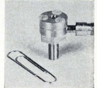
A miniature microwave generator consists of a silicon avalanching diode mounted in a radial mode cavity. The source is tunable over 3% bandwidth in the 5- to 9-Ghz frequency range and can deliver up to 100 mw continuous microwave power. The unit weighs less than  $\frac{1}{2}$  oz and has a volume of 0.06 cu. in. Sperry Microwave Electronics Co., Box 1828, Clearwater, Fla. [408]
