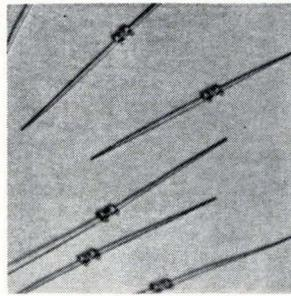
High-isolation switching diodes come in 2 types. MO-2825 is a fast-switching type with a test frequency of 8 GHz; insertion loss at 10 ma of 0.85 db max; and isolation at  $-10$  v of 15 db minimum. MO-1126 is a p-i-n switching diode with 8-GHz test frequency and insertion loss at 50 ma, 0.50 db max. Alpha Industries Inc., 381 Elliot St., Newton Upper Falls, Mass. [438]
