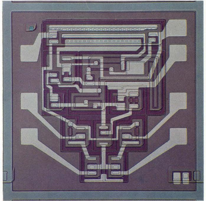
**Stable IC.** Self-tracking preamplifier mitigates performance variations caused by temperature change. An offshoot of an earlier linear amplifier, this Fairchild  $\mu$ A726 contains a two-stage feedback amplifier which senses chip temperature and regulates current supply accordingly.
