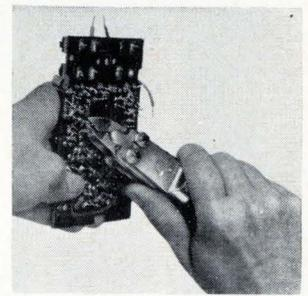
Air-operated pliers model CP-42 can cut cleanly and quickly through soldered, 0.062-in.-diameter copper wire. An adjustable jaw design prolongs jaw life, reduces down-time, and adapts jaw opening for the type of material being cut. The feather-touch throttle permits thousands of cuts with minimum effort. Chicago Pneumatic Tool Co., 6 E. 44th St., New York 10017. [424]
