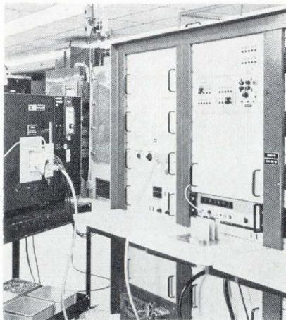
A-to-d interfacers tie the unit to computerized test system.
