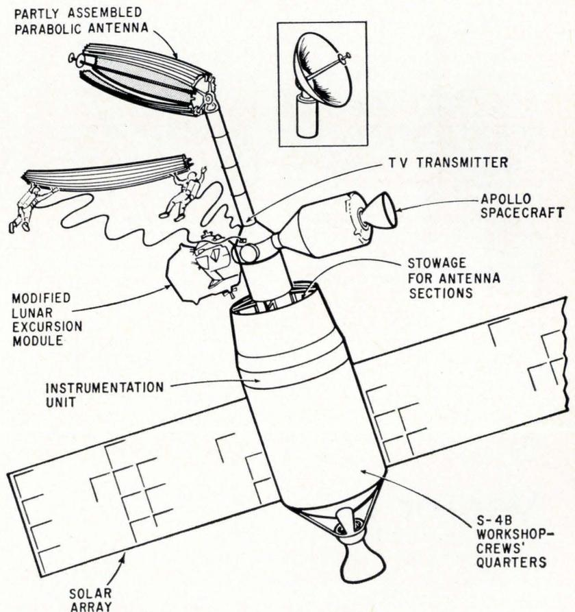
**Way out.** Orbiting tv station, envisioned by the Radio Corp. of America, would include paraboloid antenna dish that would be assembled in space.
