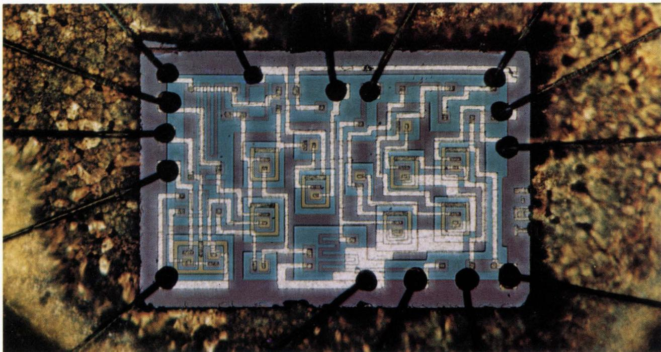
**Radio chip.** Complex IC providing five signal-processing functions is used in commercial radio-receivers. Chip amplifies audio and i-f signals, provides agc, detects envelopes, and has temperature-stabilizing network. Sony engineers developed the unit rather than use three or four commercial IC's with one or two functions each.
