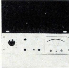
Accept-reject indication for production testing is featured in the model 503CC milliohmmeter. The unit offers sensitivity of 10 micro-ohms; 13 ranges from 1 milliohm to 10 kilohms; 1% of full-scale accuracy; 0.25% repeatability; and less than  $10\mu\text{w}$  dissipation in sample. The instrument measures  $5\frac{1}{2} \times 17\frac{1}{2} \times 13\frac{1}{2}$  in. Keithley Instruments Inc., 28775 Aurora Rd., Cleveland 44139. [371]
