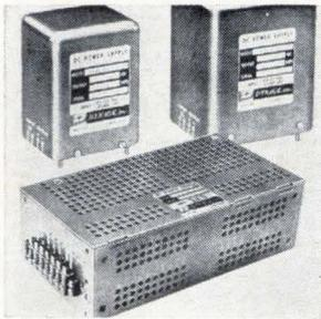
Dual modular and rack power supplies are for use with operational amplifiers. The K and KH series feature slave tracking to  $\pm 0.005\%/^{\circ}\text{C}$ , regulation to  $\pm 0.05\%$ , and a temperature coefficient to  $\pm 0.015\%$ . They are available at  $\pm 10\text{ v}$ ,  $\pm 12\text{ v}$ , and  $\pm 15\text{ v d-c}$  with current outputs from 150 ma to 2 amps per output. Dynage Inc., 390 Capitol Ave., Hartford, Conn. [381]
