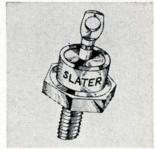
Four series of silicon power rectifiers are for use in power supplies, converters, and motor controls. The controlled-avalanche process eliminates matching while insuring reliability and conformance to MIL specs. Maximum current ratings are from 18 through 60 amps; max prv, 50 through 1,000 v. Prices start at \$1.09. Slater Electric Inc., 45 Sea Cliff Ave., Glen Cove, N.Y. [439]
