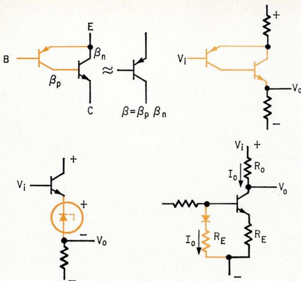
**Level shifters.** Three techniques for shifting d-c levels in IC's are the lateral pnp-npn composite (top), the zener-diode (lower left), and the resistor-constant-current source (lower right).
