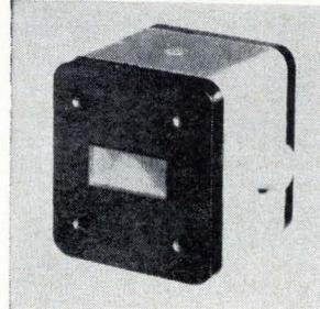
Navigation systems and airborne radar are among the applications for a compact, 21-oz beacon magnetron. The MA-250 operates at a fixed frequency in the 8.5 to 9.6 Ghz range with a 0.5  $\mu$ sec pulse width and a 0.005 duty ratio. Minimum peak power output is 7 kw. Input connections are made through flexible leads or solder lugs. Microwave Associates Inc., Burlington, Mass. [407]
