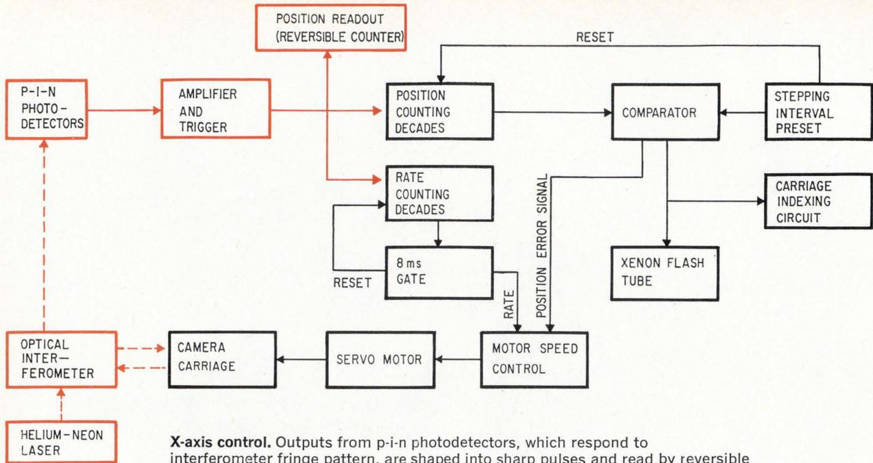
**X-axis control.** Outputs from p-i-n photodetectors, which respond to interferometer fringe pattern, are shaped into sharp pulses and read by reversible counter (color). Position and rate-counting decades are used for smooth control in d-c motor servoloop.
