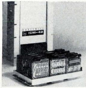
Core memory ICM-42 is for use in communications, telemetry, code conversion, machine tool control and digital buffer applications. Full cycle time is 1.5  $\mu$ sec and access time is 700 nsec. The IC-designed, self-contained system is available in capacities of 2,048 words and 1,024 words of 12 bits per word. Computer Control Division, Honeywell Inc., Framingham, Mass. [390]
