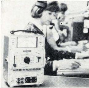
Telephone transmission/noise measuring set model 3555A will bridge or terminate lines of any standard impedances. It will measure frequencies from 30 hz to 3 Mhz. Included in the unit are C-message 3 khz flat and program weighting filters. The instrument can measure to 0 db random noise at 1 khz. Price is \$525. Hewlett-Packard Co., 1501 Page Mill Rd., Palo Alto, Calif. [361]
