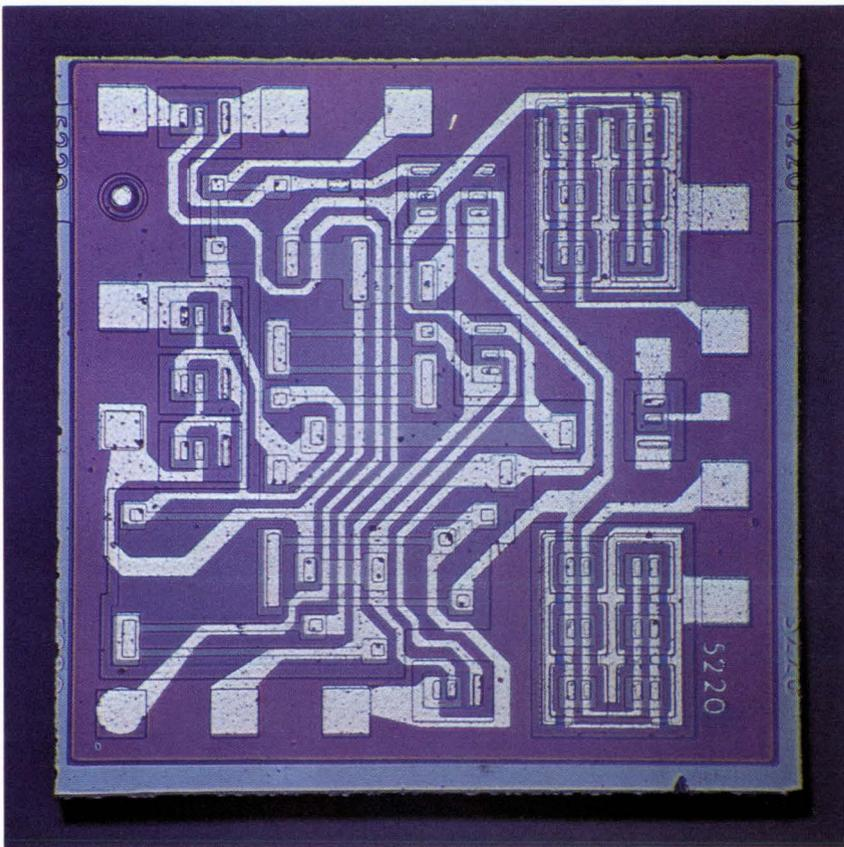
**Universal IC.** Wideband multistage circuit, RCA's CA3020, is outgrowth of simple audio-frequency differential amplifier. Modified chip contains additional stages and elements, and is configured for general-purpose applications. Unit may be used for communications, control, cable-driving, and even as a quasi-operational amplifier.
