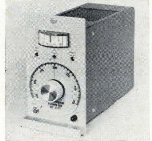
Temperatures can be held within  $0.5^\circ\text{F}$  with a solid state process controller. The unit compares the controlled temperature with the set point, automatically modulating electric heating elements to maintain desired heat. It gives virtually straight-line control. The instrument's platinum resistance bulbs operate to  $1,400^\circ\text{F}$ . Honeywell Inc., 2727 S. Fourth Ave., Minneapolis 55408. [364]
