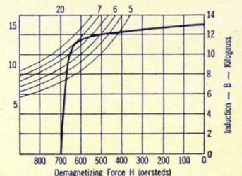
Demagnetization vs. energy output
