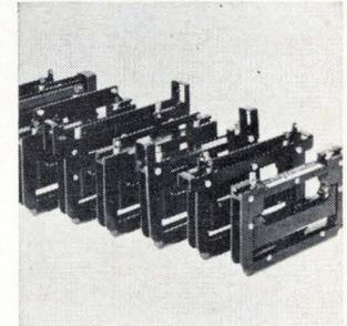
An extractor-inserter for printed circuit cards, model 30 is a pin-type tool featuring positive retention of the extracted card. It has a maximum extraction force rating of 100 lbs. Pick-up pins engage index holes in the circuit card and the card is extracted or inserted as the spring-loaded trigger is actuated. Flotron Industries Inc., 1201 E. Grand Ave., El Segundo, Calif. 90245. [356]
