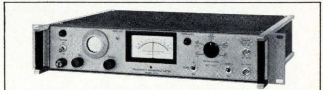
Tracor's Model 527A frequency-difference meter allows adjustment of two oscillators to the same frequency, adjustment to a specific offset, determination of offset—all instantly—plus both short-term and long-term stability analysis. No additional equipment is needed.
