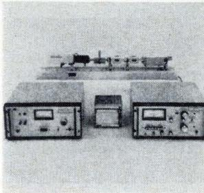
A microwave noise temperature calibrator checks sources utilizing gas-discharge noise lamps. It includes an i-f switched radiometer that compares the output of an unknown noise source to that of a reference standard noise source. Difference is read directly in db from a front panel dial. The standard has  $\pm 500^\circ$ K accuracy. Airborne Instruments Laboratory, Deer Park, N.Y. 11729. [405]
