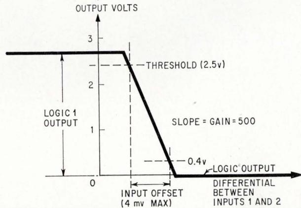
**Output.** Comparator's output characteristic has a maximum offset voltage of 4 millivolts. When the difference between the comparator inputs exceeds this value, the output switches from 1 to 0.
