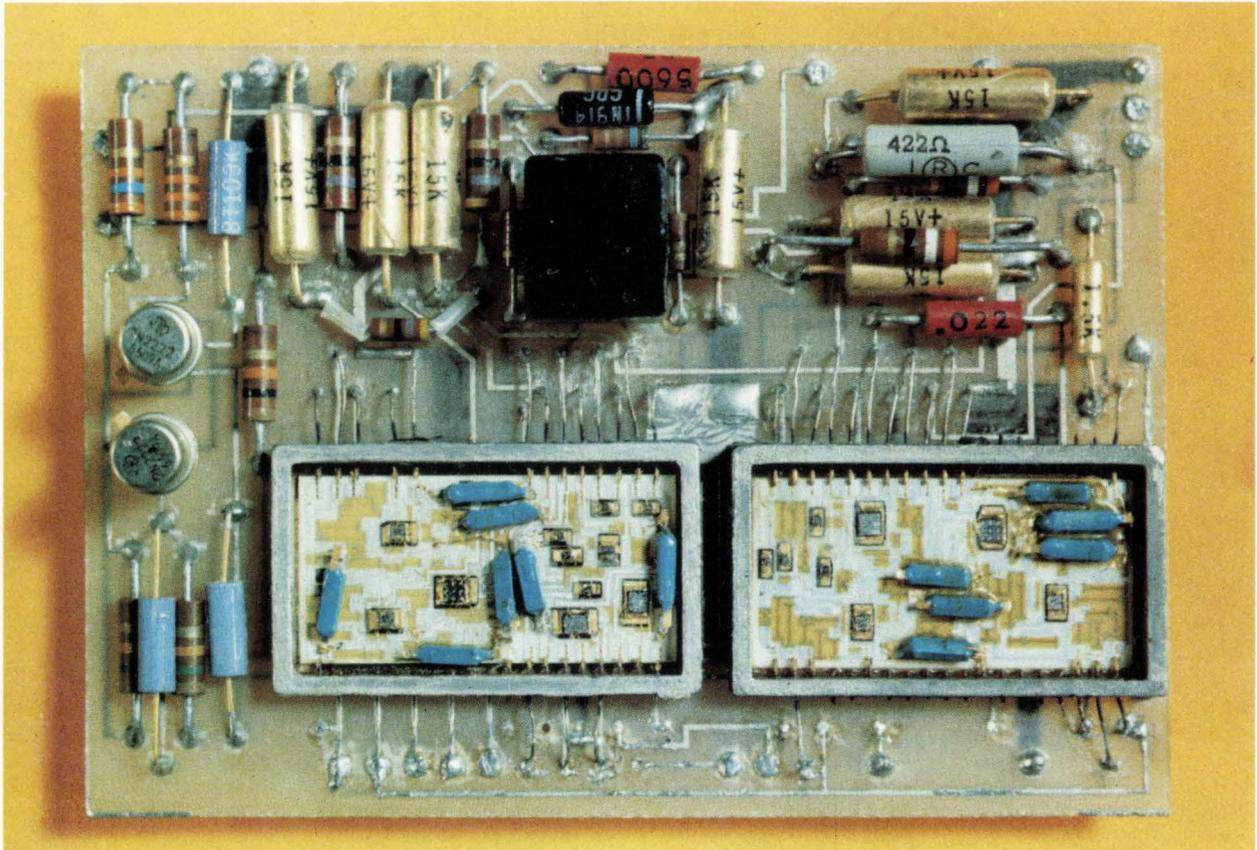
**Super card.** Video-processing subsystem, a radar range gate filter, contains two complex IC's having about 150 elements each. The 40-lead flatpacks, developed by GE Aerospace engineers, contain both monolithic and thin-film elements. The range gate filter consists of input, clutter rejection, amplifier, detector, integrator, and output circuits in a space less than one-sixth that of previous discrete semiconductor cards.
