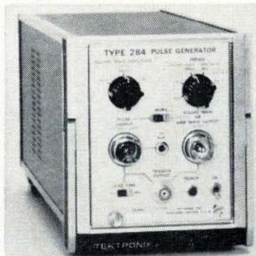
Pulse generator type 284 produces a pulse output with a rise time of less than 50 picosec and also provides the signals necessary to verify the performance of sampling oscilloscopes. Pulse output has an amplitude of approximately 200  $\mu\text{v}$  into 50 ohms. Repetition rate of the 284 is 50 khz, with a pulse duration of 1  $\mu\text{sec}$  and a flatness of  $\pm 3\%$ . Tektronix Inc., Box 500, Beaverton, Ore. [366]
