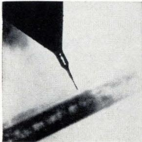
A building-block tooling system is suited for drilling IC's and printed circuits. Metal removal is a mechanical function; however, the system features optional automatic electronic and fluidic controls. Holes less than 0.001-in. diameter can be drilled on a production basis and simultaneous drilling of many holes per sq in. is possible. National Jet Co., 10 Cupler Drive, Cumberland, Md. [425]
