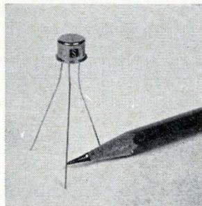
Silicon chopper transistors in TO-5 cases have voltage capabilities from 100 to 160 v. The pnp devices, series SSS1001-14, offer high reliability and 2-v saturation voltage, and can be bought in matched pairs. Applications include modulators and servos, and telemetry and multiplexing circuits. Solitron Devices Inc., 1177 Blue Heron Blvd., Riviera Beach, Fla. [442]
