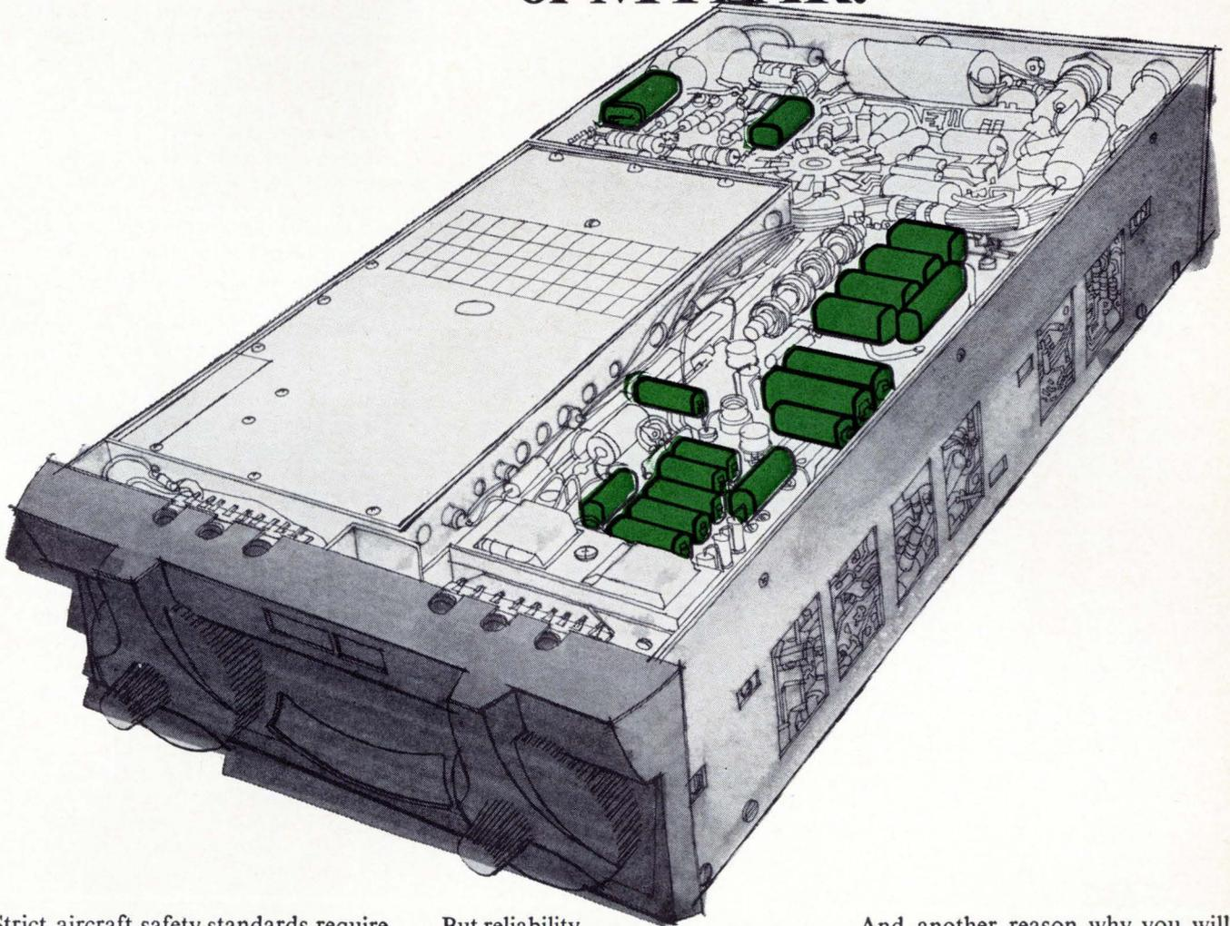
Strict aircraft safety standards require the most reliable navigation equipment available. That's why King Radio Corporation uses capacitors of MYLAR\* for their Distance Measuring Equipment. MYLAR can take temperature extremes from  $-60^{\circ}$  to  $+150^{\circ}\text{C}$ ; MYLAR remains constantly stable under humid conditions.
