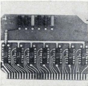
IC logic modules, designated the 14 series, feature dual in-line chips, economy and flexibility. Simplified board layouts permit mixing of chip types on a single board. The DTL integrated circuits work from a 5-v power supply at 5-Mhz operating speeds. Noise rejection is typically 1 volt. Canoga Electronics Corp., 20131 Sunburst St., Chatsworth, Calif. 91311. [393]
