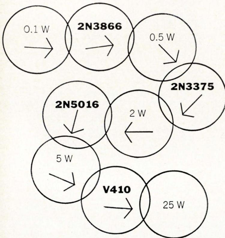
You can get 25 watts (typical) at 400 MHz from a high-gain amplifier using the four silicon transistors shown above. And, conservative per-stage power gain allows you greater design bandwidths and higher temperature operation.
