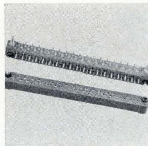
Right-angle pin and socket connectors are used where a soldered joint between connector and p-c board is required. MIG series connectors are available with 11, 15, 23, or 37 contacts, with a contact grid spacing of 0.1 in. They are furnished with standard solder cup terminations as well as in dip-solder contact versions. U.S. Components Inc., 1320 Zerega Ave., Bronx, N.Y. [347]
