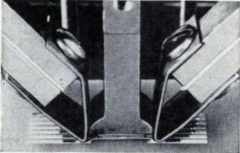
Our equipment reflow solders D.I.L.'s, flatpacks, multiple lead components — up to 40 leads at a time — without damaging the p. c. board! What's your problem?
