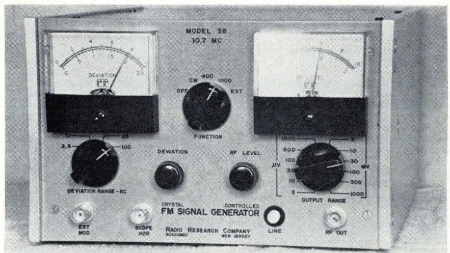
Fixed frequency. Single channel generator varies voltage continuously.
