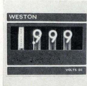
All-electronic digital panel meter 1270 is a 3-digit Nixie tube device suitable for various current and voltage measurements. A dual slope integrating technique assures an accuracy of  $0.1\% \pm 1$  digit and a stability of 0.05%. Common-mode rejection is 100 db; resolution, 1 part in  $10^3$ . Price is \$312 each. Weston Instruments Inc., 614 Frelinghuysen Ave., Newark, N.J. [363]
