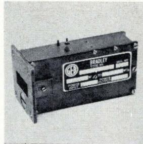
Klystrons can be replaced by an X-band, step recovery local oscillator. Simply connect a 17.5-v to 28-v supply and produce 10-mw output for 1 $\frac{3}{4}$ -w input. Bandwidth is 400 Mhz tunable with  $\pm 10$  v d-c. Noise is in the same order as a klystron. Operating range is  $+80^\circ$  to  $-40^\circ$ C. Price is \$650. Edwin Industries Corp., 5858 E. Molloy Rd., Syracuse, N.Y. [403]
