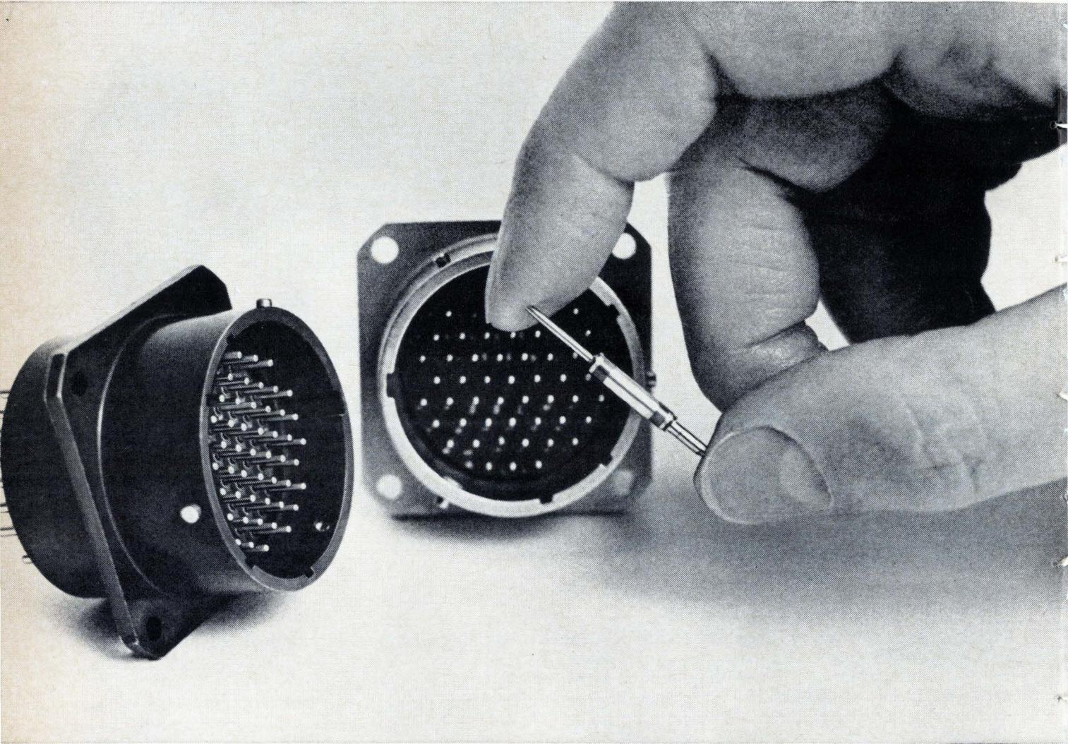
Bendix® filter-connectors can eliminate EMI (electro magnetic interference) better than conventional filtering methods ever could. The filtering action is completely built-in because we've surrounded each individual pin with a miniature ferrite filter.
