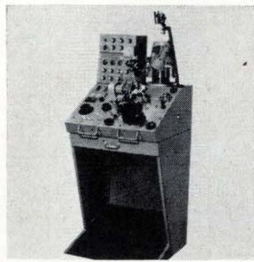
Toroidal coil winder T0-125C accommodates interchangeable shuttle heads and core holding and rotating fixtures, permitting fast changes in set-up. It produces finished coils from 0.028 in. i-d to over 5 in. o-d in wires from No. 16 to 50 Awg. It has variable winding speed controls and a 2-knob core positioning system. Leeson Corp., 131 West St., Danbury, Conn. [422]
