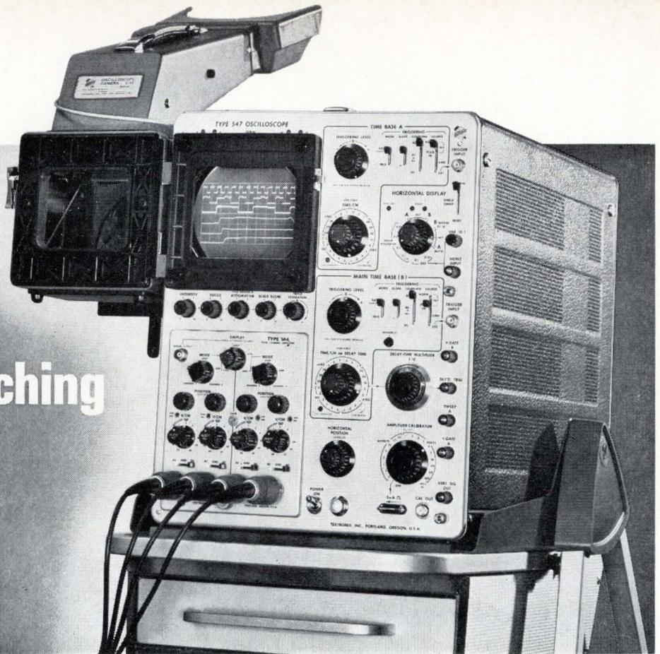
The Tektronix Type 547 is a 50-MHz, 7-ns sweep-switching oscilloscope that offers dual-beam measurement capabilities with most repetitive signals. A complete selection of plug-ins permits you to change your oscilloscope performance to meet your changing needs.
