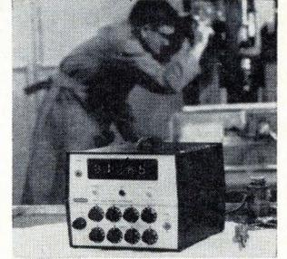
A new line of electronic counters and controllers is for nuclear counting, machine-tool control, position indication, and process or manufacturing tabulation. The 6200 series includes 7 instruments. Each has a 4-digit, in-line display, with provisions for an optional 5th digit. Prices range from \$495 to \$925. Beckman Instruments Inc., 2500 Harbor Blvd., Fullerton, Calif. [376]
