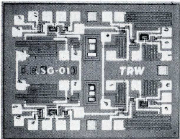
**Compatible.** Combination of monolithic active elements and thin-film resistors on a common substrate forms compatible IC's. This unit, developed by TRW Systems, is a precision multichannel level shift gate comparable to a dual three-input NAND gate.
