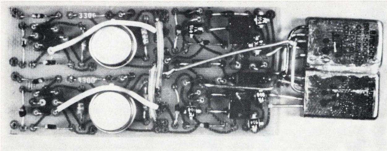
**Prototype.** Assembled two-channel control unit incorporates IC preamplifiers and miniature relays.
