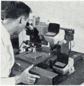
The 6X6M coordinate measuring machine has a 6-in. travel in both X and Y axes. It offers fast, reliable inspection of complex components used in IC's and related assemblies. Base and ways are made of Escondido black granite for stability and the desirable mass. Both coordinate movements are floated on air bearings. DoAll Co., 254 N. Laurel Ave., Des Plaines, Ill. [421]
