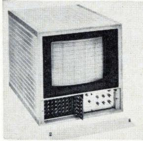
A profile monitor oscilloscope, with 10-mv full-scale deflection, displays up to 100 channels of information. The PM703 is designed for real-time transducer output displays of temperature, pressure, or other phenomena. Among its applications are the chemical and textile process control fields. Industrial Products Division, ITT Corp., 15191 Bledsoe St., San Fernando, Calif. [375]
