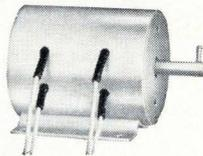
**Packaged Control Solutions** Here we put our dish-shaped solenoid to work as a driver for a miniaturized (4 $\frac{3}{16}$  x 1 $\frac{1}{32}$  x 1 $\frac{1}{32}$ ) 12-position stepping switch. Model shown is an armament control (intervalometer). It is used to fire 19 rockets in pairs sequentially, at 10 ms intervals. We can tailor one like it for your stepping or sequentially timed switch application.
