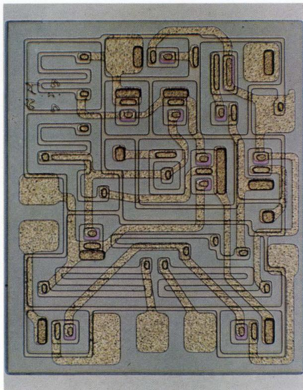
**Power play.** IC for driving-power devices such as thyristors, transistors, and relays, is capable of a-c line operation. The GE unit, type PA424, detects voltage, unbalances and generates timed, trigger-pulse outputs.
