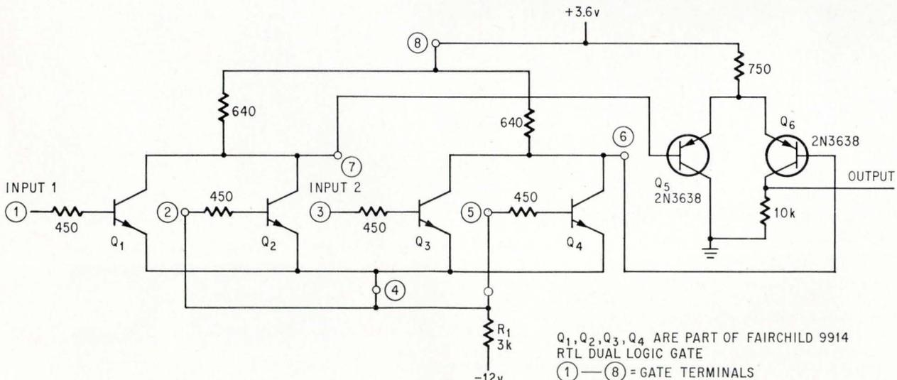
**Comparator.** Inputs applied to terminals 1 and 3 are compared and amplified, producing a logical 1 or 0 at the output.
