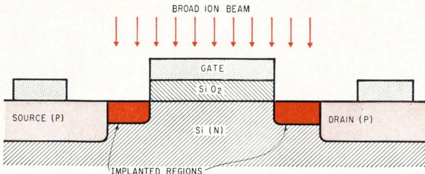
**Implanted FET.** The source and drain regions of this Hughes device were diffused and ions implanted to bring both just up to the edge of the gate. This technique avoids the necessity of diffusing under the gate lead and reduces feedback capacitance by 40 times.
