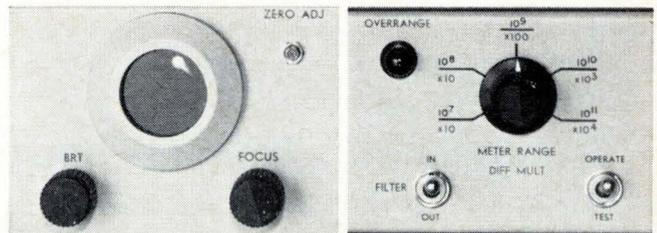
A rotating dot on the front-panel oscilloscope indicates phase relationship between compared frequencies with fractional frequency difference multiplied by 10, 100, 1000, or 10,000 as selected by the range switch.
