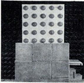
Spherical passive devices called Ecco reflectors increase radar cross section and also produce scintillation patterns useful for simulating natural targets and for identification purposes as radar beacons. Parameters are the number of reflectors, distance between them, radar frequency, and each reflector's radar cross section. Emerson & Cuming Inc., Canton, Mass. [401]
