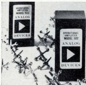
Varactor bridge operational amplifiers 302 and 303 are for inverting and noninverting circuitry, respectively. They have  $\frac{1}{2}$  picoamp max bias current and 0.05 picoamp/ $^{\circ}$ C max current drift at  $25^{\circ}$ C. Peak-to-peak noise from d-c to 1 Hz is 0.01 picoamp and 2  $\mu$ v. Differential input impedance is  $5 \times 10$  ohms. Analog Devices Inc., 221 Fifth St., Cambridge, Mass. [394]
