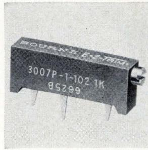
Model 3007P is a wirewound adjustment pot for space-saving commercial uses. It is offered in resistances of 10 ohms to 20,000 ohms. Power rating is 1 w at 40°C, and operating temperature range is -55° to +125°C. Temperature coefficient is 100 ppm/°C maximum. Price is 99 cents each in 1,000-piece quantities. Bourns Inc., 1200 Columbia Ave., Riverside, Calif. [343]
