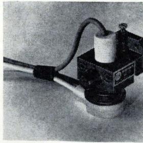
Reflex klystron oscillators covering 26.5 to 35 Ghz serve as pump tubes in parametric amplifiers. Tuning over a 1,000-Mhz range, the VA-312 delivers 150 mw at a beam voltage of 550 v. The VA-313 has a mechanical tuning range of 700 Mhz and delivers a minimum of 500 mw at 26 Ghz. The tubes weigh 4 oz. Varian Associates, 611 Hansen Way, Palo Alto, Calif. 94303. [402]
