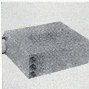
Hermetically sealed for aerospace use, the PM1570, a 3-channel d-c/d-c instrumentation power converter, has a temperature coefficient of 5 ppm/ $^{\circ}$ C without ovens. Output voltage regulation for power line excursions of 22 to 36 v d-c after load changes from  $\frac{1}{4}$  load to full load is  $\pm 0.1\%$  on all channels. Pioneer Magnetics Inc., 1745 Berkeley St., Santa Monica, Calif. [395]
