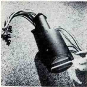
A high-resolution crt features a 4-in. long raised cylindrical faceplate of fiber optics and a yoke-shield assembly for aerial photography, single-line scan display, side-looking radar, and film recording. Type WX-30519 offers a maximum center spot size of 0.0007 in. and an edge spot size of 0.0008 in. Anode voltage is 10kv. Westinghouse Electric Corp., Elmira, N.Y. [341]
