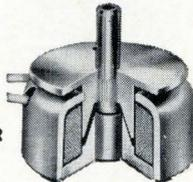
**Ledex Rotary Solenoids** Known best for their shock resistant ability, high torque-to-size rotary motion, and relatively flat output curve. 8 basic sizes, strokes from 20° to 95°, torque to 117 pound-inches.
