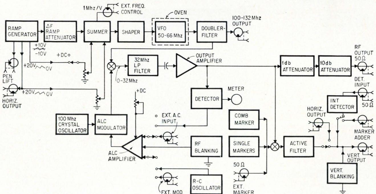
**ALC loop.** Output of VFO is doubled and mixed with 100-MHz crystal-controlled signal. Oscillator injection amplitude is controlled by ALC voltage derived from generator output. Ramp-generating and summing circuits produce signal sweep.
