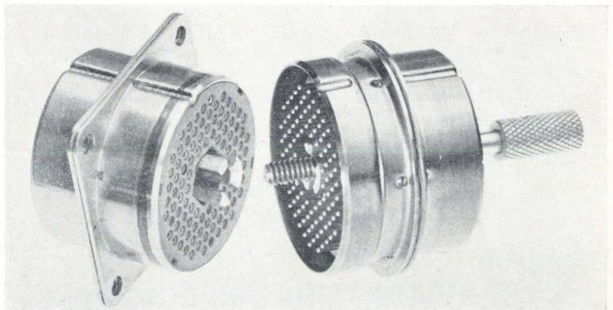
**Bayonet gone.** Center jack screw replaces conventional bayonet whose locking mechanism takes a lot of room. As a result, more connectors can be squeezed onto a panel.
