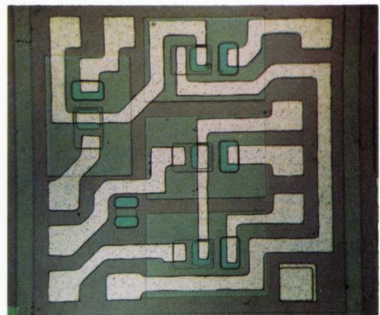
**Active pattern.** Monolithic dual common-emitter pairs provide the active functions in hybrids. Access to each of the four transistor elements gives users the option of any or all devices and bypassing of substandard units.
