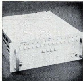
DADIT is a 15-bit integrating a-d converter with common-mode rejection of 10 million-to-1 at d-c to line frequency. It is for monitoring such low-level transducers as strain gauges in high-level a-c environments, and also works well with multiplexers. No preamplification or individual point filtering is needed. Control Data Corp., 4455 Eastgate Mall, La Jolla, Calif. [387]
