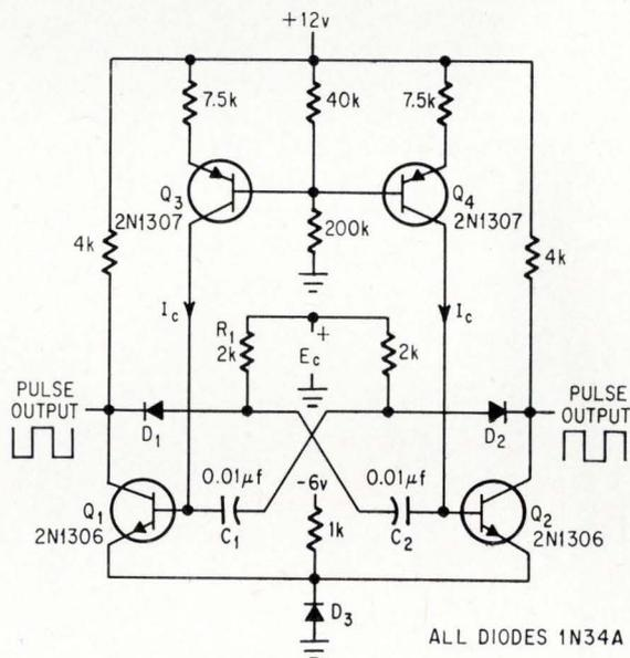
**Variable output.** Pulse width is proportional to the control voltage,  $E_c$ . Before  $Q_1$  or  $Q_2$  conducts, constant current,  $I_c$ , must charge capacitor  $C_1$  or  $C_2$  to  $E_c$ .
