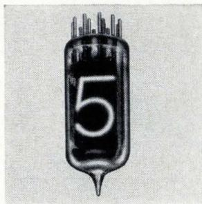
Numerical readout tube NL-874, with an inverted base, is mounted vertically with the base at the top to permit optimum use of panel spacing. It is a side-view display tube with 0.310-in. characters, 0 to 9. It requires a minimum d-c supply of 170 v at maximum cathode current of 3 ma average; minimum, 1.5 ma average. National Electronics Inc., Geneva, Ill. [342]
