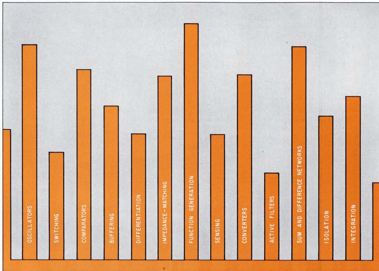
**Versatility.** More than a dozen major classes of applications are satisfied by operational amplifiers; users merely alter external feedback and coupling components for amplifying, switching, detecting, and other signal-processing needs.
