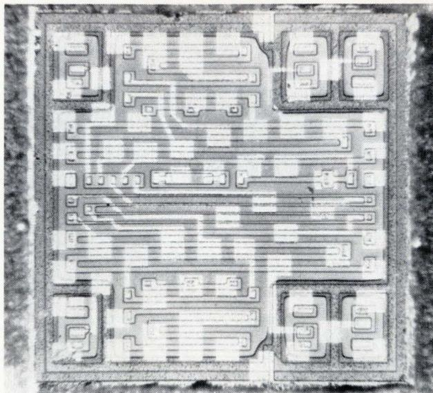
**Master circuit.** Universal IC breadboard performs various jobs—at user's discretion. Circuit interconnections are made to fit differing requirements; six transistor elements and 33 resistors on Norden's NM3025 chip may be connected to function as amplifiers, power-switch drivers, Schmitt triggers, even RTL digital logic gates.
