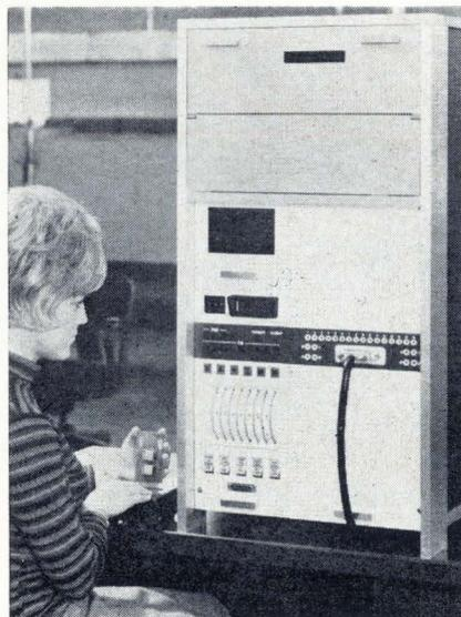
**D-c tester.** Model 668 administers d-c tests to integrated circuits, can also check out printed circuit cards.
