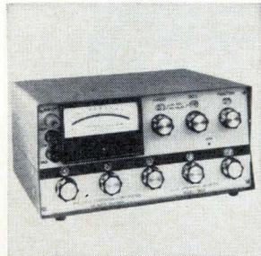
An a-c/d-c voltmeter has high accuracy and stability due to an integral proportional controlled oven for the zener reference. The 365A offers ranges of  $\pm 1,100$  v,  $\pm 110$  v,  $\pm 11$  v, 1,100 mv, and 110 mv. It has a 6-digit readout. High sensitivity and resolution are achieved through a  $110\text{-}\mu\text{v}$  full scale null detector. Precision Standards Corp., 911 Westminster Ave., Alhambra, Calif. [370]
