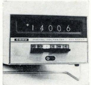
Integrating digital voltmeter series 540 has an accuracy of 0.01% of reading  $\pm 1$  digit in 4 ranges from 1.5000 to 1000.0 v d-c. It maintains accuracy specs for 6 months. Unit features 5-digit readout with overranging digit, polarity and decimal; manual and automatic range selection; constant 10-megohm input impedance. Cohu Electronics Inc., Box 623, San Diego, Calif. [368]
