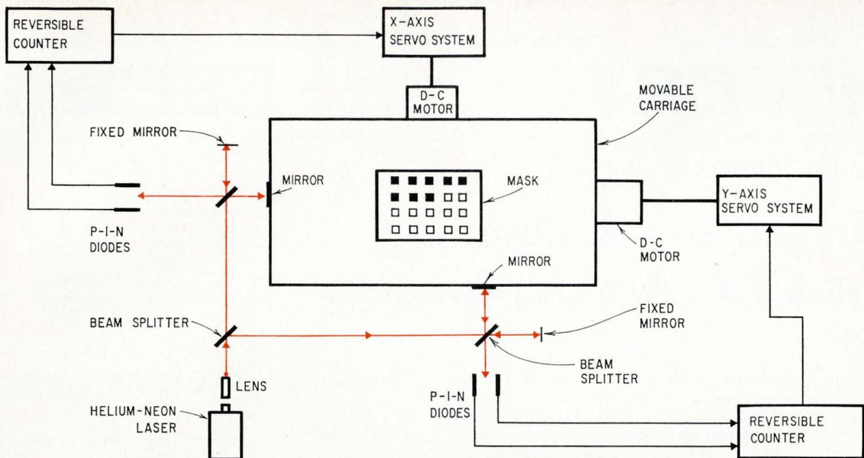
**Reflected light.** Interference fringes are created as the laser beam (color) is reflected from quartz mirrors. The absolute value of the carriage's position is displayed on two 2-megahertz reversible counters.
