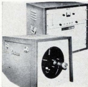
Large-screen television projector model 260 features a resolution of 1,000 lines and adjustable scan rates to as high as 1,203 lines at 60 fields per sec. The system uses a 6-in. crt and a high-powered video amplifier. The projection head measures 27 x 24 $\frac{3}{4}$  x 36 in., the control unit measures 19 $\frac{1}{4}$  x 21 x 20 in. Price is \$11,000. Amphicon Systems Inc., Oak St., Norwood, N.J. [382]
