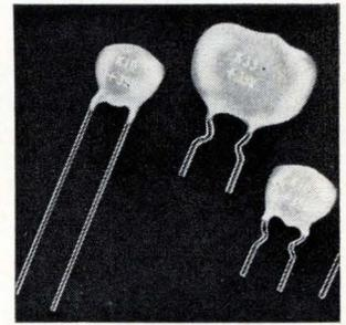
Polar, solid tantalum capacitors in the E series use a dip-coated, hard epoxy encapsulation process. They are suited for decoupling, bypass, filtering, and blocking circuit uses. Units are offered in working voltages of 6 (330  $\mu$ f max), 10, 15, 20, 25, 35, and 50 (15  $\mu$ f max.) v. Electronics Division, Union Carbide Corp., 30-20 Thomson Ave., Long Island City, N.Y. [352]
