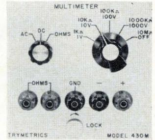
Plug-in module 430 M provides d-c, a-c, and ohms measurement capabilities for the company's 4000 and 4100 series digital voltmeters. It offers 4 d-c ranges from 0.9999 to 999.9 v d-c; 4 a-c ranges of the same voltages; and 5 ohms ranges from 999.9 ohms to 9.999 megohms. The function head costs \$295. Trymetrics Corp., 204 Babylon Turnpike, Roosevelt, N.Y. 11575. [372]
