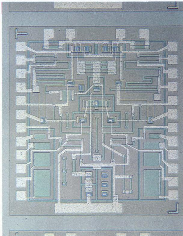
**Citizen-soldier.** Elaborate gain-control circuit can be used in both color-tv sets and radar i-f strips. Designed by Sprague Electric, variable electronic attenuator works directly with IC amplifiers to provide the agc function.
