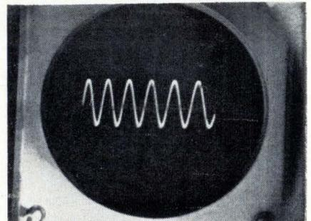
**Sine wave.** Undistorted sinusoidal waveforms have the accuracy of a tuning fork oscillator.
