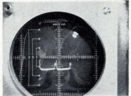
**Marker pulses.** Typical fast rise time pulses can be used as frequency markers or as synchronized oscillator triggers.
