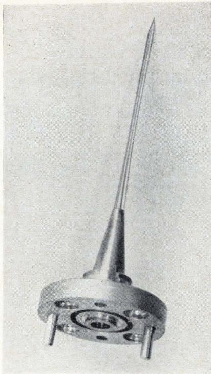
Tip of the line. Taper of plastic rod decides beam shape of polyrod antenna.
