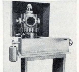
The 120 LEED (low-energy electron diffraction) system for crystal-surface studies is used primarily for obtaining data regarding atomic geometry. It permits direct study of corrosion, oxidation, epitaxial growth, and catalytic processes. Vacuum chamber pressures down to  $3 \times 10^{-8}$  torr are available. Varian Associates, 611 Hansen Way, Palo Alto, Calif. [396]
