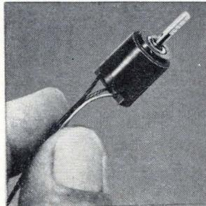
Potentiometer type CP40 was developed for use in precision servo units, or as a feedback device on miniature actuators where only very low torque outputs are available. Resistance values are from 5,000 to 20,000 ohms. Torque is approximately 3 gr-cm, or less if specified. The unit measures 0.5 x 0.68 in. Humphrey Inc., 2805 Canon St., San Diego, Calif. 92106. [353]
