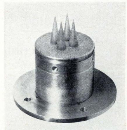
**Spiked.** Higher antenna efficiency and lower sidelobes resulted when TRG substituted spikelike polyrod antennas for horns in this 94-ghz scanning feed.
