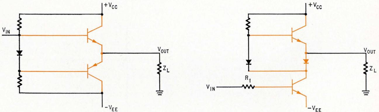
**Comparing techniques.** IC power circuit design differs from discrete semiconductor versions. Classic class B output stage (left) requires complementary npn and pnp transistors. IC makers use design tricks—such as diode-coupled npn cascodes (right) that avoid need for high-quality pnp's that are costly and difficult to fabricate.
