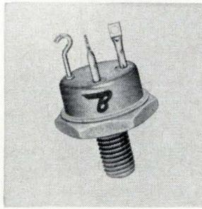
Radiation-resistant silicon power transistors feature a continuous collector current of 20 amps. They withstand exposure levels of  $5 \times 10^{14}$  NVT (total integrated neutron flux with energy levels greater than 10 KEV). Power dissipation is 50 w; collector-to-emitter voltage, 40 to 75 v; and gain bandwidth product, 200 Mhz at 28 v and 0.5 amp. Bendix Corp., Holmdel, N.J. [437]
