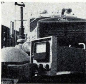
Smoke meter model 912 measures the amount of smoke emitted by diesel trucks. A movable arm positions the sensor above exhaust stacks. Physical connection to the truck is not required. Readout is in both Ringelmann units, the standard smoke-shade unit of measurement, and in % absorbance. Accuracy is  $\pm 2\%$ . Beckman Instruments Inc., 2500 Harbor Blvd., Fullerton, Calif. [369]
