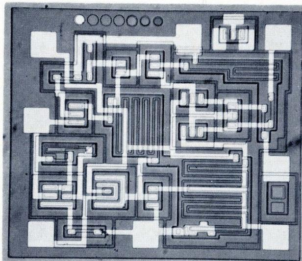
**Kingpin.** The most popular linear IC is the 709, a premium operational amplifier invented by Fairchild Semiconductor. Containing 14 transistors and 14 resistors, it has a gain of 45,000, an output swing of 14 volts, and accepts input signals as large as 10 volts. More 709's have been designed into linear systems than any other linear IC product—one reason why at least 12 IC makers manufacture it. This is Amelco's version.
