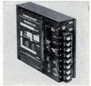
Temperature transmitters 18-111 and 18-112 receive signals from thermocouples and other millivolt sources and provide d-c voltage or current output signals. Accuracy of the output signal is to  $\pm 0.1\%$  with linearity of  $\pm 0.05\%$  of a straight line connecting actual end points, suiting the output for computation or control. Bell & Howell Co., 706 Bostwick Ave., Bridgeport, Conn. [384]
