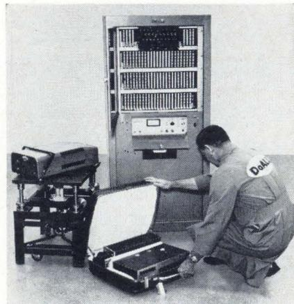
Portable. The bulk is taken out of new laser interferometer.
