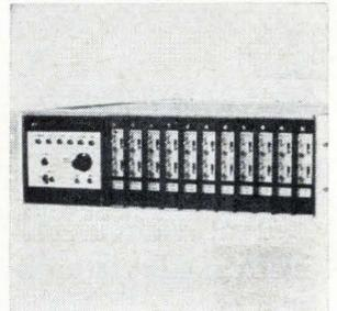
Calibration system model 8812 is designed for subcarrier discriminators. It generates all 21 constant-bandwidth channel frequencies and a reference frequency simultaneously and applies the resulting frequency-multiplex group to the discriminator system. Deviation bandwidths for each channel can be set at  $\pm 2$ ,  $\pm 4$ , or  $\pm 8\text{ khz}$ . Vidar Corp., 77 Ortega Ave., Mountain View, Calif. [388]
