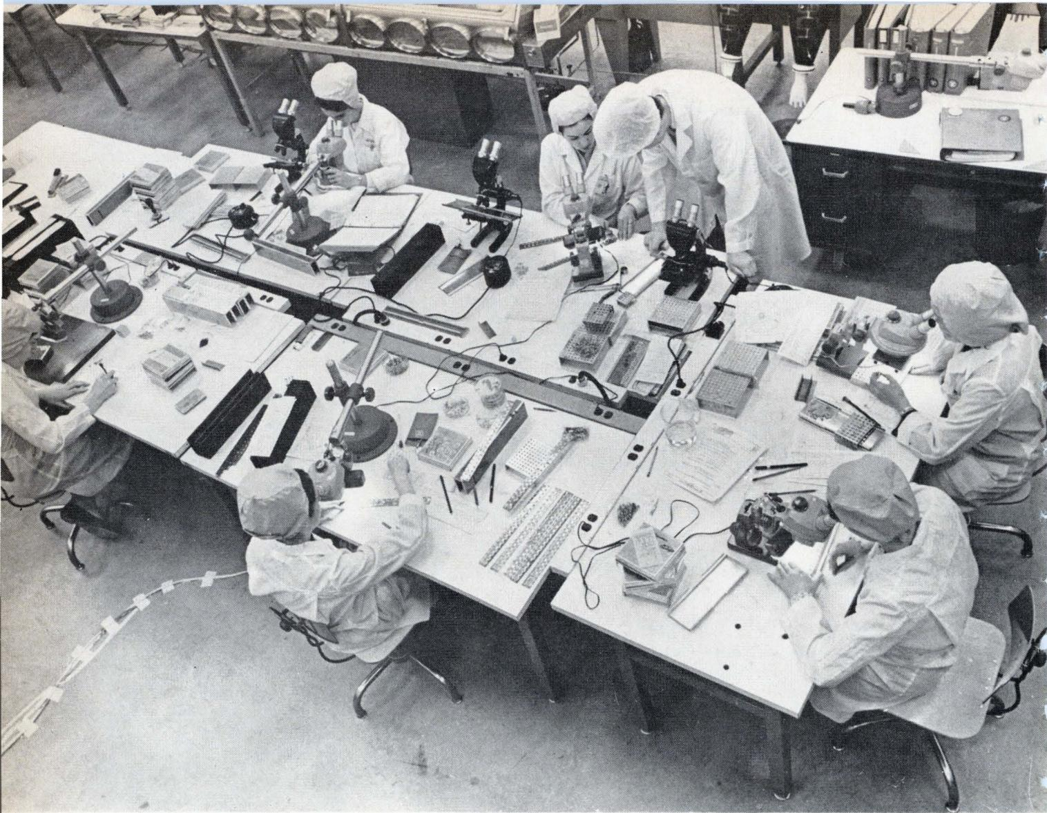
**Line up.** Inspection workers examine linear integrated circuits prior to sealing and shipment at Westinghouse's Molecular Electronics plant.
