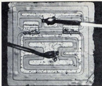
**High gain.** Two npn transistors are connected in a Darlington amplifier to increase the gain of the detector. Both are made by planar technology.
