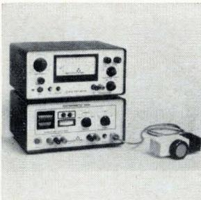
An integrating photometer digitally totalizes light energy for periods ranging from 0.1 sec to many weeks. The IL600/620 has synchronized and predetermined outputs for delivering preset dosages. It can totalize energy at any wavelength from 200 to 1,200 millimicrons. Price ranges from \$1,490 to \$2,100. International Light Inc., 12 Unicorn St., Newburyport, Mass. [365]
