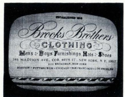
Clear image. Quality of picture after it has passed through the two converters is still good enough so that printing can be easily read. One big application could be in banks where the system would verify signatures and speed check cashing.
