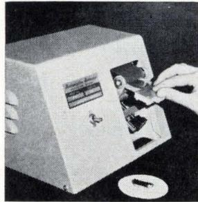
Model 1180A is an automatic belt-type fracturer for semiconductor wafers that works equally well on thick-film scribed substrates. In the wafer-fracturing process the wafers are batch spray coated on the reverse side with a quick, air-drying emulsion that holds the die together after fracturing. Price is \$390. Mechanization Associates, Mountain View, Calif. [426]
