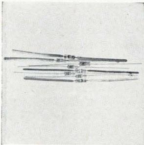
Point-contact diodes called Pico-Min are designed as broadband mixers and detectors for series mounting in stripline and coax circuits. They are housed in a microminiature glass case with axial wire or ribbon leads. Typical is the MA-4811D S-band mixer type with a maximum noise figure of 5.5 db at a test frequency of 3,060 Mhz. Microwave Associates Inc., Burlington, Mass. [440]
