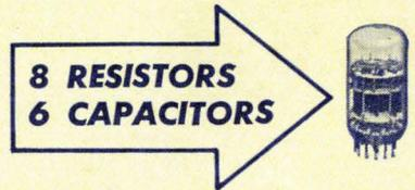
Takes passive elements off the circuit board and puts them inside the compactron
