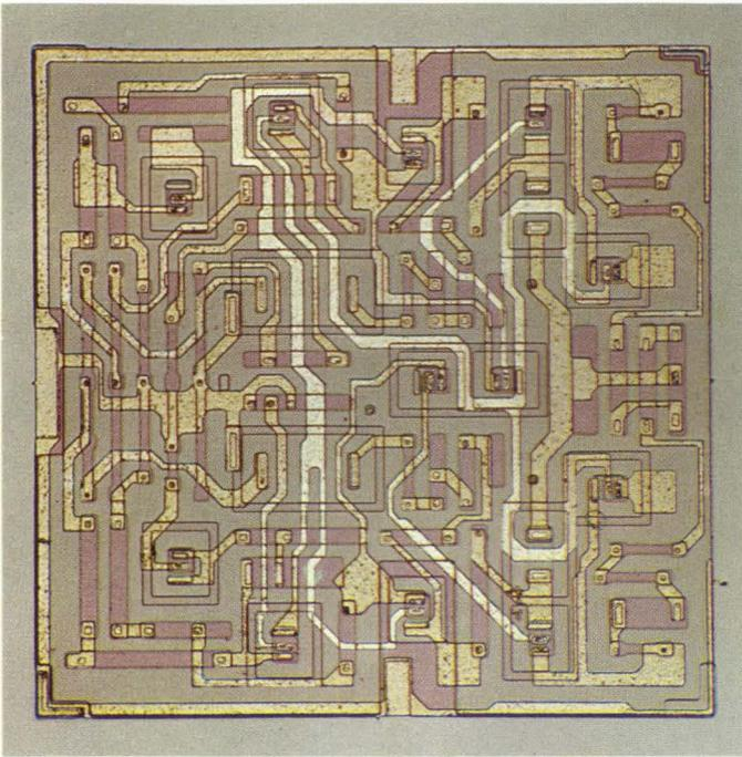
**Wide screen.** High-gain video amplifier from TI is improved version of earlier wideband differential amplifier. The SN5511's stages have a three-octave spread in frequency breakpoints; additional elements on chip help maintain 30 db of gain over a 35-Mhz bandwidth.
