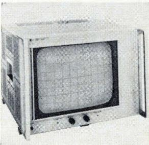
Crt monitor model 1300A has an 8 x 10-in. display area. It offers 20-Mhz on horizontal, vertical, and intensity axes, and the crt writing rate is faster than 20 in./ $\mu\text{sec}$ . Deflection linearity is better than 1% full screen for accurate presentation of high-frequency x-y plots. The unit requires 175 w. Price is \$1,900. Hewlett-Packard Co., 1501 Page Mill Rd., Palo Alto, Calif. [373]
