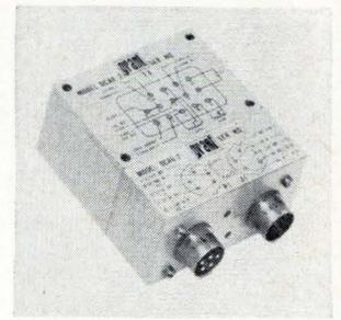
Airborne d-c instrumentation amplifier DCA8-2 offers flexible design, permitting a variety of sensor inputs. It contains an isolated, regulated 5-v transducer excitation supply. The unit withstands high shock. Output operates into a load of 10,000 ohms or greater without degradation. Operating temperature is  $-65^{\circ}$  to  $+185^{\circ}$ F. Grant Electronics, 2017 Glendon Ave., Los Angeles. [392]
