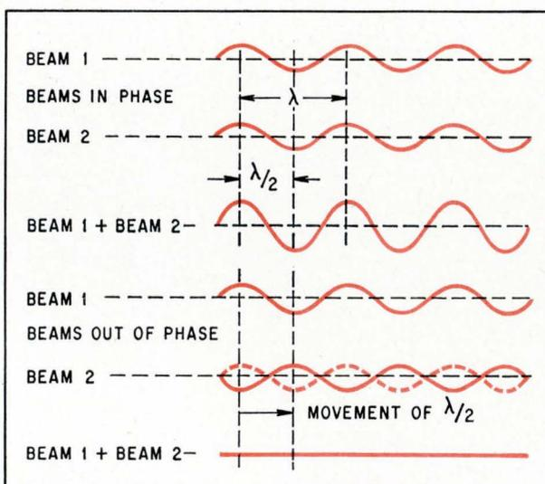
**Interference.** In-phase beams produce constructive interference or a bright line at the detector of the interferometer. Out-of-phase beams interfere destructively so there is no light at all when phases are a half wavelength apart.
