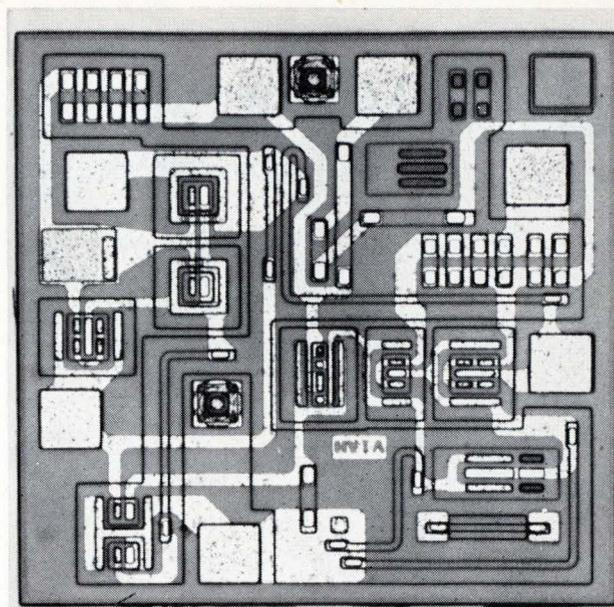
**High-gain amplifiers.** Extensive internal feedback staging in newer wideband amplifiers results in higher and higher open-loop gain-bandwidth products. Philco-Ford's PA7600 (left) has 9-Ghz product; Motorola's MC1553 (right) has a 7-Ghz gain-bandwidth product. Under closed-loop operation the 7600 develops 28 db of gain over a 130-Mhz bandwidth; 1553 in closed-loop mode maintains 46 db of gain over 35-Mhz bandwidth.
