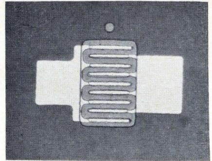
**Power pushed.** A power gain of 10 db is achieved at 2 Ghz by improved diffusion techniques in the L-186.
