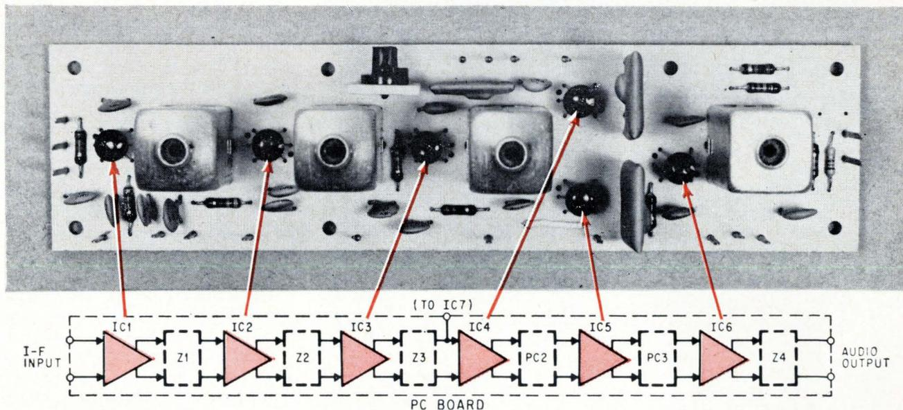
**Hi-fi IC's.** Fisher Radio will introduce a high-fidelity receiver this fall that uses seven integrated circuits: six in the intermediate-frequency and limiter stages and one in the meter and muting circuit. The receiver will sell for a little less than comparable high-fidelity receivers. Aside from cutting costs, the application of IC's produces better sound, Fisher maintains. Also, the IC's improve the receiver's capture ratio.
