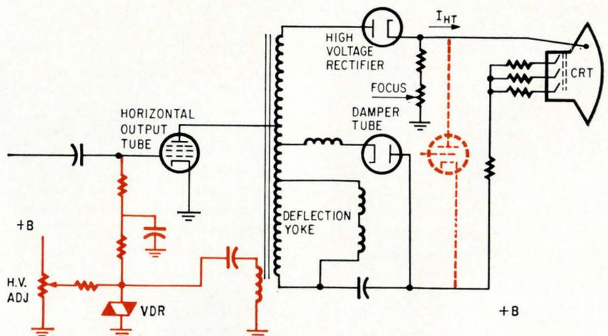
**Banished tube.** Negative feedback circuit in Matsushita color set does away with the shunt-regulator tube normally used to stabilize the high-voltage supply. For simplicity, the grid circuit that would be used with the shunt regulator tube (broken lines) is not shown.
