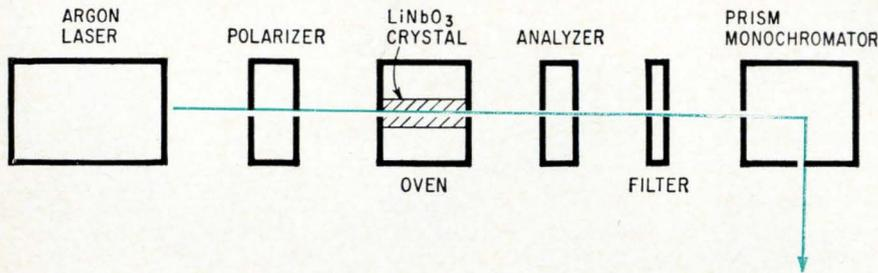
Temperature tuning. Laser goes from infrared to blue-green.
