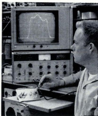
**Solid state.** Model 675A is both a sweeping and continuous-wave signal generator over a range of 10 khz to 32 Mhz. Completely solid state design incorporates an oven to stabilize the variable frequency oscillator. The display oscilloscope above the generator isn't part of the instrument as it comes from the manufacturer.
