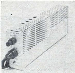
D-c amplifier 1-168 drives high-frequency, light beam galvanometers. The single plug-in module provides isolation between input and output and between circuitry and ground. Voltage gain ranges from 0.1 to 500. Frequency response is from  $\pm 1\%$  d-c to 5 khz. Overload recovery time is 100  $\mu\text{sec}$ . Consolidated Electrodynamics Corp., 460 Sierra Madre Villa, Pasadena, Calif. [386]
