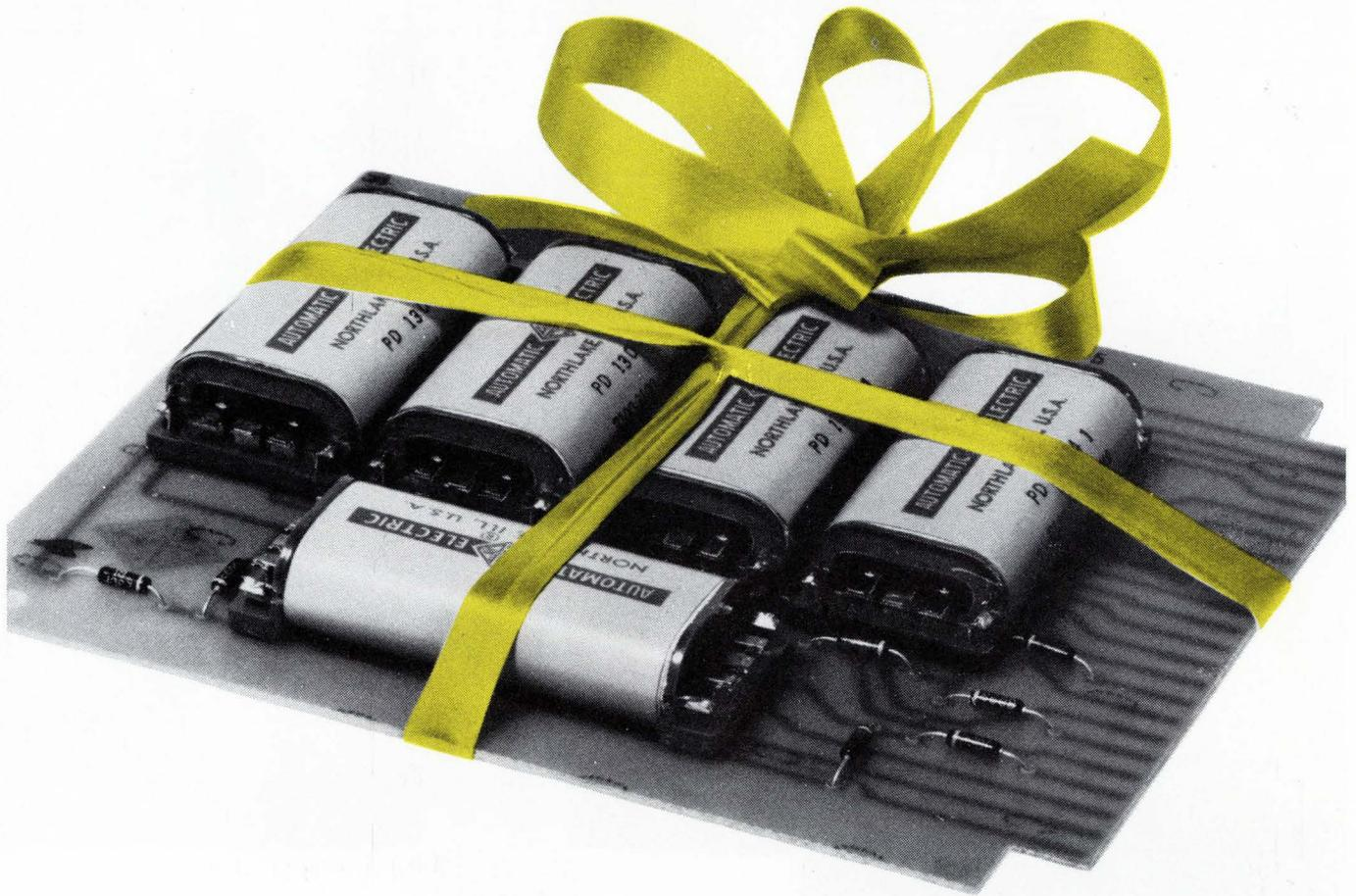
The Automatic Electric PC Correed (dry reed switch) is now available as an integral part of a complete printed circuit board assembly. It's made up of type G10 epoxy-glass laminate, 1/16 inch thick, with the necessary PC Correeds and associated components mounted and soldered. The assembly is a complete circuit package—ready for direct insertion into an edge-type connector.
