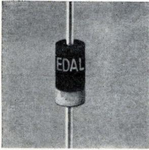
Subminiature silicon rectifiers have compact tubular construction and flexible leads that facilitate circuit mounting and provide high thermal conductivity. Length is  $\frac{1}{4}$  in. and diameter is 0.115 in. Voltage ratings for the series B223 run from 1,000 to 6,000 v piv; current ranges from 200 to 1,000 ma are standard. Edal Industries Inc., 4 Short Beach Rd., East Haven, Conn. [436]
