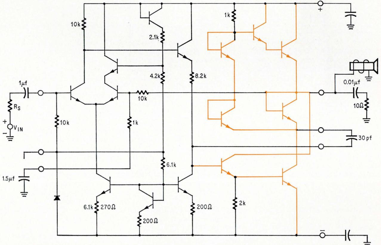
**Monolithic power.** Totem pole output stages boost power-handling capabilities of IC's. This circuit, Motorola's MC1554, produces 3-watt output as a class B amplifier.
