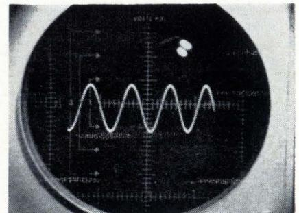
**Frequency division.** The frequency of the output sine wave is proportional to the filters angular velocity.
