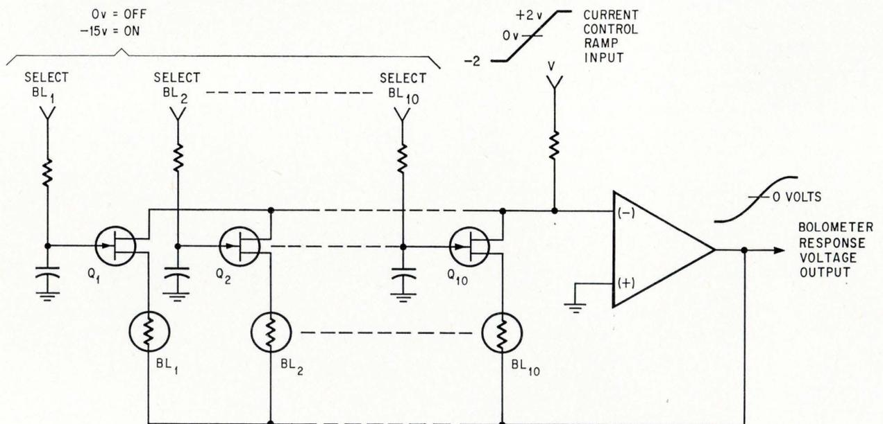
ALL CAPACITORS  $0.1\ \mu\text{f}$  MYLAR LOCATED AT TRANSISTOR
