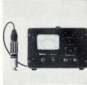
Pressure measurement is provided by a Pirani-type gauge, the Piravac S. The unit measures from 100 to  $10^{-3}$  torr, and two independent electronically-controlled relays can be set within the range of 100 torr to  $3 \times 10^{-2}$  torr while the instrument is in operation. Output terminals are provided for 10-mv recorders. Heraeus-Engelhard Vacuum Inc., 600 Seco Rd., Monroeville, Pa. 15146. [374]
