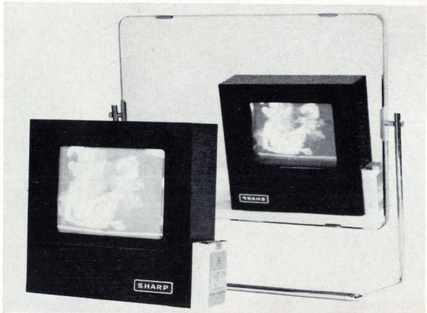
**Front and back.** Conductive-glass deflection electrodes make image visible from either side of flat cathode-ray tube.
