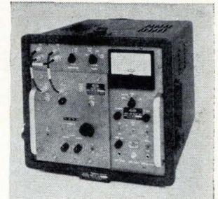
Tuning unit T-RW spans 2 to 75 Ghz and plugs into model TR general-purpose/antenna-pattern receiver. The first mixer is mounted externally for direct connection at the receiving antenna, at distances up to 100 ft from the receiver. Operating modes include a-m, f-m, c-w, and pulse. Price is \$2,750. Polarad Electronic Instruments, 34-02 Queens Blvd., Long Island City, N.Y. [404]
