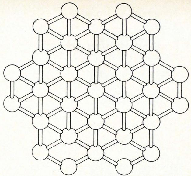
**Two way.** Along a 110 plane of the diamond structure at left, several atoms superimpose, leaving channels wide open for deep penetration by implanted ions. Along a 111 axis, at right, there are fewer atoms and channels are narrower.
