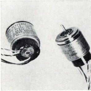
Limited rotation, long-life synchros feature hairspring conductors in place of brushes. They are for use where environmental conditions are detrimental to conventional brushes and rotation does not exceed 330°. The hairsprings pick off rotor winding information and allow a rotation of  $\pm 165^\circ$ . Harowe Servo Controls Inc., Westtown Rd., West Chester, Pa. 19380. [349]
