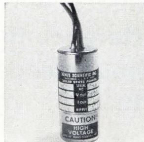
Model K15 photomultiplier power supply is a d-c/d-c converter that delivers up to 1 ma of current with a ripple of 0.1% or less for inputs ranging from  $\pm 35$  to  $\pm 15\text{ v d-c}$ . Output voltage is from  $\pm 300\text{ v}$  to  $\pm 1,500\text{ v}$ . The unit is reverse polarity protected. It measures 1 x 2 $\frac{1}{4}$  in. Price is \$178 in small quantities. Venus Scientific Inc., 25 Bloomingdale Rd., Hicksville, N.Y. [383]
