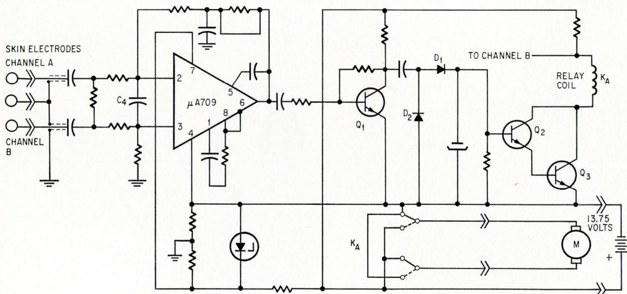
**Control amplifier.** Off-the-shelf integrated-circuit preamplifier stage saves space, cuts costs, and resists noise. Miniature relay  $K_A$  functions as on-off control for motor. Each two-channel amplifier can handle two actuators.
