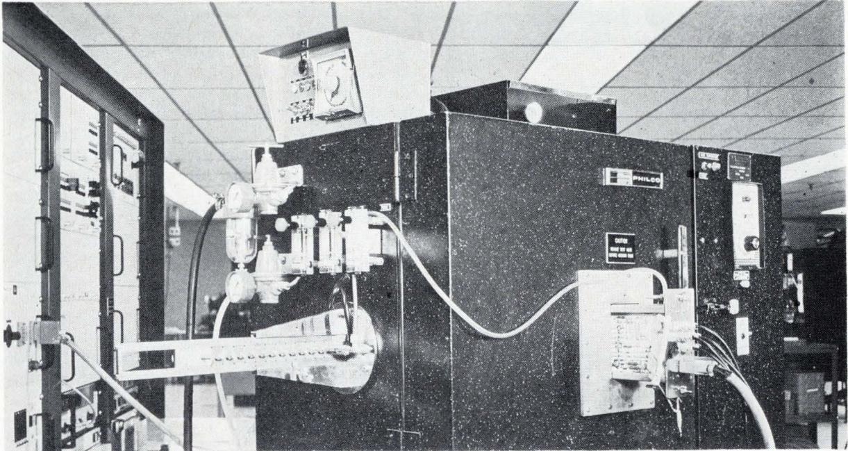
Environmental chamber blows IC's hot and cold.
