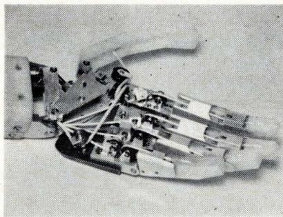
**Finger control.** Experimental Swedish prosthetic hand is first with five independent fingers.
