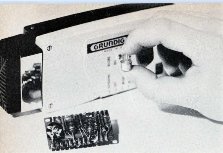
**Monolithic audio amplifier.** Hand-carried dictating machine uses IC amplifier. A three-stage audio circuit, Siemens AG's TAA311, replaces discrete components on printed circuit card in the Grundig Model EN-3 tape recorder.
