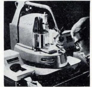
Thickness of evaporated and other thin-film deposits is measured and recorded by the Talystep. Step heights are electronically recorded at 8 magnifications from 5,000 X to 1,000,000 X. A variable stylus pressure of 0 to 30 milligrams prevents damage to soft deposits. Stylus tips are 0.0001, 0.0005, and 0.003 in. Engis Equipment Co., 8035 Austin Ave., Morton Grove, Ill. [428]
