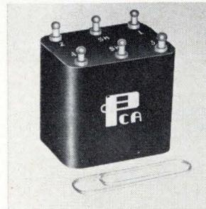
An interstage pulse transformer occupying 1 cu in. and weighing 75 grams can operate at altitudes up to 50,000 ft and withstand shock and vibration of 50 g. With a working voltage of 10 kv d-c, the unit has a 1:1 turns ratio, a rise time of 0.5  $\mu$ sec, and meets applicable MIL-T-27 specs. Price is \$32.42 in small quantities. PCA Electronics Inc., 16799 Schoenborn St., Sepulveda, Calif. [354]
