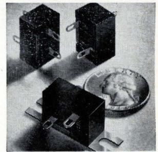
Single-phase bridge rectifier model S-896 is made from a superconductive selenium material. Life expectancy is over 100,000 hours when operated at full load at  $35^{\circ}\text{C}$ . The plastic-cased unit is rated at 60 ma and 230 v rms. It measures  $\frac{3}{8} \times \frac{25}{32} \times \frac{1}{2}$  in. high, exclusive of terminals. Price is 82 cents each in 100-unit lots. Sarkes Tarzian Inc., 415 N. College Ave., Bloomington, Ind. [443]
