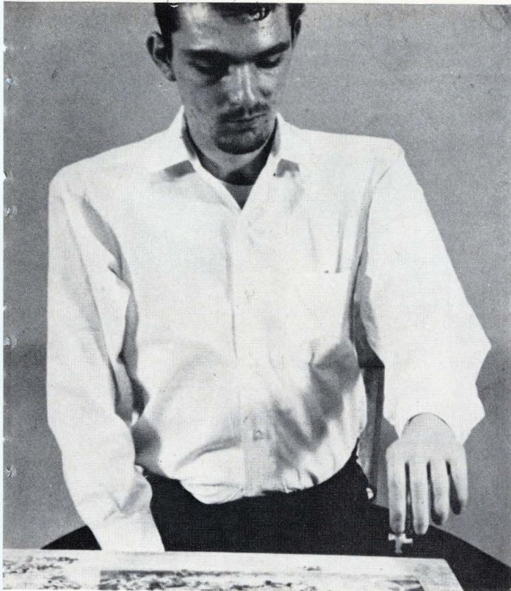
**Rehabilitation.** Fitted with myoelectrically controlled hand, this amputee demonstrates dexterity.
