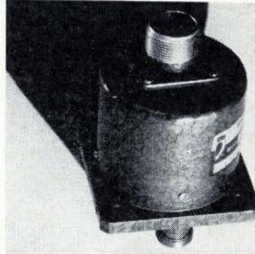
Fail-safe coaxial switches are single pole, triple throw. The SDN3120EFS provides minimum isolation of 60 db, max insertion loss of 0.2 db, and max vswr of 1.2, from d-c to 3 Ghz. Switching time is 10 msec and life expectancy is 1 million operations. Units return to position 1 in event of power failure. Price is \$325. Sage Laboratories Inc., 3 Huron Dr., Natick, Mass. [406]
