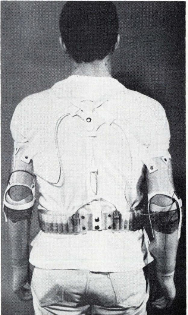
**Fitted out.** Patient with double amputation below the elbow wears myoelectric hands. Battery pack is installed on belt.
