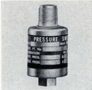
Absolute pressure switch 1857-2261 switches circuits in response to pressure changes in gases and liquids. It has a working range to 350 psi; burst pressure, 250% of proof rating. Electrical rating is 5 amps at 125 v, 60 hz, inductive or resistive; 4 amps at 30 v d-c resistive; 2.5 amps at 30 v d-c inductive. Occo Manufacturing Corp., 8 Romanelli Ave., S. Hackensack, N.J. [345]
