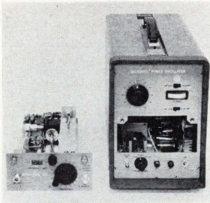
**Broad range.** Power meter reads over the visible and near-infrared spectrum.
