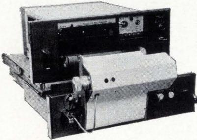
**Type 5-124**—Shown with the DataFlash Takeup Accessory which requires only 1 second to readout, the 5-124 has become a new "must" for industry. Portable, easy to operate, this instrument offers big recorder capability in a small-size, low-cost package. The 5-124 provides up to 18-channel print-out recording, 10 speed ranges, and record-drive systems with 16 options from 0.25 ipm to 128 ips.
