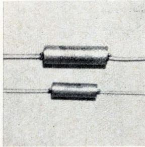
Miniature, metalized polycarbonate capacitors are for use in transistorized circuits requiring low-loss components. The 50-v devices need no voltage derating from  $-55^\circ$  to  $+125^\circ$  C. They exhibit a dissipation factor of less than 0.3% and an insulation resistance of 100,000 megohms at room temperature. Marshall Industries, 1960 Walker Ave., Monrovia, Calif. [342]
