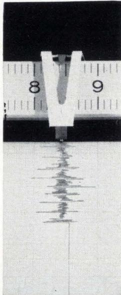
voltage electric writing method gives you sharp and clear printing on unique electro-sensitive paper—and with instant start-up.
