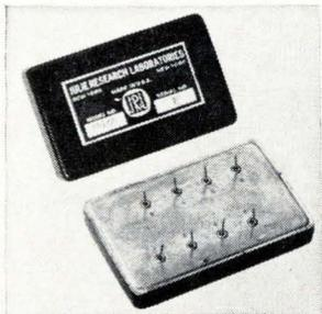
Precision resistor networks designed for plug-in to p-c boards cover a range from 10 ohms to 1 megohm. The line is available in accuracies from 0.0005% to 0.1% absolute and  $\pm 0.0002\%$  to  $\pm 0.1\%$  ratio. Stability is  $\pm 0.0015\%$  per year absolute and  $\pm 0.0002\%$  ratio. Price varies from \$20 to \$200. Julie Research Laboratories Inc., 211 W. 61st St., New York. [389]
