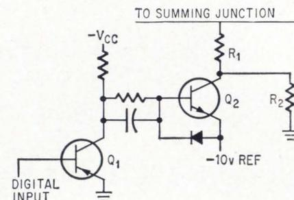
**Sums current.** A single current-summing stage consists of amplifying transistor  $Q_1$  driving switch  $Q_2$ . Resistor  $R_2$  shunts  $Q_2$ 's leakage current and is a low-impedance path for the discharge of stray capacitance.  $R_1$  is a precision resistor.
