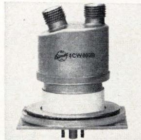
Power tetrodes 4CW800B and 4CW800F, designed for distributed amplifier applications, feature 4 individual circuit connectors to the active part of the grid. Filament voltage ratings are 6 v and 26.5 v, respectively. Units are capable of 1,000-w output. Minimum self-resonant frequency is over 900 Mhz. Eimac division, Varian Associates, 301 Industrial Way, San Carlos, Calif. [403]
