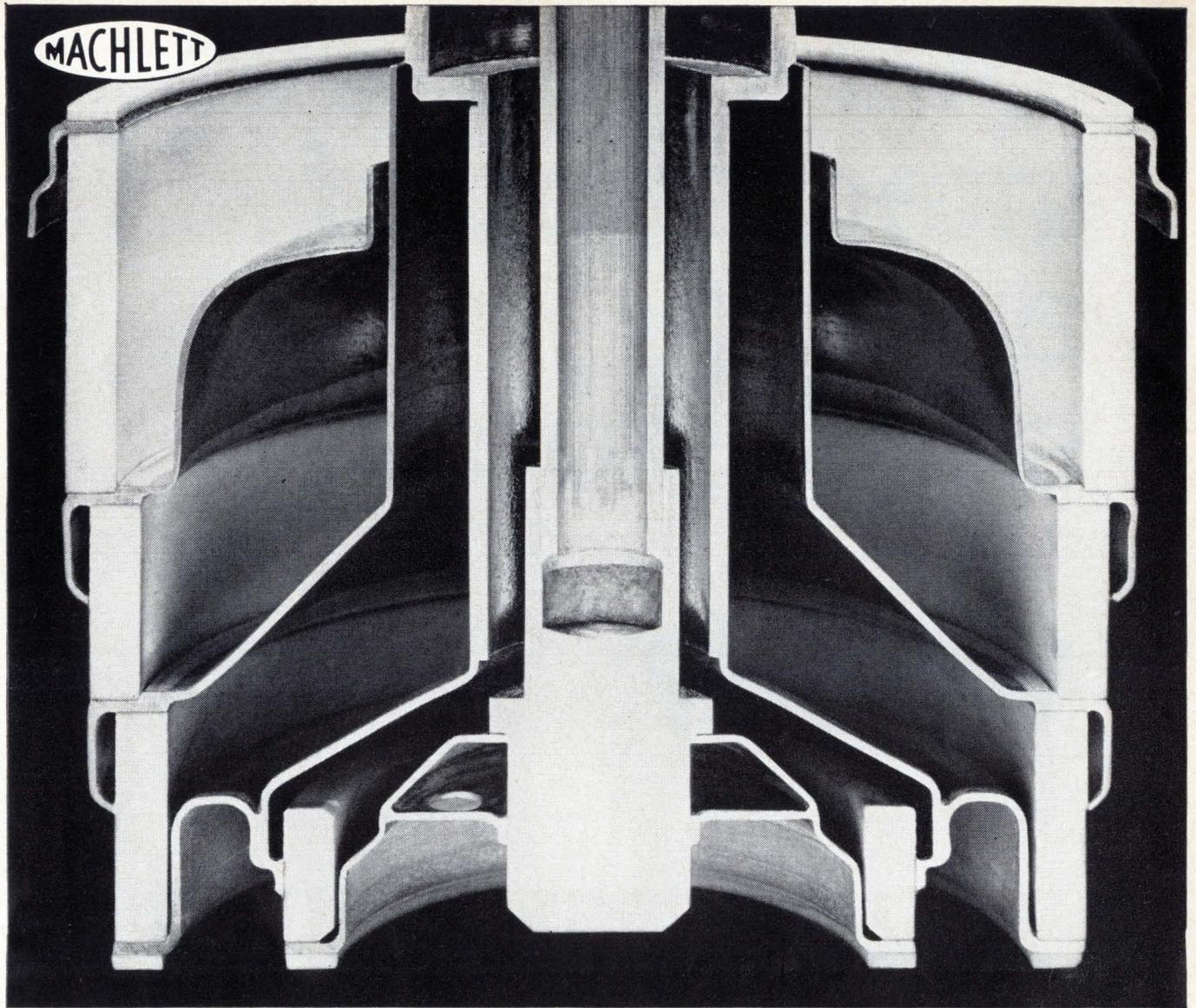
**Continuous cone electrode geometry: designed into all these tetrodes only by Machlett**
