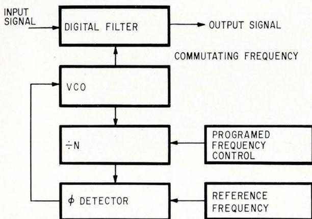
**Frequency hopping.** Stages for a digitally controlled system indicate the operation sequence. By regulating the voltage-controlled oscillator from the phase detector, the commutating frequency changes, thereby retuning the digital filter.
