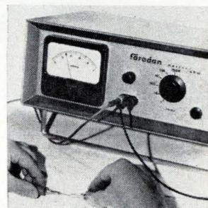
Ohmmeters for production lines have easy-to-read linear meters. Operational amplifier circuitry allows full-scale accuracy of 0.5%. Current through the item under test is 3 ma max on the 0-to-1-ohm scale. Model 40 has resistance scales of 0 to 1, 0 to 10, 0 to 100, 0 to 1,000, 0 to 10,000, and 0 to 100,000 ohms. Price is \$245. Faradan Corp., 4130 Menenes Ave., Riverside, Calif. [376]
