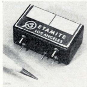
A solid state voltage switch, model RT-128-3, closes when a-c input voltage reaches 30 v rms  $\pm 10\%$ , 400 hz or more. With max input voltage of 45 v rms for 5 msec, it can be used in 28-v d-c gyro systems. It has 5 or 7 pins, 2- and 4-pole contacts, rated for 2 and 10 amps resistive. Betamite Electronic Devices, 6321 W. Slauson Ave., Culver City, Calif. 90230. [354]
