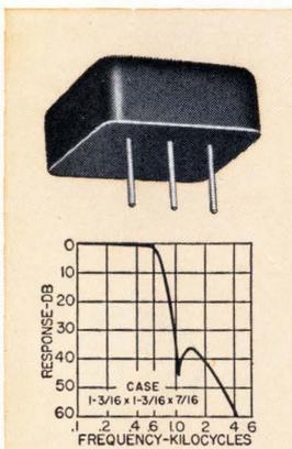
560 — Telemetering low pass filter. Available from 400 ~ to 70 KC.  $\pm$  7.5% bandwidth flat to 1 db. Attenuation greater than 35 db beyond the 2nd harmonic of  $\pm$  7.5% frequency. Impedance 47K ohms. MIL-F-18327B. Wt. 0.8 oz.
