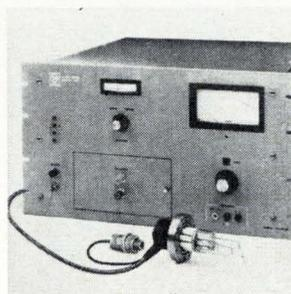
The Helmer gauge measures pressures obtained by vacuum equipment accurately down to  $1 \times 10^{-13}$  torr because the ion collector is optically shielded from the main source of X-ray current with no sacrifice in gauge sensitivity. Pressure is displayed on a single meter with a one-cycle logarithmic scale. Vacuum division, Varian Associates, 611 Hansen Way, Palo Alto, Calif. [371]
