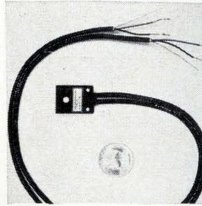
Hall-effect transducers measure steady-state, pulse, or transient currents without connection to the conductor under test. The CT-7W offers a rise time less than 1  $\mu$ sec, dynamic range of less than 1 ma to 30 amps peak, and frequency response flat to over 1 Mhz. It measures  $1\frac{3}{4} \times \frac{3}{8}$  in. with a  $\frac{3}{16}$ -in.-diameter opening. Ohio Semitronics Inc., 1205 Chesapeake Ave., Columbus, Ohio. [363]
