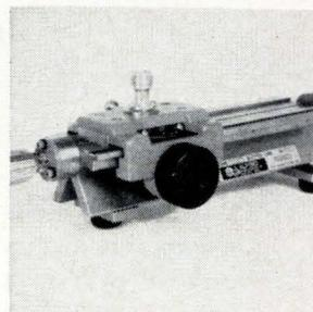
Precision 7-mm coaxial slotted line type 2852-05 is equipped with an APC-7 connector. It uses compensated dielectric pins instead of a conventional bead to support the inner conductor. Rated residual swr is under 1.025 up to 18 Ghz. Over-all dimensions are 2.7 x 3.6 x 10.6 in. Weight is 2.7 lbs. Price is \$1,140. Alford Manufacturing Co., 120 Cross St., Winchester, Mass. [415]
