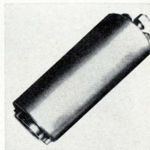
Infrared detector QKN1304 is for airborne and lab use. It uses an N-type indium-antimonide detector element that is sensitive in the 300-micron to 8-mm-long wavelength region, with 250-nsec response time. Standard aperture area is 4-mm diameter. Price is \$5,590; delivery time, from 30 to 60 days. Raytheon Co., 130 Second Ave., Waltham, Mass. 02154. [372]
