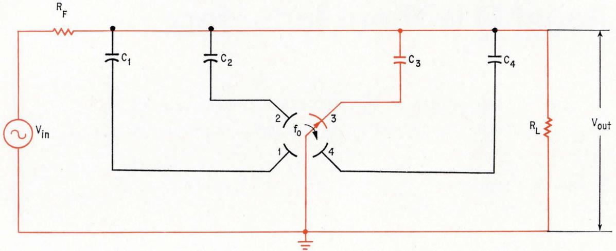
A simple shunt-switched digital filter is formed by connecting several capacitors in parallel to segments of a rotary switch. The circuit is returned to ground through a series resistor,  $R_F$ , and the switch. Output is the voltage developed across the grounded capacitor,  $C_3$ . Color indicates grounded capacitors in all diagrams.
