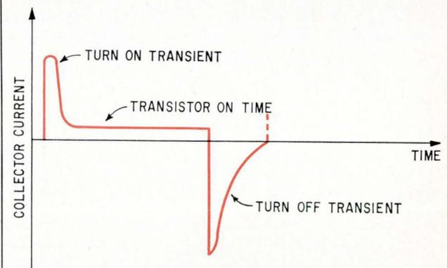
**On-off plot.** Positive regions of the current versus time plot represent the charge obtained from the external collector circuit of the switch. Charge stored in the base of the transistor is represented by the area of the negative-collector current spike. Transistor turn on is abrupt but the turn off occurs over a delayed period, needed to remove the charge.
