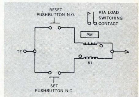
This double-duty circuit provides (1) memory and (2) switching from low level to 50 watts. Specify an inexpensive P&B dry reed relay and get high speed (in the low millisecond range), extremely long life (20 million operations) and compact size. Metal enclosures provide electrical shielding as well as physical protection for the coils and capsules.
