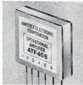
High-frequency, hybrid IC operational amplifiers are designated types ATF406 and ATF408. The thin-film circuits are fully frequency compensated at 25 khz for 6 db/octave rolloff. Open-loop gain is 100,000. Gain bandwidth product is 5 Mhz. Noise voltage is  $10 \mu\text{V}$  maximum. Micro-electronics division, Amperex Electronic Corp., Slatersville, R.I. [438]
