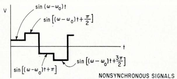
similar to that of a single-section LC filter. In its simplest form, the shunt-switched filter is represented by several parallel capacitors connected to segments of a rotary switch and returned to ground through the switch contact. The switch, which needn't be mechanical, rotates at a commutating frequency,  $f_0$ .
