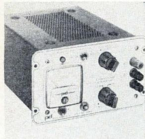
Regulated supply model 630 is suited for applications involving digital or linear IC's. It provides a continuously adjustable output voltage from 0 to 6 v at a maximum current of 3 amps. Dual concentric coarse and fine voltage controls enable voltage adjustment resolution of better than 1 mv. Power Designs Inc., 1700 Shames Dr., Westbury, N.Y. [385]
