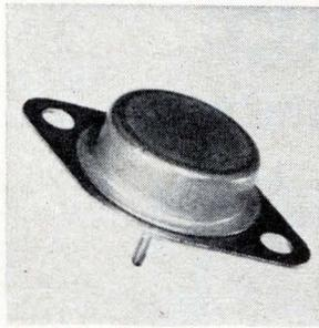
Six npn silicon transistors are available at 200, 300, and 400 VCER, with either 1- or 2-amp beta ratings. The 200-v units have a 200 VCEO(sus), the 300-v units have a 325VCEO(sus), and the 400-v units have a 400VCEO(sus). The entire line of triple-diffused devices has a power rating of 75 watts. Industro Transistor Corp., 35-10 36th Ave., Long Island City, N.Y. [437]
