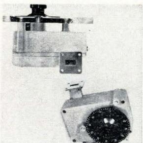
Eight compact, direct-reading attenuators span 7.05 to 90 Ghz. Attenuation range of each unit is 0 to 50 db. Vswr of 1.15, accuracies to  $\pm 0.5$  db, and maximum insertion losses of 0.5 db are attained. The units, all panel-mountable, range in price from \$350 to \$700. DeMornay-Bonardi division, Datapulse Inc., 1313 N. Lincoln Ave., Pasadena, Calif. 91103. [405]
