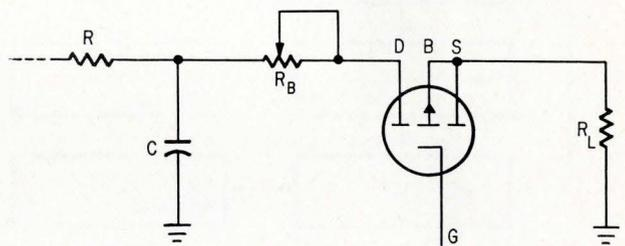
**Reducing noise.** For the FET, a balance network incorporating a potentiometer reduces the zero-signal voltage to below 50 microvolts.
