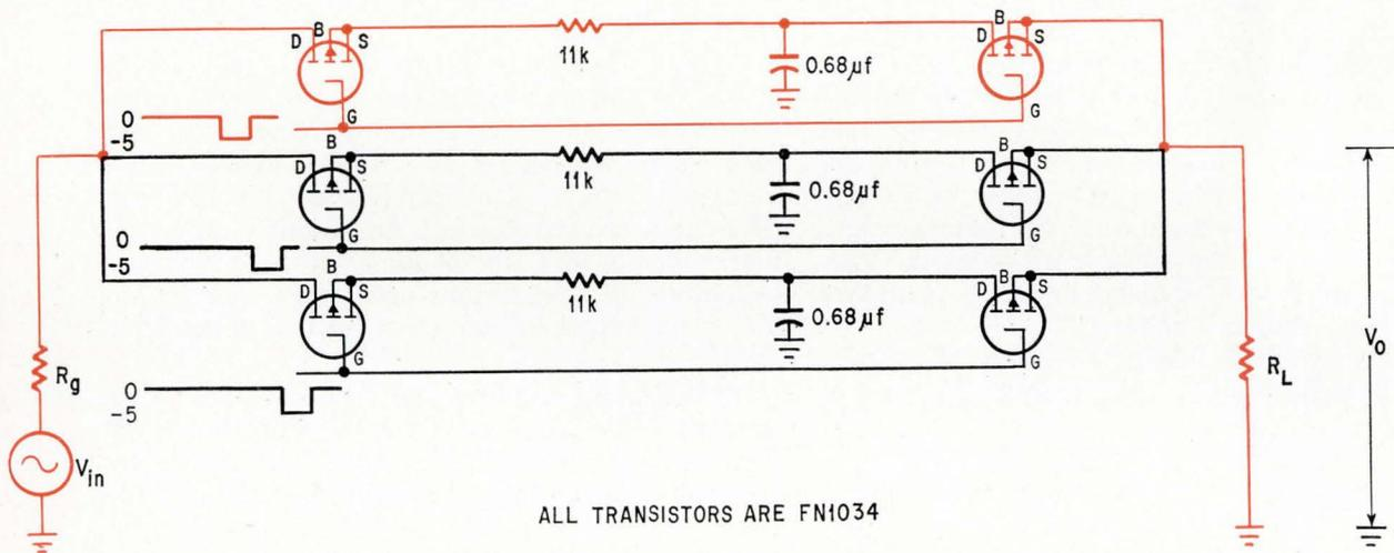
**Two field effect transistors** replace the pair of rotary switches used in the mechanical arrangement. Switching is controlled by a chain of delayed pulses applied to the coupled gates and the output is taken across the grounded capacitor.
