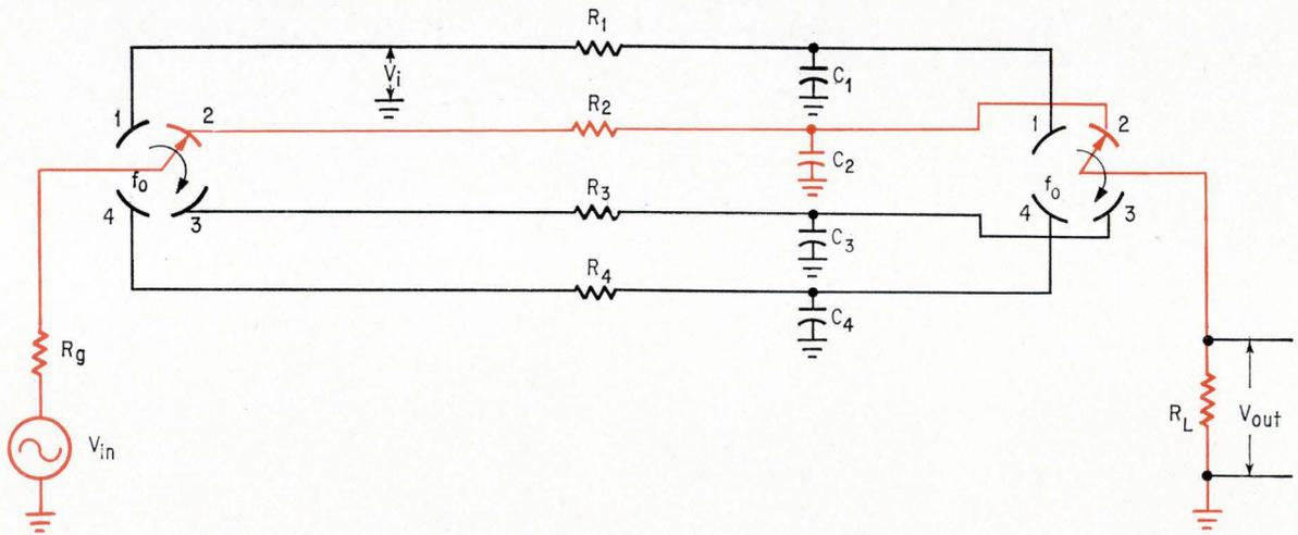
In the series-switched digital filter both the input and output signals are sampled by a pair of rotary switches revolving at a frequency  $f_0$ . Each time a pair of switches close, a quarter of a sine wave appears across the RC filter arm of the circuit. The output is the voltage developed across the grounded capacitor,  $C_2$ .
