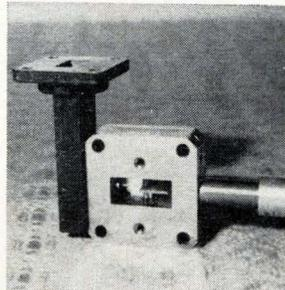
Frequency converter CX-7 has 8 to 12 Ghz (r-f) and 2 to 6 Ghz (i-f) bandwidths. Noise figure is 8 db; conversion loss, 7 db average. Harmonically related spurs are 30 db, other spurs 70 db below desired output for an input level of 3 mw or less. An i-o delivering 3 mw for low level and 20 mw for high level use at 14 Ghz is required. Spacekom Inc., Box 235, Goleta, Calif. [410]
