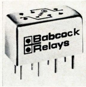
Half-size crystal can relays incorporate a magnetic circuit that locates the armature inside the coil, reducing leakage and coil power requirements for switching. Units, designated BR17 and BR16 for latching and nonlatching versions, require only 175 mw pull-in power to switch any load from dry circuit to 2 amps. Babcock Electronics Corp., 3501 Harbor Blvd., Costa Mesa, Calif. [347]
