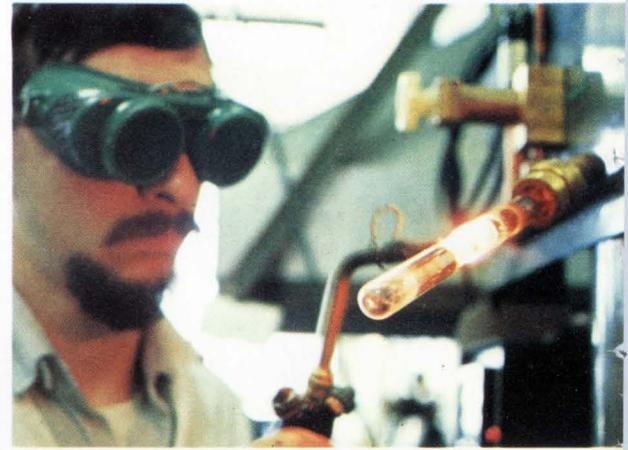
**Bomb fusing.** Technician prepares bomb by fusing the tube's open end, which is connected to a vacuum line to remove air.
