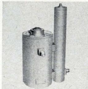
Pulse-amplifier cavity model 11026 can be used in phased-array and broadband-radar systems. It is rated at 10-kw output and operates in L band. Basic frequency is 425 Mhz and it is tuned manually. Bandwidth is 50 Mhz at 1.0-db points. Power input is 2.5 kw peak; maximum input vswr, 1.5:1. Microwave Cavity Laboratories Inc., 10 North Beach Ave., LaGrange, Ill. [414]
