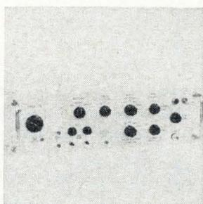
Phase measurements and impedance plots can be made with pulsed r-f signals using the model 306 pulse adapter. Among the applications is testing phase shift through microwave tubes with pulses as short as 0.2  $\mu\text{sec}$  and having a phase resolution of better than  $1^\circ$  from 2 Mhz to 40 Ghz. Wiltron Co., 930 East Meadow Dr., Palo Alto, Calif. [406]
