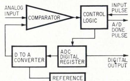
**Comparison made.** An input pulse triggers the control logic to set the most significant bit of the digital register. The bit is changed to a binary-weighted current in the digital-to-analog converter. The D/A current is then compared to the analog input, and the bit is either kept or rejected, depending on its size relative to the input current.
