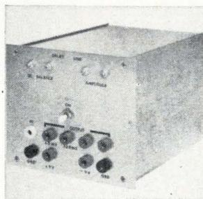
Portable active delay lines, called Delay Long, have applications in low-frequency signal-processing fields. Model APD 120 provides a delay of 120 msec. Delay to rise time ratio is 5:1. Input impedance is 1 megohm; output impedance, 4,000 ohms; maximum signal level,  $\pm 4$  v. Size is  $4\frac{5}{8} \times 5\frac{1}{4} \times 6\frac{5}{8}$  in.; price, \$650. A.P. Circuit Corp., 865 West End Ave., New York. [391]
