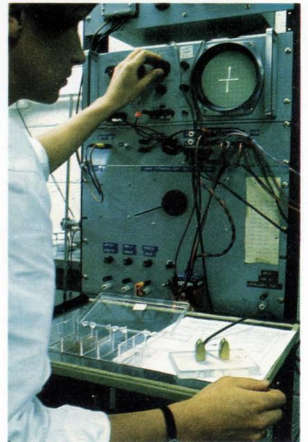
**Final test.** Symmetrical scope pattern tells the operator that there is a good switch in the test contacts on the table.
