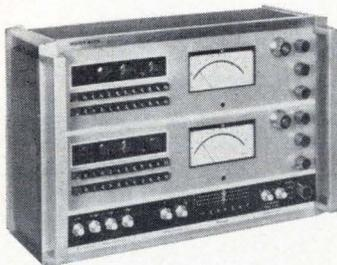
The Bridge produces analog voltage proportional to the meter readings and BCD (in a 1248 code), for the nixie readout.
