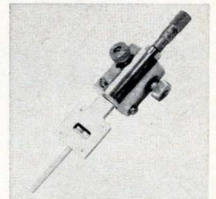
Model 410-A09 automatic frequency control and monitor cavity has a stability of  $\pm 1$  Mhz from  $-30^\circ$  to  $75^\circ$  C. It can be used to stabilize klystrons in discriminator circuits. The cavity offers a tuning resolution of  $\pm 0.5$  Mhz from 5.9 to 7.4 Ghz. A locking device protects the frequency setting against accidental change. Microlab/FXR, 10 Microlab Rd., Livingston, N.J. [416]
