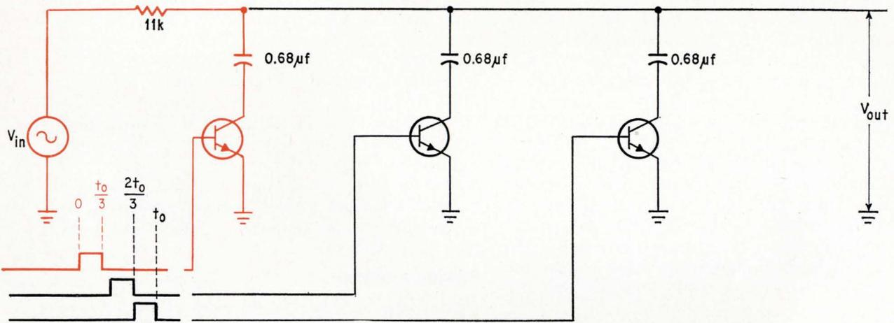
**Transistors** replace the rotary-switch segments used in the mechanical arrangement, and the switching is accomplished with a chain of delayed pulses. The output appears across the 0.68-microfarad capacitor. Circuits on this page are for three-section filters; opposite page contains four-section filters.
