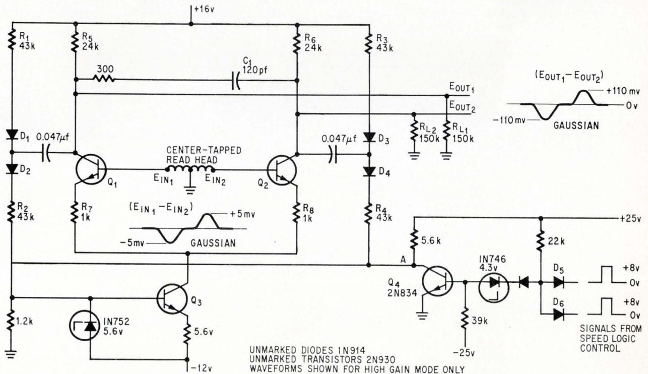
**Digital gain control.** Positive signals at D<sub>5</sub> and D<sub>6</sub> turn on Q<sub>4</sub>, and forward bias diodes D<sub>1</sub>, D<sub>3</sub>, D<sub>3</sub>, and D<sub>4</sub> so that resistors R<sub>1</sub>, R<sub>2</sub>, R<sub>3</sub>, and R<sub>4</sub> load the amplifier and reduce its gain.
