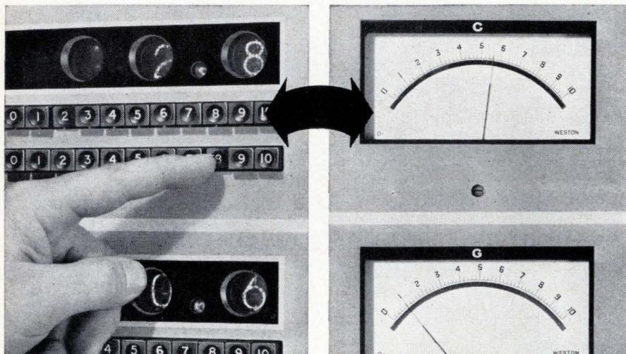
Once the Bridge is trimmed, a series of front-panel range push-buttons are suppressed in sequence until a reading is obtained on the meter. Setting up the first one or two digits of this reading on push-button decade controls gives the final reading.
