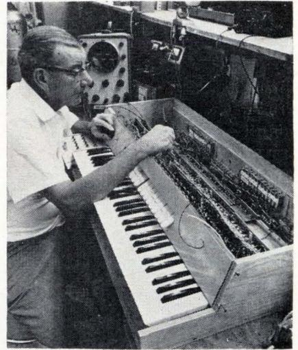
**On the inside.** Motorola engineers built this organ with a 5-octave, 61-note keyboard, and 18 function and voicing stops, to demonstrate what its new MOS IC's could do.
