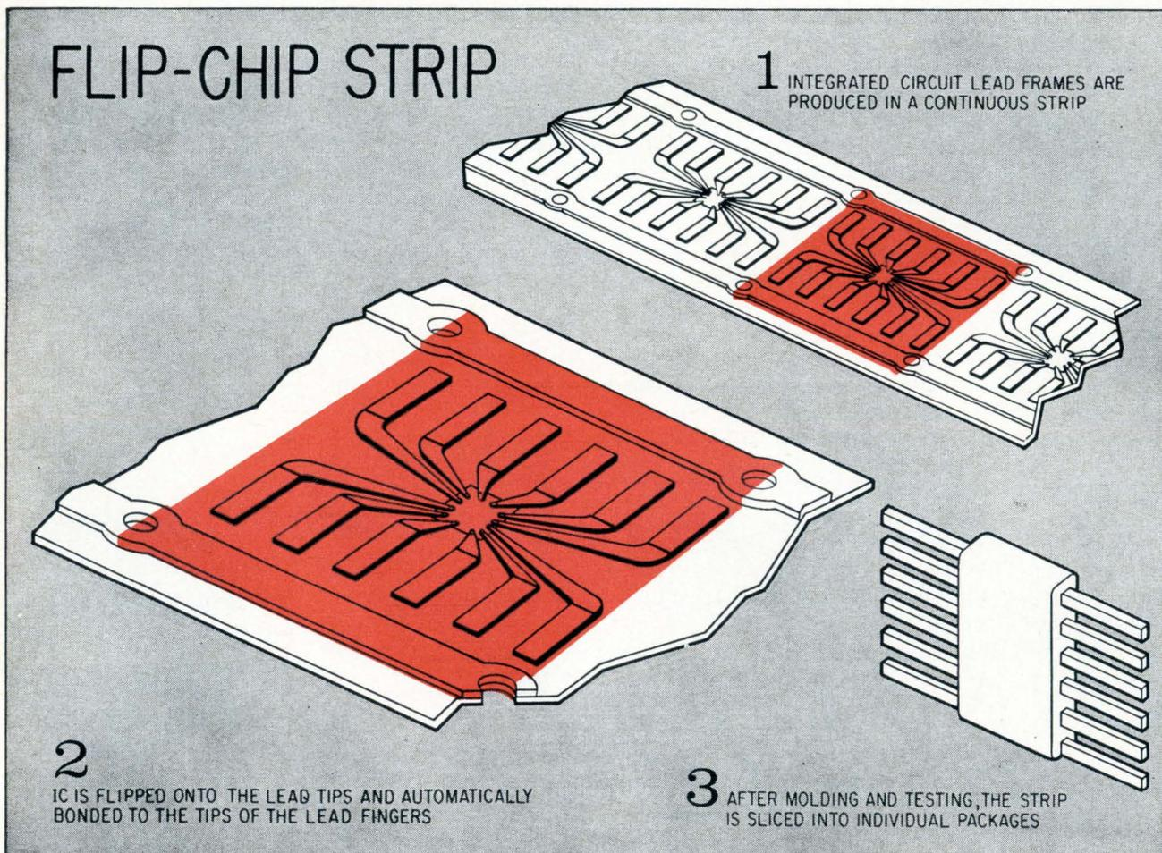
looks at a mirror underneath the strip and registers the chip optically, instead of referring both chip and frame to a third point, such as a microscope reticle.
