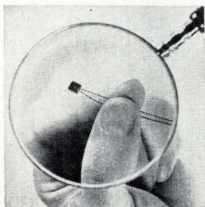
Ceramic-encapsulated platinum temperature transducer 5001-19 is designed for surface measurement over a range of  $-260^\circ$  to  $+400^\circ\text{C}$ . Resistance at  $32^\circ\text{C}$  is 500 ohms  $\pm 1\%$ , and resistance-vs.-temperature relationship is linear over the entire temperature range. Time constant is 250 msec; repeatability,  $\pm 0.1^\circ\text{C}$ . Thermal Systems Inc., 13920 S. Broadway, Gardena, Calif. [370]
