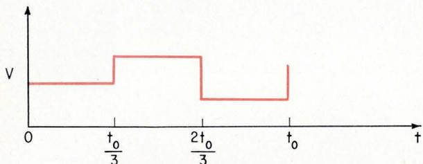
**Voltage waveshape.** Imperfection of transistor switches are obtained from the filter output's waveshape when the input is zero.
