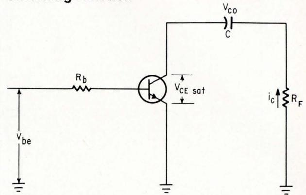
**Circuit operation.** An a-c switch requires current flow in both directions to charge and discharge the capacitor properly. When both the collector and emitter-base diodes are switched from reverse-bias potentials to their forward-bias values the transistor is turned on. To turn the transistor off, the charged stored in the base is removed and both the collector and emitter are reverse biased.
