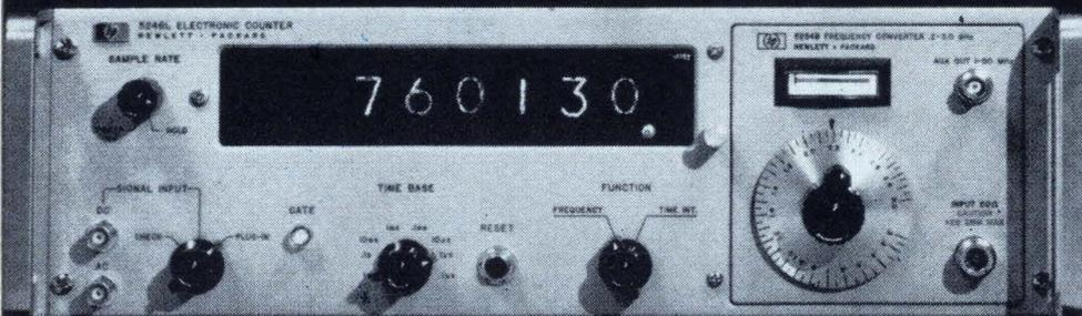
Model 5246L Counter with new 5254B Frequency Converter
