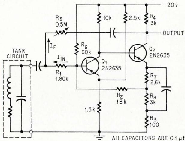
**Impedance converter.** Positive feedback through  $R_5$  and negative feedback through  $R_2$  combine to give amplifier  $Q_1$ - $Q_2$  a negative input impedance.
