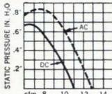
**VAX-1-AC** 26 v.a.c. (115 v.a.c. w/1.2 MFD capacitor in series), 400 cps, 320 MA, 2.0 MFD phasing capacitor 1 1/8" dia. x 1 1/2" long. 1.5 oz.
