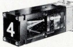
Illustrated: IEE Series 120 Readout—160° circular viewing angle; character boundaries  $\frac{5}{8}$ " wide horizontal band drawn through .800" D circle. Brightness to 100 F. L.
