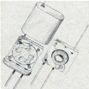
A six-pole quartz filter for use at or above 8 Mhz is contained in an HC 6/U package. The filter network is prepared using vacuum deposition with all resonators on a single quartz wafer. Foil leads are attached to the wafer and these leads, in turn, to the terminals of a p-c board. This allows 2 half-lattice sections on the wafer. Clevite Corp., 232 Forbes Rd., Bedford, Ohio. [353]
