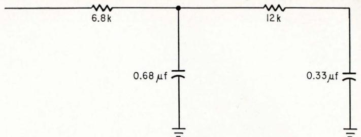
**Altering the response.** By changing the number of RC sections in a series-switched digital filter the engineer controls the shape of the frequency response. For a two-section filter the falloff is 12 decibels per octave.
