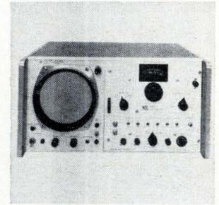
A spectrum analyzer designed for the community-antenna tv industry covers a range of 1 to 300 Mhz. A sensitivity of -90 dbm, flat responses, high stability, and spurious-free displays characterize its design. The Mark I analyzer has a 60-db display dynamic range and a 46-db distortion dynamic range. Price is \$1,500. Nelson-Ross Electronics Inc., 5-05 Burns Ave., Hicksville, N.Y. [368]
