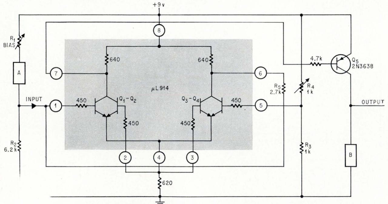
Versatile: The voltage at pin 1 turns on  $Q_1$ - $Q_2$ , turns off  $Q_3$ - $Q_4$ , and saturates output transistor  $Q_5$ .
