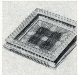
Core memory storage planes called Platrics can be used in memory systems for digital instrumentation and control equipment. A stack of Platrics is mounted on a p-c board through connection pins at the bottom of the stack. Units are available in 8 standard configurations with bit capacities ranging from 256 to 1,024. Ferroxcube Corp., Saugerties, N.Y. 12477. [352]
