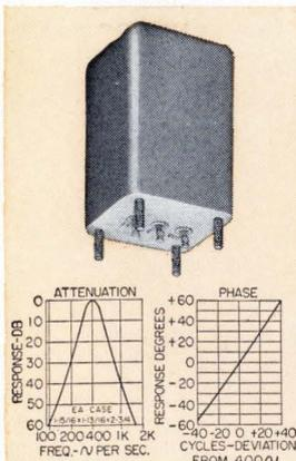
Band pass 400 cycle Gaussian filter. Linear phase response in pass band. Attenuation 380 to 420 cps within 0.5 db. 2nd harmonic down 25 db, 3rd harmonic down 45 db. Source and load 5K ohms. MIL-F-18327B Wt., 0.9 lbs.
