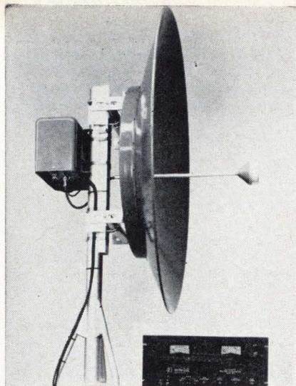
**Four-foot dish.** Mounted behind antenna is transmitter sending to . . .
