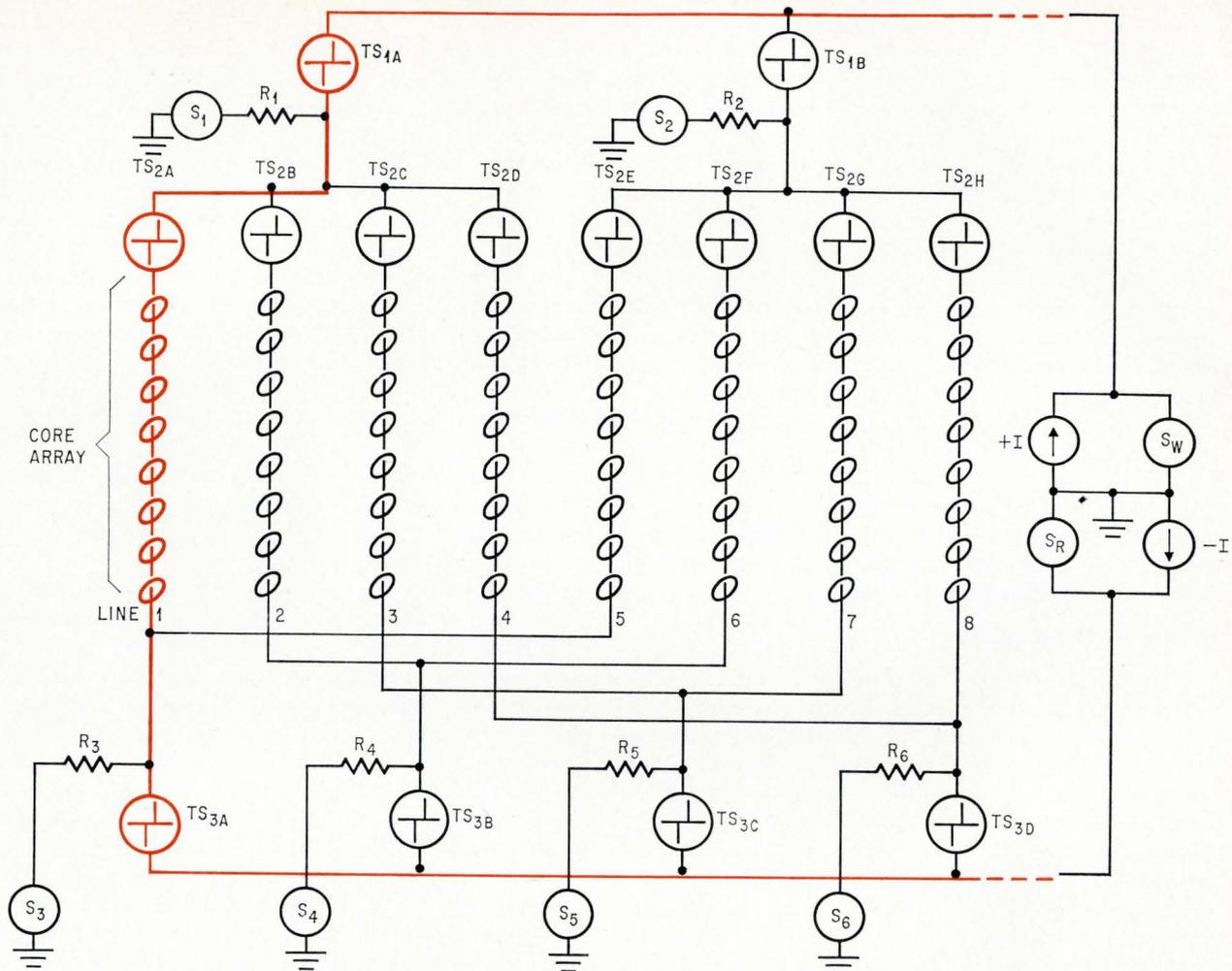
**Dual-polarity drivers.** Partial internal decoding is possible when threshold switches are applied as dual-polarity drivers. External decoding is still required for switches at bottom. One complete loop for a half-select current is shown in color.
