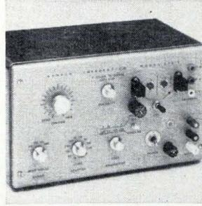
Transistor curve tracer CTA-2 displays a family of curves for both bipolar and field effect devices when used with any general purpose d-c scope. Base current steps of 20, 100, and 200  $\mu$ a are provided with 4 ranges of sweep voltage to 240 v. Voltage steps for FET testing are continuously adjustable. Price is \$435. Rameco Corp., Box 580, Deerfield Beach, Fla. [362]
