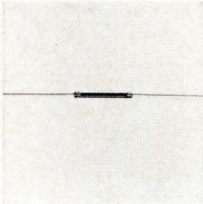
Resistors with 0.1-in. diameter, range in values from 10 to 5,000 megohms in the  $\frac{1}{4}$ -watt size, type HACW, and 10 to 10,000 megohms in the  $\frac{1}{2}$ -watt size, type HADW. They are rated at 1,000 v and 5,000 v maximum, respectively. Both are terminated with  $1\frac{1}{2}$ -in., No. 20 tinned-copper leads. Prices start at \$2.50. Resistance Products Co., Harrisburg, Pa. [345]
