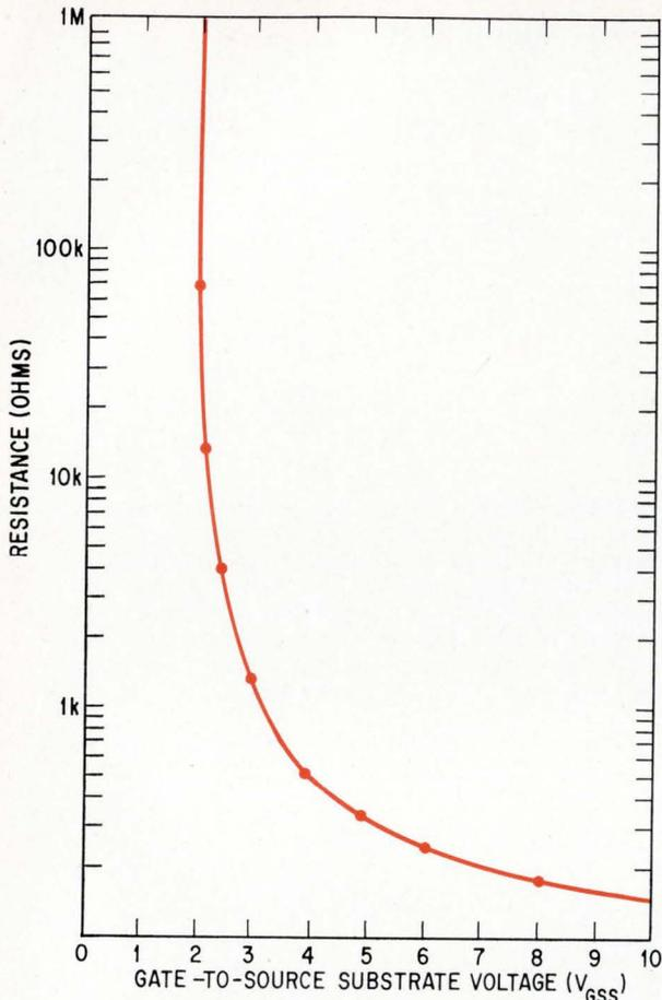
**Switching capabilities.** Plot of gate-to-source substrate voltage versus resistance for an MOS field effect transistor indicates a value of 200 ohms when  $V_{GSS}$  equals 5 volts. Resistance increases infinitely at  $V_{GSS}$  of 2 volts.
