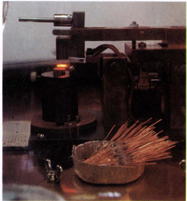
**Package sealing.** Resistance-heating coil around the switch assembly fuses the glass film to the upper lead and seals the switch.
