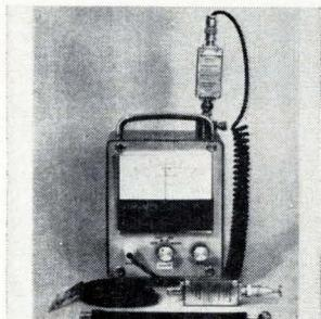
Charge detector CM467 measures electrostatic fields. Two interchangeable sensor probes are available. One measures charges in the  $10^{-9}$  coulomb range by direct contact. The other measures charges as low as  $10^{-12}$  coulombs, and is used for remote monitoring. Price of the Coulometer, with either probe is \$195. Metronics Associates Inc., 3201 Porter Drive, Palo Alto, Calif. [373]
