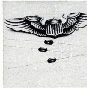
Fast-recovery rectifiers IN4942, -4, -6, -7, and -8 are suited for use in high-reliability airborne- and missile-power supplies. Typical reverse recovery is 100 nsec up to 600 v, and 250 nsec up to 1,000 v piv. Units handle 1-amp average rectified current at  $55^\circ\text{C}$ , with low leakage current of  $0.1 \mu\text{A}$  at rated piv,  $25^\circ\text{C}$ . Semtech Corp., 652 Mitchell Rd., Newbury Park, Calif. [442]
