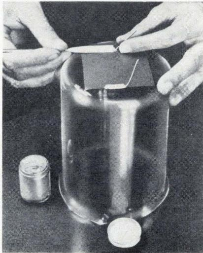
A cement containing silver in a thermosetting resin has good conductivity under a variety of environmental conditions. It can be
