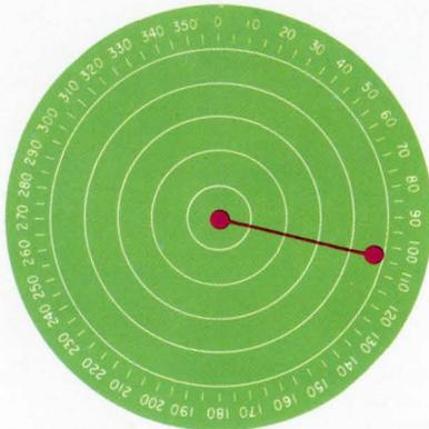
When the target is designated, the calculator automatically estimates its position. If the radar input from the target exceeds a predetermined signal-to-noise threshold, a binary 1 is generated. The range is divided into  $\frac{1}{4}$  mile intervals, or cells. When three consecutive 1's (one per sweep) are received in adjacent range cells, the target is confirmed. Three 0's in a row mark the end of the target. The azimuth position of a target is calculated from the start and end signals.
