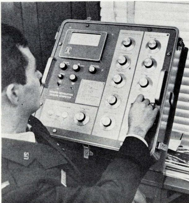
**Ground resolution** analog computer predicts resolution for a given sensor under expected conditions.
