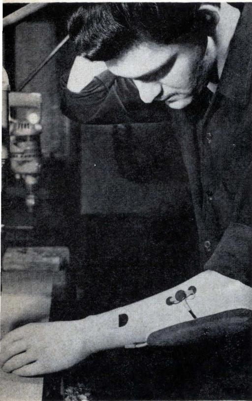
**Steady.** Electromyographic-controlled artificial hand manufactured in Austria has selective amplifier circuits that protect users from spurious finger movements.
