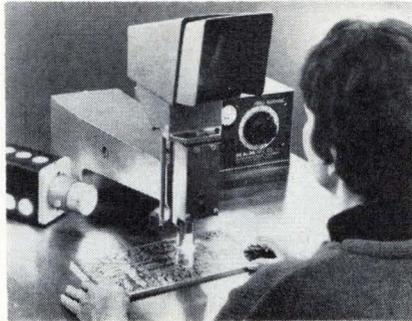
Though the prime purpose of a new production drill is to make holes in stacks of circuit boards, it is also useful for drilling very small holes, to exact specifications.
