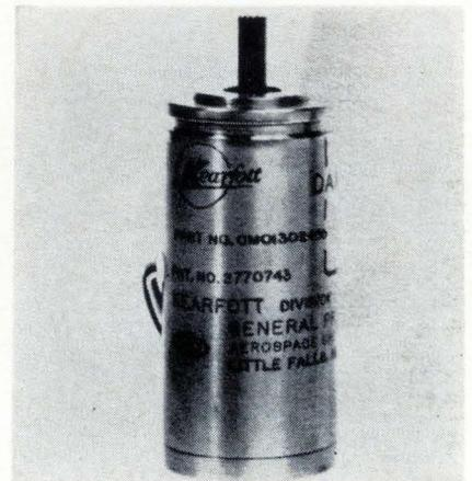
A size 8 inertial damped servo-motor is suited for high-gain or high-speed servosystem applications. Weighing only 2.6 oz, the component is totally enclosed within a single stainless steel housing measuring only 1.68 in. in length. A rugged and reliable 400-hz unit, the motor has two windings on the control phase, permitting either series or parallel operation. Stainless steel, high-precision bearings assure long, trouble-free service.
