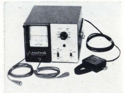
A portable power tester and recorder handles voltage, current, or both. The instrument features a time-sharing system that permits the stylus to record independent traces for both voltage and current. This system provides full chart-width resolution with voltage plotted as a continuous trace and current as an interrupted trace for easy identification.
