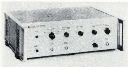
Pulses with rise and fall times less than a nanosecond are supplied by a new pulse generator. The unit is suitable for testing state-of-the-art oscilloscopes, broadband amplifiers, high-speed solid state switching circuits, nuclear instruments, coaxial cables, (by time domain reflectometry) and other analog circuits.
