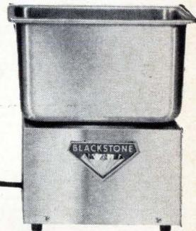
Enables precision scrubbing of a variety of small parts including... electronic components, printed circuit boards, sub-assemblies, optical equipment and assembled instruments or parts at strategically located cleaning stations. Available with two tank capacities — .5 gallon (Model SOBCT.5) and 1 gallon (Model S1BCT1). Tanks removable from assembly for emptying. High efficiency lead zirconate titanate transducer. Solid state, automatically-tuned generator.
