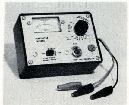
A go-no-go type, battery-operated instrument determines whether transistors are operational or faulty. Model 20 will show, in two steps, whether the transistor type is npn or pnp, if it is operating properly, and its d-c beta.
