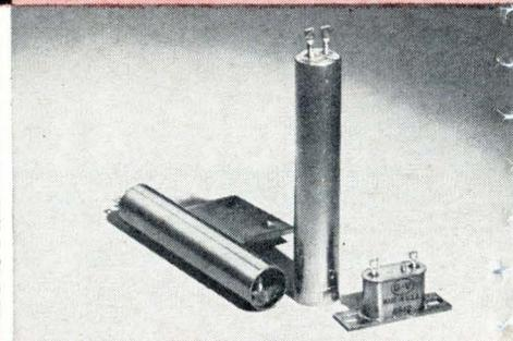
**Cartridge Type:** Series C8 hermetically sealed and still adjustable. Contact rating up to 5 amps. **Crystal Can Size:** Series VE-2 hermetically sealed. Contact rating up to 3 amps. **Features:** Rapid rate of response; minimal differential; operating range,  $-65^{\circ}$  to  $+300^{\circ}\text{F}$ ; vibration to 2000 Hz; shock to 50g.
