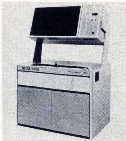
The first of a new family of incremental plotters operates at 800 steps per second. The series features high speed and accuracy,
