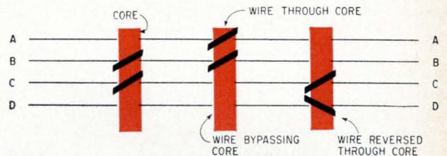
Transformer memory contains, in most cases, a series of cores plus wires that either thread or do not thread each core. In the symbolic diagram at the bottom, a slash mark indicates both the presence and the direction of a wire passing through a core.
