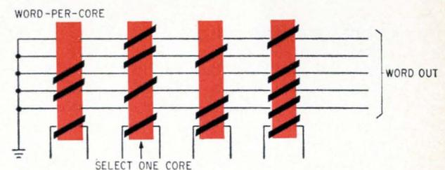
Word-per-core organization is basis of rope memory. The wires making up the rope are sense wires on which a word appears when a single core is switched.
