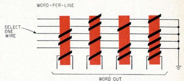
Word-per-line organization is basis of braid memory. The wires making up the braid are word lines. They couple a signal to sense lines by way of the cores.
