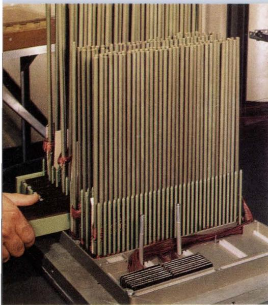
The completed braid is transferred from the temporary separators onto the nails. When the vertical slide is pulled out, the separators and braid drop into the frame. After the separators are removed, the nails retain the braid separations. Replacing the slide holds the braid down so that a new braid can be woven on top of the previous ones.
