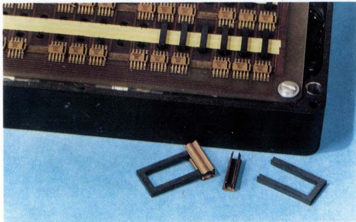
The sense board, with some cores in place, is mounted on the braid. Multiturn sense windings are part of the multilayer board. Two U-cores and their cross-pieces are at the bottom.
