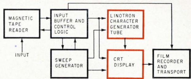
**Linotron photocomposing system** accepts instructions on magnetic tape, generates electronic analogs of characters in the Linotron tube and displays 1,000 characters per second on the cathode-ray tube. Printing plate is made from photograph taken of crt faceplate.
