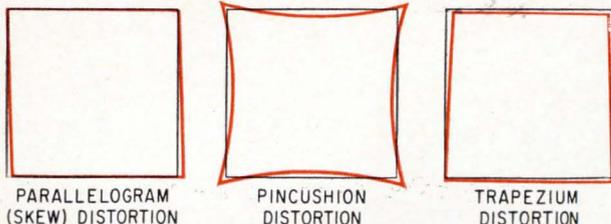
PARALLELOGRAM (SKEW) DISTORTION
