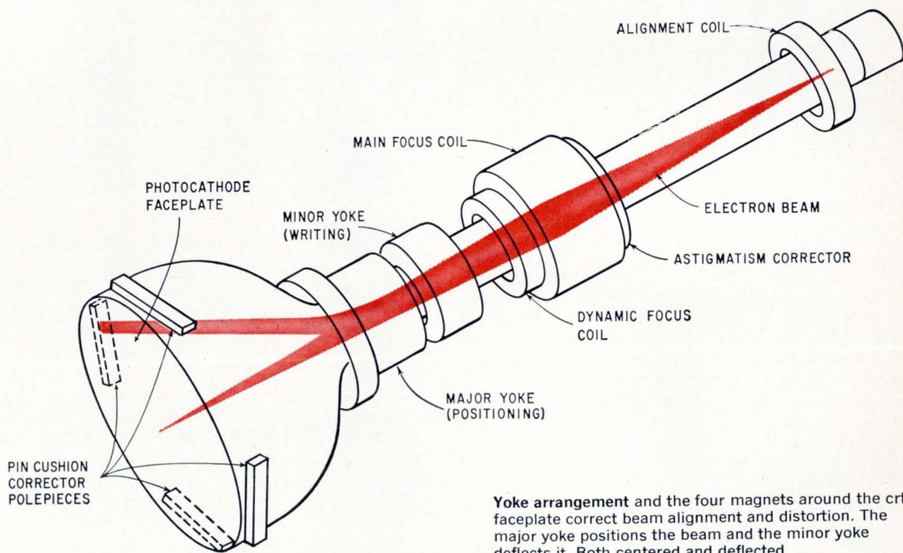
Yoke arrangement and the four magnets around the crt faceplate correct beam alignment and distortion. The major yoke positions the beam and the minor yoke deflects it. Both centered and deflected beams are shown.
