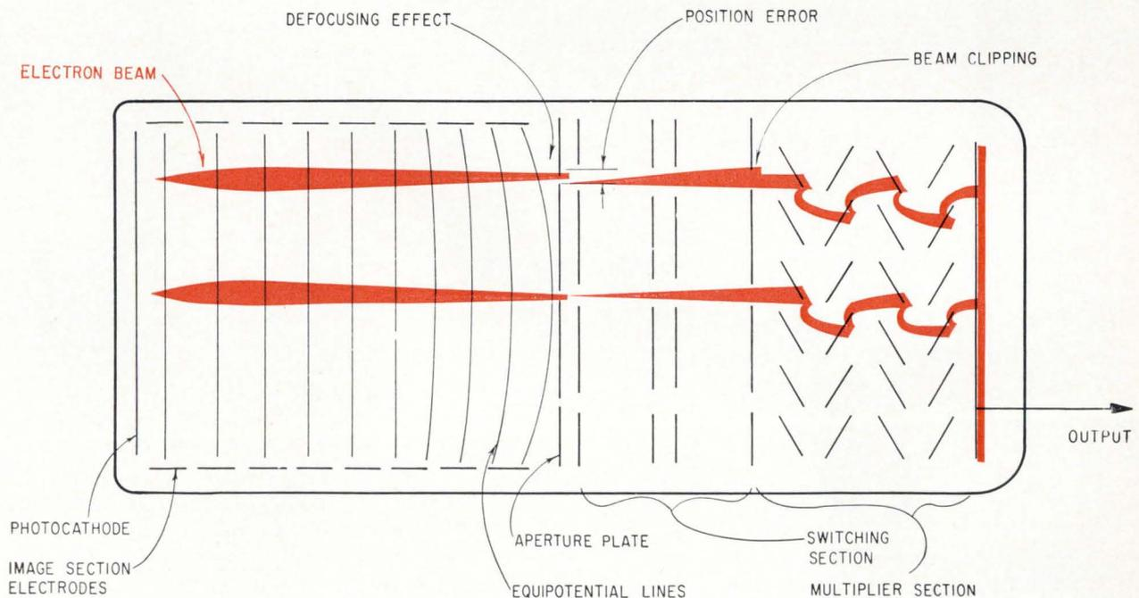
A uniform electrostatic field in the image section and the switching and multiplier sections (the beam at the center). If the field were not uniform, an off-axis beam (the upper beam) would not be focused exactly at its aperture. The result would be characters printed out of focus or with nonuniform intensities.
