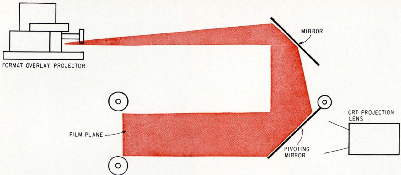
**Standard overlays** may be projected onto film after completed page has been composed. Pivoting mirror drops into place so that it reflects slide image from format overlay projector.
