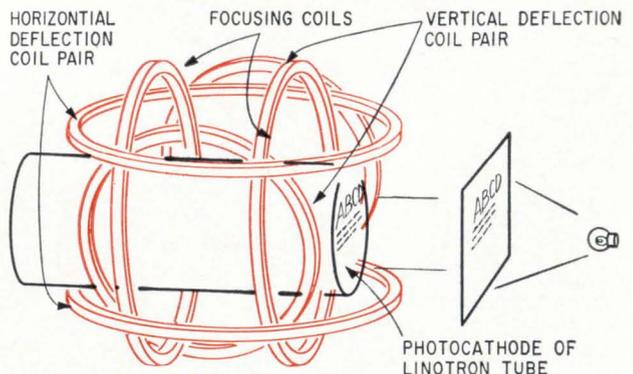
**Helmholtz coils** over the image section focus the beams at the aperture plate and scan them across the aperture holes.
