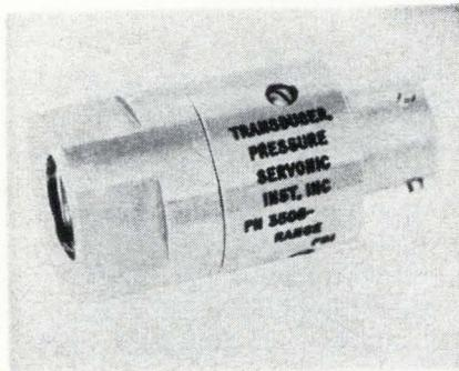
A semiconductor strain-gauge pressure transducer that provides an unamplified 1-volt output is intended for both airborne and industrial uses. It will measure and monitor air, fuel, lubricants, hydraulic fluids, and corrosive gases and liquids.
