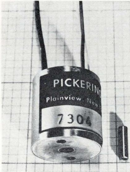
Conversion of motion to linear d-c output from 6-v d-c input is achieved by a linear variable differential transformer. Besides measuring, detecting, and controlling linear motion from a d-c supply, the unit can also be used for force and pressure measurement.
