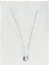
The Sippican Expendable Bathythermograph System accurately and rapidly measures and records the temperature of ocean waters down to depths of 1,500 feet. Heart of the system is an 8-inch probe, that carries, as its temperature-sensing element, a miniature-sized thermistor, shown on the left.
