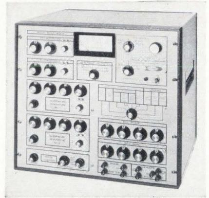
built with solid state devices, which operates over the frequency range from 4 khz to 500 khz.
