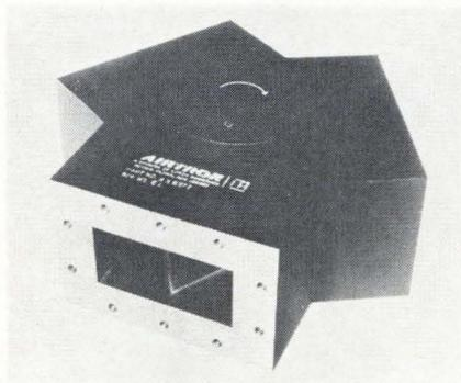
Application of a high-power ferrite material makes possible a junction circulator that can handle 5 kilowatts c-w at 2.4 to 2.5 Ghz. This is reportedly about 10 times the capability of previous units. The necessary electrical symmetry is provided by a Y-junction.
