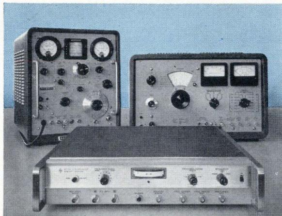
Using the HP 8708A Synchronizer with the improved 606B and 608F Signal Generators gives you a frequency stability of  $2 \times 10^7$  per ten minutes over the universally important range of 50 KHz to 455 MHz. This is a 250 times improvement over previous signal generator performance. And that's at any frequency you choose, not just at discrete points.
