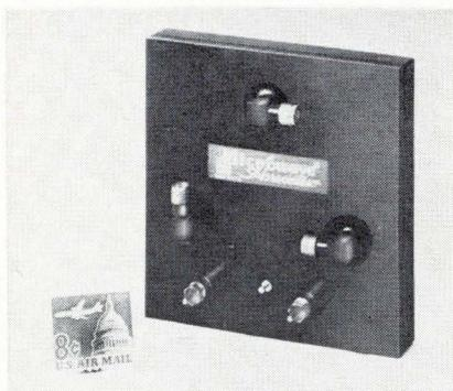
Designed for fast switching, a coaxial spdt diode switch is suited for antenna lobing in compact commercial transponder systems.
