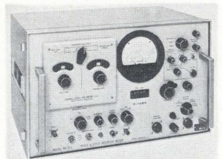
Automatic scanning is featured in a solid state noise and field intensity meter. The instrument is designed to meet the requirements of all applicable federal and military standards and specifications.
