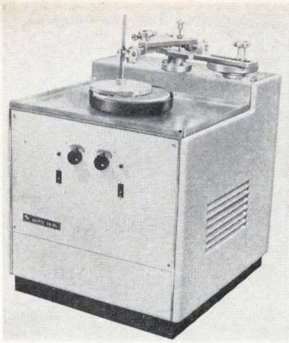
The Model PAS18 is powered by a  $\frac{3}{4}$ -horsepower motor with continuous variable speed control up to 175 rpm. The 18-in. stainless steel wheel rests on a heavy duty 8-in. thrust bearing. The polishing wheel will accommodate four  $6\frac{3}{4}$ -in.-diameter pressure plates that can be independently driven to accelerate the polishing action.
