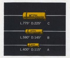
During 3.500.000 unit hours of life test at 85°C, at full rated voltage, using a low impedance power source, not one MTPH capacitor has failed through short circuiting or excessive DC leakage current. Type MTPH capacitors were developed by Mallory as a result of experience
