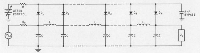
Circuit diagram of stripline attenuator. The line's distributed contents are represented by C and L.
