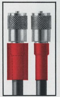
New ITT Heat Shrink Tubing easily fits over coax connector, yet, because it shrinks to 50% of its original size with the application of heat, the tubing forms a tight insulating bond around both the coax and the connector.
