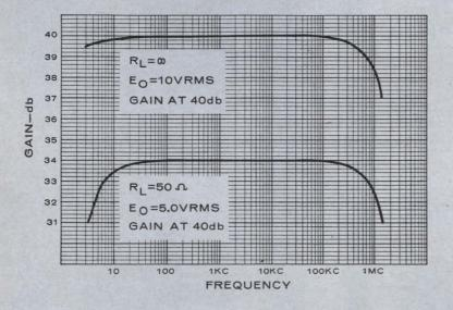
Here's a wide bandwidth solid-state, amplifier useful as a generalpurpose lab instrument, an oscilloscope preamp, an in-system amplifier component. With its 5 x 10° power gain, it serves as an excellent power amplifier for solid-state oscillators, and its 10megohm to 50-ohm impedance ratio make it ideal for application as an impedance converter.
