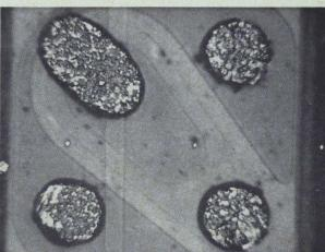
**Bump-contacted chip.** In this one, npn and pnp transistors share contacts 1 and 3. Photo shows top of chip. Large bump orients chip.
