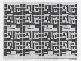
After copper plating, resistor networks look like this. There are eight networks on the substrate.
