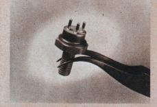
NPN silicon annular amplifier transistor (2N3818) provides 18 watts output power @ 100 mc using 25 volt source.
