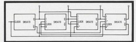
Figure 3, This complete synchronous binary decade counter uses only four SN5470 flip-flops
