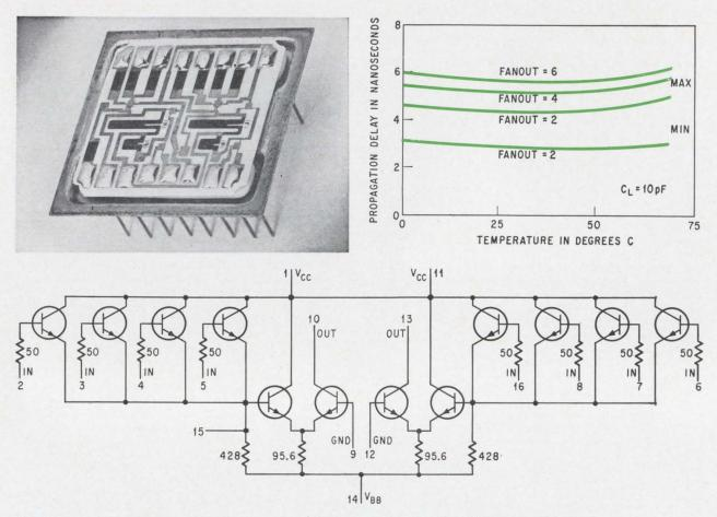
**Dual four-input gate circuit**, schematic and propagation-delay characteristics. While the schematic shows eight individual transistors being used with the eight input resistors, the actual circuit has a single multiple device in each input section. Note the tailoring notches and guide marks at the precision resistors.
