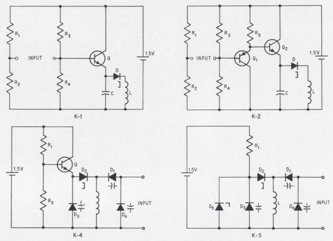
**Tunnel diode oscillator** circuits used in biotelemetry transmitters designed at Case Institute of Technology. In the K-1 and K-2 models, the bias of the tunnel diode is varied to change the oscillating frequency. The K-4 and K-5 units use a varactor-diode to vary the tuned-tank circuit resonance.
