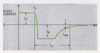
**Reverse recovery time,**  $t_{rr}$  is measured between the turnoff point  $t_0$  to point where reverse recovery current,  $I_{RR}$ is 10% of the turn-off current  $I_R$ , which is equal in magnitude to  $I_F$ , the forward bias current.
