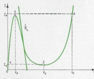
Tunnel diode current-voltage characteristic. Negative resistance exhibited over segment bc allows device to function as oscillator. Load line with slope  $1/R_L$  is for astable operation.
