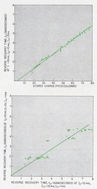
**Correlation between reverse recovery time** measurement and stored charge measurement techniques is shown in the top graph. Deviation from the straight line which shows exact correlation is largely due to the reverse recovery time measurement. This is illustrated in the lower graph, a correlation plot of reverse recovery time measurements on the same group of diodes for two test conditions.
