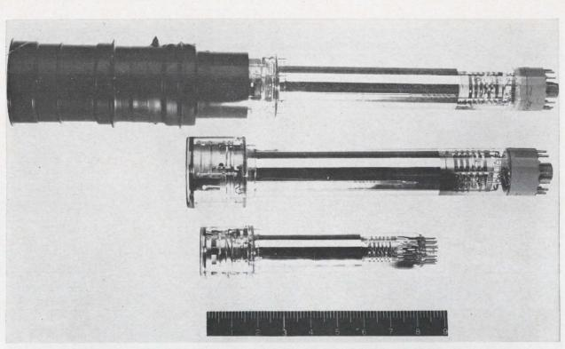
**Three image orthicons** made by RCA for low light level tv. The bottom tube is a 2-inch model, the middle a 3-inch tube, and the top a 3-inch tube fitted with a two-stage image intensifier section.
