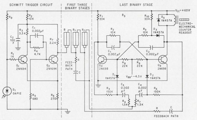
**Counter consists** of a photocell, Schmitt trigger, four binary circuits in series, and an electromechanical counter readout. Each time the photocell is unblocked from its light source, the Schmitt trigger produces an output pulse that changes the state of the binary circuits.
