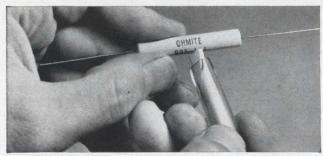
**ABRADE IT!** Use a glass fiber eraser, for example, on the markings. Rub them hard. Nothing happens. The markings don't come off, because they are vitreous ceramic, *fired into* the molded vitreous coating.
