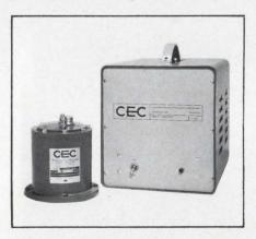
CEC's Universal Electromanometer is comprised basically of two parts: a transducer and a servo amplifier. Known as the Precision Pressure Balance, the transducer operates on the nondisplacement force-balance principle, affording accuracy and unique long-term calibration stability.
