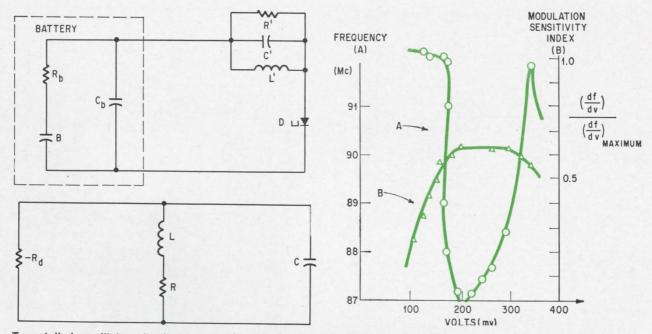
**Tunnel diode oscillator**, circuit at top, and its radio-frequency equivalent circuit. At the right, frequency and modulation-sensitivity index characteristics of a tunnel diode are plotted against voltage. For large modulation index, operating point is selected to lie in region of constant modulation sensitivity.
