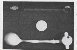
Fully assembled K-5 transmitter is connected to battery at left with twisted lead pair in tube. Lower unit is encapsulated and ready for use. Size is demonstrated by comparison with aspirin tablet in center.
