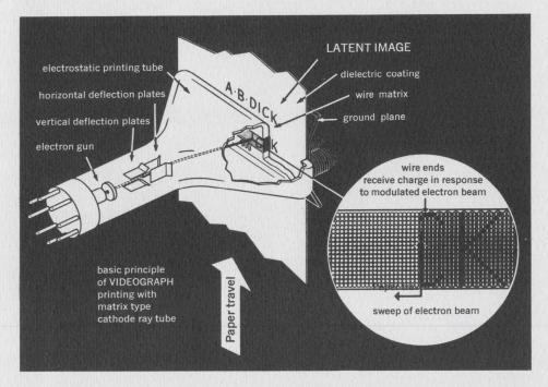
It's a well-known fact that characterproducing cathode ray tubes are playing an increasingly large role in non-impact printing systems. For example, modern CRT's are essential to data output printers on high-speed computers; they're also vital to facsimile data-transmission systems.
