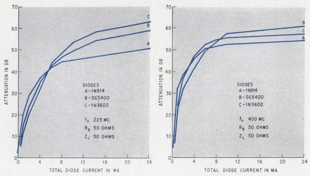
Variable attenuator versus total diode current for an operating frequency of 225 Mc (left) shows greater differences in diode current vs. attenuation than at 400 megacycles (right) among three types of diodes.
