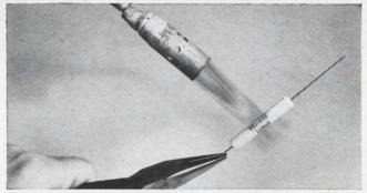
**TORCH IT!** Withstands temperatures of 1500°F without a sign of deformation. No other vitreous-enameled resistor will stand 1500°F without burning, softening, or dripping away. There's absolutely no effect on markings either.
