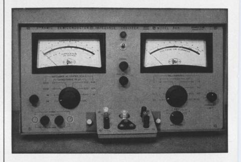
**Bootstrapped** operational amplifiers can be used in a linear bridge circuit to measure semiconductor parameters at low signal levels. An instrument named the dynamic semiconductor impedance analyzer eliminates the distortion that occurs when general purpose bridges are used with high level signals.
