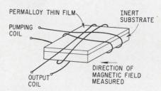
Thin-film magnetometer is built on wafer-thin substrate and measures only about a half-inch square.
