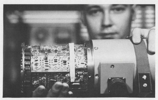
GE engineer makes final adjustments on the control circuit for a low light level camera.
