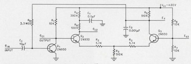
**Differential amplifier**  $Q_2$ - $Q_3$  regulates bias voltage of  $Q_1$  amplifier, which stabilizes its gain even though the load changes significantly.
