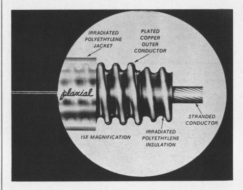
An extended helical outer conductor offers a solution to one problem that plagues small flexible coaxial cables: leakage and broken wires. The braided wires in conventional cable tend to snap when the cable is bent or twisted; and since it is hard to weave wires evenly around a small core, air holes often cause signal leakage at high frequencies.
