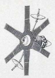
Lightning 1 is Soviet version of Early Bird. Bulblike objects on cylinder are small jets to correct orientation. Coils around cylinder are for cooling by radiation.
