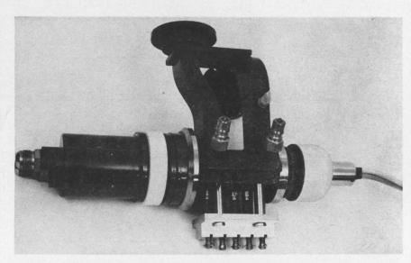
Klystron amplifier offers wide bandwidth, high gain and efficiency in a small package. The tube is 16.3 inches long and weighs only 22 pounds.
