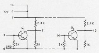
Schematic of Sixpac, showing first and last stages and pin numbers. An artist's rendering of this chip circuit made up of six logic inverters is on the cover.
