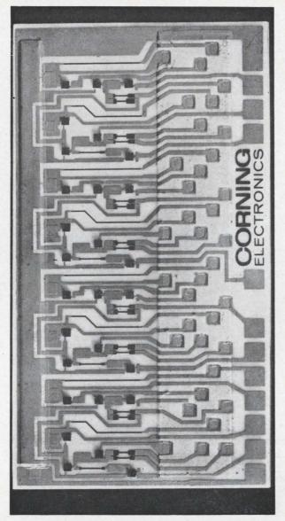
**Bonded wire leads,** generally used to connect active devices and capacitors to resistor-conductor networks, are missing from this hybrid microcircuit. The circuit has 28 face-bonded semiconductor devices (the black squares), 28 resistors (black lines), eight film capacitors (squared patterns at the left) and 102 conductor crossovers (gold stripes, invisible under a glaze, running vertically at the right). The conductors atop the glaze reach the stripes through windows in the glaze.
