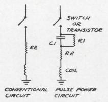
Pulse power, commonly used to operate latching relays, can also be used advantageously to operate non-latching relays, both polar and non-polar.
