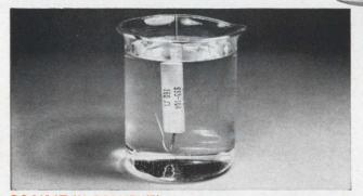
**SOAK IT IN SOLVENT!** Soak a Series 99 resistor in any organic solvent used in degreasing and flux removal. Then try to rub off the markings. You can't; they're *part* of the coating.
