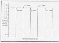
The pure mercuric oxide batteries ... identified by an "R" suffix ... have a no-load voltage of  $1.350 \pm 0.007$  volts. These are recommended where maximum voltage precision is needed. Furthermore, the no-load voltage of Mallory Mercury Batteries is extremely consistent on every production lot. The chart shows cell voltages taken from samples produced during a 5 year period.
