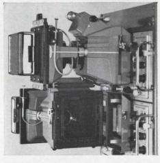
**C-27 camera** With viewing tunnels removed and carrying handles folded out of the way, the new C-27 Cameras can be stacked one atop the other—on such rack-mount oscillo-scopes as the Tektronix multi-purpose Type RM561A (upper) and split-screen storage Type RM564 (lower).
