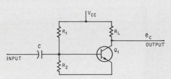
**Amplifier** uses a low-current, high-beta transistor for  $Q_{1}$ , as voltage gain that is a function of only the bias point if the supply voltage is constant.
