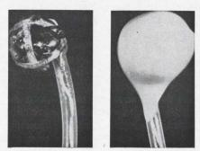
Power detector package before and after encapsulation.
