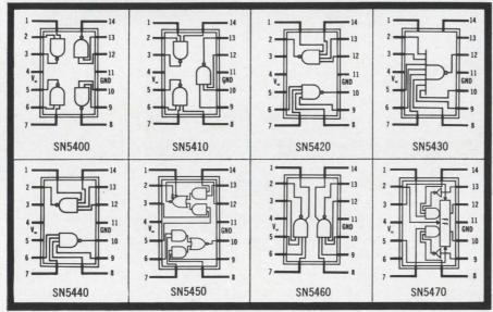
Figure 2. Logic diagrams for Series 54 TTL integrated circuits
