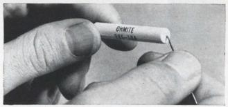
**BEND THE LEAD** at the resistor body! There's no damage. Conventional (dipped) vitreous-enameled resistors have a meniscus at this point which ruptures, damaging the coating. Series 99 (molded) have no meniscus.
