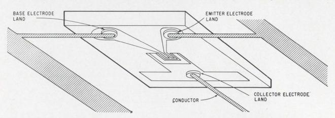
Face-bonded transistor, as it would appear if one looked up at it through a transparent substrate.
