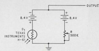
**Detector circuit** becomes unbalanced when a light from pulse waveshape displayed on scope A illuminates the photoconductor.
