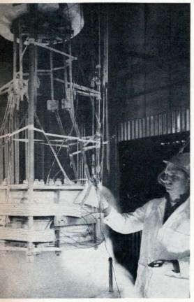
Wide-bore magnet provides elbowroom for scientists conducting research on subnuclear particles. This magnet, developed at Argonne National Laboratory, has an 11-inch bore and provides 42,000 gauss.
