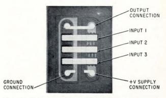
View of NOR integrated circuit shows the n-channel transistors on the left side and the p-channel units on the right.
