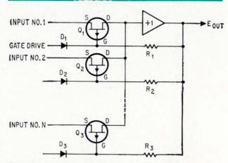
Typical commutator cricuit uses the FET switch configuration with a buffer amplifier.
