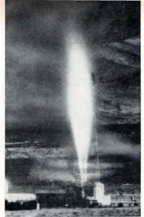
Space systems that use nuclear reactors, such as this reactor being test-fired, emit ionizing gamma rays and neutrons. Nearby circuits must be radiation-hard.
