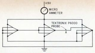
Ring oscillator using three NOR integrated circuits is an example of how the FET's can be used. Each integrated circuit has an effective fan out of three.
