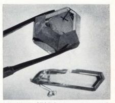
SEMICONDUCTOR. Beginning in the 1930's Bell Laboratories people carried out extensive studies of semiconductors—studies that led to the invention of the transistor. Photograph shows crystals of zinc oxide, a semiconductor with piezoelectric properties, grown at Bell Laboratories by a hydrothermal method.
