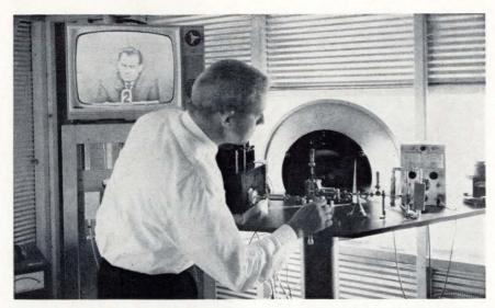
Engineer compared performance of television signals over 3-millimeter television link and f-m link in program to improve communications on small-wavelengths.
