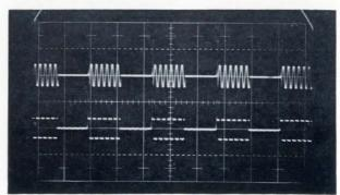
Output waveforms for a differential analog switch. the dpst module (see circuit on p. 53) receives a square wave at point A and a sine wave having the same frequency at point A'.
