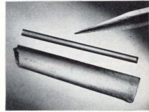
LASER MATERIAL. Among many materials developed at Bell Laboratories is nickel-doped magnesium fluoride, shown here as grown from melt and in polished rod form. Laser action in this material generates lattice phonons as well as a beam of coherent infrared photons.
