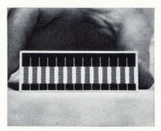
THIN-FILM RESISTORS. Tantalum thinfilm resistors (zigzag patterns above) offer new possibilities for reliable, low-cost circuits. Bell Laboratories people discovered how to fabricate films routinely with values precise to one part in five thousand, and with expected aging during a 20-year life of less than one part in a thousand.
