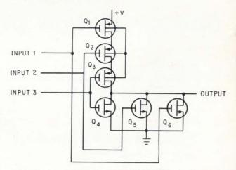
NOR circuit uses three p-channel MOS FET's ( $Q_1$ ,  $Q_2$ , and  $Q_3$ ) and three n-channel MOS FET's ( $Q_4$ ,  $Q_5$ , and  $Q_6$ ). Low dissipation of circuit during both on and off states makes it attractive for use in equipment where space and power are limited.
