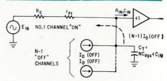
Commutator network with the first channel on and the remaining channels off.
