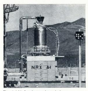
Pipe at right of nuclear reactor on test stand in Nevada contains leads attached to instruments for measuring pressures, temperatures and vibrations. Reactor controls are in building under the reactor.
