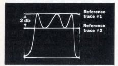
Typical network rf loss displayed with minimum and maximum references by Jerrold 890 Sweep Generator and TC-3 Solid-State Coaxial Three-Way Switcher.
