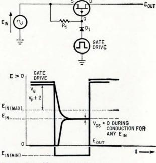
This circuit provides a zero gate-to-source voltage for any input signal. Positive gate (see waveform) turns the switch off.
