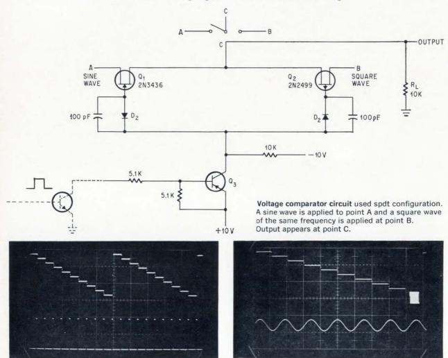
Upper trace shows two frames of a staircase waveform applied to the 10 input positions of an experimental 10-channel commutator built with spst modules. The lower trace shows the voltage applied to the logic units.
