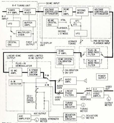
TR-711, with heavy line representing signal going through receiver
