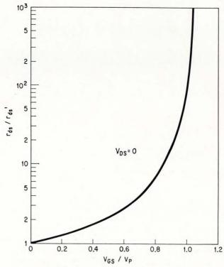
$V_{P}$  = VALUE OF  $V_{GS}$  WHEN  $~I_{D}~/~I_{DSS}$  = 0.001  $r_{ds}$  = VALUE OF  $~r_{ds}$  WHEN  $V_{GS}$  = 0
