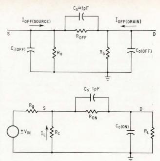
Switch in the on condition (FET<sub>2</sub> conducting) is represented by lower circuit. Upper circuit applies for the off condition ( $Q_{\rm FET}$  not conducting).
