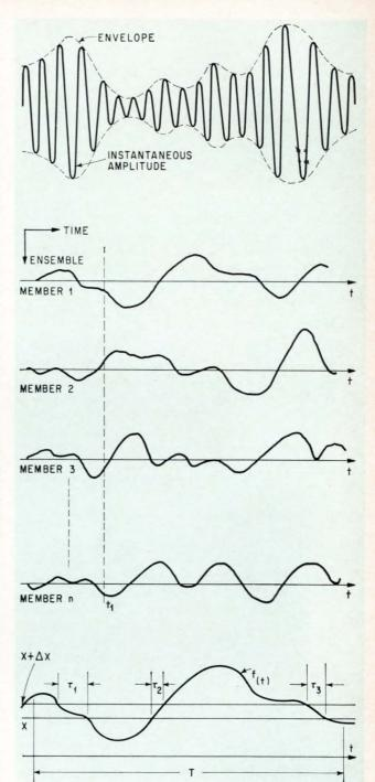
**Definitions:** noise-modulated carrier (top) demonstrates the different between envelope and instantaneous amplitude; measurements of the random waveforms (center) could be taken from each waveform as a function of time (time statistics) or taken at one instant over the ensemble (ensemble statistics); coordinate system (bottom) for the probability density function.
