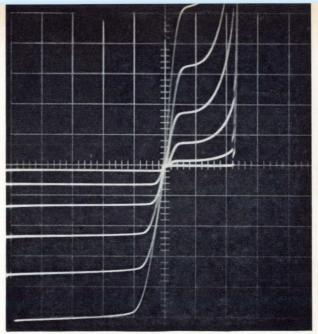
Set of oscilloscope traces shows drain characteristics for one n-channel unit and three p-channel units in series in the NOR circuit. The upper traces are for the n-channel unit. The highest trace is for a  $V_{\rm G8}$  of +9 volts; the lowest trace is for a  $V_{\rm G8}$  of -9 volts. Each vertical division (y-axis) represents 0.2 milliamperes. Each horizontal division is 5 volts. One-volt gate steps were used.
