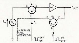
An alternate version of the series switch with a buffer amplifier. A bipolar transistor,  $Q_2$  is used instead of a turn-on resistor in this circuit.
