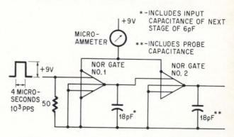
Circuit arrangement for measurement of propagation delay and power consumption for a pair of NOR integrated circuits. The simulated fan out for each NOR circuit is three.
