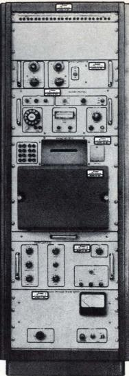
This precision, high-speed Interstate VIDEOSCAN combines images from a high-resolution cathode ray tube with galvanometer traces onto single, moving 12-inch film or paper... providing a detailed, permanent recording for data analysis that up to now was impossible.
