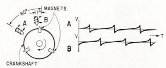
First step in controlling ignition firing time. Equally spaced magnets on crankshaft rotating at engine speed, induce voltage in trigger coils A and B.
