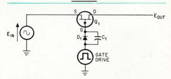
Capacitance-coupled series switch is used for systems with fixed sampling rates.
