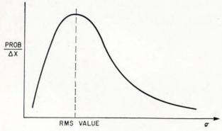
Rayleigh probability density function represents the envelope of Gaussian noise measured at the output of a linear detector.
