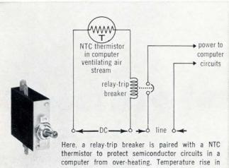
ventilating air will drop thermistor resistance, raise breaker coil voltage, and cause instantaneous tripping. Breaker contacts open power lines to semiconductor circuits, prevent burnout. Design was chosen as the most economical means of providing high-temperature cutoff with manual reset.
