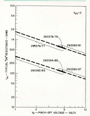
Relationship of pinch-off voltage to on resistance for various junction FETs.
