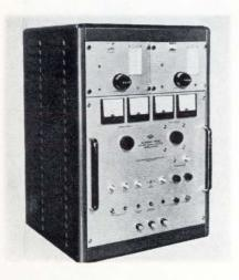
Plug-in heads permit frequency coverage from 100 to 6,000 Mc with excellent resolution. Pulse widths are available from 0.1 to 25 μsec. The completely self-contained instrument includes many metering, monitoring and safety features. Applied Microwave Laboratory, Inc., 106 Albion St., Wakefield, Mass. [425]
