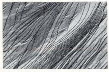
INSULATOR. Electron microscope photograph of polyethylene, 9800 diameters magnification, showing overlapping ribbon-like crystals, a structure characteristic of many polymers. At Bell Laboratories, studies of the formation of such groups of crystals have contributed to an understanding of the electrical and mechanical properties of these materials.
