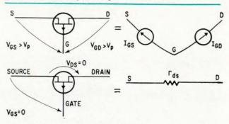
On and off equivalent circuits. In the on condition, there is no offset voltage and the switch may be represented as a resistor.
