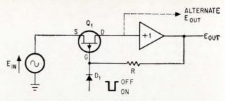
Series switch with a buffer amplifier. The unity-gain buffer amplifier provides complete isolation between the channels and the gate-driving voltage. As indicated by the alternate connection shown, the output signal may be taken at a point before the buffer amplifier as well as after it.
