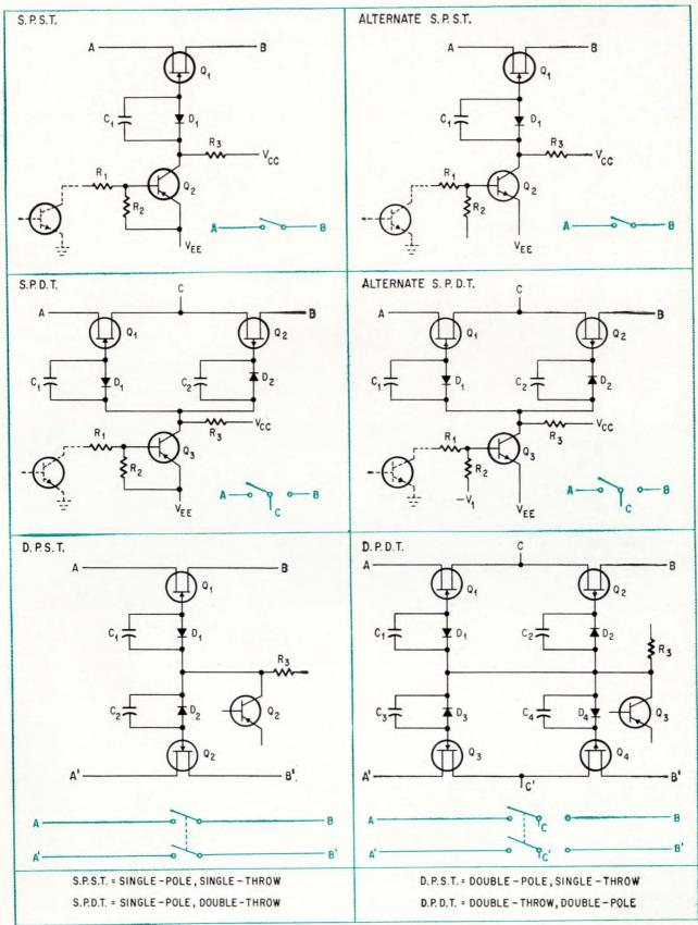
Modular analog switches allow compact design of complex switching functions. The four basic building blocks and two alternate versions are shown. The two alternate-version switching circuits substitute an npn transistor for the pnp transistor.
