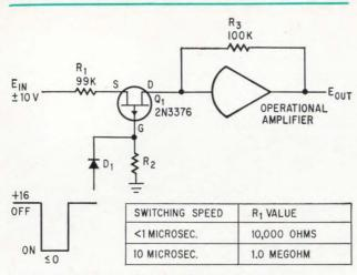
Analog gate circuit uses a 2N3376 junction FET. This transistor has a  $V_{\rm P}$  of 2 volts, an  $r_{\rm ds}$  of 1000 ohms and an  $I_{\rm D_0off)}$  of less than 0.4 nanoamperes. Output of gate is -10.0025 volts for an input of +10 volts and +9.9975 volts for an input of -10 volts.
