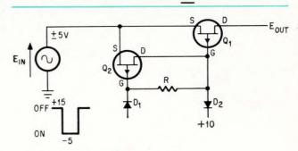
Instead of a turn-on resistor, this circuit employs another field-effect transistor, Q<sub>2</sub>. Transistor Q<sub>2</sub> prevents excess current from being injected into the signal path.
