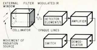
**Detector** mounts inside the pole of parking meter. Filter eliminates false triggering.
