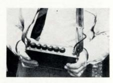
**Command box** weighs only  $51/_2$  pounds, yet controls a 100-ton train engine. New model will have control buttons on front instead of top.
