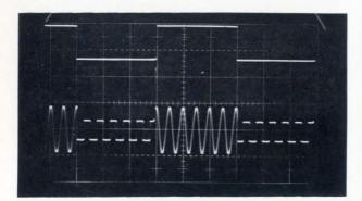
Upper trace represents the output waveform for the voltage comparator. Lower trace shows the control inverted waveform. The scales are: vertical, one volt per centimeter; horizontal, 20 microseconds per centimeter.
