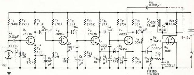
Amplifier follows receiver optics. Silicon npn transistors are used in each stage in straightforward design. Relay resets meter to zero.
