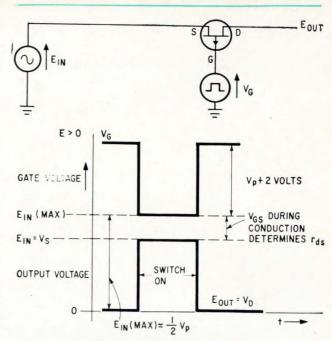
Simple series FET switching circuit and associated waveforms. The input signal is supplied to the source. The output signal is delivered to the bus bar.
