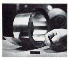
MAGNETIC MATERIAL. Remendur, latest member of a large family of high-performance magnetic materials developed at Bell Laboratories, is shown here in sheet form and as element of new telephone switch. A malleable, ductile cobalt-iron-vanadium alloy, Remendur has a remanence of 21,500 gauss.
