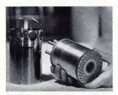
SUPERCONDUCTOR. Experimental 75 kilogauss superconducting solenoid. Wire consisting of compacted niobium and tin in a niobium jacket is wound and later heated to form niobium-tin compound (Nb<sub>3</sub>Sn), which has a transition temperature of 18° Kelvin and a critical field greater than 200 kilogauss. Compound and wireforming technique were developed at Bell Laboratories.
