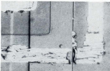
Fig. 7 An open at a scratch over an oxide step, caused by aluminum melting
