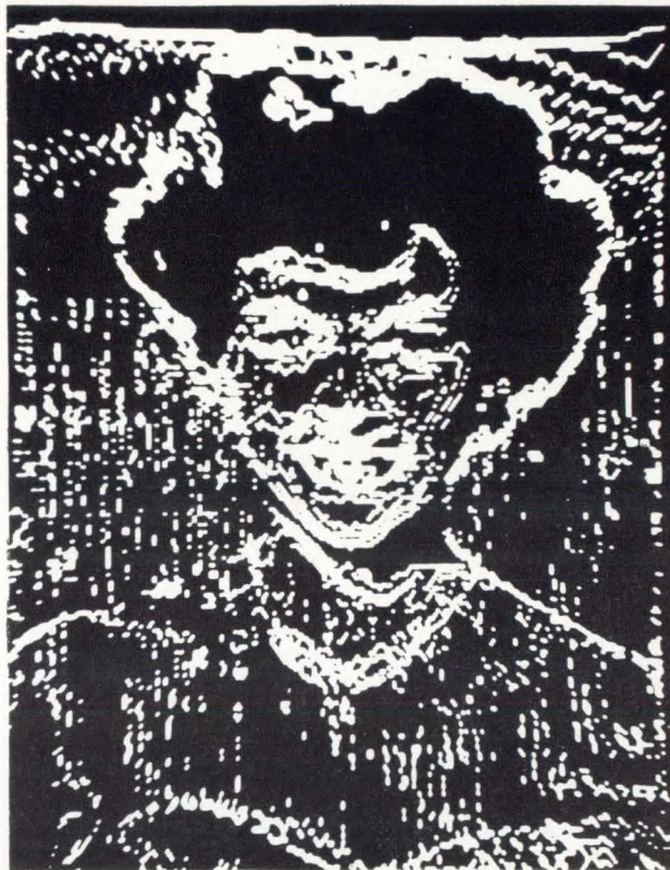
Each white dot in the picture at the right represents a picture element from the original (left) that is unlike its previous neighboring element. The black areas indicate the amount of picture redundancy.
