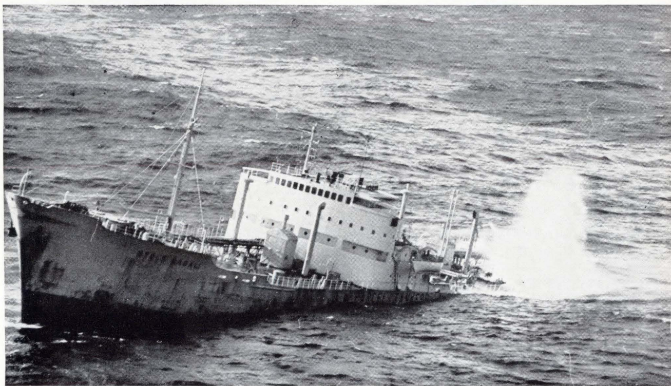
Norwegian tanker Stolt Dagali flounders off New Jersey after being split in two by the Israeli liner Shalom . The collision occurred in fog and heavy seas. The Shalom's captain said his radar was operating.
