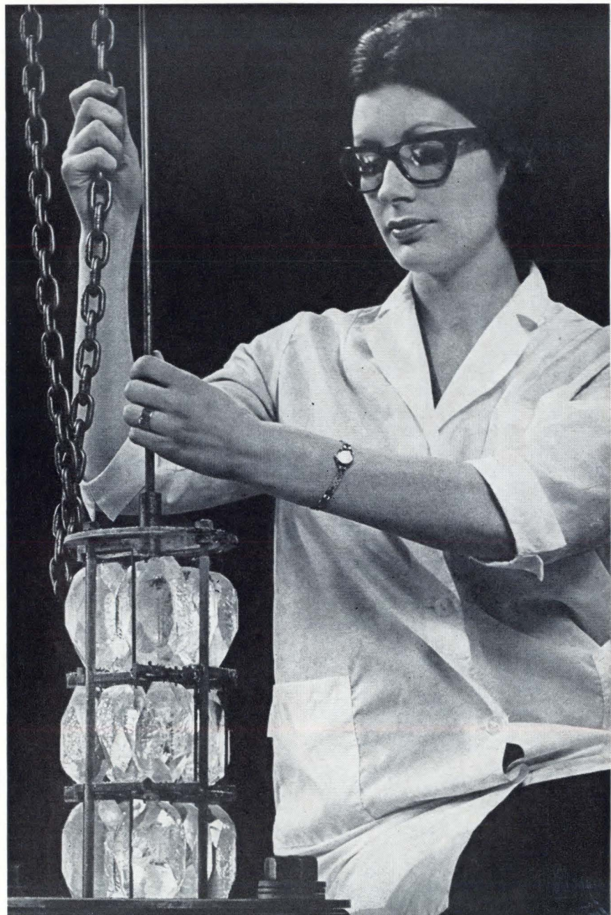
Homemade quartz, in one-pound slabs, comes out of pressure chamber.
