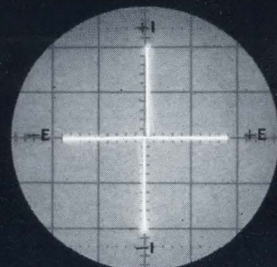
Oscilloscope trace showing E-I characteristic of the OVONIC threshold switch. Note instantaneous change from non-conductive state to the fully conductive state.
