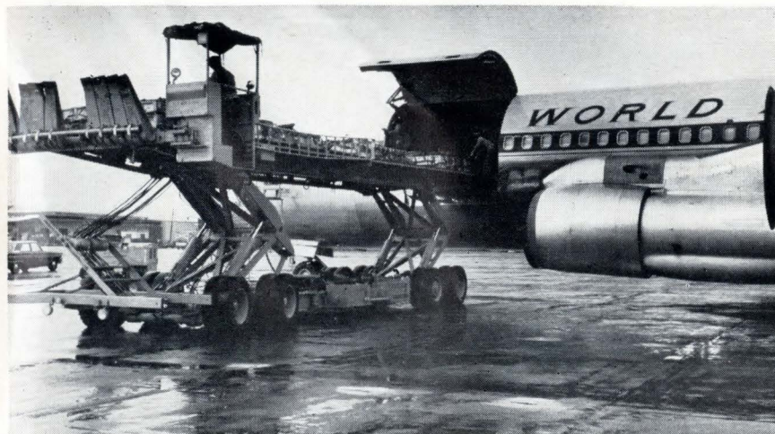
As the aircraft is loaded, the weight and center of gravity are automatically registered on meters in the cockpit
