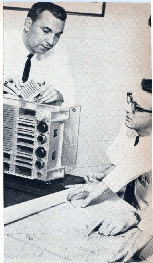
Saturn V computer is about the size of a two-suiter. It contains 80,000 components.
