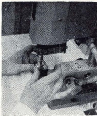
Dicing silicon wafer into individual transistor chips is accomplished with a pantograph cutting machine.
