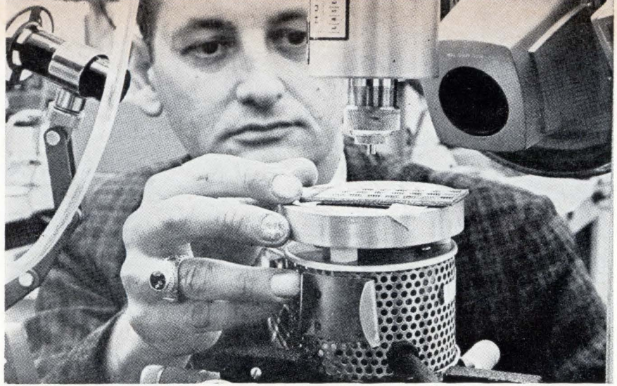
Most aerospace electronics companies are experimenting with laser welding for microcircuit assembly. This test setup at the Autonetics division of North American Aviation, Inc., uses a laser made by Hughes Aircraft Co.
