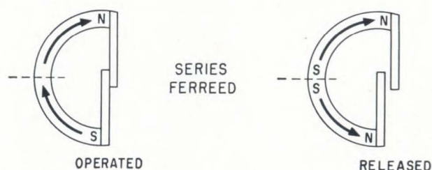
When magnetic windings aid, the ferreed switch is closed; a pulse that energizes windings in opposition releases the contacts.
