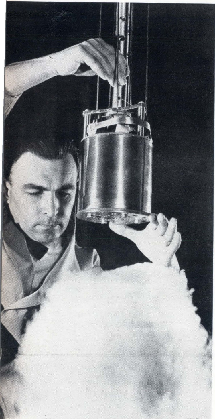
107,000-gauss superconducting magnet developed at the Radio Corp. of America's research center uses 15,370 turns of Nb 3 Sn thin-film ribbon in a compound structure (coil within coil within coil), stores 20,500 joules of energy at full field strength.
