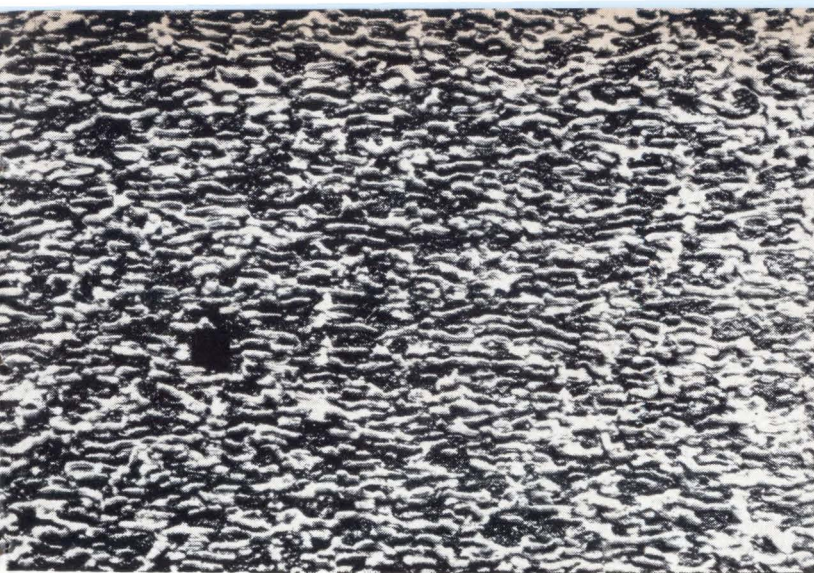
Metallurgical structure of Alnico, left, contains elongated single-domain regions developed by aging the alloy in a magnetic field, whereas Lodex, a synthetic structure,
