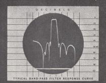
This extremely accurate log amplifier enables exact measurements of attenuation in networks, filters, amplifiers, and other devices exhibiting dynamic operating ranges down to 90 db. Write for complete technical data.
