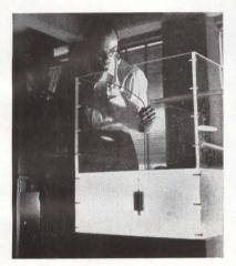
PINPOINTING UNDERWATER temperatures accurately is important in submarine sonar systems, since the speed of sound is affected by temperature. New transducer determines temperature to within 0.05 deg F
