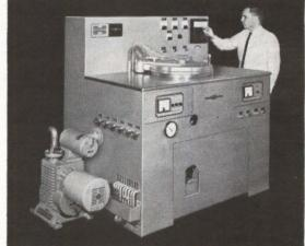
**Speeds up & upgrades brazing & hardening processes!** Model VCT, the newest Hayes Vacu-Master® Furnace, out-performs metal element furnaces for processing work in vacuums from several hundred microns down to 10<sup>-6</sup> Torr, at temperatures from ambient to 2000°C (3632°F).
