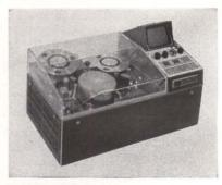
MINIATURE video recorder uses micro-tv set for monitoring. Set, built by Victor Co. of Japan, is for nonbroadcast applications and records 64 minutes on 1,800 feet of 1-inch tape by the two-head method
