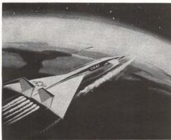
FLYING AT 2,000 mph at an altitude of 70,000 feet, the RS-70 would assess damage done by ICBM's to enemy and seek targets. The first RS-70 will fly this spring on airframe tests
