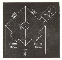
BRIDGE CIRCUIT of rat's nest calorimeter—Fig. 1
