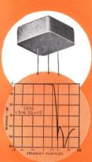
Miniaturized 3.5 KC low pass filter. 10K ohms to 10K ohms. Within 1 db up to 3500 cycles. Greater than 40 db beyond 4800 cycles.
