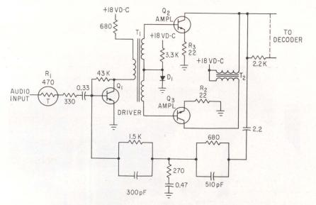
DECODER DRIVE unit accepts audio signals from receiver, amplifies them and drives 20 parallel decoders—Fig. 3
