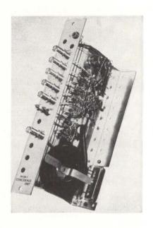
figuration at 100 Mc, output pulse is nominal 5 ma negative, 5 nsec wide and double clipped for automatic base line restoration. All inputs are at least 5 ma negative with 1 nsec extra overlap required for the *no* input. Except for power busses, printed circuits are not used because of special technique required for low-inductance grounds.
