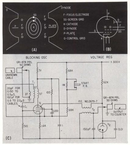
PHYSICAL LAYOUT of secondary emission tube (A) and schematic representation of same tube (B); secondary emission tube in 10-nanosecond pulse generator, (C), with each reflected pulse causing the circuit to emit a fresh output—Fig. 1
