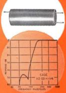
High frequency Minifilters, .33 oz. MIL-T-27A Grade 5. 150 KC High Pass 3 db to 150 KC, down 45 db below 85 KC, 7500 ohms.
