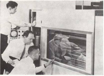
MASS STORAGE system announced by Univac can store 64.9 million characters of information and deliver them in 92 µsec. It has two drums rotating at 870 rpm and searched by 54 flying heads. Theoretically, 96 of these units can be used with a Univac 490 computer
