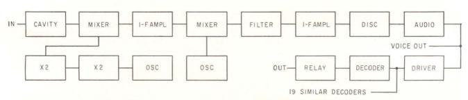
COMMAND receiver is a double-conversion f-m superheterodyne with both local oscillators crystal controlled. The audio amplifier drives 20 similar decoders and also is an emergency voice channel—Fig. 1
