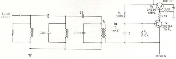
THERE ARE 20 similar decoders in the system, each tuned to its particular frequency and operating its own relay—Fig. 4
