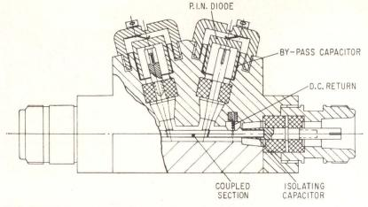
EXPERIMENTAL microwave modulator from Mullard for 3 to 7 Ge has peak isolation of 30 db at 5 Ge  $\,$
