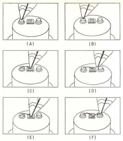
WIRE breaks right next to bond because of machine-tool motion and clamping action. Machine operates at high speed with most bonding variables under its control rather than operator's—Fig. 2
