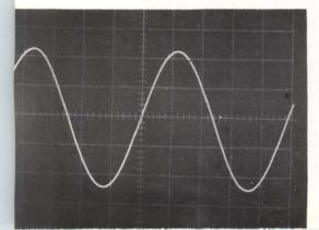
Extensive negative feedback is used in this circuit both to minimize the effects of the unstable transistor characteristics and to make the oscillator independent of load variations. With this feedback the amplifier gain mainly depends on stable resistors. The result is low distortion and excellent amplitude and frequency stability.
