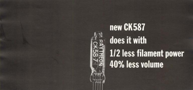
Newest addition to Raytheon's line of subminiature electrometer tubes is the CK587. The CK587 is small in size (.230" x .290" x 1"), requires the lowest input power of any electrometer tube available (.00625 watts), and stands up under rugged service with reduced filament resonance effects by virtue of its shorter structure. Compared with the CK5886 under similar gain conditions, the CK587 requires 1/2 less filament power and is over 40% smaller in volume.
