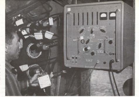
COAX CABLE delay determines oscillator frequency. Engineer reads off frequency from digital meter
