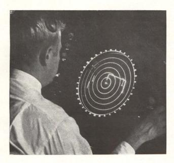
CRYSTAL BALL. Our lead feature article this week (p 27) is an exclusive report on a new traffic control system that is the electronic equivalent of a crystal ball. It shows the controller where planes circling the airport will be in the next several minutes. By looking at this radar view of the future, he can detect when planes are on convergent flight paths and avert a possible disaster.
