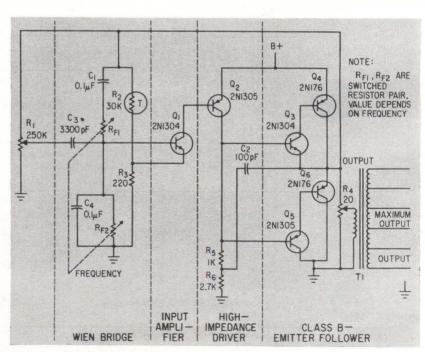
COMPLETE CIRCUIT diagram of the oscillator-amplifier; the negative feedback path goes from the output, to thermistor  $R_z$  and resistor  $R_s$ —Fig. 2
