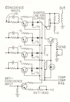
diodes turn off, signifying pulse coincidence, the tunnel diode will switch to the high-voltage state for duration of pulse coincidence, thus delivering an output. When any input is not connected, corresponding buffer transistor current is cut off so that input is effectively out of the circuit. This allows the number of connected inputs to determine the coincidence configuration. The circuit will handle coincidence con-
