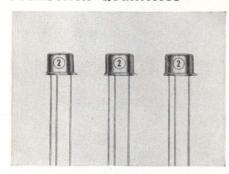
High speed Silicon Precision Alloy Transistors specifically designed for use as low-level choppers and developed by the Sprague Electric Company are now available in a broad range of types and performance characteristics.
