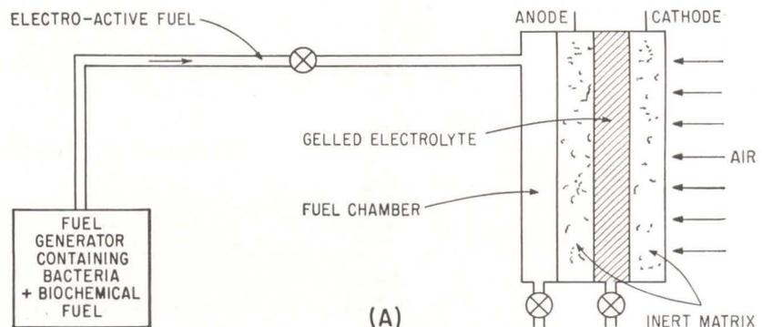
*Conceptual drawings of indirect (A) and direct (B, on facing page) cells*
