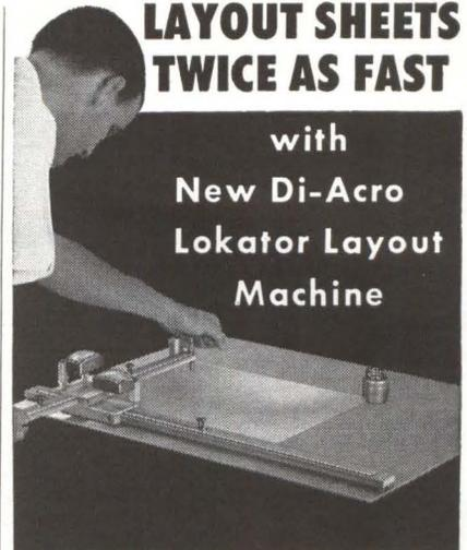
Here's a fast low cost method for laying out sheets and plates without individual use of squares, scribes, scales, punches and hammers. New sliding secondary scales on the primary transverse and longitudinal scales permit direct reading of all locations whether dimensioned from material edges or from each other.
