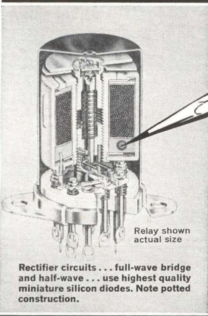
Rectifier circuits . . . full-wave bridge and half-wave . . . use highest quality miniature silicon diodes. Note potted construction.
