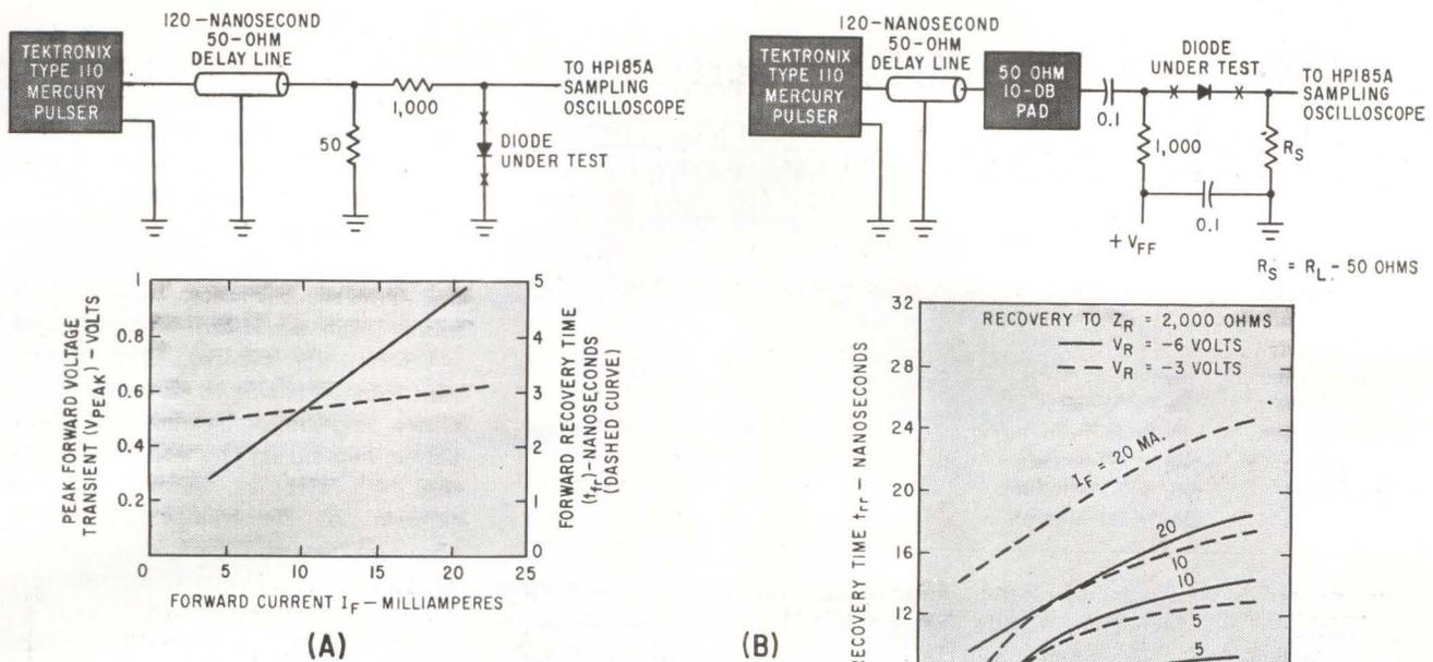
FIG. 3—Typical recovery characteristics for the 3DG001 and 2DG001 diodes: forward recovery time, (A), reverse recovery time, (B)
