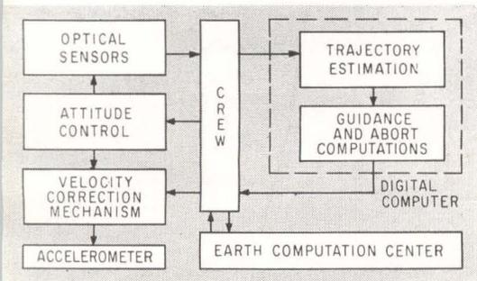
*Velocity correction system is directed by the crew. Earth-based computing facility backs up on-board system*
