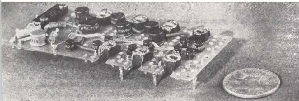
Timer-programmer designed for satellite application uses incrementally magnetized cores. Reliability is excellent
