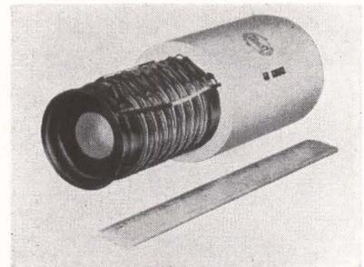
Magnetically focused image intensifier with encapsulation partially sectioned
