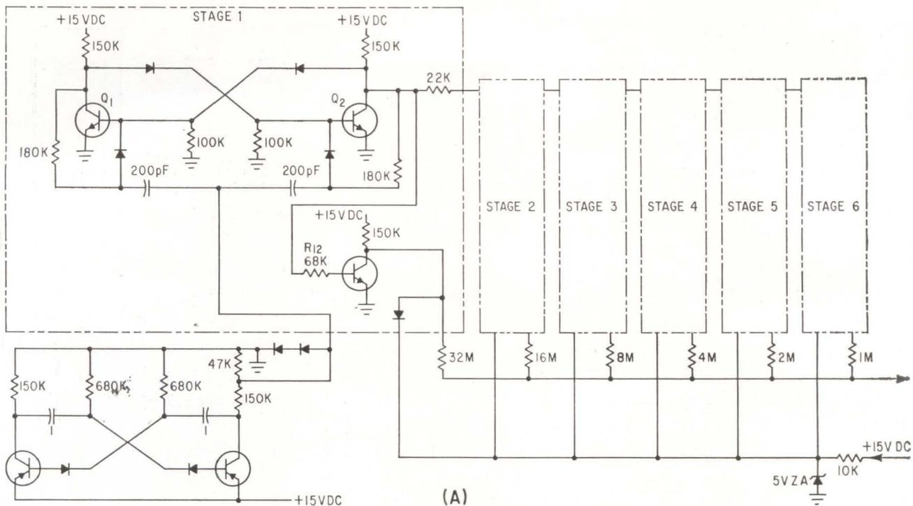
FIG. 1—Original circuit of the staircase generator before modification for thin-film construction (A), and modified
