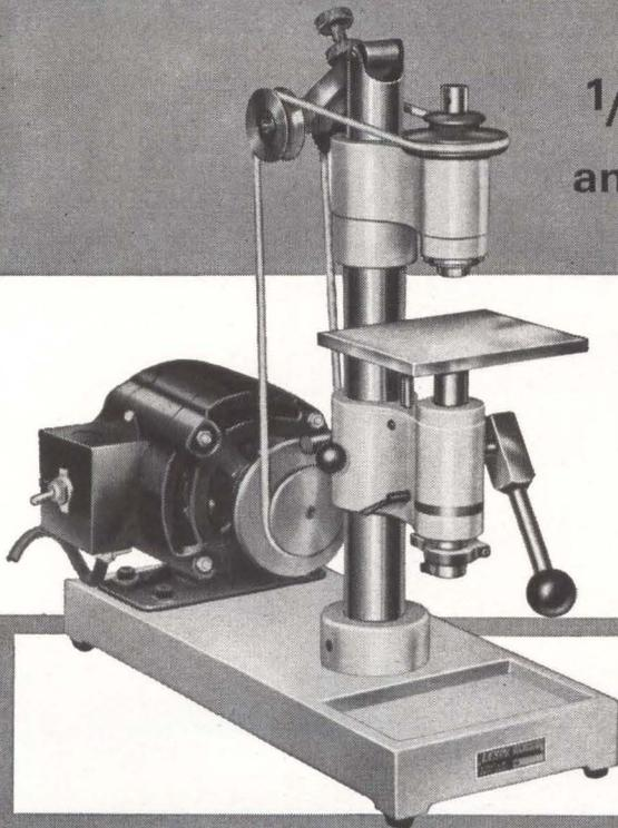
**LEVIN**® MICRO DRILL PRESSES are *sensitive* because there are no sliding quills and splines to cause drag. They are *accurate* because the precision preloaded ball bearing spindle is made to hold Levin WW Style Collets. For drilling holes from 1/8th inch down to 1/1000 inch and smaller look to Levin for the finest in Micro-Drilling equipment.
