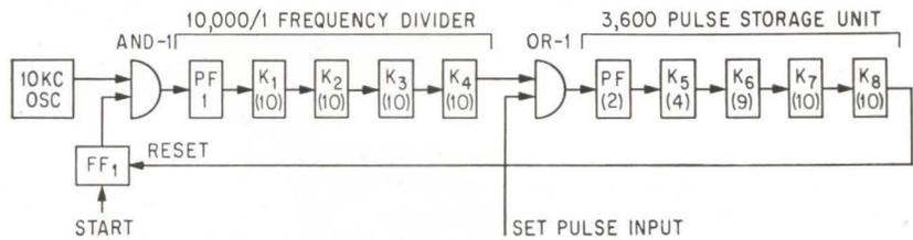
FIG. 3—Divider chain delivers output pulse after preset number of seconds when driven by 10 Kc oscillator. Storage unit is partly filled (saturated) before counting; delivers output when last stage reaches saturation. Information may be stored for days without deterioration
