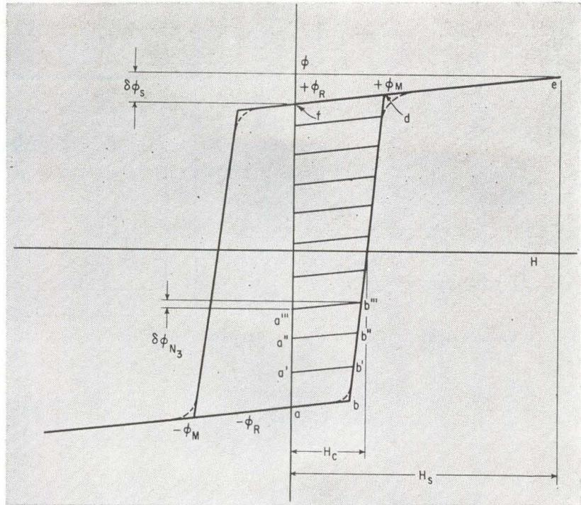
FIG. 2—Hysteresis loop shows this core is saturated by tenth input pulse. For given core, external circuit resistance and other parameters are adjusted to insure correct count. Adjustable counting is available with some cores; maximum count is 16
