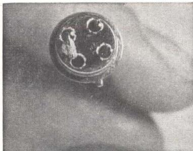
*Transistor lead is grounded to header*
