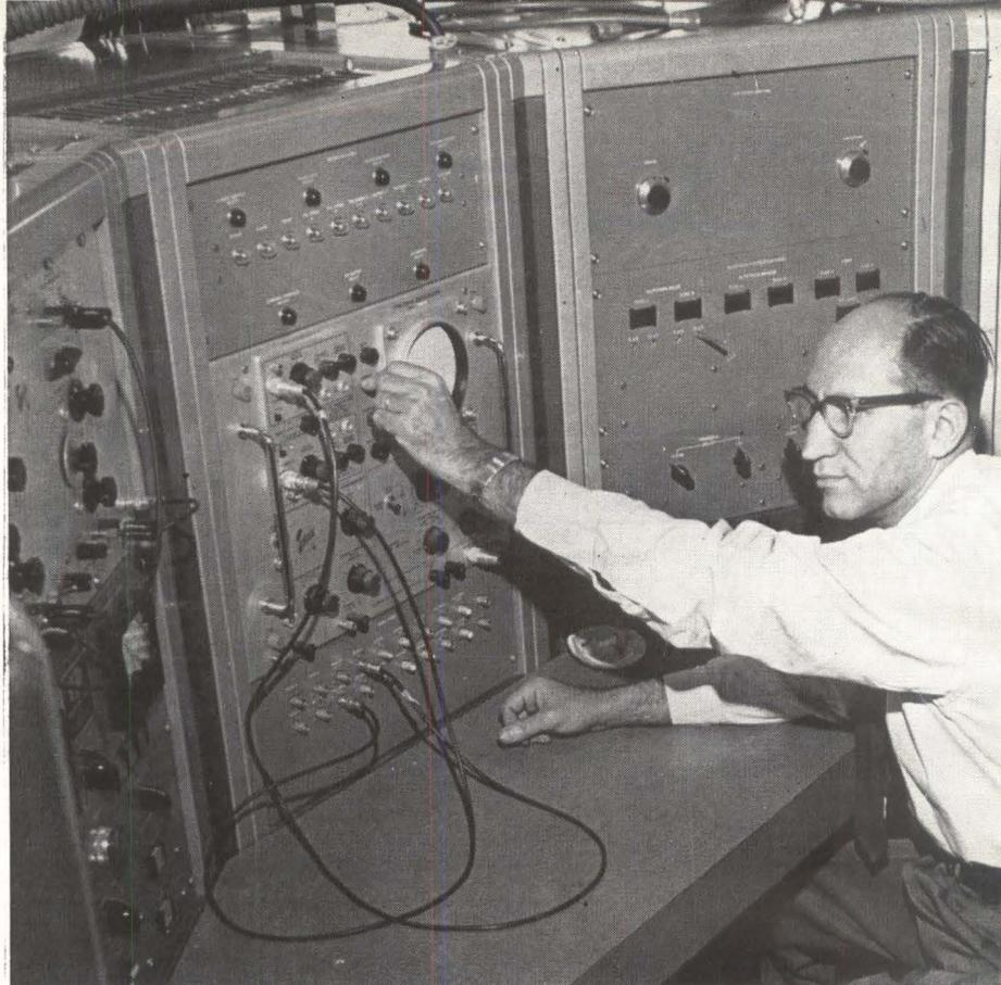
*Prof. Saul W. Rosenthal, Polytechnic Institute of Brooklyn, at the control console of the high-power klystron C-band amplifier at which all operating, monitoring and control functions are located*
