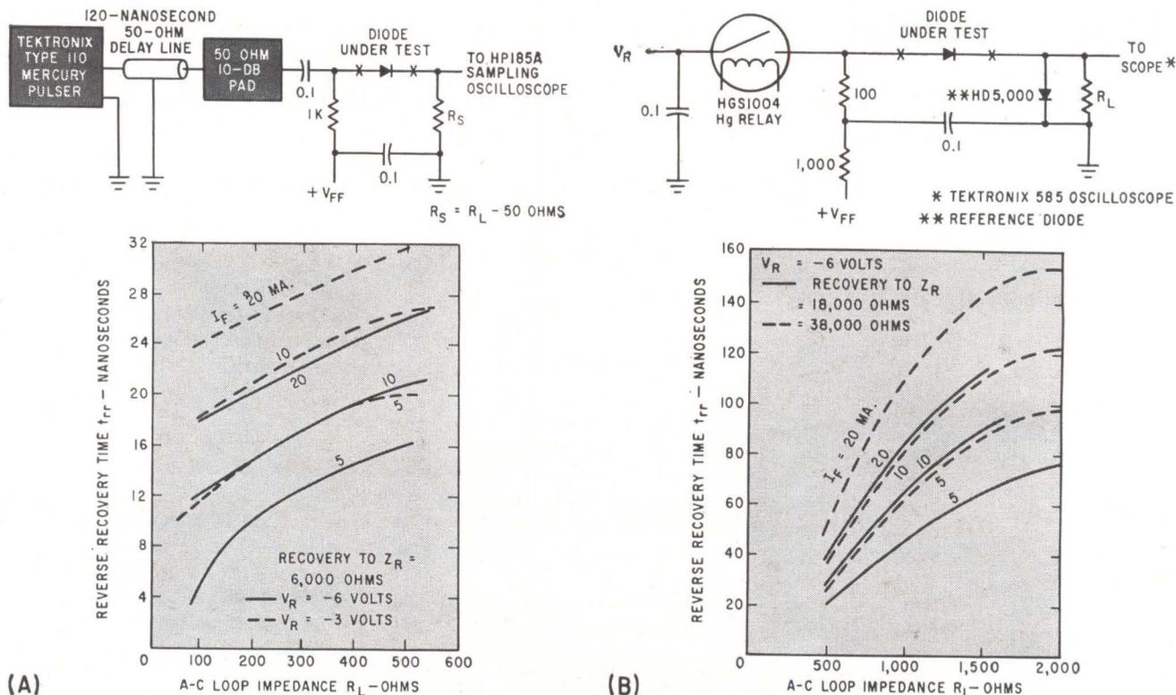
FIG. 4—Reverse recovery characteristics for 3DG001 and 2DG001 diodes, with different circuit parameters
