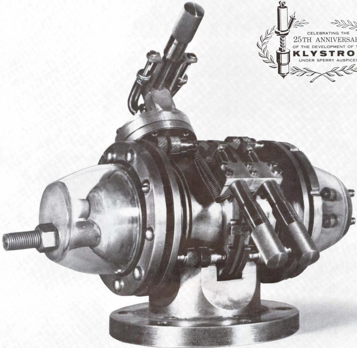
Early klystrons delivered only 5 to 10 W across a relatively narrow bandwidth. Today's Sperry klystron family blankets the spectrum at outputs from milliwatts to megawatts.
