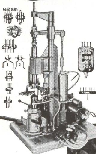
At left: No. 105-BST1 Single position Button Stem and Wafer making machine—Fully automatic. Designed for small production runs on special tube parts or for laboratory use. Produces button stems up to 1/4" diameter. Machine can be supplied with up to 24 positions.
