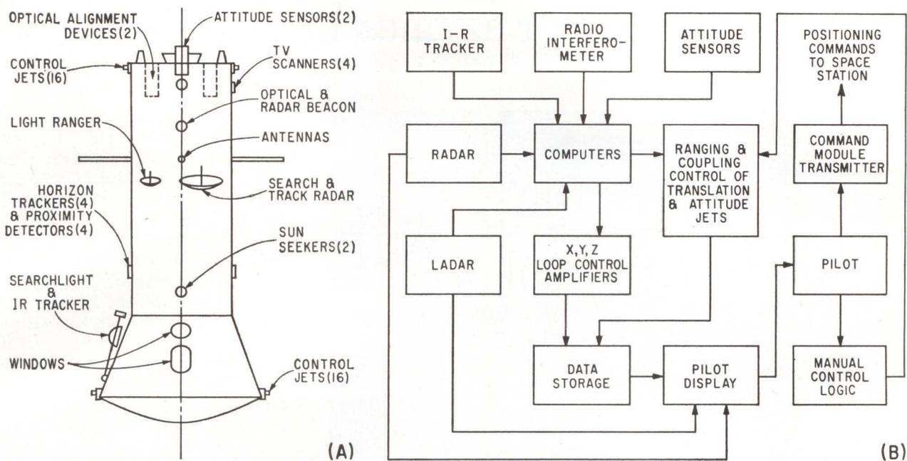
Space rendezvous homing and docking system proposed by Northrop. Sensors on manned capsule (A) would provide data for automatic and pilot control systems (B)
