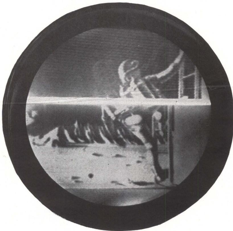
*Man-on-moon rehearsal is simulated view of what a tv camera on the moon would send, by narrow band transmission, back to storage tube displays on earth. Advantage of new multi-mode tubes in this application is that persistence and rate of image display can be controlled. Lower part of photo was stored from previous scan*
