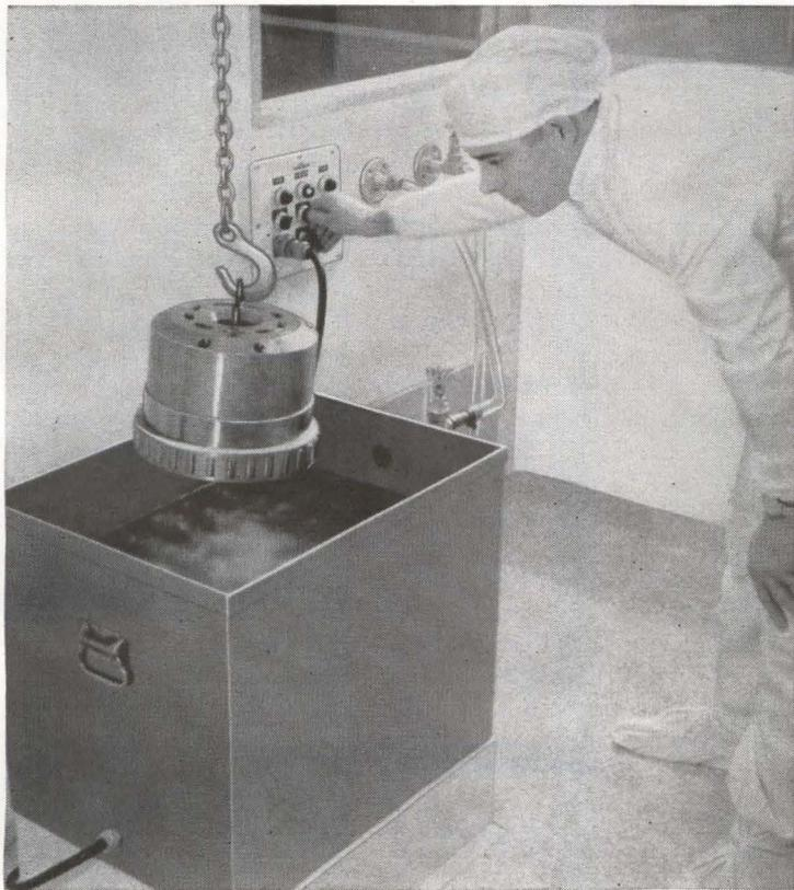
**PROBLEM:** Denison Engineering Div., American Brake Shoe Co., needed reliable precision-cleaning of metal hydraulic components for missile-ground-support equipment they manufacture. Clearances down to .0002 in. had to be maintained, yet cleaned. A familiar situation . . . except that these components weigh up to 180 lbs.!
