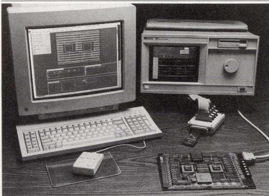
**FAST PROTOTYPING** for pc-board and ASIC applications is promised by Aptix's development system for the field-programmable interconnect component. The FPIC/D device, with its on-chip 64-channel diagnostic port, is easily linked to logic analyzers for rapid debugging.
