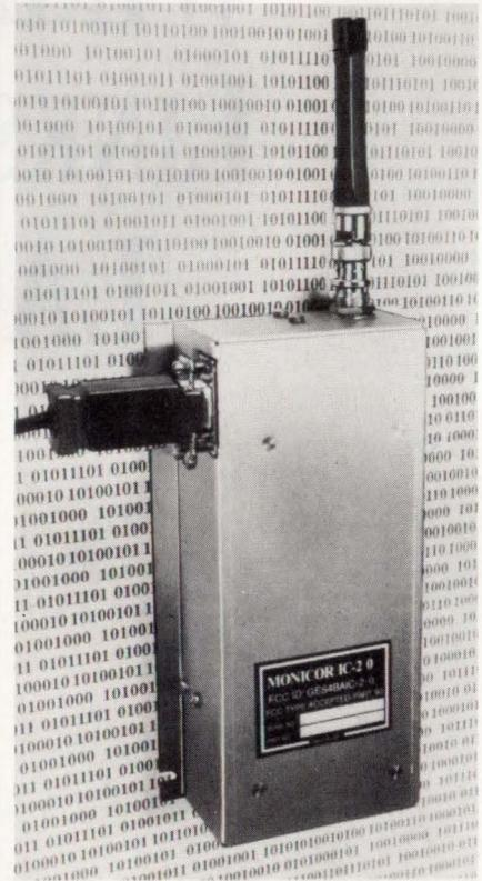
**2. THE IC-20** radio modem from Monicor uses narrowband transmission for two-way data transfer. Designed for use in large warehouses and process-control facilities, the battery-operated handheld unit has a maximum line-of-sight range of 75 miles. It can act as a base station or a mobile station.
