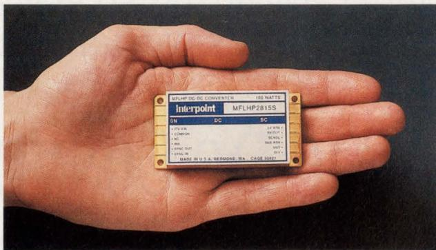
**1. OCCUPYING LESS** than 1.5 in.<sup>2</sup>, the MFLHP dc-dc converter from Interpoint is the first board-mounted unit with a rating that exceeds 50 W/in.<sup>2</sup>. The converter owes its density, to among other things, a fundamentally new control system designed to minimize transformer losses.
