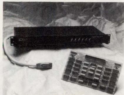
puts or outputs in 8-bit multiples. Each 40-line channel has six handshake lines: trigger, data strobe, inhibit, clear output, service request, and external data ready. An optional HVCX1 daughter board allows each port to control 200-mA open-collector drivers. The option also makes the interface compatible with 12-, 24-, and 48-V logic when the unit is used with non-TTL devices. The Digital488/80A costs \$995 and the
