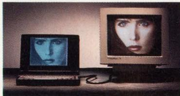
*The CL-GD6410: the first VGA controller with SimulSCAN. Simultaneously drives both LCD and CRT displays for your presentations, demos and seminars.*
