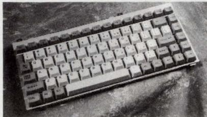
The long waits and high costs for custom notebook-computer keyboards can be sidestepped by using the FKB7200 series keyboards. The standard keyboards with a low profile and membrane keyboard were developed with input from major OEM customers. The unit measures 11.56 in. long by 5.02 in. wide by 0.59 in. high and weighs about 9 oz. Keystroke travel is a full 3 mm with quiet tactile feedback. Pricing is \$21 in lots of 5000. Delivery is from stock.
