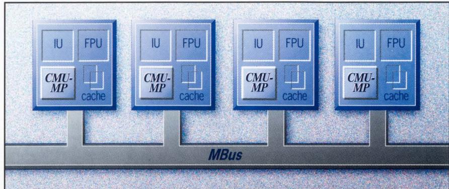
*SPARC multiprocessing is now enabled. Now you can design-in multiple high-performance SPARC chipsets. Our revolutionary Multiprocessing Cache Controller and Memory Management Unit (CMU-MP/CY7C605) provides memory management facilities and a unique cache architecture for higher performance. Our complete SPARC chipset solution shortens your time to market.*
