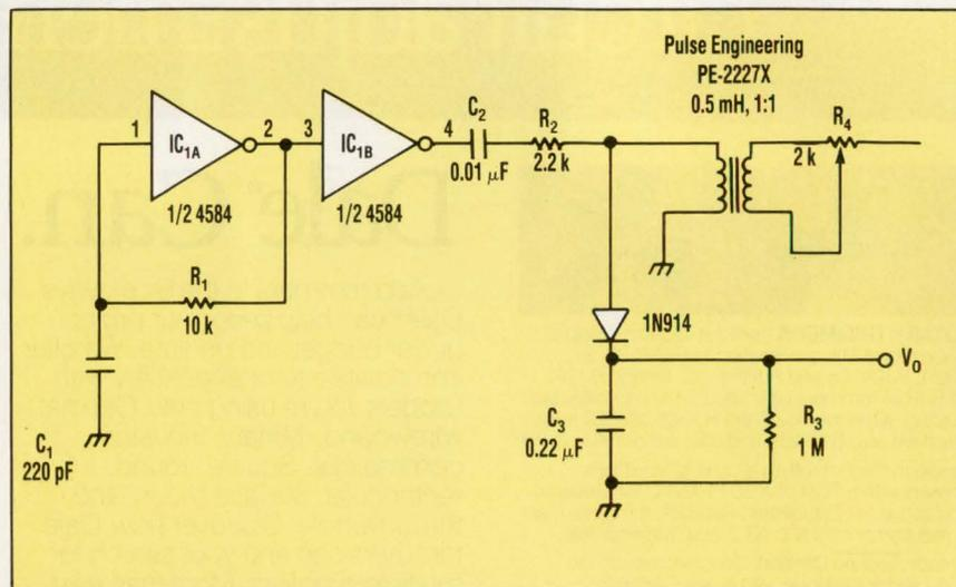
**NO ACTIVE COMPONENTS** are required on the far side of the isolation barrier with this monitor circuit. The monitored resistance, R<sub>4</sub>, loads down the voltage at the output end of R<sub>2</sub> despite the interposed transformer. □
