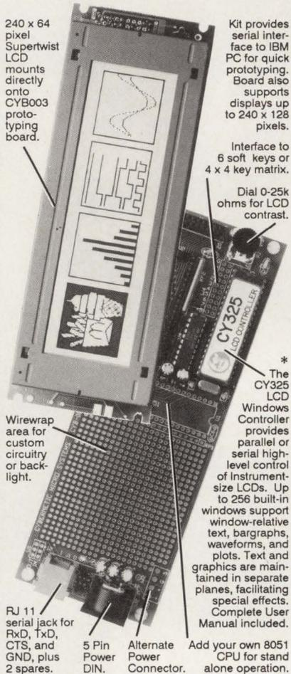
Kit provides serial interface to IBM PC for quick prototyping. Board also supports displays up to 240 x 128 pixels.
