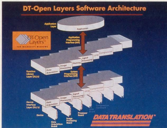
which are hardware independent. It contains the protocols for allocating devices in terms of whether the device is being used by a particular library or application. For example, if an FFT board is being im-
