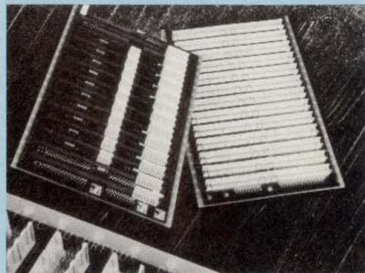
0-V rails is supplied to the backplane through the company's LOMET connector, which offers a low-impedance interconnect to the multiple power and ground planes. The backplane costs about \$2000.
