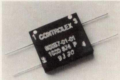
winding geometry and a high flux-density core, the transformers support 2500 V/ $\mu$ s voltage changes while delivering rise times of under 100 ns. Applications are in dc-ac inverters, ac-power controllers, pulse-width modulators, and high-frequency power transformation. Typical pricing is in the \$25 range for OEM lots. Delivery is from stock to 60 days.
