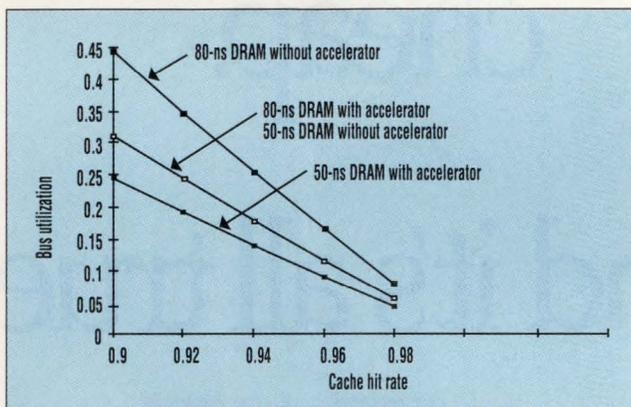
**2. IN A TYPICAL**, simple RISC-based system that only uses an on-chip cache and external DRAM, bus utilization changes considerably as the cache hit rate increases. Four cases are shown in the graph: using 80- and 50-ns DRAMs with and without the accelerator module. Matching performance can be achieved using the accelerator with 80-ns DRAMs or 50-ns DRAMs without the accelerator. The smallest bus utilization percentage is achieved using 50-ns DRAMs and the accelerator module.
