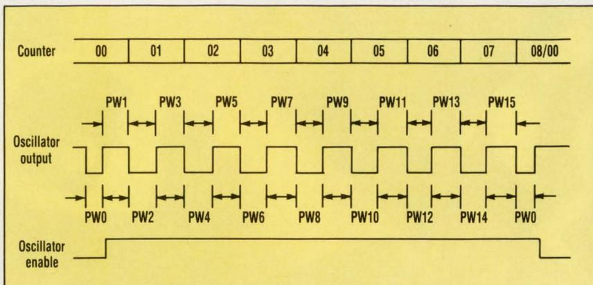
**2. THE OUTPUT PULSE TRAIN** consists of 16 consecutive pulse widths, 15 being proportional to the temperature of an individual sensor. The exception is the first pulse, designated PW0, which is distinguished by its narrowness. It serves as the synchronizing pulse to indicate the start of the train.
