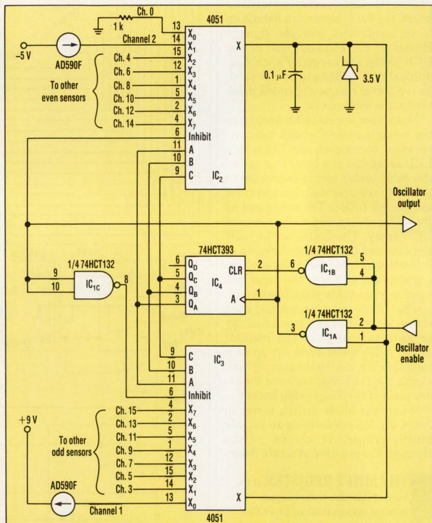
**1. THE EVEN-NUMBERED** channels in this multiplexed temperature-sensing circuit are connected to IC<sub>2</sub>, where they form the lower half of the output pulse train (see figure 2). The odd-numbered channels, connected to IC<sub>3</sub>, make up the other half.
