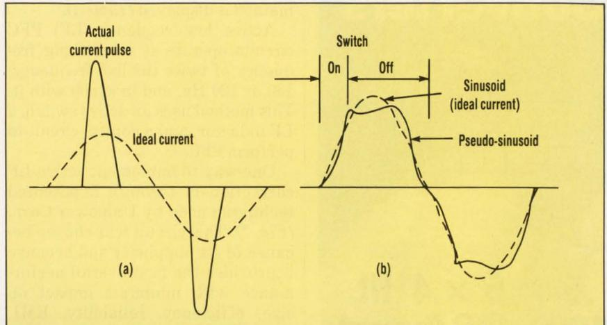
**8. BOTH THE UNCORRECTED** input current to a switching power supply (a) and the pseudo-sinusoidal input current produced by active LF power-factor correction (b) are illustrated.
