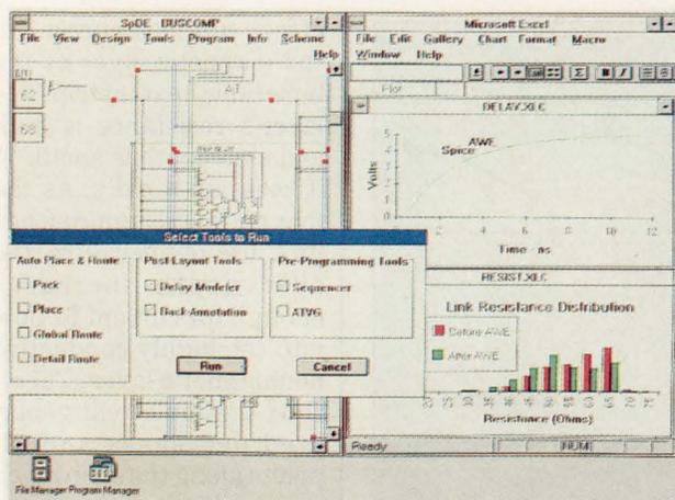
ymptotic Waveform Evaluation (AWE) describes FPGA circuit interconnects to an nth-order approximation. As a result, simulations of the same run time as previous techniques produce far more accurate results.
