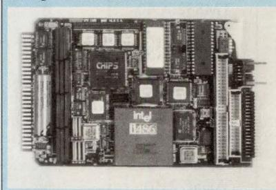
comes with standard PC/AT peripheral devices, including a keyboard interface, two RS-232 serial ports, a parallel port, interrupt and DMA controllers, a counter-timer, and a battery-backed real-time clock. An optional VGA video board can be added. With 4 Mbytes of RAM, the 25-MHz board goes for \$2995.
