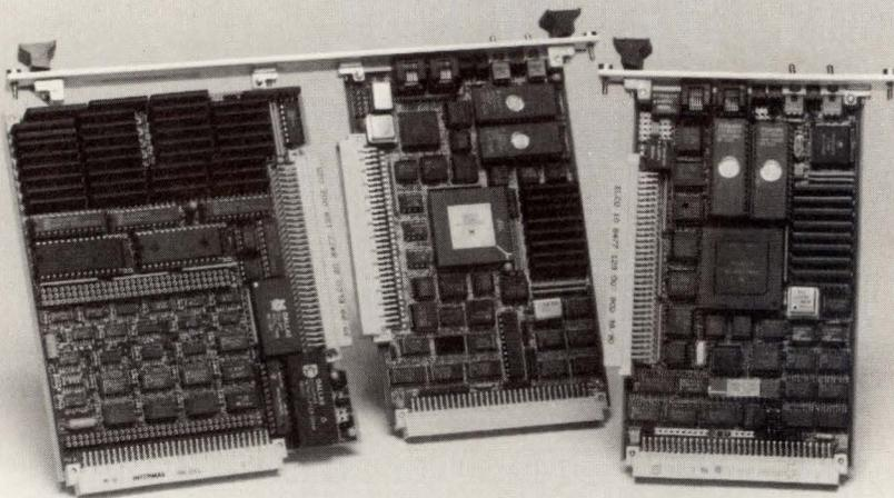
**2. WITH THE 3U CARDS' MXBUS CONNECTOR** mounted on the side, two cards can be joined together to fit into a 6U slot. The proprietary structure from Mizar contains a family of modules ranging from simple I/O ports to complex parallel-processor expansion modules.
