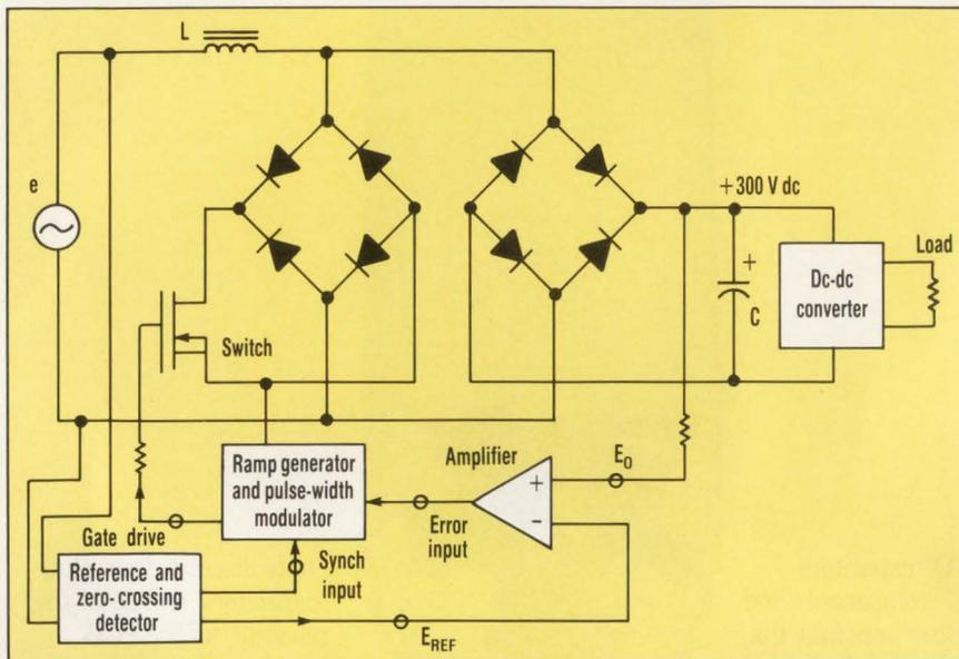
**7. THE ACTIVE LOW-FREQUENCY** power-factor-correction circuit uses a switched inductor to produce a pseudo-sinusoidal input current with low harmonic currents. A pulse-width modulator controls the operation of the MOSFET switch. Power factors between 0.96 and 0.98 are realized.
