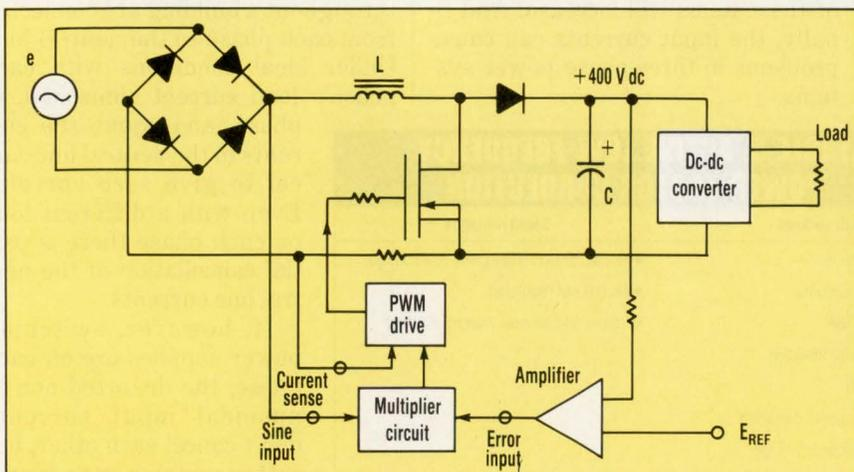
**6. THE ACTIVE HIGH-FREQUENCY** power-factor-correction circuit forces the input current to be sinusoidal. It also regulates the voltage going to the dc-dc-converter part of the power supply. Power factors from 0.97 to 0.99 are achieved.
