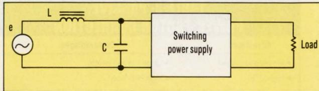
**5. A PASSIVE** power-factor-correction circuit can be a simple LC filter when the correction must be performed external to the power supply.
