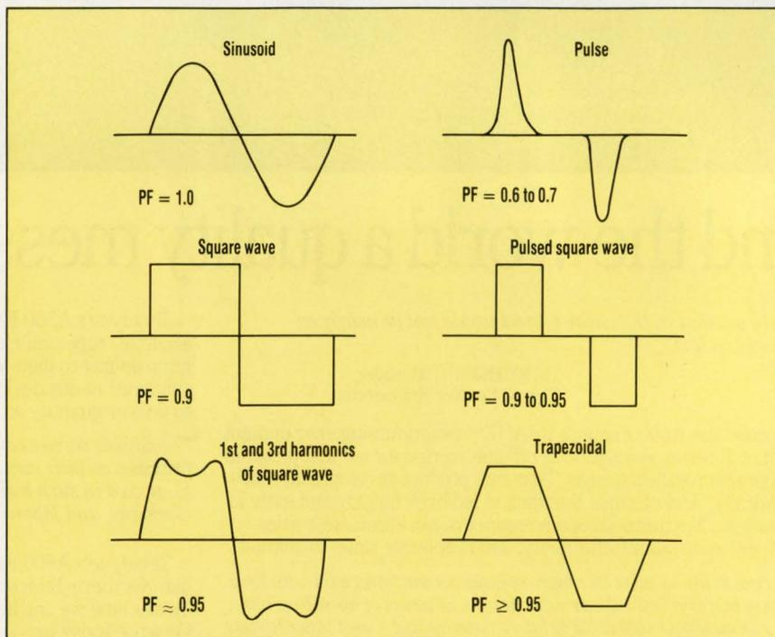
**4. MANY INPUT-CURRENT** waveshapes yield a relatively high power factor, but the shape must be close to a sinusoid to also attain low harmonic currents.
