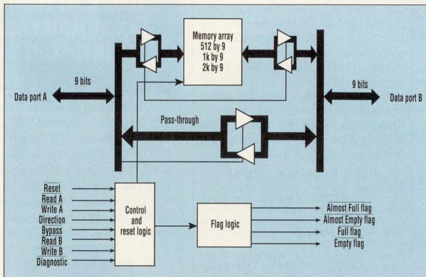
**REQUIRING A SINGLE** bank of memory, Integrated Device Technology's bidirectional FIFO chip uses a Direction pin to control the direction of data flow between Ports A and B. A memory bypass feature lets critical data skirt the memory array and the delay it imposes, thereby allowing time-critical data to immediately reach the opposite port.
