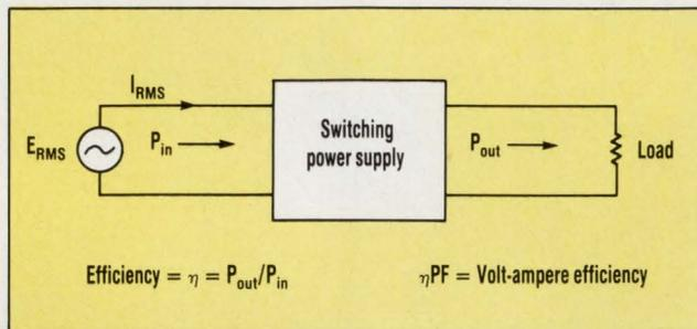
**3. VOLT-AMPERE** efficiency,  $\eta$ PF, is the figure of merit that determines the input current for a switching power supply.
