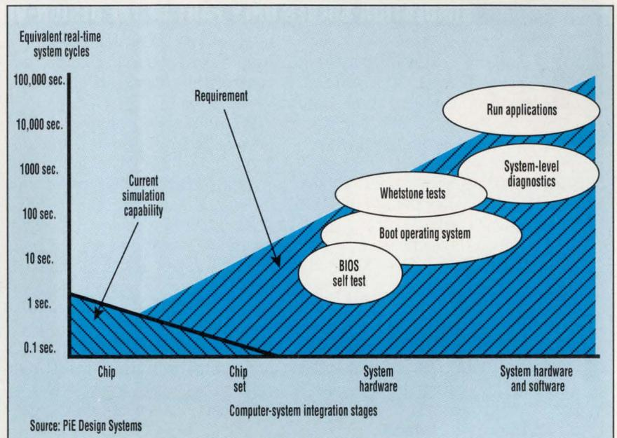
**2. THIS GRAPH ILLUSTRATES** why today's software-simulation approaches fall short when trying to verify a computer system. The simulator must perform almost 100 seconds of equivalent real-time system cycles just to boot the operating system.
