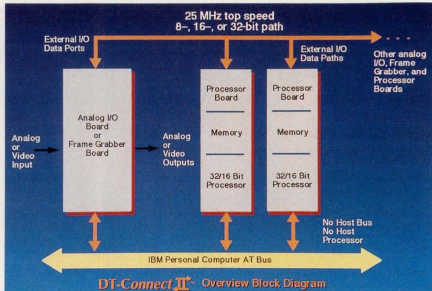
**3. DESIGNED FOR THE PC/AT'S ISA architecture, DT-Connect II from Data Translation transfers data at speeds up to 100 Mbytes/s. This specification is logically and electrically compatible with its predecessor, DT-Connect, thus making it backward-compatible. Because the standard's 32-bit modes are symmetrical, any board can transfer data to and from any other board within the connection.**
