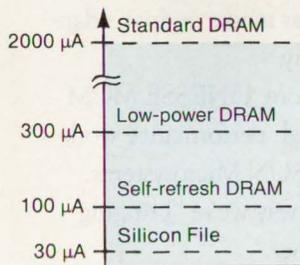
be your highest priority, but you'll be glad to know that DRAM memories from NEC operate on an absolute minimum power supply. Based on a 0.7 µm, stacked capacitor process, NEC's 4 Megabit DRAMs offer high access speeds and convenient configurations for a wide range of desktop and portable applications. Competitively priced standard DRAMs have
