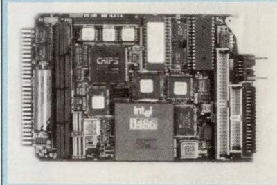
comes with standard PC/AT peripheral devices, including a keyboard interface, two RS-232 serial ports, a parallel port, interrupt and DMA controllers, a counter-timer, and a battery-backed real-time clock. An optional VGA video board can be added. With 4 Mbytes of RAM, the 25-MHz board goes for \$2995.
