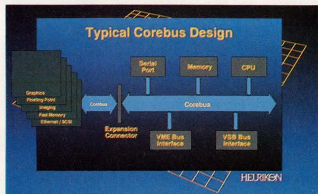
**1. COREBUS IS A HIGH-END synchronous mezzanine bus** from Heurikon that features a 50-MHz clock speed and a maximum bandwidth of 200 Mbytes/s. The bus can handle graphics, networking, and floating-point operations. It also supports four interrupt lines, each with a separate Acknowledge signal.
