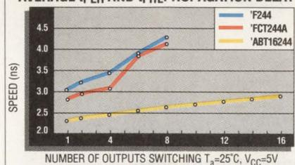
**TI's speed advantage:** In a one-to-one comparison, a TI 'ABT16244 16-bit Advanced BiCMOS driver proves to be much faster and more stable than Advanced Bipolar and standard CMOS octal drivers.
