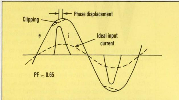
**2. THE INPUT CURRENT** of a switching power supply is a non-symmetrical pulse that occurs near the peak of the ac voltage. This pulse can cause clipping of the voltage waveform.
