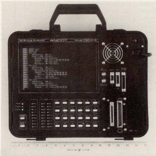
1. THE DSC-216 SCSI BUS ANALYZER fits into a compact attache-style case. The display is an 80-character-by-24-line electroluminescent panel.
