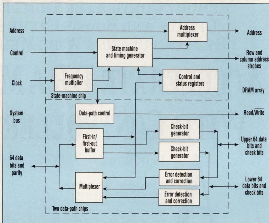
**1. THREE CHIPS** form the CYM7232 or 7264 DRAM accelerator and controller module from Cypress Semiconductor. Two of the three custom chips are identical, with each forming a 32-bit slice (7232 only; 64-bit paths in the 7264) of the data path. The third chip, a multiple-state-machine IC, controls the module's interfaces and word-transfer timing.
