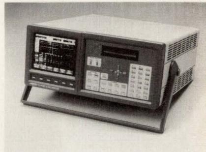
channels at 200 MHz, both synchronously and asynchronously. This mode includes eight clock inputs with full Boolean, master-slave, or double-edge clocking. In the split mode Paladin offers 80 channels of 100-MHz synchronous data collection along with 20 asynchronous channels. In the high-speed mode the system supplies 10 asynchronous channels at 1 GHz and 20 asynchronous channels at 500 MHz. Multiple modules can be connected together.
