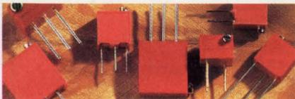
**MILITARY TRIMMERS** from the Techno Division include broad MIL qualification to RT24, 26, 27; RTR24; RJ24, 26 and RJR24, 26. Techno RJ24 and RJR24 trimmers offer you 25 turns for precision adjusting, while the RJ26 and RJR26 offer 22 turns. They have zero backlash and offer a monolithic clutch.
