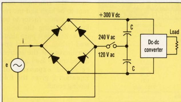
**1. AN OFF-LINE SWITCHING** power supply's input circuit has a full-bridge rectifier and storage capacitor. The circuit is a voltage doubler for 120-V ac input.
