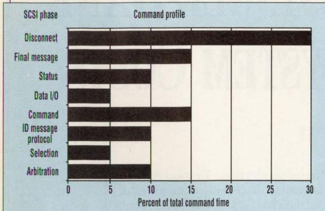
**2. THE ANALYZER'S COMMAND** profiling capability helps users identify SCSI command overhead during bus utilization. The report shows the time spent on each phase of a SCSI command.
