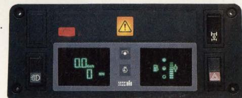
*Electronic Instrument Panel to J.I. CASE Tractors.*
