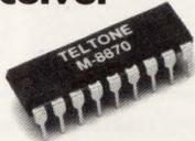
M-8870 is a full DTMF receiver that integrates bandsplit filter and digital decoder on one 18-pin CMOS DIP.
