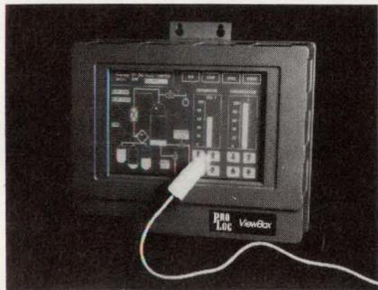
Functioning as either a standard EGA terminal or as a touch screen, the ViewBox electroluminescent (EL) display is enclosed in a rugged, splash-proof cast-aluminum housing. The EL display has a resolution of 640 by 350 pixels with a highly visible bright-orange screen. The optional touch screen, which contains 1024 by 1024 points, uses a capacitive method to detect operator touches. The touch screen comes with calibration and mouse-driver software. The ViewBox sells for \$1995; the touch-
