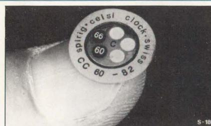
Put a low cost CelsiClock® temperature monitor on any surface.
