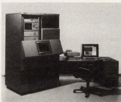
test firmware enhancements allow the same test system to be used for testing small- and medium-size production runs. The system's software and true tester-per-pin architecture allow all channels to operate at the maximum frequency, so users can perform thorough tests on even the most complex devices. Per-channel cost is about \$2000. In a typical 128-channel configuration, the HP 82000 Model D100 costs \$260,000. Delivery is estimated at 14 weeks after receipt of an order.
