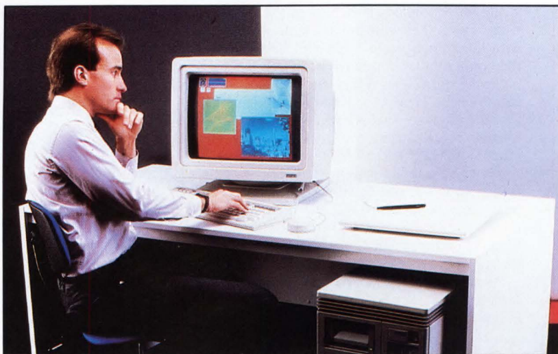
1. Digital Equipment's VAXstation II/GPX sports two processors. The main processor is a 32-bit workstation version of the successful VAX architecture, the MicroVAX II. The graphics processor is in the display where it speeds up graphic processing.
