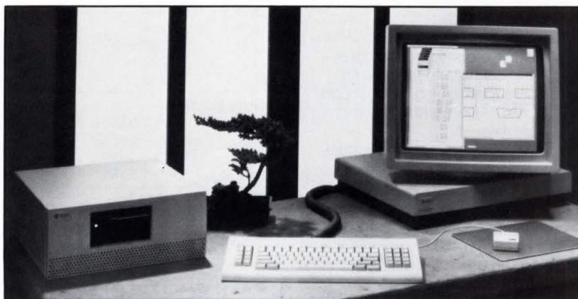
3. The Sun 3/52M is one of the least expensive, 32-bit stand-alone workstations. It also has a slightly slower, cheaper cousin, the 3/50M (see directory on the next page), that sells for $7900 without a disk but with a 68020 processor and 4 Mbytes of memory.
