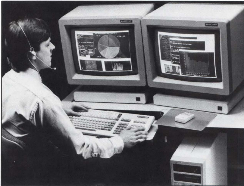
4. While the Masscomp 5300 is a moderate-cost 32-bit workstation, it is also a base station for data acquisition. With hardware additions, it can handle up to 1 million samples per second.
