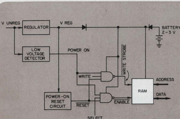
1. A battery-backup RAM circuit has gates that are powered by the battery when +V REG is off. Typical power-on reset circuits generate premature outputs,
