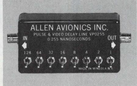
**TV STUDIOS & VIDEO INDUSTRY** New Allen Avionics Video & Pulse Delay Lines replace 75 ohm coaxial cable, provide a more suitable method of achieving precise short delays. The units reduce size, weight, installation cost, and save time and effort in making delay changes. Finest specs. Lowest pricing. Catalog also discusses Video Filters. See us at Electro/78, Booth 1538. Allen Avionics, Inc., 224 E. 2nd St., Mineola, N.Y. 11501, 516-248-8080.
