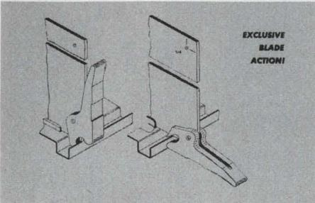
**FREE SAMPLES** of new, low-cost Electro-Flex injector/ejector for damage free insertion and extraction of P.C. boards. Unique design utilizes both surfaces of a single blade . . . eliminating need for very close tolerances. Full 5/8" travel in each direction assures straight-line card movement. Meets established industry standards for mounting. Molded in rugged UL-approved nylon for 1/16" through 1/8" boards. **ELECTRO-SPACE FABRICATORS**, Tipton, Pa. 19562. (215) 682-7181
