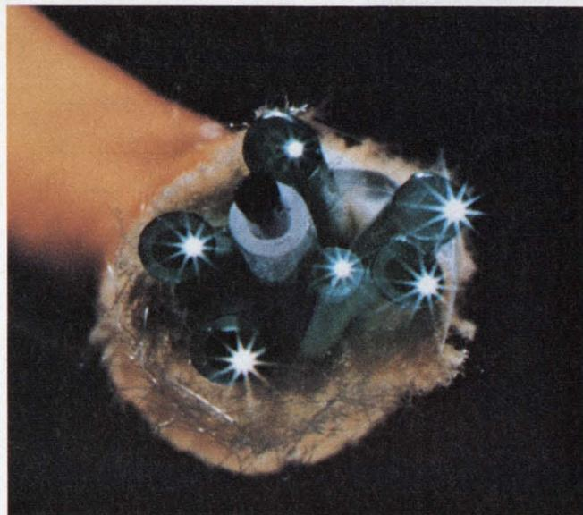
The key to long-range optical communication systems lies in continuing improvements in optical fibers and cables, such as this new Siacor six-fiber structure.
