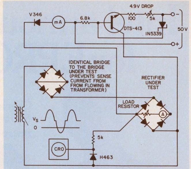
3. Acting like a full-wave bridge rectifier, this test circuit treats the diode as if it were in actual use in its intended circuit and applies sensing current as well.
