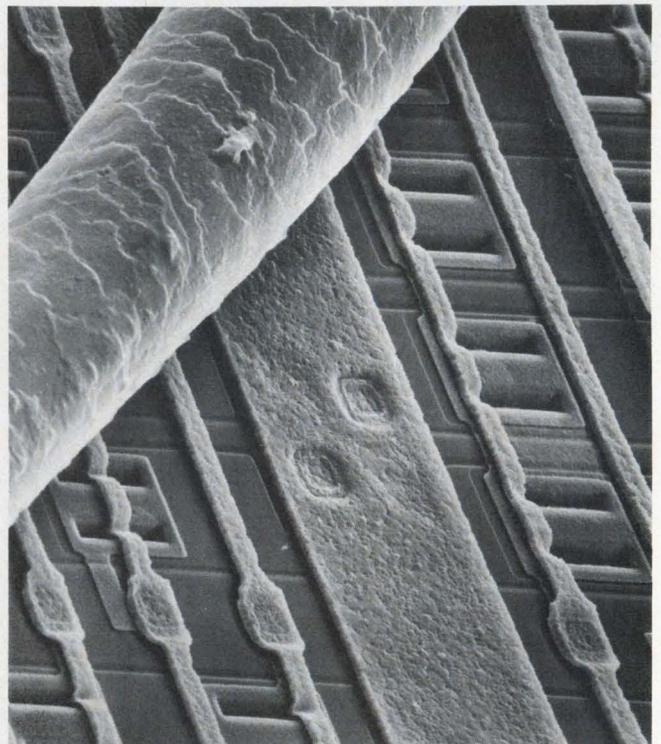
**Using three dimensions,** VMOS shrinks memory cells until eight fit in the cross-section of a human hair. This photo is a 10,000-time enlargement from AMI.
