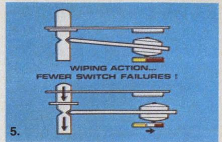
5. Wiping action helps clean away surface contamination in low level circuits, where contact resistance must be kept low. Breaks through minor contact welds that cause switch failure under high current conditions.
