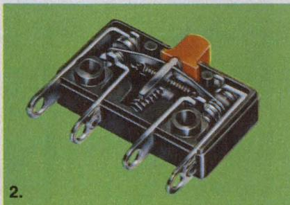
2. Coil spring snap-action mechanism extends life of switch. (Outlasts stressed blades in terms of metal fatigue.) Overcenter and compression springs are not stressed to their limits even under full overtravel as are stressed blades. Coil springs retain characteristics longer under usage than stressed blades.
