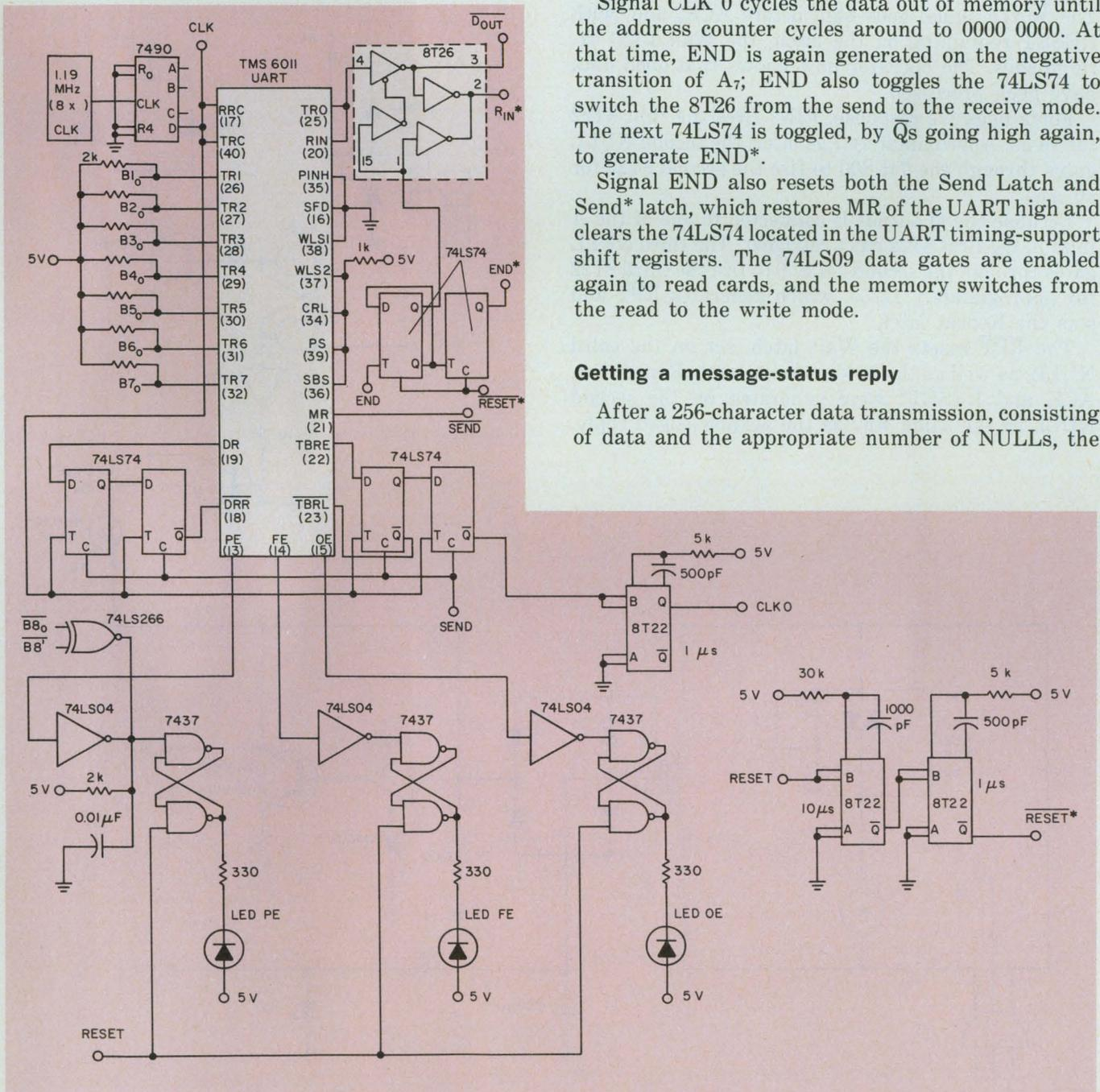
6. Data parity is tested again as information leaves the memory and enters the UART. The CPU acknowledges or
