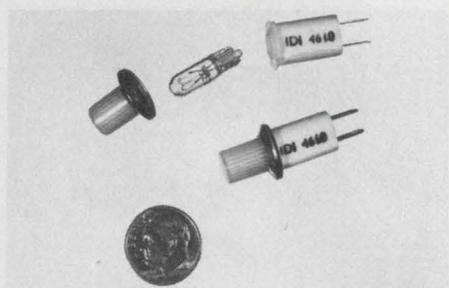
**New subminiature replaceable-lamp incandescent lights.** 50% cheaper than conventional submini flange-base or bi-pan because lamp base formed for bulb's glass and lead wires permits high-speed production. Socket-and-assembly design for one-hole mounting. Flat, dome, seven colors, 2 to 28 V. Samples and specs: Industrial Devices, Inc., Edgewater, N.J. 07020.
