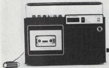
**PROGRAM LOADER . . . uses computer's existing RS232 terminal port.**
