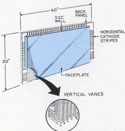
This feedback-multiplier TV-display tube is in a viewing position. Its vertical vanes are internal glass platelets with metalized electrodes that form the feedback-multiplier cells.
