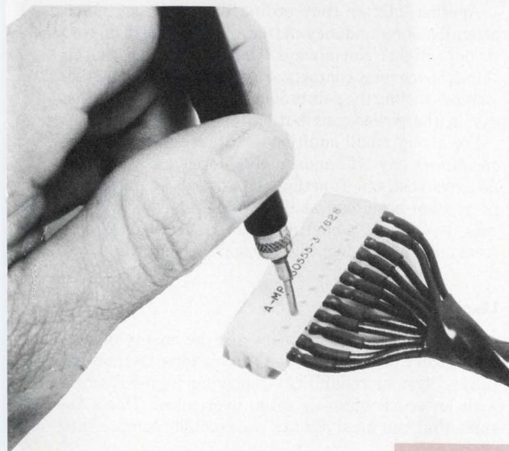
3. **Quick-disconnect-type connectors** from AMP mate a PC card to a cable and provide test-probe holes so the cable can be accessed while it is connected to the circuit.
