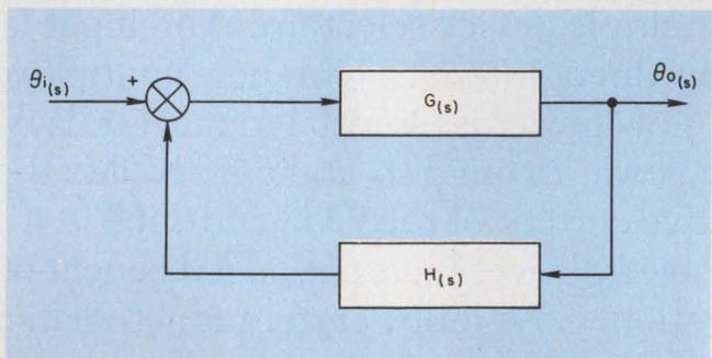
2. The phase-lock loop's generalized open-loop transfer function,  $G(s)H(s)$ , has a third-order denominator—from which the circuit's name is derived.
