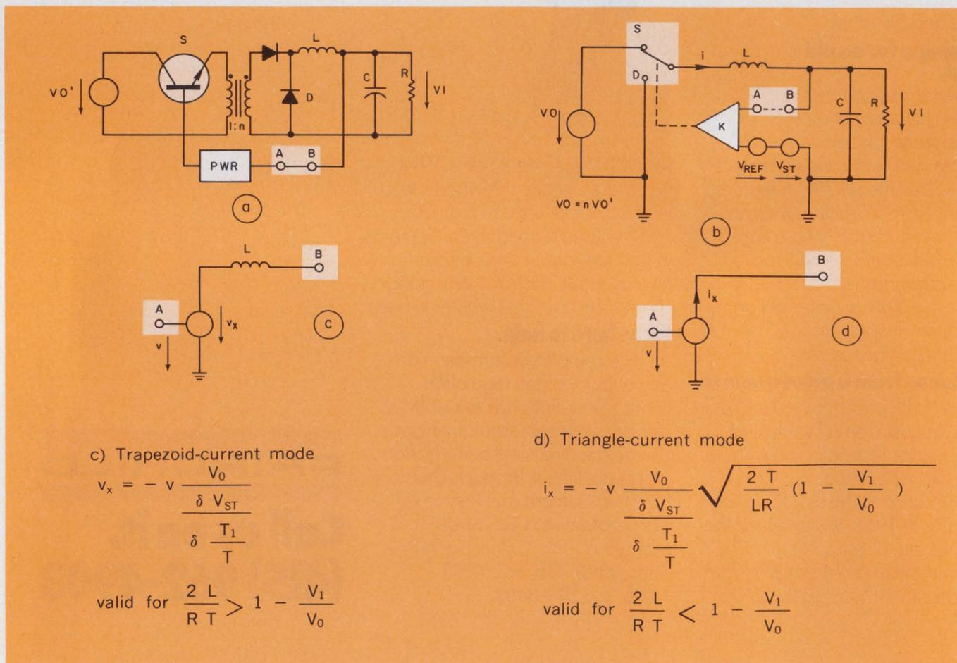
1. A down-converter switching supply (a) relies on constant-frequency switching. Varying the switching-pulse width regulates the output. The equivalent circuit for the entire supply (b) shows that the PWR responds
