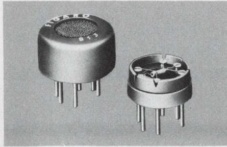
**FIGARO GAS SENSOR TGS** is a gas sensitive semiconductor. When combustible gas is absorbed on the sensor surface, a marked decrease of electrical resistance occurs. Major features of the sensor include high sensitivity, long term reliability and low cost. The applications are: GAS-LEAK ALARM, AUTOMATIC FAN CONTROL, FIRE ALARM, ALCOHOL DETECTOR, etc. Figaro Engineering Inc., North America Office-3303 Harbor Boulevard, Suite D-8, Costa Mesa, Calif. 92626 Tel: (714) 751-4103 Telex: 678396
