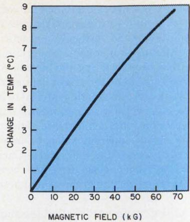
1. Applying a strong magnetic field changes the temperature of gadolinium. The variation of temperature with field shown above was obtained in NASA experiments.
