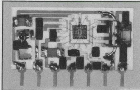
**ULTRA SMALL ACTIVE BAND PASS FILTER** fabricated using OP Amp incorporated Hybrids Circuit. Operating Voltage 1-2.5V/4-15V, Frequency Range 288.5-2800Hz, Q 180+20, 35+5 and etc. .788" x .138" x .433". By adding Feed Back Circuit of extra Diode and Capacitor, it does the job of small but reliable Oscillator. Active Filters can be tailor-made to customer's specifications. IWATA ELECTRIC CO., LTD. Mansei Bldg., 1-1-16 Sotokanda, Chiyodaku, Tokyo, Japan.
