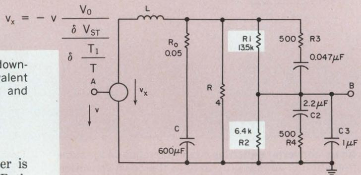
apply the dc voltage,  $V_1$ , at A. The same  $V_1$  then appears at B, which means that the circuit's steady state isn't disturbed by breaking the loop.
