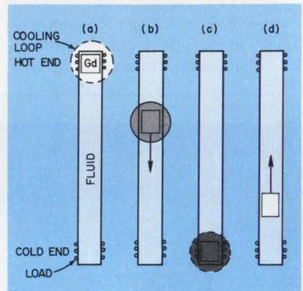
2. A magnetic heating-cooling cycle is obtained with a gadolinium working element that exchanges heat with a working fluid. The dotted circle (a) represents an increasing field while that in (c) is a decreasing field. For operation, see text.
