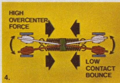
4. High overcenter force, small contact mass and short blade length maintain high contact pressure longer than usual stressed blade assemblies. This results in better resistance to shock and vibration. It also provides high contact pressure essential to low contact resistance for low level current use. Extremely short rebound time, when contacts collide minimizes bounce (mechanical) to increase (electrical) life.
