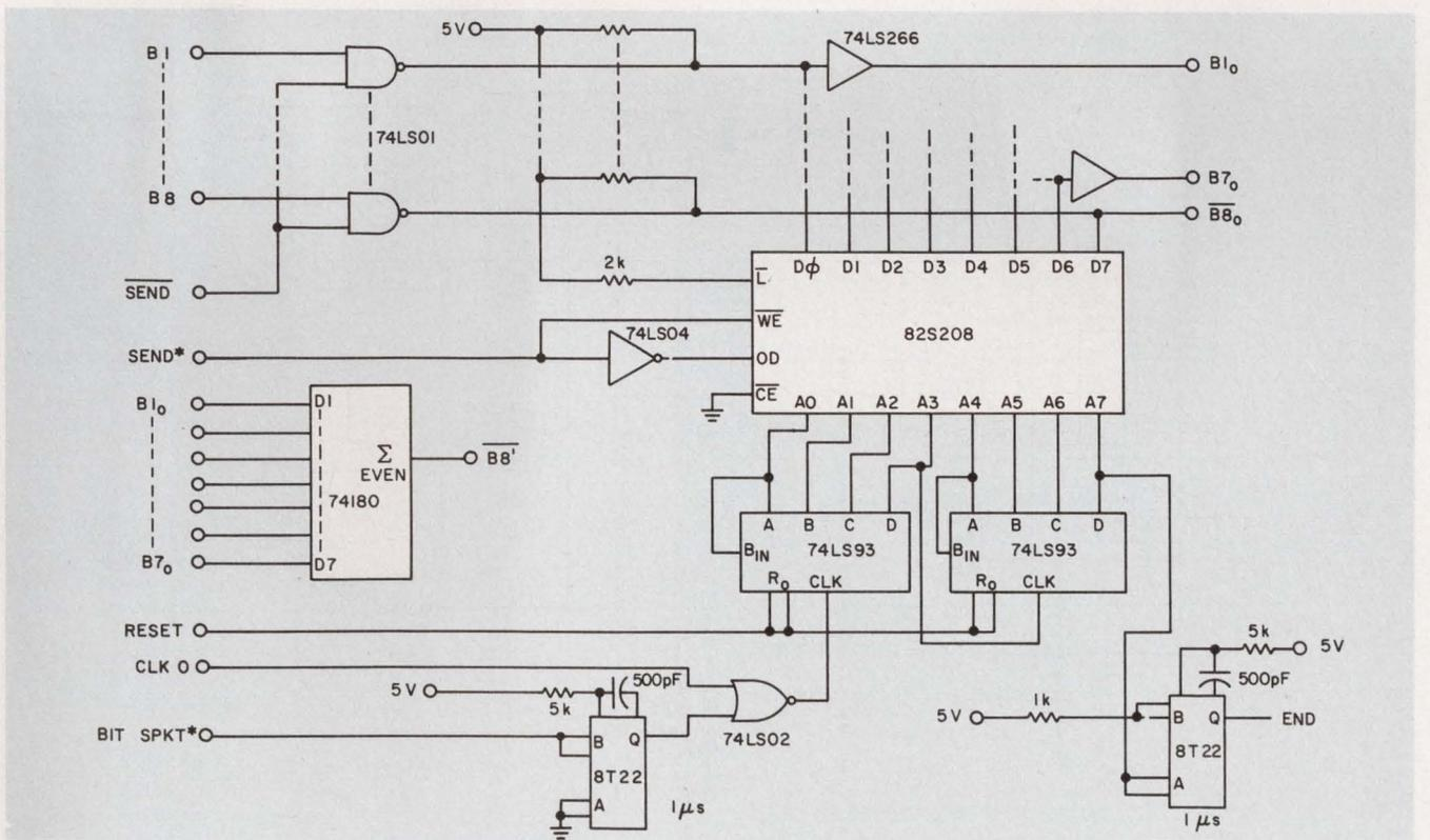
4. Data are checked for parity errors by an exclusive-NOR gate during memory loading. If the parity bit, as read in
