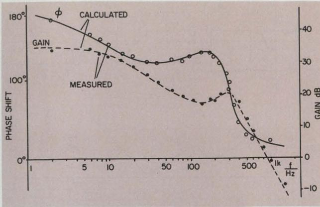
5. Calculated and measured gain and phase-shift values for the down-converter PWR of Fig. 4 correspond closely. The closeness shows that the equivalent circuit indeed represents the actual circuit.
