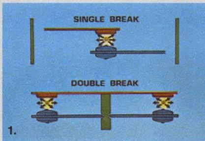
1. The Licon double break design offers twice the arc breaking and current interrupting ability with a bonus of much better heat dissipation than single break switches of similar size.
