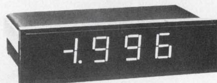
Check carefully to make sure digital outputs are compatible with your system. At one time, TTL-compatible outputs were the norm in DPMs, but higher-density, large-scale MOS chips have changed that. As a result, some DPMs now have digital interfaces with voltage swings of 12 V instead of the TTL standard 5 V.
