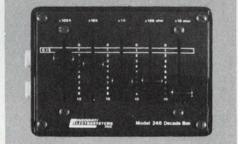
**DECADE RESISTANCE BOX Model 246** offers a selection of 1% 1/2 watt resistance values from 10 ohms to 1,111,110 ohms in 10 ohm steps. 0.1% calibrating resistors are provided at 100, 1000, 10,000, and 100,000 ohms. Five 11-position slide switches allow ease of operation. SIZE: 4" x 2-7/8" x 1-9/16" PRICE: \$34.95. CINCINNATI ELECTROSYSTEMS, 469 Wards Corner Road, Loveland, Ohio 45140, (513) 831-4347
