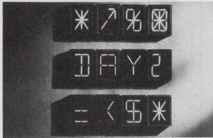
**ALPHANUMERIC DISPLAY, 16 Segment - Day 2 series** offers a large, bright 5/8" character that can be read in high ambient light, including direct sunlight. Rated @ 5 volts, 18ma per segment, the DAY-2 plugs into a standard 18 pin DIP socket. Withstand a wide temp. range, -55° C to +100° C. Color can be displayed w/ filters. Uniglass construction insures high reliability, 100,000 hr life rating. DAY-LIGHT DISPLAY CORP., 11 Fairfield Pl., P.O. Box 1231, West Caldwell, N.J. 07006 (201) 575-1045
