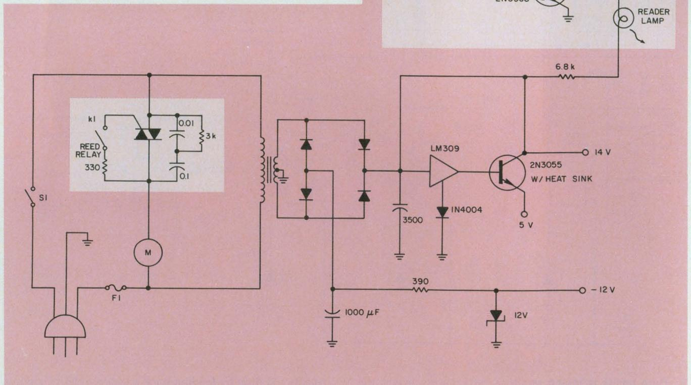
7. Power-supply and motor-control circuits are straightforward. The RC across the triac suppresses noise.
