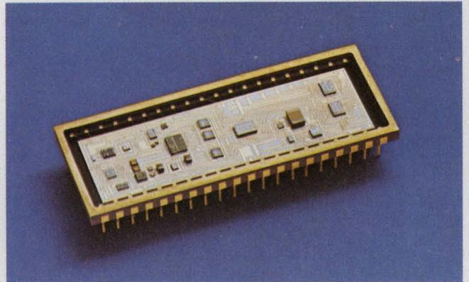
**Local control of data acquisition at the sensors** is provided by new hybrid components like this d/a microperipheral interface package, the MN5500 by Micro Networks.
