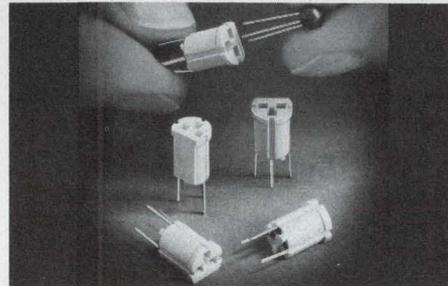
**NEW 3-LEAD TRANSISTOR SOCKETS** from Methode have an extended funnel-shaped lead-in which eliminates the need for transistor lead preforming or trimming. Also, ideally suited for automatic insertion of transistors into the socket. Contacts are reliable dual leaf cantilever type of phosphor bronze with tin plating. Insulation is flame retardant polyester rated 94VO. Methode Electronics, Inc., 1700 Hicks Rd., Rolling Meadows, IL 60008. (312) 392-3500.
