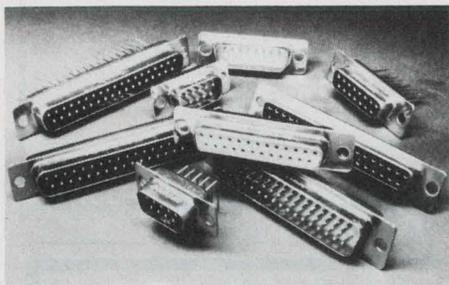
**SOURIAU Sub "D" Series 8634 NORMAN-D connectors** are low cost, crimp type, w/ stamped & reeled contacts for lower install. costs; intermateable w/ all "D" connectors. SOURIAU has "D" connectors in 1-piece thermoset, 2-piece thermoplastic insulator, non-removable solder contacts, rigid & float mount shells, crimp, rear release contacts, operating temp of -55°C to +125°C qualified to MIL-C-24308. SOURIAU, INC., 7740 Lemona Ave., Van Nuys, CA 91405 (213) 787-5341.
