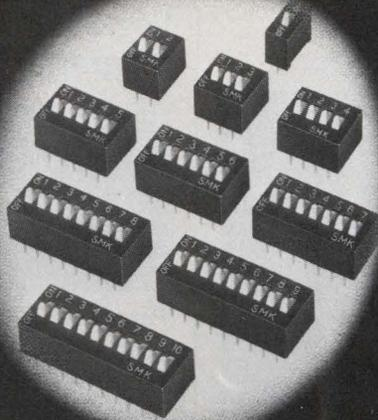
The **JS-8722 Series** is a complete line of DIP Switches, from 1 to 10 positions, featuring sealed construction to prevent flux contamination during wave soldering. A clip-type wiper design assures positive 2-sided contact to provide excellent shock and vibration characteristics.
