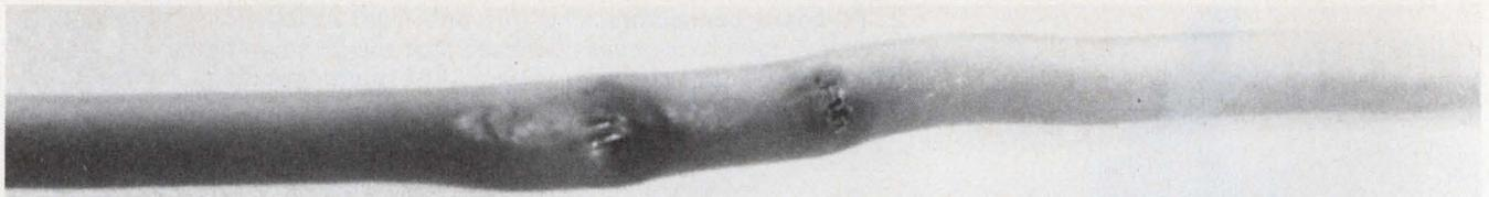
4. **Exposed insulated wire** can short to the equipment frame due to "cold flowing" of the insulation. Pressing,
