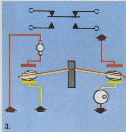
3. Dual circuit capability—with two normally open and two normally closed contacts, two isolated circuits can be controlled with one single pole Licon switch. That's a unique advantage of Form Z switching.
