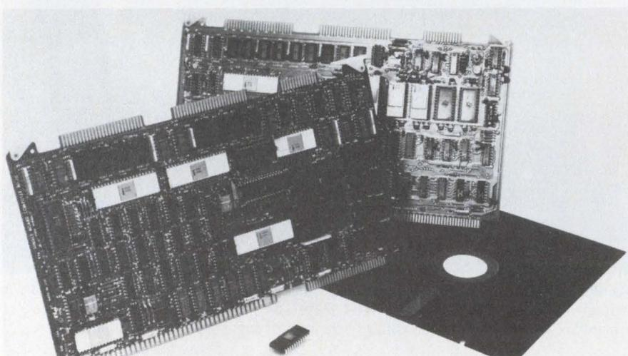
**Software operating systems can be stored** on Intel's SBC 80 single-board microcomputers internally in semiconductor ROM or externally on diskettes. This feature is possible thanks to Intel's new RMX/80 Real-Time Multi-Tasking Executive software package.
