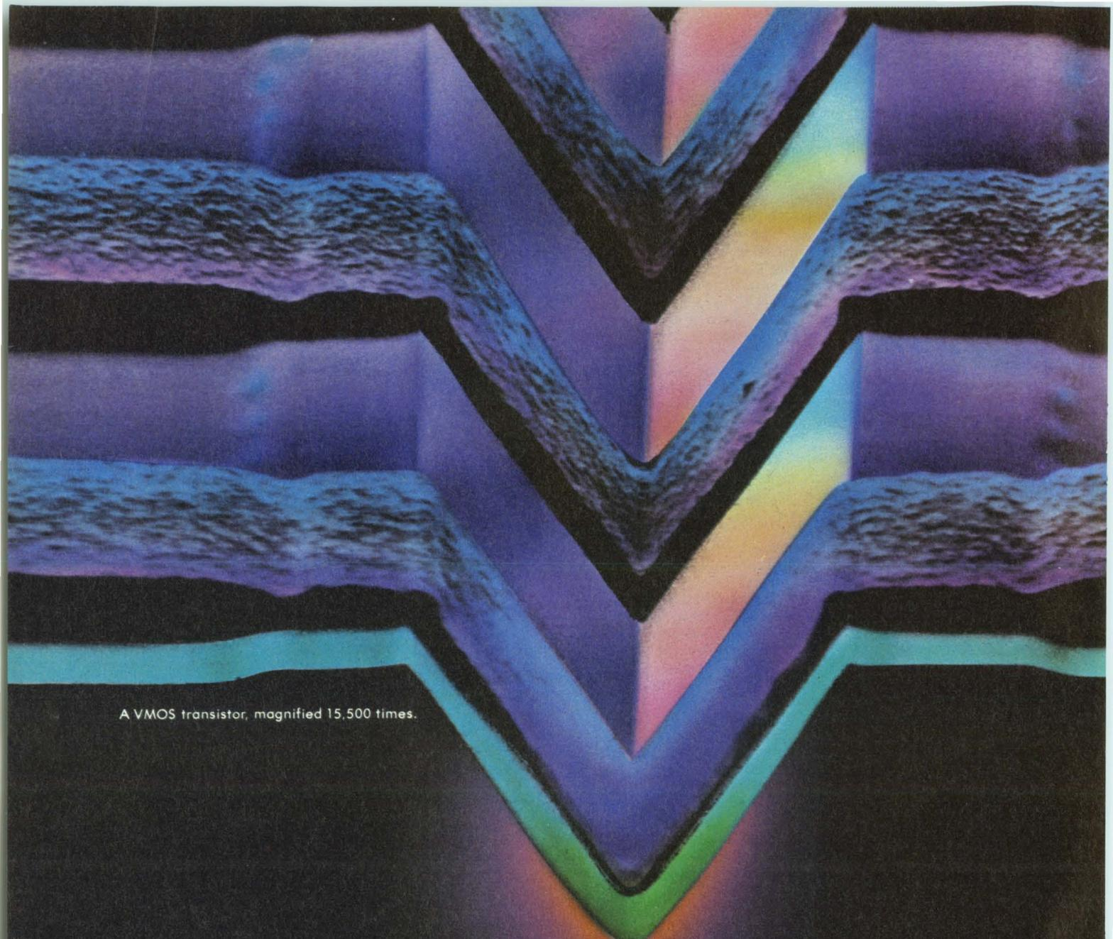
A VMOS transistor, magnified 15,500 times.
