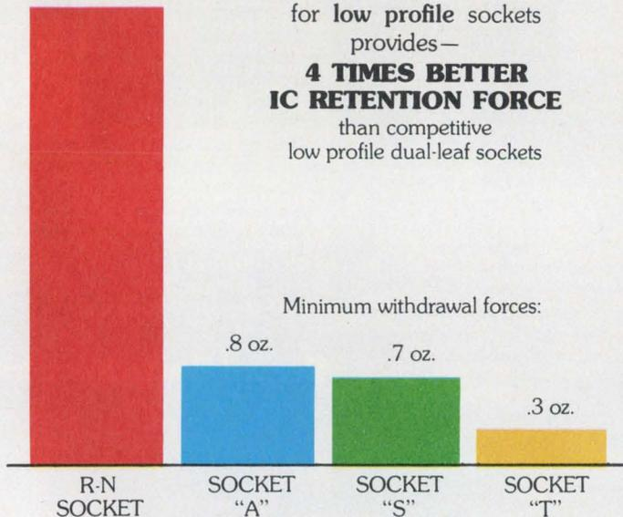
\* In "Fat-Skinny test," withdrawal forces are measured using the smallest size (.008") lead after insertion of largest size (.012") lead.
