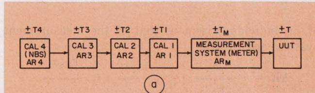
$$T_a = \sqrt{T_M^2 + T_1^2 + T_2^2 + T_3^2 + T_4^2}$$
