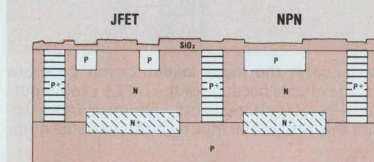
Next, p-type diffusion forms the JFET drains and sources as well as the bipolar bases:
