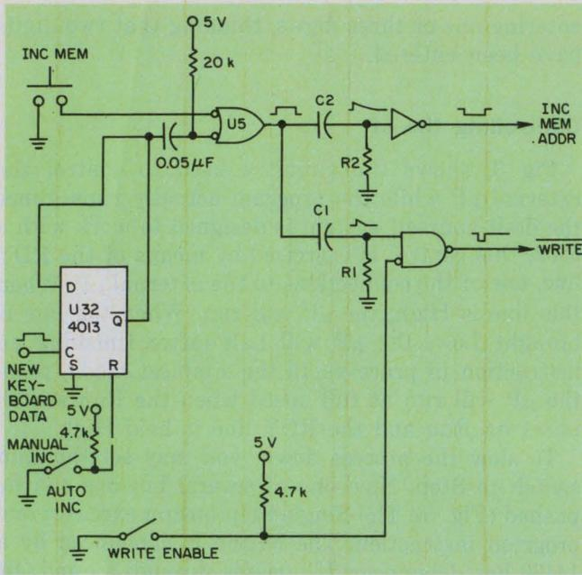
**4. Memory-write control is simple** and straightforward. When the write-enable switch is closed, pressing the Inc Mem button will generate first a write pulse (through  $C_1R_1$ ), then a positive edge to increment the memory address through  $C_2R_2$ .
