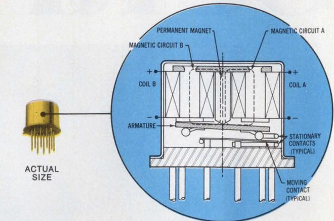
size makes them ideal for high density pc board packaging, and they're available in SPDT, DPDT and 4PST contact forms. And for RF switching, their low intercontact capacitance and contact circuit losses provide high isolation and low insertion loss up through UHF.
