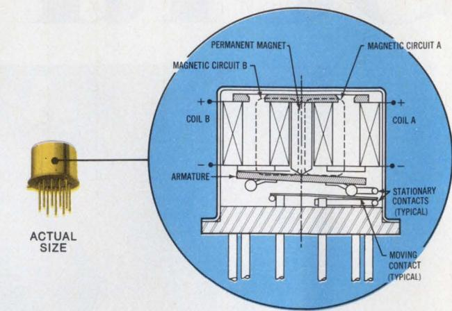
size makes them ideal for high density pc board packaging, and they're available in SPDT, DPDT and 4PST contact forms. And for RF switching, their low intercontact capacitance and contact circuit losses provide high isolation and low insertion loss up through UHF.
