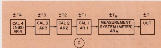
$$T_Q = \sqrt{T_M^2 + T_1^2 + T_2^2 + T_3^2 + T_4^2}$$
