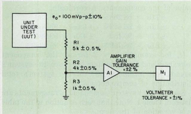
1. Only the tolerance limits of each system component are needed to establish the over-all accuracy of the readings taken in a measuring system.
