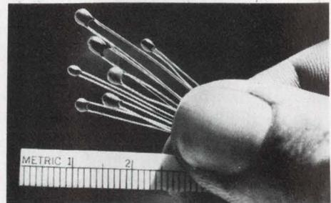
**THERMISTORS** with leads and coating are highly reliable low cost components in small dimensions more compatible with modern circuit design. R @ 25°C 100 $\Omega$  to 1 meg  $\Omega$   $\pm 10\%$  to  $\pm 1\%$ . CURVE MATCHED INTERCHANGEABLES to  $\pm .25^\circ\text{C}$ . POINT MATCHED INTERCHANGEABLES to  $\pm .2^\circ\text{C}$ . Call or write for HP97 or TI SR52 THERMISTOR LINEARIZATION PROGRAM. WESTERN THERMISTOR CORPORATION, 354 Via Del Monte, Ocean-side, CA 92054. (714) 433-4484.
