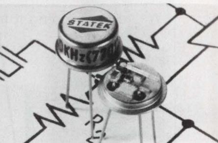
**CMOS Crystal Oscillators in Low profile TO-5.** Frequency range is 10 kHz to 300 kHz (divided outputs to 1 kHz, low as one cycle per month available). Low milliamp current consumption. Accuracy  $\pm 0.01\%$ . Shock 1000 g. Hybrid thick and thin film chip and wire design is rugged and ideally suited for portable equipment. Details in Gold Book & EEM \* STATEK CORP \* 512 N. Main, Orange, Ca. 92668 \* (714) 639-7810 \* Telex 67-8394.
