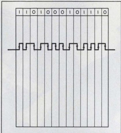
"Phase-encoded recording solved the problem. At every bit time, at least one flux reversal occurs—one reversal indicates a ZERO, two reversals indicate a ONE. The flux reversal is in one direction for a ZERO, another for a ONE. This scheme provides a self-clocking mechanism that can track a string of repetitive bits, no matter how long it is."
