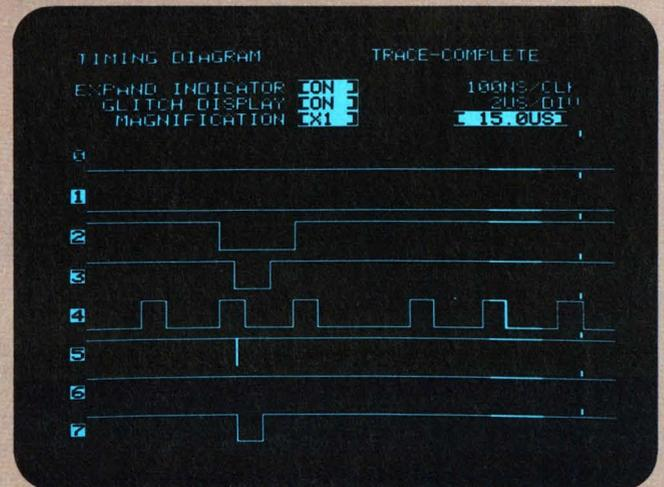
**Observing timing display** of signals on I/O and one-shot shows that the glitch on the input to the one shot (channel 5) occurs four machine cycles before the trigger point and is coincident with the transition on I/O read (line 3) indicating possible capacitive coupling.
