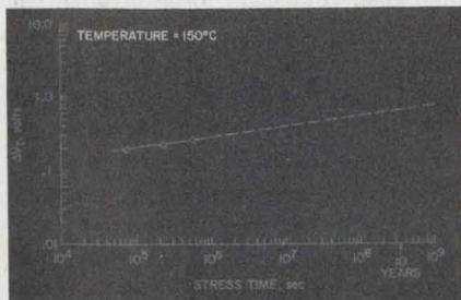
**3. The stress-vs-time curve** shows that American Micro Systems' VMOS EPROM will lose less than 1 V after 40 years at 150 C.
