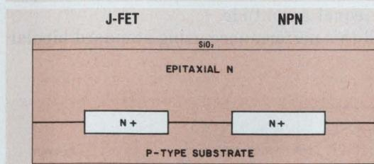
To start,  $n^+$  is diffused into the substrate's n-type epitaxial layer:
