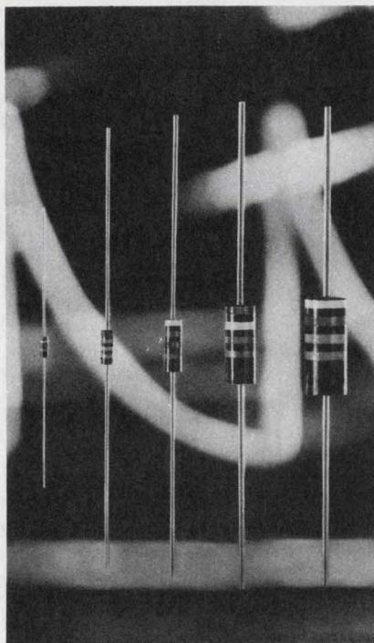
**Hot-molded carbon-composition resistors**, though under fire from film-type resistors, are here to stay, according to Allen-Bradley. Their ruggedness, reliability, low cost, and wide range of sizes and applications are hard to beat.
