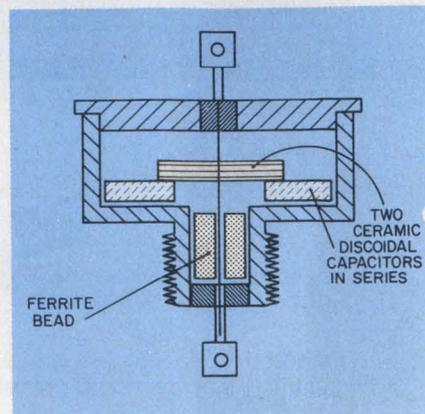
a dc resistance of less than 6 m $\Omega$ . The filter can have a 0.375-in. diameter and is fitted with a 1/4-28 threaded mounting stud.
