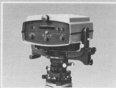
New HP 3810A Total Station electronic distance and angle measuring device.
