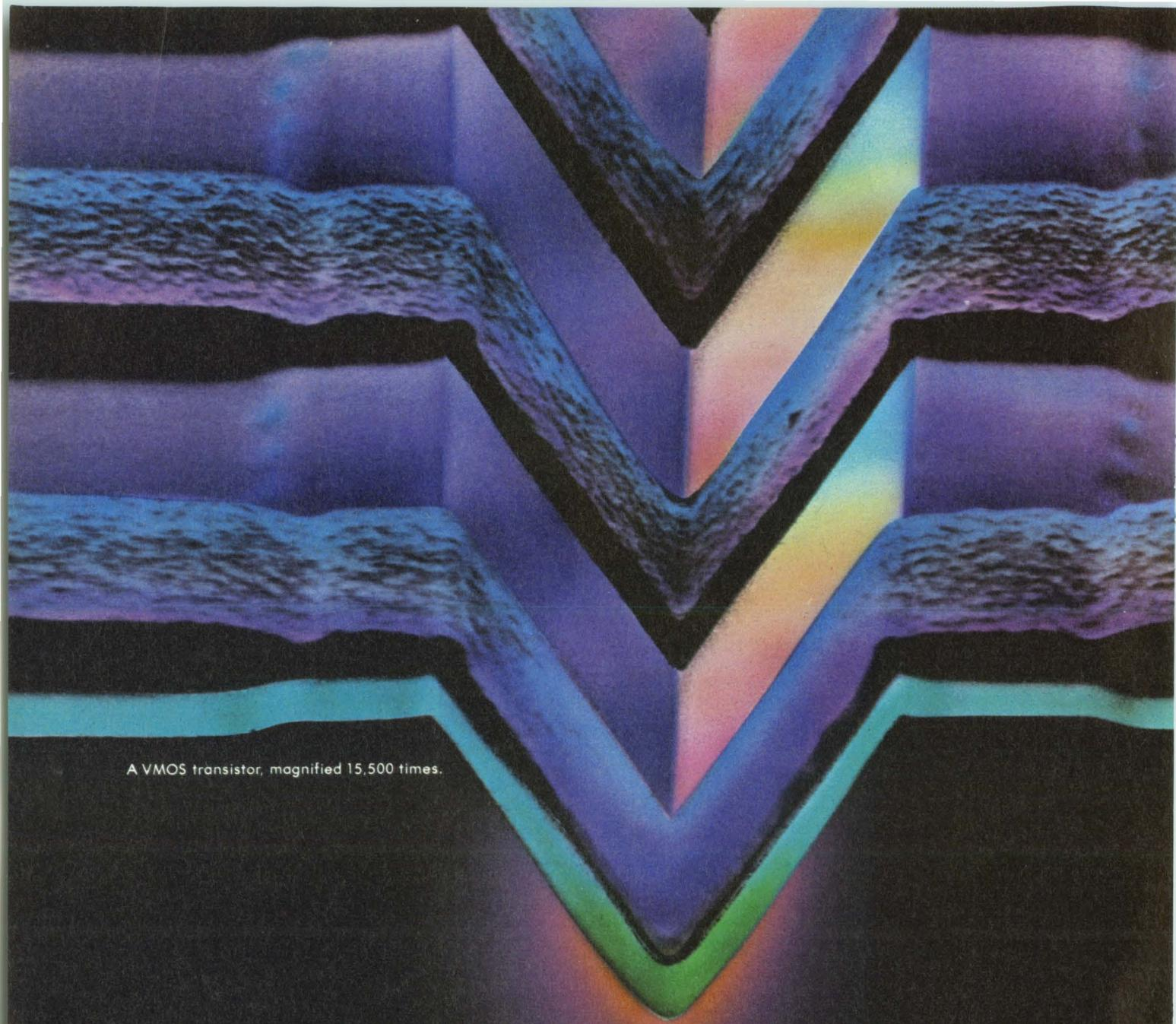
A VMOS transistor, magnified 15,500 times.
