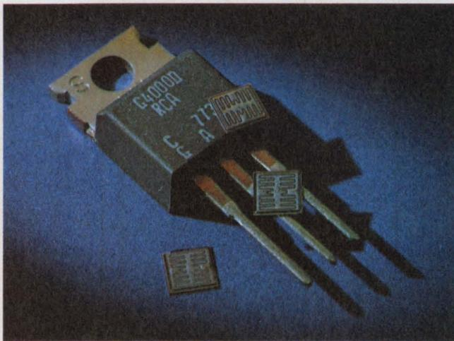
**New thyristor designs:** The G4000 Versawatt gate turn-off thyristor (left) simplifies turn-off, and the S7310 asymmetrical SCR (right) operates to 40 kHz. With easier control and higher speed, RCA pushes aside former SCR
