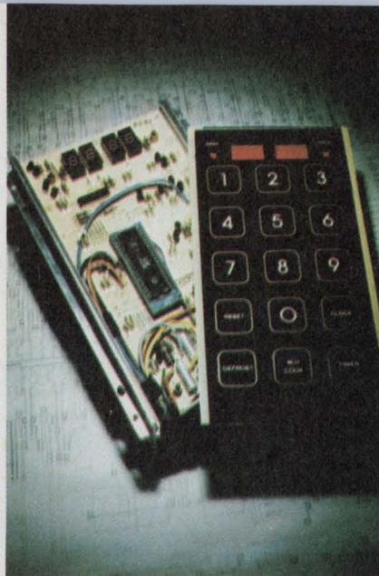
**By bringing down the cost of microprocessors,** General Instrument has been able to design them into cost-conscious items such as this microwave oven controller.
