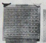
A new line of Multi-Universal High-Density wire-wrappable packaging panels, particularly suitable for use in microprocessor and digital-circuit applications, is now available from the maker, Garry Manufacturing Co., of New Brunswick, NJ.
