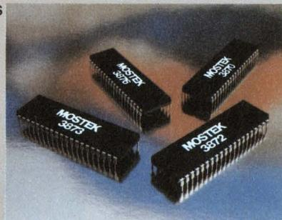
**Coming in '78.** The Mostek 3870 family will continue to grow, giving you the flexibility and expandability required for new applications. The 3873 Serial I/O version will interface to serial devices such as shift registers and CCD memories, and allow implementation of an asynchronous serial I/O port making low cost multi-processing
