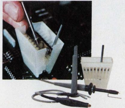
And here's something NEW for scopes. HP's **Easy-IC Probes**. A new idea for probing high-density IC circuits that eliminates shorting hazards, simplifies probe connection to DIP's and generally speeds IC trouble-shooting. The probes are standard equipment with this scope.
