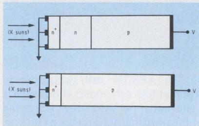
**A high-efficiency solar cell** (top) has an additional layer of n-type material between the n<sup>+</sup> and p-type layers of the normal solar cell. The extra layer acts as a shunt for electrons flowing toward the left-hand electrodes.
