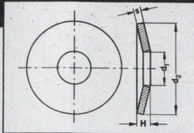
No other locking washer design can hold preloads with the security of the conical Schnorr principle.
