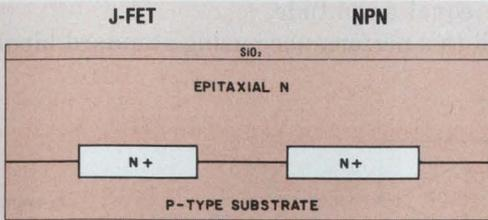
To start, n<sup>+</sup> is diffused into the substrate's n-type epitaxial layer:
