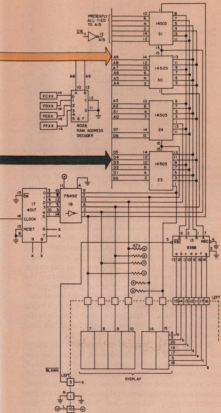
3. Thirty chips and a few other components are all that's needed to build a complete ROM emulator, or development system for a microprocessor.
