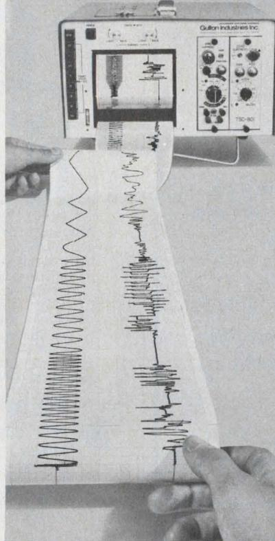
There's more to Gulton's portable oscillographic recorders than clear, easy-to-read tracings. For example, our thermal writing styli eliminate the need for priming, refilling and changing of pen cartridges. And there's never a smear, skip or puddle on your chart.
