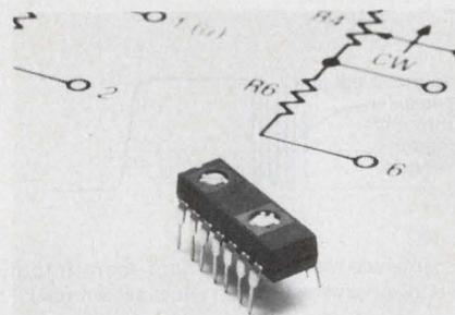
7105A offers one single-turn trimmer with one series-fixed resistor in a 6-pin DIP. Model 7107C is designed for op-amp gain-trim applications. It consists of one single-turn trimmer with two series fixed resistors and one discrete fixed resistor in a 14-pin DIP.
