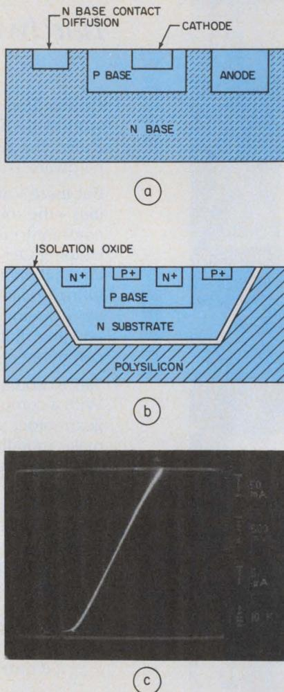
**1. Conventional planar SCRs** (a) aren't suitable for ICs. Harris' dielectric isolation prevents diffused SCRs from interacting with the substrate (b). A DI SCR's forward voltage with both gates floating is fairly linear when plotted vs current (c).
