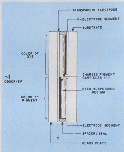
**A small voltage change** on electrode segments changes the colors observed in an electrophoretic display by moving charged pigment particles forward and backward in the display.
