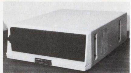
**A dual floppy-disc system** with on-line storage of a half-million 8-bit bytes, the Motorola EXORDisk II will be a component of M6800 systems tailored for small-business needs.
