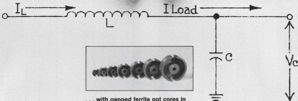
... with gapped ferrite pot cores in 3C8 material from The Cube
