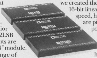
But we didn't stop there. For similar performance in a low cost 16-bit DAC we created the DAC1136 with true 16-bit linearity. Both our high speed, high resolution DAC's are pin compatible with our popular QM Series.
