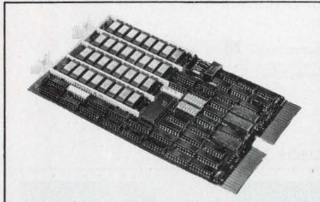
**MINI/BUS® HELPS PACKAGE** up to 32K words on a single high density add-in expansion memory. Low cost, low-inductance, high-capacitance bus bars can solve your printed circuit space problems and shorten assembly time while reducing and isolating noise. Call or write Rogers Corporation, Chandler, AZ 85224. Phone: (602) 963-4584. (EUROPE: Mektron NV, Gent, Belgium; JAPAN: Nippon Mektron, Tokyo.)
