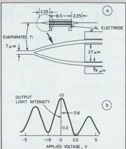
170 Å thick, is formed by evaporation. The film is then diffused in air at 990 F for 4.5 hours to form a waveguide that branches into two parallel waveguides. These guides are then recombined into a single waveguide. Aluminum electrodes are formed on the parallel portion of the waveguide.
