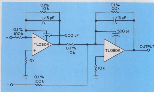
2. This instrumentation amplifier handles  $\pm 100$  V of common-mode signal. Also, the BIFETs provide a power bandwidth of 1 MHz at a gain of 10, plus the BIFET specialty—an input impedance of 10<sup>12</sup>  $\Omega$ .
