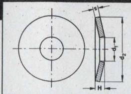
No other locking washer design can hold preloads with the security of the conical Schnorr principle.
