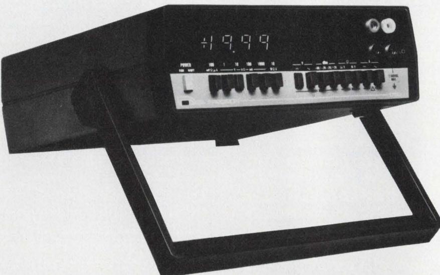
**More features for the dollar** is the trend in digital multimeters like this Data Precision 1750. For \$279, it includes dB scales, true-rms response, and 0.1% basic dc accuracy.
