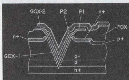
**2. The EPROM cell** (photomicrograph at top, schematic at bottom) is a short-channel VMOS device crossed by the word line, P2, and the n+bitline.
