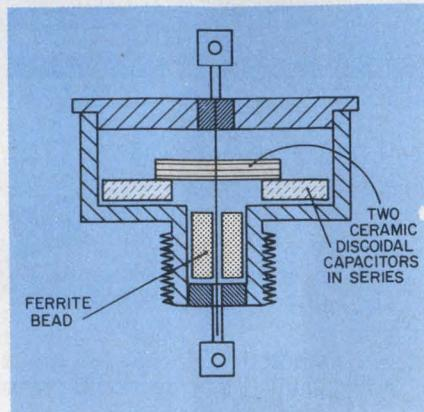
a dc resistance of less than 6 mΩ. The filter can have a 0.375-in. diameter and is fitted with a 1/4-28 threaded mounting stud.
