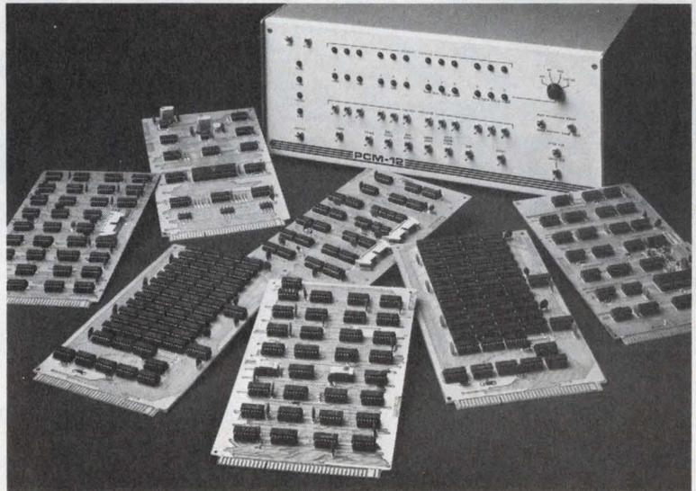
Low-cost PCM microcomputer modules offer full TTL bus compatibility, a variety of static and non-volatile memory modules expandable to 32K words, and a wide selection of I/O interfaces. Ask for complete product information.
