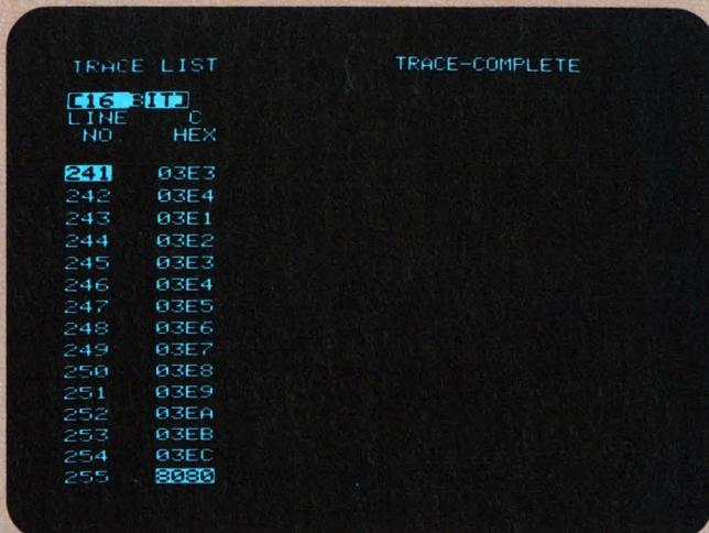
**Observing state display** shows address flow at the moment the glitch occurs and reveals that the I/O port address 8080 always occurs at the same time. This would lead you to observe I/O related signals for transitions occurring simultaneously with the glitch.
