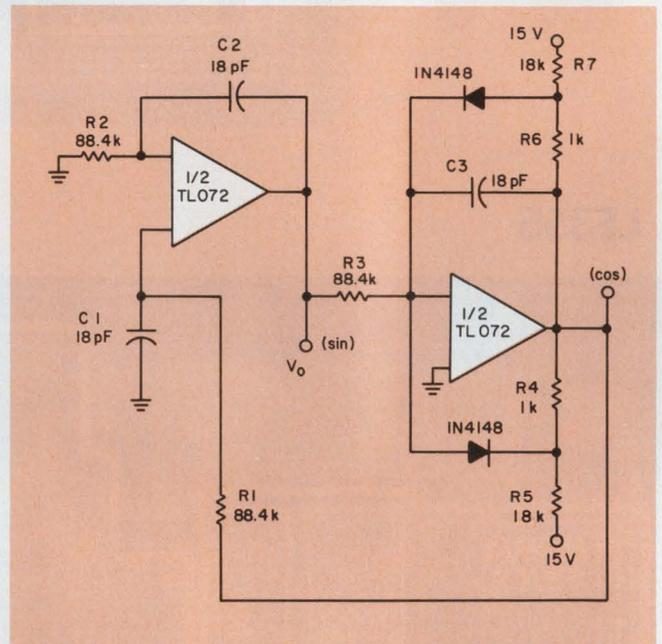
5. Stable operation at 100 kHz from this precision quadrature oscillator is due to the BIFETs. Only R<sub>5</sub> and R<sub>7</sub> must be trimmed for a symmetrical output.
