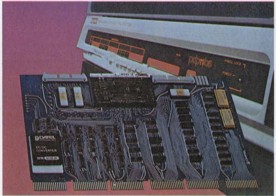
**Analog-to-digital and digital-to-analog acquisition-system interface boards** are appearing with new features. This Datel ST-PDP, which plugs into PDP-11 hardware, is supplied with diagnostic prototype software to speed use.
