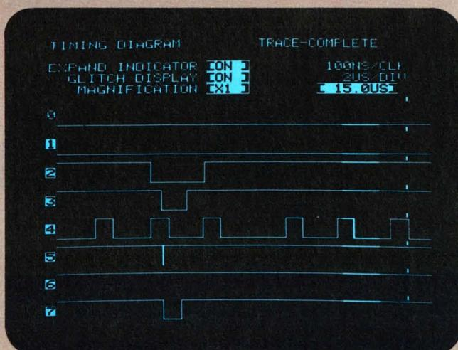
**Observing timing display** of signals on I/O and one-shot shows that the glitch on the input to the one shot (channel 5) occurs four machine cycles before the trigger point and is coincident with the transition on I/O read (line 3) indicating possible capacitive coupling.
