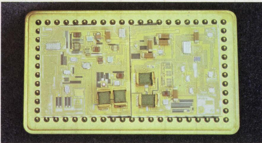
**Hybrid-circuit complexity** continues to amaze—entire data-acquisition systems now come in one or two packages. The Datal Systems HDAS-16 measures only  $2.3 \times 1.4 \times 0.24$  in., yet holds sixteen 12-bit data channels.
