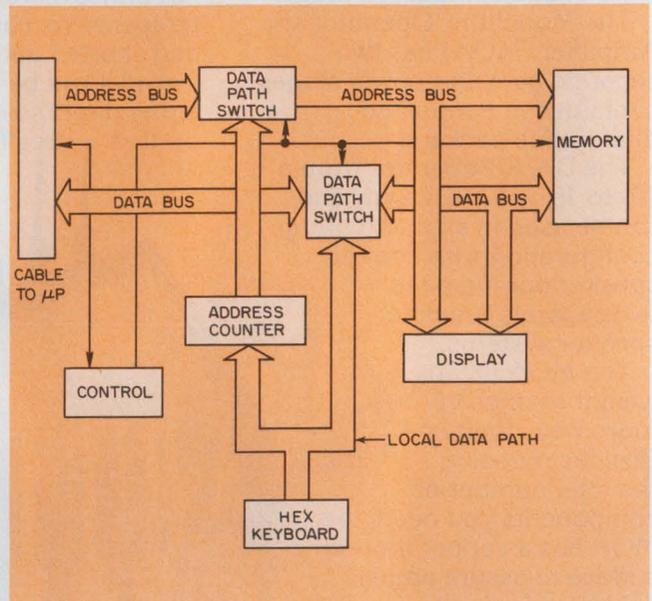
1. A simple microprocessor development system can be built quickly and inexpensively. The memory connects either to an internal keyboard or to an external  $\mu$ P. In either mode, the information on the address and data buses is displayed on a simple, calculator-like display.
