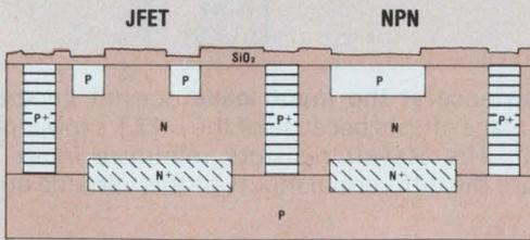
Next, p-type diffusion forms the JFET drains and sources as well as the bipolar bases:
