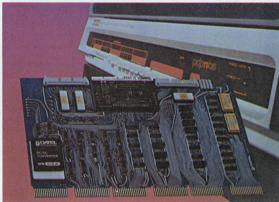
Analog-to-digital and digital-to-analog acquisition-system interface boards are appearing with new features. This Datel ST-PDP, which plugs into PDP-11 hardware, is supplied with diagnostic prototype software to speed use.
