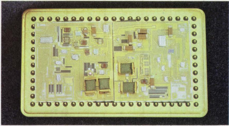
**Hybrid-circuit complexity** continues to amaze—entire data-acquisition systems now come in one or two packages. The Datel Systems HDAS-16 measures only  $2.3 \times 1.4 \times 0.24$  in., yet holds sixteen 12-bit data channels.
