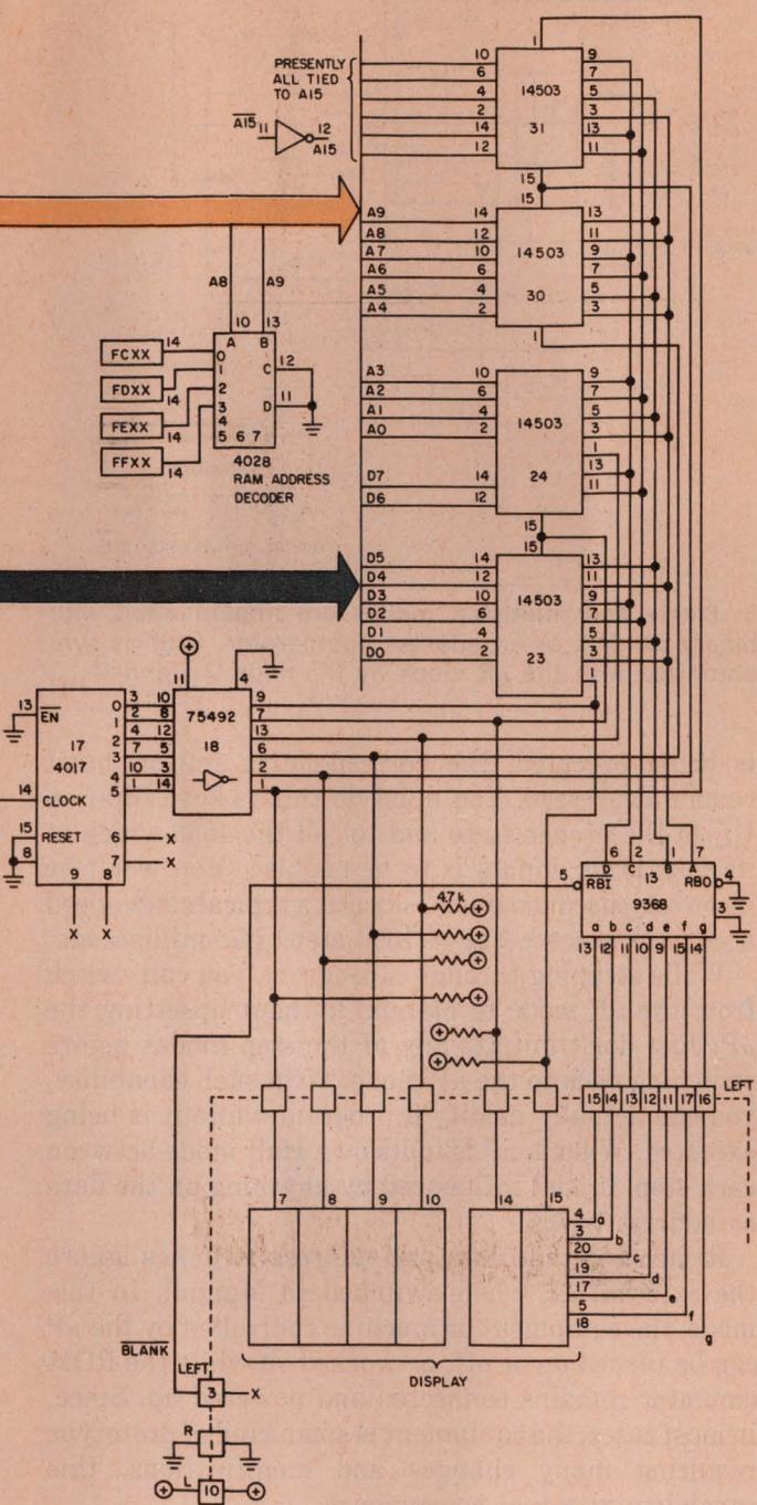
3. Thirty chips and a few other components are all that's needed to build a complete ROM emulator, or development system for a microprocessor.
