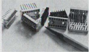
The new sockets have an ultra-low profile, for the most compact packaging of components.
