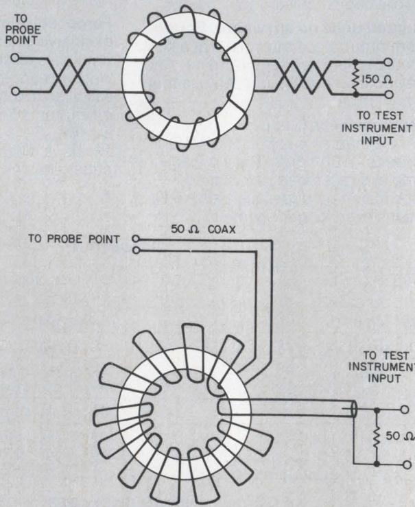
**Ferrite-cored baluns can eliminate common-mode interference signals** when ahead of test probes in unbalanced-input test instruments.
