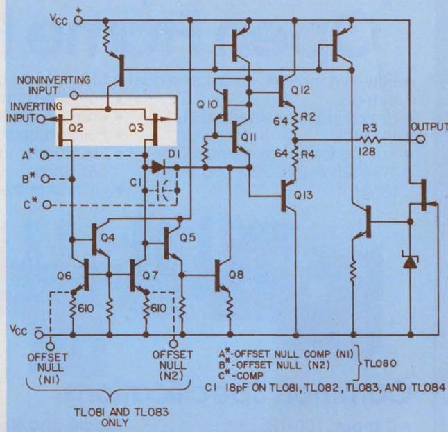
drives the output stage consisting of bias transistors  $Q_{10}$  and  $Q_{11}$  and output drivers  $Q_{12}$  and  $Q_{13}$ .
