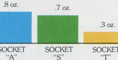
\* In "Fat-Skinny test," withdrawal forces are measured using the smallest size (.008") lead **after** insertion of largest size (.012") lead.
