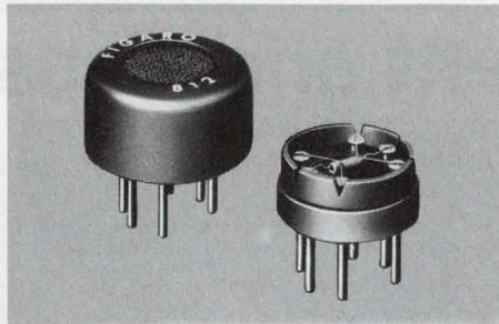
FIGARO GAS SENSOR TGS is a gas sensitive semiconductor. When combustible gas is absorbed on the sensor surface, a marked decrease of electrical resistance occurs. Major features of the sensor include high sensitivity, long term reliability and low cost. The applications are: GAS-LEAK ALARM, AUTOMATIC FAN CONTROL, FIRE ALARM, ALCOHOL DETECTOR, etc. Figaro Engineering Inc., North America Office-3303 Habor Boulevard, Suite D-8, Costa Mesa, Calif. 92626 Tel: (714) 751-4103 Telex: 678396
