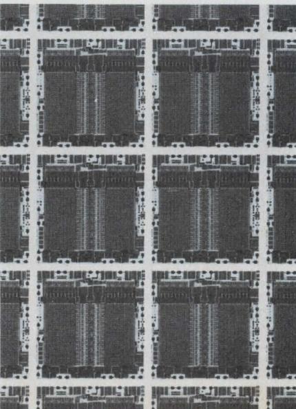
**Silicon-on-sapphire products,** such as this memory circuit from RCA, promise to keep speeds high without increasing power requirements.
