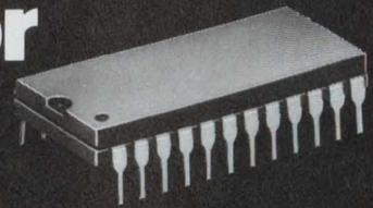
The Ferranti Model ZN1066E Pulse Width Modulator for use in:
