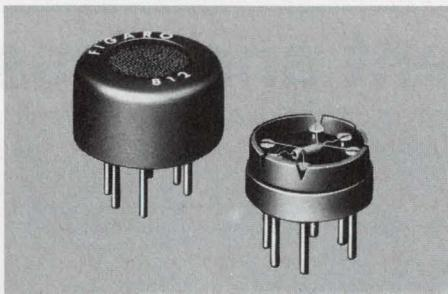
**FIGARO GAS SENSOR TGS** is a gas sensitive semiconductor. When combustible gas is absorbed on the sensor surface, a marked decrease of electrical resistance occurs. Major features of the sensor include high sensitivity, long term reliability and low cost. The applications are: GAS-LEAK ALARM, AUTOMATIC FAN CONTROL, FIRE ALARM, ALCOHOL DETECTOR, etc. Figaro Engineering Inc., North America Office-3303 Harbor Boulevard, Suite D-8, Costa Mesa, Calif. 92626 Tel: (714) 751-4103 Telex: 678396
