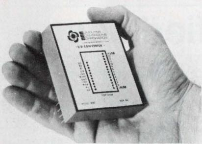
**Synchro to digital converters** - 10, 12, or 14 bit output, errorless tracking up to 4 r.p.s., accuracy  $\pm 4$  min. of arc  $\pm .9$  LSB, resolution - 1.3 minutes, 60 or 400 Hz input, Module 2.6 x 3.1 x .82" H, Price From \$350 in qty. Other CCC products are Synchro to BCD or DC, Digital or DC to Synchro Converters, Solid State C.T.'s or CDX's, and Absolute Encoders. Send for Free Catalog & Application Notes. Computer Conversions Corp., East Northport, NY 11731 (516) 261-3300.
