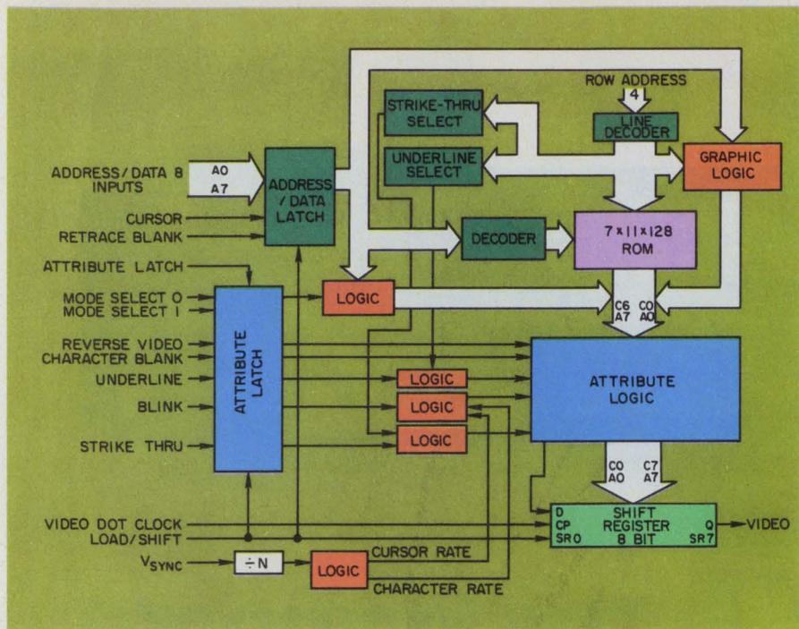
**Capable of performing the attribute control and character generation** for a CRT terminal, the CRT8002 developed by Standard Microsystems, further reduces the complex circuitry necessary to build a terminal.
