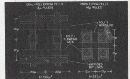
**4. A VMOS EPROM cell** (right) takes less than half the area needed by a conventional NMOS dual-polysilicon EPROM cell (left).
