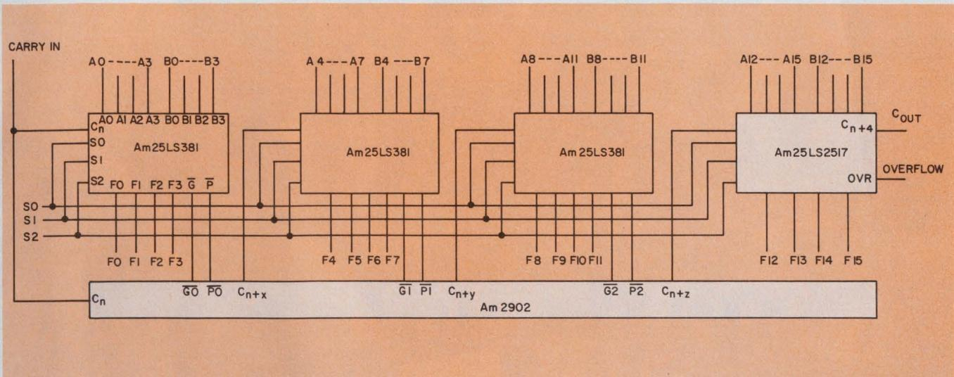
**6. High-speed arithmetic is achieved** by using a lookahead carry generator such as the Am2902 with arithmetic
