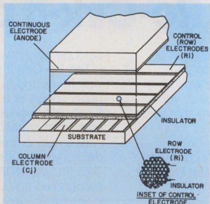
**A switching point** from one color to another is established by adding a control electrode so that each element is either on or off, not in between.
