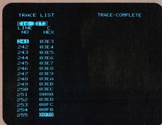
**Trigger on state.** The interrupt vector (0030) can be used as the trigger point to observe address flow prior to the false interrupt. Evaluation shows that the I/O port address 8080 always appears four machine cycles prior to the interrupt vector.
