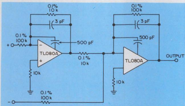
2. This instrumentation amplifier handles  $\pm 100$  V of common-mode signal. Also, the BIFETs provide a power bandwidth of 1 MHz at a gain of 10, plus the BIFET specialty—an input impedance of 10<sup>12</sup>  $\Omega$ .
