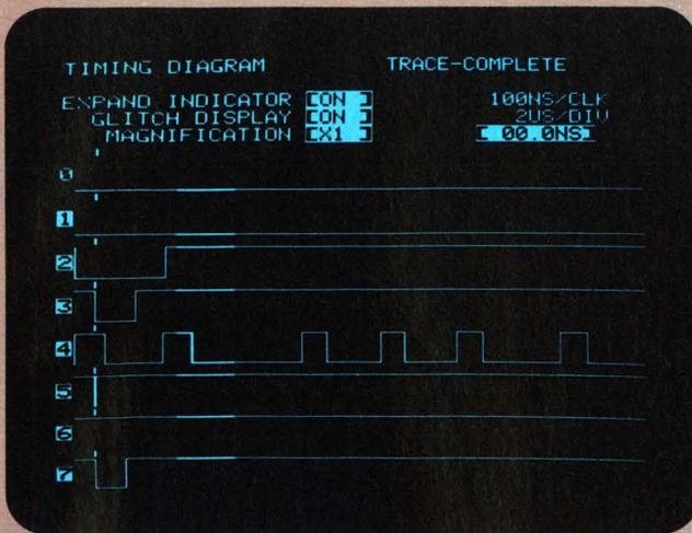
**Trigger on glitches.** A glitch on an input to a one shot (channel 5) is causing a false interrupt (channel 7). This glitch (which is intensified to distinguish it from data) can be used to trigger state as well as time displays.
