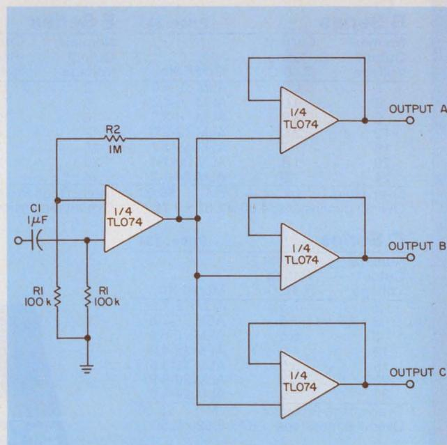
6. Process audio signals with 100-k $\Omega$  input impedance plus low distortion and noise over the full audio bandwidth, with only one BIFET quad.
