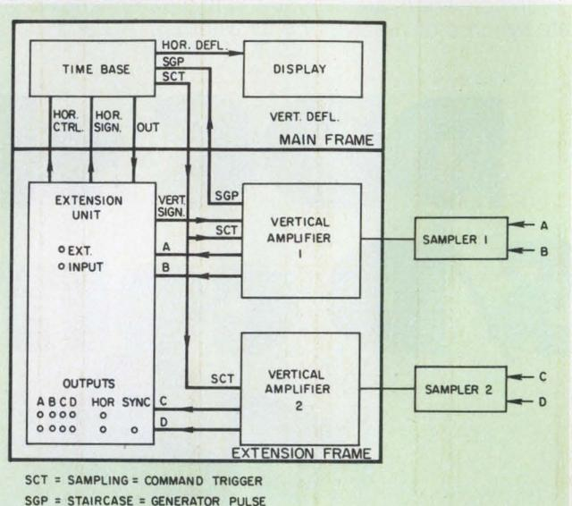
**1. Four channels of sampling** require two vertical input amplifiers. The extension unit contains the channel logic, control signals and output amplifiers.
