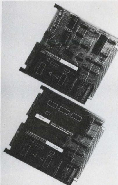
**Boards for the Zilog Z-80  $\mu$ C** are based on Data Translation's DATAX modules and feature analog I/O and analog-input systems.
