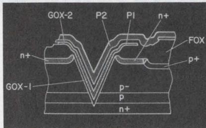
**2. The EPROM cell** (photomicrograph at top, schematic at bottom) is a short-channel VMOS device crossed by the word line, P2, and the n<sup>+</sup> bit line.
