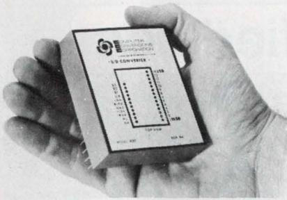
"Synchro to digital converters - 10, 12, or 14 bit output, errorless tracking up to 4 r.p.s., accuracy  $\pm 4$  min. of arc  $\pm .9$ LSB, resolution - 1.3 minutes, 60 or 400 Hz input, Module 2.6 x 3.1 x .82" H, Price From \$350 in qty. Other CCC products are Synchro to BCD or DC, Digital or DC to Synchro Converters, Solid State C.T.'s or CDX's, and Absolute Encoders. Send for Free Catalog & Application Notes. Computer Conversions Corp., East Northport, NY 11731 (515) 261-3300.
