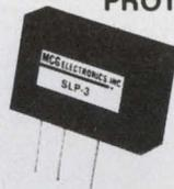
The SLP protectors were expressly designed to protect signal/data/telephone lines from transient overvoltages caused by lightning, heavy machinery, elevator motors, generators, etc. The SLP interfaces between the signal lines and the sensitive circuit to provide a sophisticated blend of high speed (nanoseconds) voltage limiting and brute force protection. The SLP's recoverer automatically to standby when the need for protection has passed.
