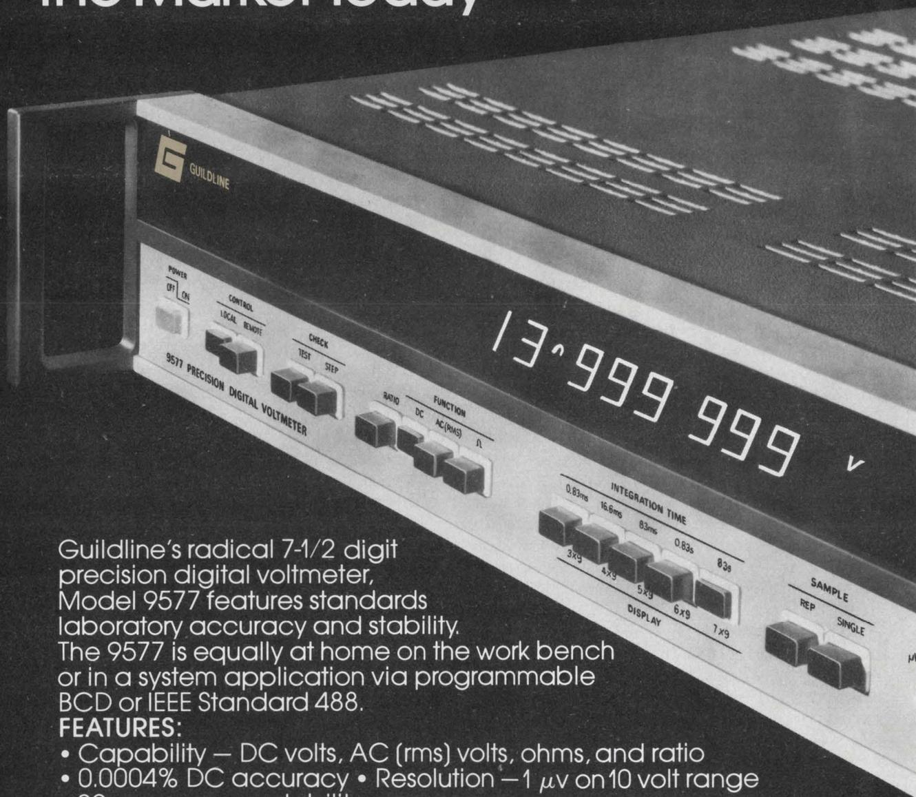
Guildline's radical 7-1/2 digit precision digital voltmeter, Model 9577 features standards laboratory accuracy and stability. The 9577 is equally at home on the work bench or in a system application via programmable BCD or IEEE Standard 488.
