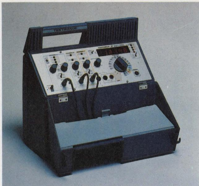
Temperature scales and an auxiliary hand probe permit the designer to measure device or component temperatures from  $-55$  to  $150$  C or F with this Tektronix 851 digital tester.
