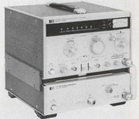
New HF down converter now covers test applications in the 10 kHz to 11 MHz band.
