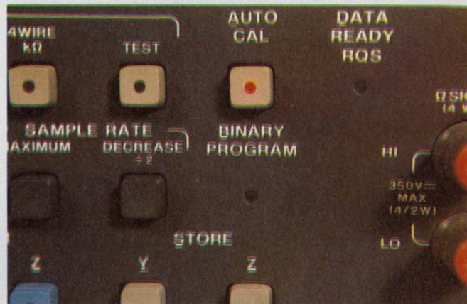
Self-calibration in a smart DMM consists of removing a reference module (top), adjusting the ohms and dc V functions, and replacing the module. You then hit the auto cal button (bottom), and the unit quickly corrects itself.
