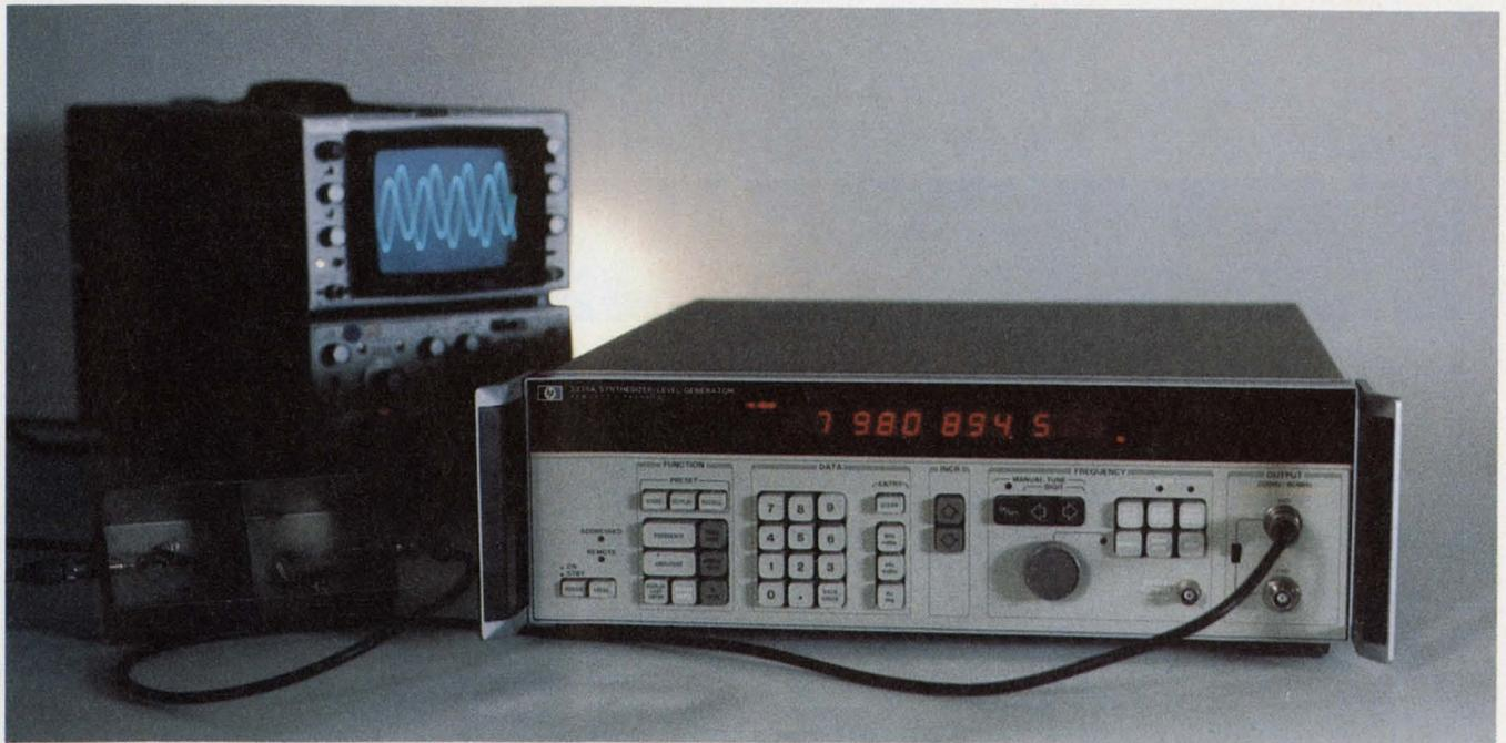
**Frequency and amplitude in an HP 3335A** are controlled by a microprocessor. Ten front-panel settings can be stored and recalled from the internal memory. A 200-Hz
