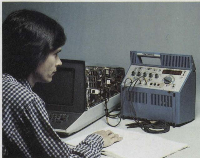
**Diagnostic decisions:** After the Tektronix 851 tests other equipment, it can help test itself. Just plug in the probes, step through the function switch and read the display.
