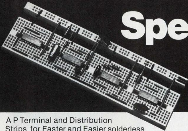
A P Terminal and Distribution Strips for Faster and Easier solderless circuit building and testing. No special patch cords are required, and any solid wire up to No. 20 AWG can be used for connection. Strips accept all components with leads up to .032" diameter, and hardware and mounting templates are provided with every strip. Terminals are non-corrosive nickel/silver.
