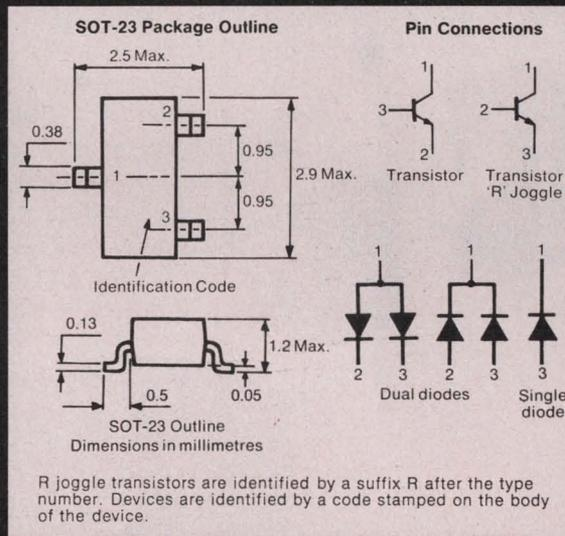
R joggle transistors are identified by a suffix R after the type number. Devices are identified by a code stamped on the body of the device.
