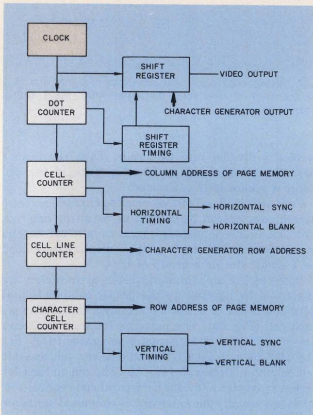
4. **Inside the sync generator** many counters are used to generate all the various timing signals and provide the addresses for the RAM where the displayed data are temporarily stored.
