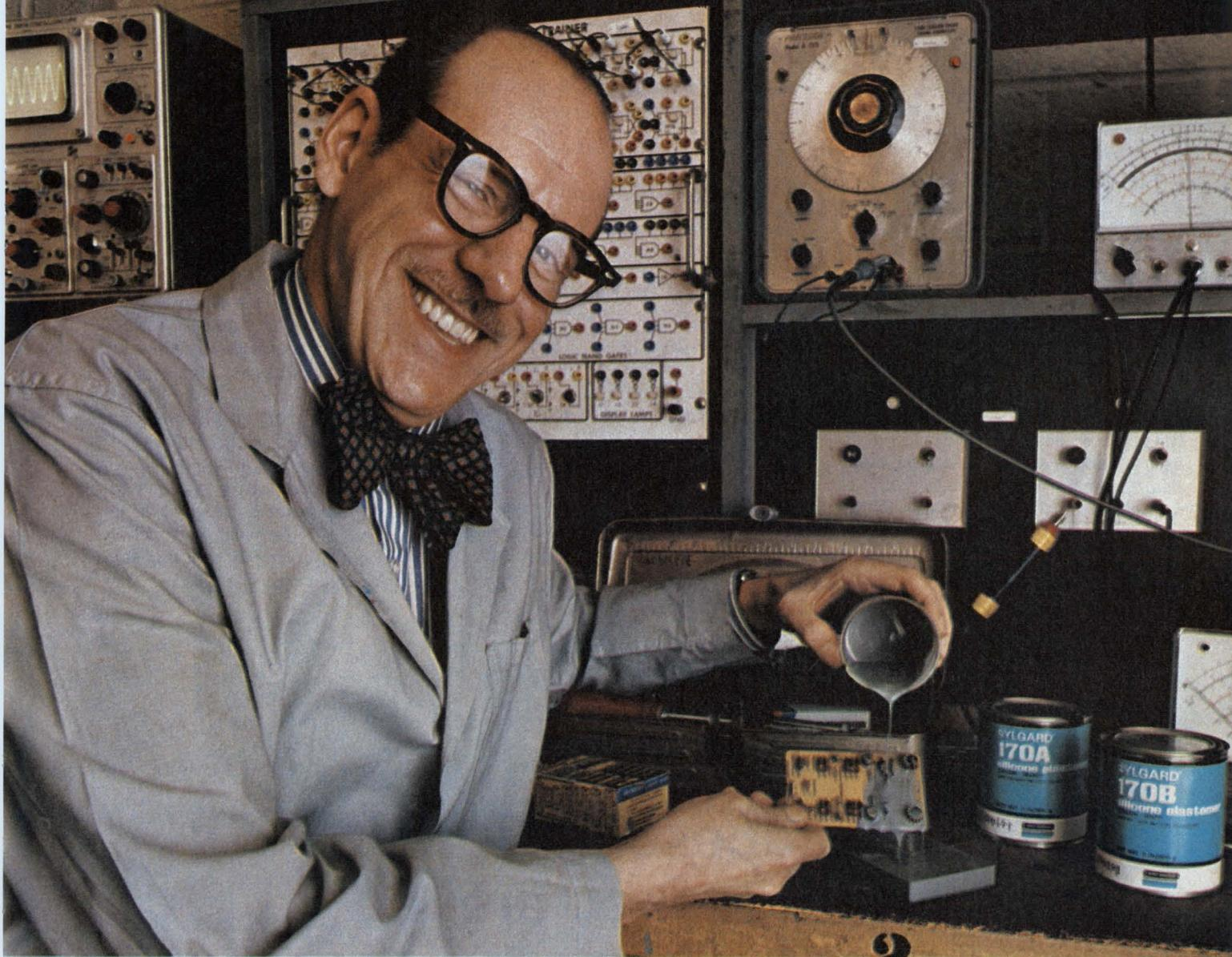
Now there's an all-purpose encapsulant that gives you silicone performance at the price of organics. Dow Corning Sylgard® 170 A&B silicone elastomer. A two-part liquid encapsulant that cures at room temperature or can be heat accelerated to increase production rates.
