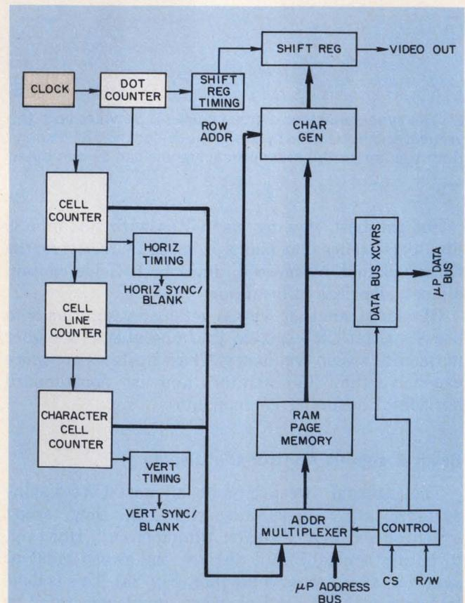
5. **A video RAM circuit** combines the sync generator with all the counting circuits, the character generator and the necessary memory pages to form an almost complete video display system.
