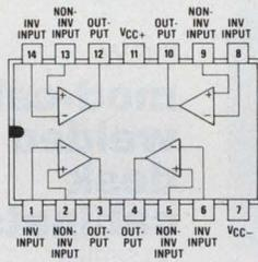
Compensated with RC4136 pinout.
