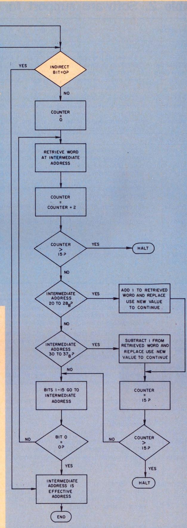
4. To calculate the effective address, the microNova goes through a very complex procedure. The first step in the process is to check the two index bits so that the processor knows what to do with the displacement bits in the instruction before performing the calculation.
