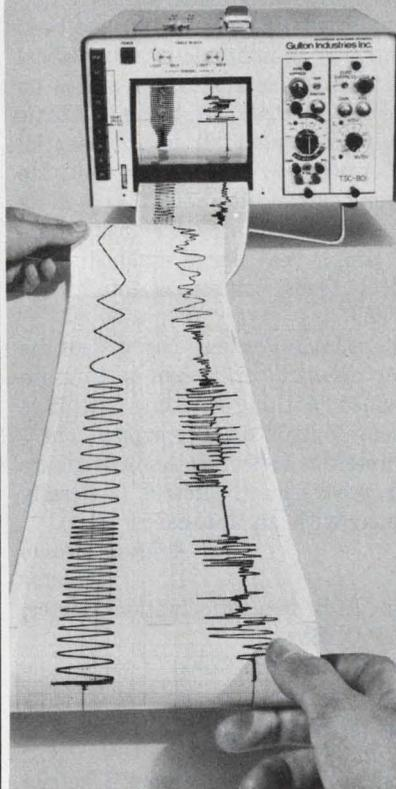
There's more to Gulston's portable oscillographic recorders than clear, easy-to-read tracings. For example, our thermal writing styli eliminate the need for priming, refilling and changing of pen cartridges. And there's never a smear, skip or puddle on your chart.
