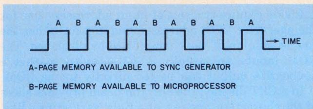
8. To control the timing all that's needed is a single-phase clock. When High it lets the sync generator feed into the multiplexer. When Low, it lets the processor control the display memory through the multiplexer.
