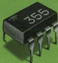
When the output of a 555 timer switches high, a large current spike is generated which can drag down your power supply and upset your flip-flops. One way to cure it is with several hundred  $\mu\text{F}$  of capacitance. But that's awkward and space-consuming. Teledyne's new 355 timer is a better way.
