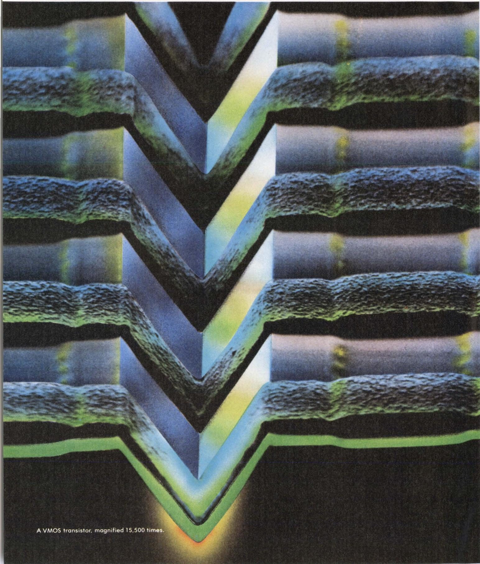
A VMOS transistor, magnified 15,500 times.
