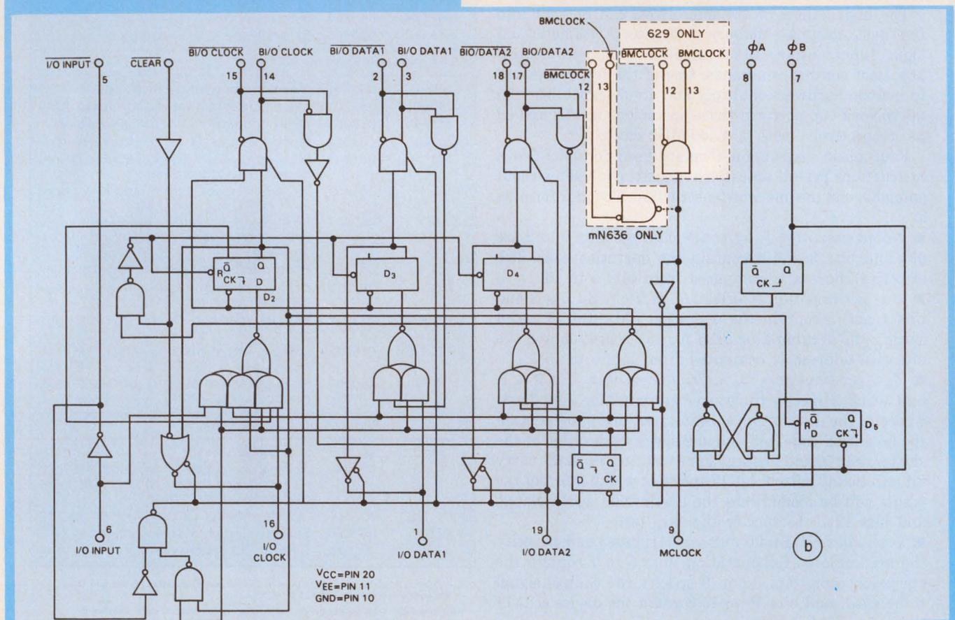
7. Designed to buffer clock and data signals, the mN629 and 636 transceivers are used for I/O expansion. One 629
