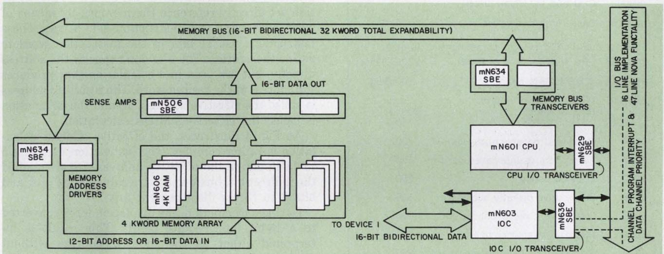
2. There are three major buses on the processor—the memory bus, the serial I/O bus and the control bus. And
