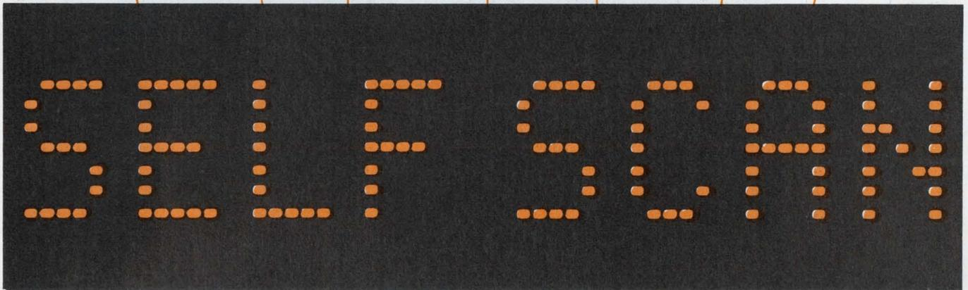
The new Burroughs SELF-SCAN® II single register gas plasma panels are breakthroughs in visibility and readability, making them ideal for all types of applications — from audience information displays to instrumentation applications. They are digitally addressed to interface easily with microprocessors and computers.
