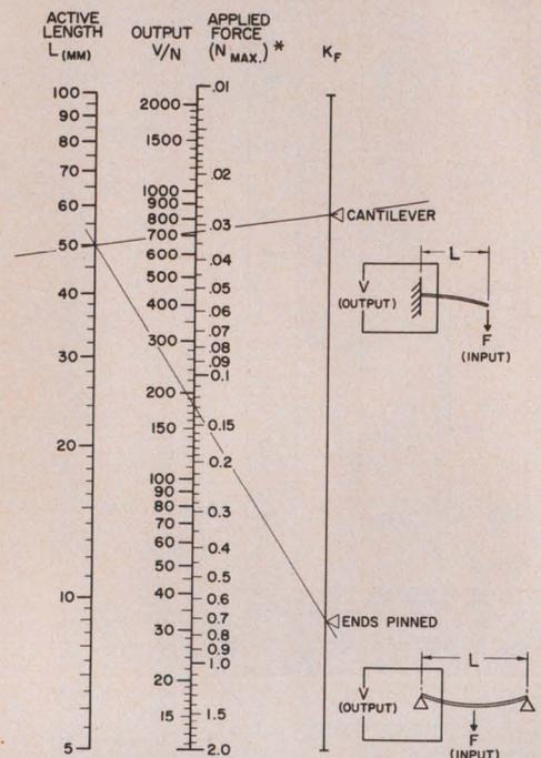
THE OPEN CIRCUIT OUTPUT VOLTAGE DERIVED FROM THE NOMOGRAPH ASSUMES THE MULTIMORPHS OVERALL AND ACTIVE LENGTH TO BE IDENTICAL AND CAN BE USED TO GOOD APPROXIMATION. HOWEVER, VIEWING THE MULTIMORPH UNDER ACTUAL OPERATING CONDITIONS, THE OVERALL LENGTH EXCEEDS THE ACTIVE LENGTH AND THE OUTPUT VOLTAGE MAY BE CALCULATED TO A CLOSER APPROXIMATION BY FIRST CALCULATING THE CHARGE (OUTPUT/APPLIED FORCE):  $(q_F) \mu C/N$
