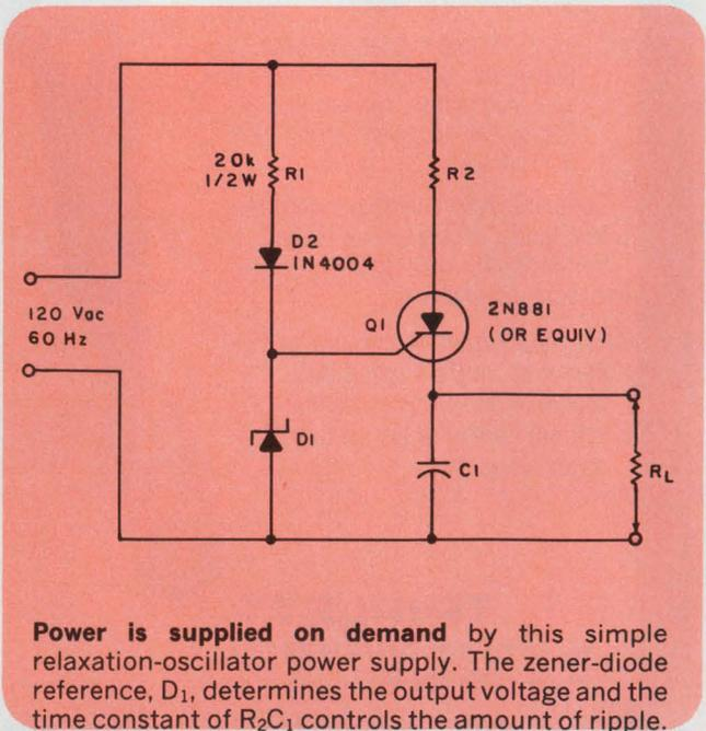
Power is supplied on demand by this simple relaxation-oscillator power supply. The zener-diode reference,  $D_1$ , determines the output voltage and the time constant of  $R_2C_1$  controls the amount of ripple.
