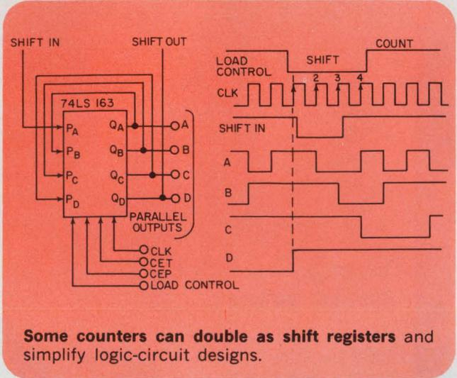
Some counters can double as shift registers and simplify logic-circuit designs.
