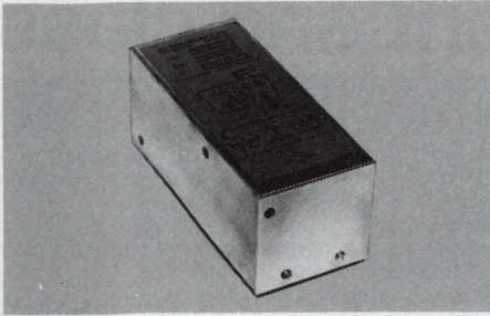
**HIGH PERFORMANCE CRYSTAL OSCILLATOR** This compact, highly stable, rugged oscillator operates over a wide range of temperatures and conditions and features excellent frequency stability (5x10<sup>-10</sup>/day), phase noise (90 db, 1 Hz from carrier), low power consumption, and low cost. The B 1325 oscillator meets performance requirements for modern instruments and systems. Frequency and Time Systems, Inc., 182 Conant Street, Danvers, MA 01923 (617) 777-1255 Telex: 94-0518
