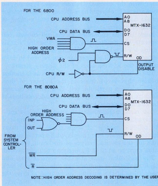
10. Connecting the video RAM to either the 8080A or 6800 is easily done with some gates and the  $\mu$ P's read/write line. The video RAM can be located anywhere in the computer's memory space and is, in fact, addressable just like any random-access memory.
