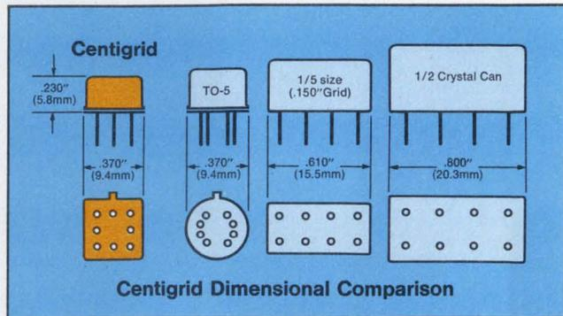
Out of Teledyne's TO-5 relay technology has evolved the Centigrad® — the ultimate subminiature relay. It combines the proven TO-5 relay design concept and internal construction into an even more compact package. Low profile height — just .230" (5.84mm) — with terminals spaced on a .100" (2.54mm) grid permitting direct pc board mounting without the need for lead spreading.
