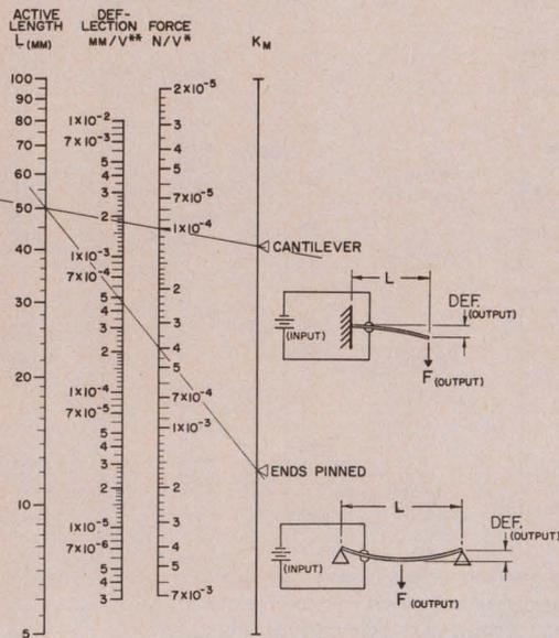
for an active length of 50 mm with a cantilevered configuration, you can obtain a deflection of  $1.8 \times 10^{-3}$  mm/V. With a supply voltage of 20 V applied to the outer electrodes a deflection of 0.04 mm (0.0015 in.) can be obtained. Higher drive levels can produce larger displacements, and nonlinear effects tend to increase the displacement.
