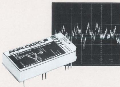
Check that scope photo. It's the output of our MP221 ultra-low-noise, ultra-low-drift chopper amplifier, the best in its class by *at least* an order of magnitude. What's really impressive about that photo is that it was taken at a gain of 1000, and with a 10 kHz bandwidth... a "tell-it-all" test that other amplifiers costing far more will flunk miserably!
