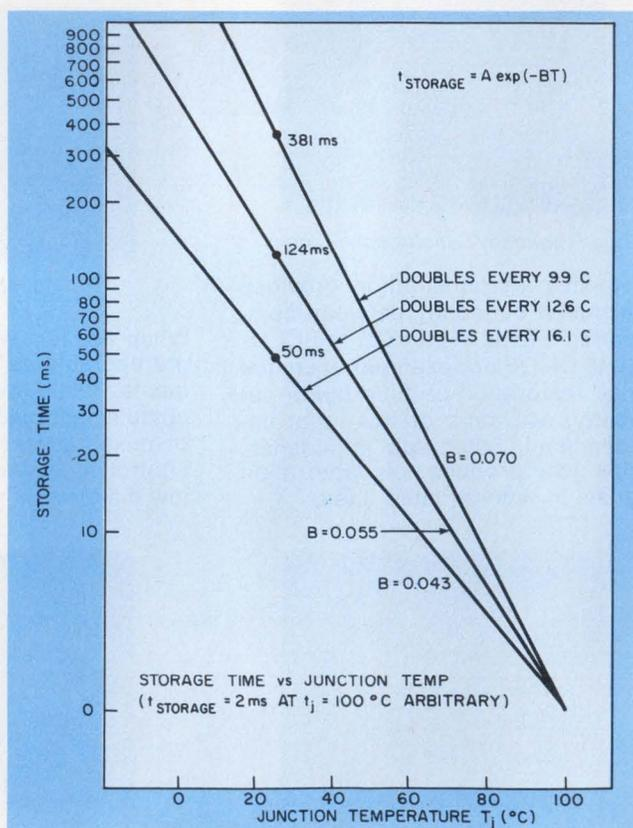
1. Storage time doesn't necessarily double for every 10-C decrease in junction temperature, as the "conventional wisdom" states. Setting the correct refresh intervals during testing requires an accurate knowledge of the minimum storage time for the memory.
