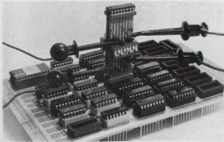
**Dual-In-Line TEST/MODIFICATION Fixture** Simplifies testing and provides a means for nondestructive circuit modification. DIP switches provide a means of isolating each circuit lead, test points are provided on both sides of the switches for testing or circuit modification. High rel components are used through out. 14 pin \$21.95, 16 pin \$22.95, 24 pin \$28.95, 40 pin \$40.95. Other sizes quoted on request. EMD Co., 7891 Camp Chaffee Rd., Ventura, CA 93001. 805-649-1513.
