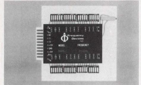
**PROGRAMMABLE ACTIVE FILTERS** provide a convenient breadboarding tool for designers. Series 744/FC102 are 4 pole lowpass filters with cutoff frequency ( $F_c$ ) that can be varied over a 500:1 tuning range in 0.2% increments via self contained programming switches. Ten models cover the frequency range from 0.1 Hz to 50 kHz with Butterworth and Bessel transfer functions. Frequency Devices, Inc., 25 Locust Street, Haverhill, MA 01830. (617) 374-0761.
