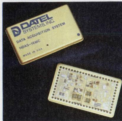
**For the engineer who builds his own boards,** Datel's new HDAS-16 packs 16 channels of 12-bit conversion in a tiny hybrid IC measuring only 2.3 × 1.4 × 0.24 in.
