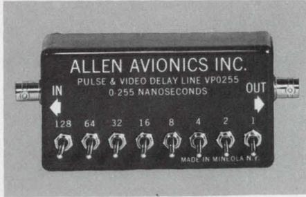
**TV STUDIOS & VIDEO INDUSTRY** New Allen Avionics Video & Pulse Delay Lines replace 75 ohm coaxial cable, provide a more suitable method of achieving precise short delays. The units reduce size, weight, installation cost, and save time and effort in making delay changes. Catalog also discusses Video Filters. See us at Wescon, Booth 1122. Allen Avionics, Inc., 224 E. 2nd St., Mineola, N.Y. 11501, 516-248-8080.
