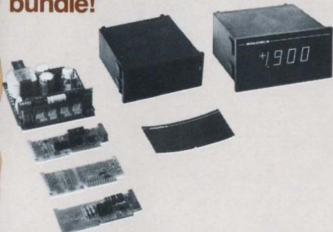
At first glance, the AN2553 is merely another superb Analogic DPI—a digital panel instrument, not a “meter”... but that’s another subject. What’s unique about *this* DPI is that it **comes ready to take apart**—with or without our help—and to be equipped with *optimized* plug-in interface circuitry that lets it measure virtually *anything*, from nanoamperes to Amperes, from microvolts to kilovolts, from degrees F or C to pounds or kilograms... and (literally) *hundreds* of other parameters.
