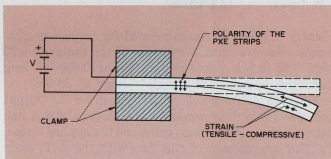
2. The flexure mode, as in this bimorph configuration, is used where larger deflections and smaller forces are involved than are possible with rings or discs.
