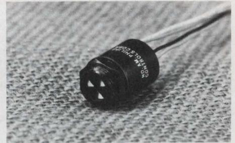
**ELECTRIC RESET "BITE" INDICATOR** Meets M83827/02. Monitors systems or components. Pinpoints malfunctions by providing automatic and permanent (until reset) warning of fault condition. Miniature size. Can be compactly grouped. 3 to 28V dc. 40 ms response. Wire leads or turret terminals. North American Philips Controls Corp., Cheshire, Conn. 06410.
