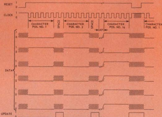
1. The Reset and Update pulses from the timing diagram of this visual-display refresh-memory system are used to synchronize the slow-down circuit for hard-copy readout.
