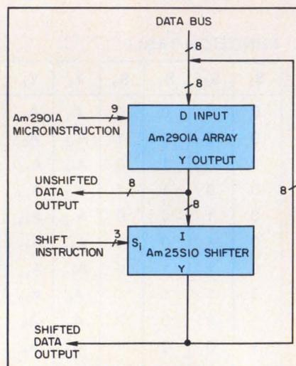
7. Connecting an 8-bit barrel shifter to a 2900-based processor requires that the input lines of the scalers be connected to the output port of the 2901A, and that the output lines of the 25S10 be connected to the data bus/input port of the 2901A.
