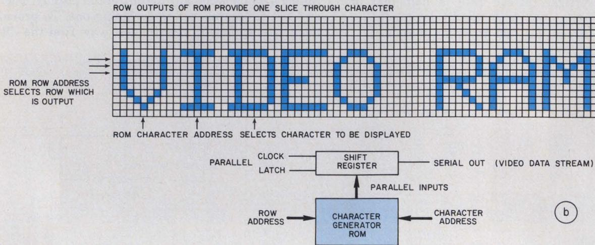
3. **Standard 7x9 and 5x7-dot matrix displays** can be generated from ROM-based data (a). To actually form the
