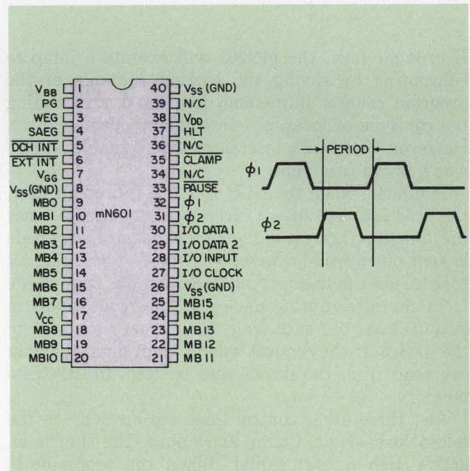
3. Of the 40 pins on the microNova, 16 are required by the memory bus, four are used for the serial I/O, eight for control, seven for power, two for the clock and three more are not connected (a). The two-phase nonoverlapping clock (b) controls all system timing.
