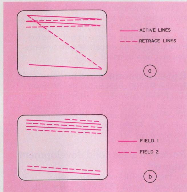
1. Both a non-interlaced video display (a) and an interlaced display (b) generate images on a CRT screen. But, the interlaced display effectively provides double the resolution of the non-interlaced version.
