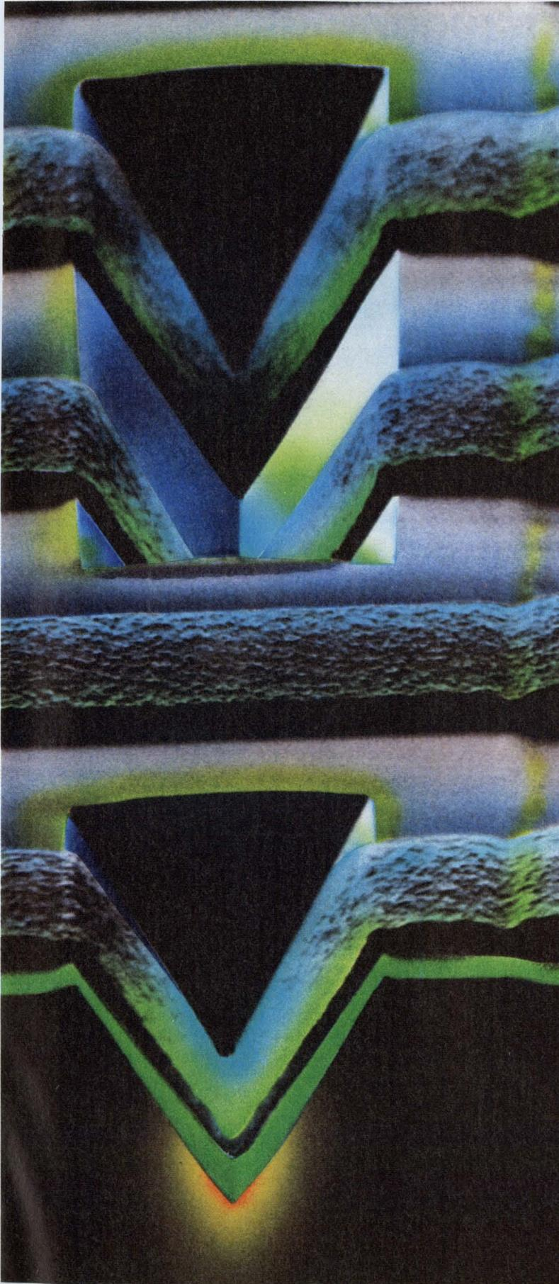
**AMI creates VMOS.** This revolutionary idea revolves around a three-dimensional transistor, etched into the silicon substrate.
