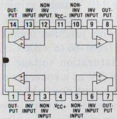
Compensated with LM324 pinout.
