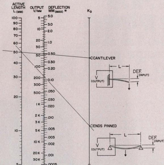
THE OPEN CIRCUIT OUTPUT VOLTAGE DERIVED FROM THE NOMOGRAPH ASSUMES THE MULTIMORPHS OVERALL AND ACTIVE LENGTH TO BE IDENTICAL AND CAN BE USED TO GOOD APPROXIMATION. HOWEVER, VIEWING THE MULTIMORPH UNDER ACTUAL OPERATING CONDITIONS, THE OVERALL LENGTH EXCEEDS THE ACTIVE LENGTH AND THE OUTPUT VOLTAGE MAY BE CALCULATED TO A CLOSER APPROXIMATION BY FIRST CALCULATING THE CHARGE OUTPUT/AMOUNT OF DEFLECTION ( $q_D$ )  $\mu\text{C}/\text{MM}$
