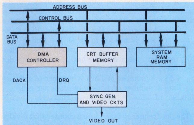
9. By using a DMA interface between the processor and the video display, the main system memory can be constantly updated then transferred to the display's buffer in one operation every time the display wants an update.
