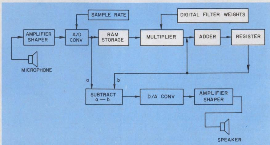
**This digital audio processor is the first to operate in real time.** Since it eliminates the conventional recording step required in other digital audio processors, it can be used in real-time communications systems.
