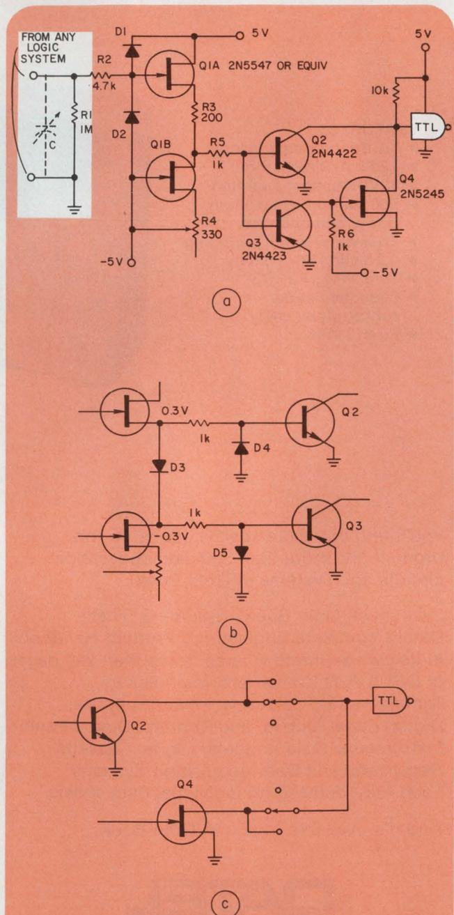
**1. The basic level-converting circuit (a) can couple a wide range of logic families of either voltage polarity to TTL. The 1-to-15-V range of the basic circuit is extended down to 0.4 V with the addition of three diodes (b) and an optional switch can be added to make the circuit polarity-sensitive (c).**
