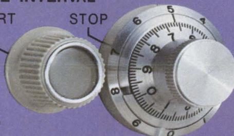
1 You simply set two intensified markers at the desired points using the START and STOP controls.
