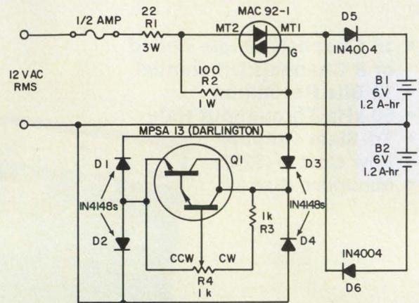
**Battery-charger circuit charges two series-connected batteries independently** with only one voltage-level adjustment,  $R_4$ . Moreover, the circuit's temperature coefficient automatically adjusts for proper charging as the temperature changes.
