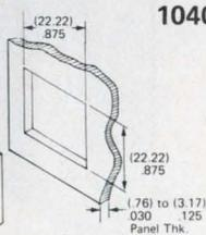
well as a square or pyramidal shaped lens. Recommended panel cutout dimensions include an .875 x .875 (10410 and 10420) and .875 x 1.050 (10400 versions) which are compatible with most comparable switches presently available today. The 10400 with integrally molded mounting ears will accommodate a panel thickness from .030 to .093, while the 10410 and 10420 versions offer a front removable feature from .030 to .125 thick panels. Spade terminals are .02 x .19 x .30 length.
