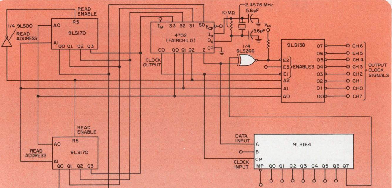
**The addition of an Exclusive-NOR gate and a shift register generates 32 times the final bit rate instead of the usual 16 produced by a programmable baud**
