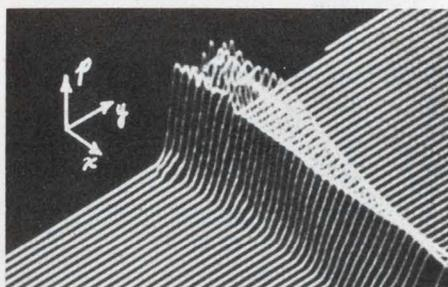
**ELECTRONIC ISOMETRIC PROJECTOR** generates 3D images of data applied to X, Y, Z inputs. Single-wide plug-in fits the Tektronix TM500 system. Image can be rotated, tilted, and magnified with front panel controls for optimum view. Image may be presented on CRT display, recorder, etc. Input and output offset controls are incorporated. Applications include ultrasonic field mapping and imaging, infrared imaging, eddy current testing, scanning electron microscopy. METROTEK, INC. (509) 946-4778
