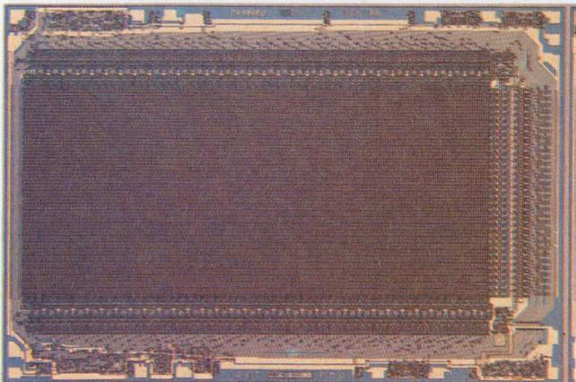
**This colorful dynamic, bipolar RAM** combines the good attributes of bipolar technology (5 V, 280-ns  $t_{cy}$ , 120-ns  $t_{acc}$ ) with low MOS power (350 mW active), and high density (4096  $\times$  1 bits). Fairchild makes this memory with isoplanar integrated injection logic.
