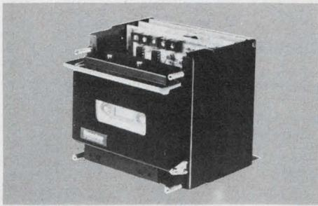
**HIGH SPEED RECORDER FOR MICRO-PROCESSORS** Model 764 has a patented constant speed tape drive using only 2 moving parts. No capstans, tachometers or clock tracks are necessary. Records up to 32,000 bits per second. Searches at 100 inches per second. Can store up to 5 megabits per 300 foot cassette. ANSI/ECMA compatible. Priced under \$500.00/OEM quantities. MEMODYNE CORPORATION, 385 Elliot Street, Newton Upper Falls, MA 02164. Telephone (617) 527-6600.
