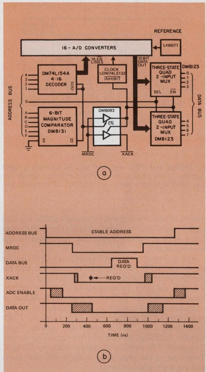
4. A data-ready signal  $\overline{MRDC}$  returns to the 8080  $\mu$ P from the 16-channel parallel-conversion system (a) to prevent extending the Memory Access cycle.  $\overline{MRDC}$  goes out on the XACK line at least 300 ns before it is needed (b).
