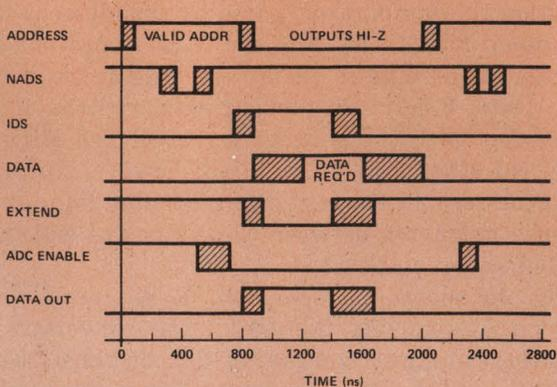
6. The comparator output ANDed with IDS enables the three-state output buffers and inhibits the clock in the 16-channel, 12-bit, parallel-conversion system for the PACE (a). Data are put on the PACE's Data/Address bus about 500 ns after the IDS signal comes up.
