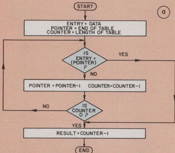
For example, if the data is 6D, the program would search through the memory starting in location 1009 (see Figure 2) and ending when it finds the code in location 1005. The backward search is convenient since the counter is always one more than the index.
