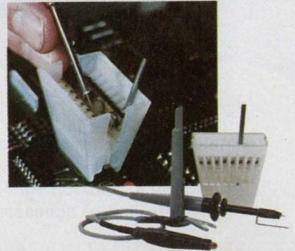
And here's something NEW for scopes. HP's **Easy-IC Probes**. A new idea for probing high-density IC circuits that eliminates shorting hazards, simplifies probe connection to DIPs and generally speeds IC troubleshooting. The probes are standard equipment with these two scopes.
