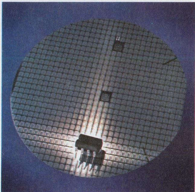
**Nonvolatile semiconductor memories don't forget** after the power is off. Nitron's 256-bit electrically alterable, read-only memory (EAROM) retains data for a year. Serial data input and output keep pin count low.
