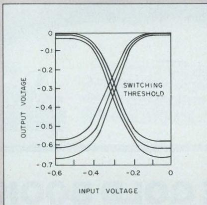
2. Switching curves for the BCL logic-gate inverter
