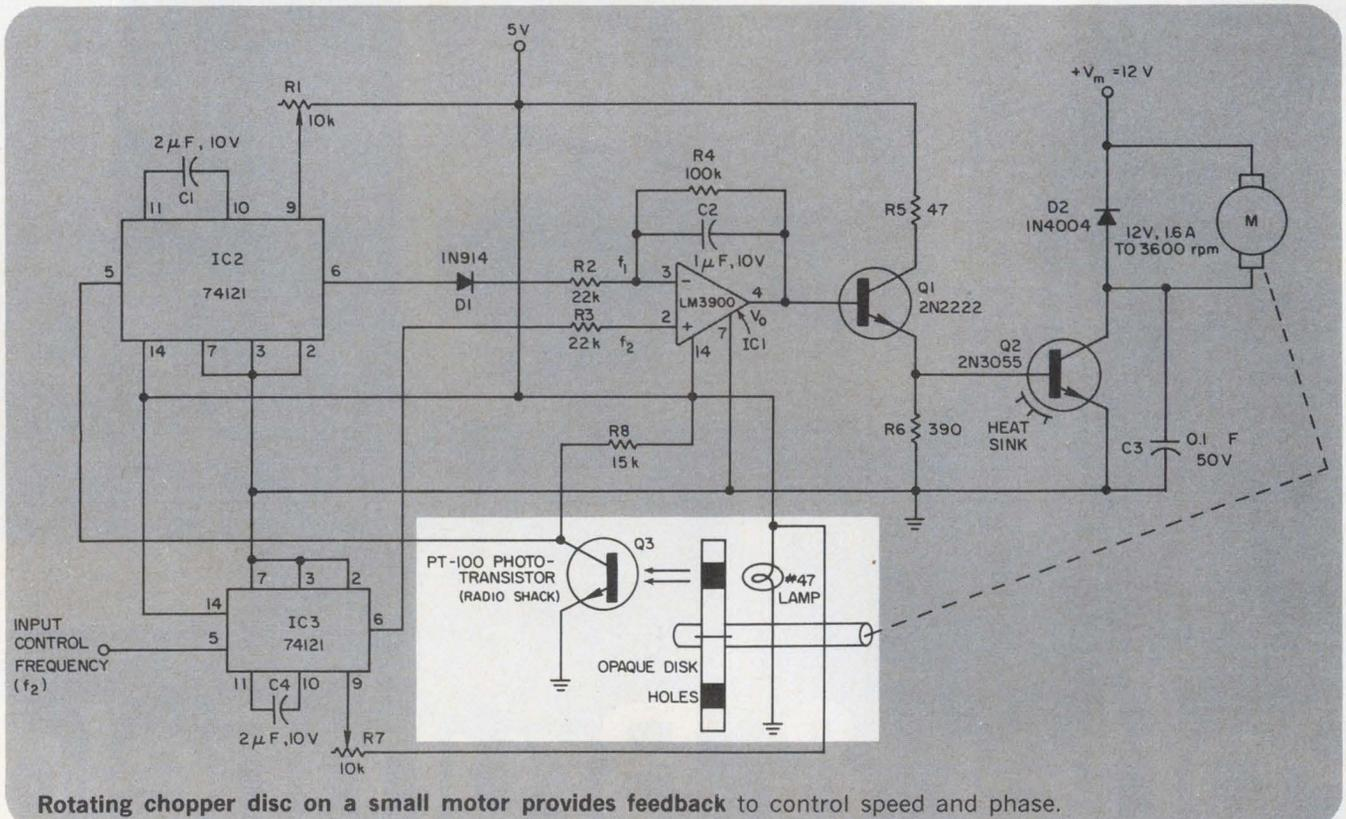
Rotating chopper disc on a small motor provides feedback to control speed and phase.
