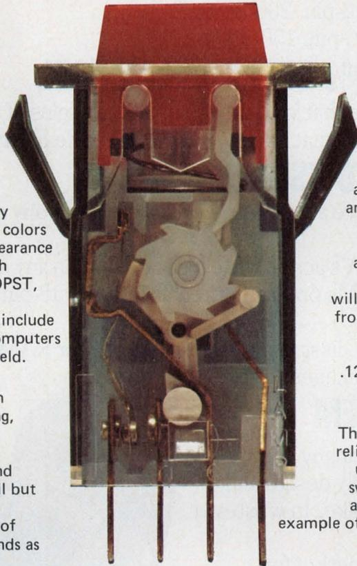
well as a square or pyramidal shaped lens. Recommended panel cutout dimensions include an .875 x .875 (10410 and 10420) and .875 x 1.050 (10400 versions) which are compatible with most comparable switches presently available today. The 10400 with integrally molded mounting ears will accommodate a panel thickness from .030 to .093, while the 10410 and 10420 versions offer a front removable feature from .030 to .125 thick panels. Spade terminals are .02 x .19 x .30 length.
