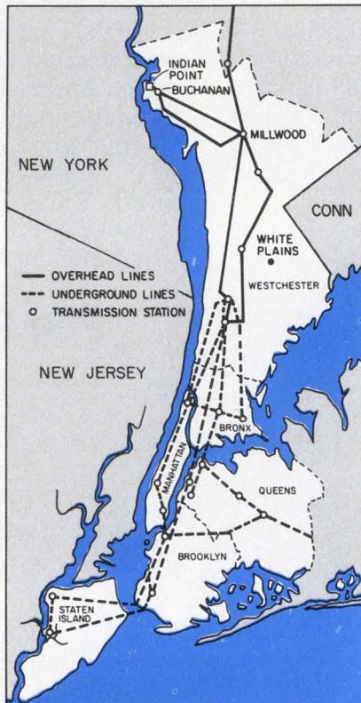
**Power problems cascaded from the north** as Consolidated Edison Co. of New York lost power from Indian Point, then the tie lines to upstate sources. Tie lines to New Jersey and Long Island overloaded and cut out, leaving the burden on Con Ed's major power plants in Queens.
