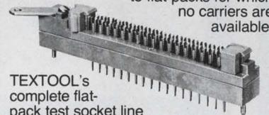
TEXTOOOL's complete flat-pack test socket line now includes units to accept devices with 50, 52, 64, 70, 76, 82 and 96 leads (two and four sided). All sockets feature maximum device protection while insuring consistently good electrical contact. Wiping contacts eliminate "dimpling" or gold removal, and lids are reinforced in the contact area.
