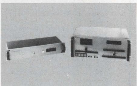
**COMPUTER PROGRAMMABLE MAGNETIC FIELD CONTROLLER.** Model FFC-4DP can interface with most regulated power supplies and virtually any computer with 6 decades of BCD output. Offers 1 part in  $10^6$  full range setting of field amplitude of an electromagnet. Manual input also provided. Features stray field compensation and elimination of hysteresis effects and temperature gradient effects. Many applications. Write: Walker Scientific, Inc., Rockdale Street, Worcester, MA 01606
