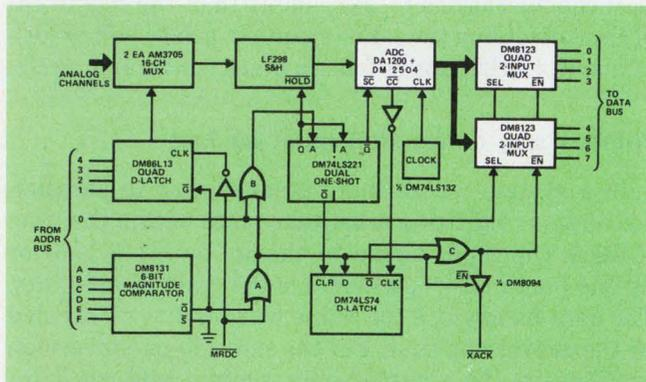
2. Three-state outputs and address-LSB compatibility of the Select inputs, allow the quad two-input MUX units to easily split the 12-bit data from the a/d converter into two bytes for the microprocessor's data bus.
