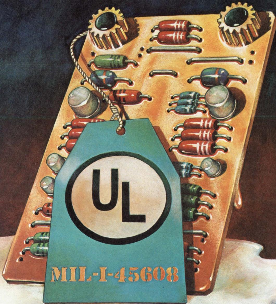
Dow Corning 3140 RTV silicone coating is the only conformal coating that has UL recognition to 180°C and also meets the requirements of Mil Spec MIL-I-45608. But, there's more.
