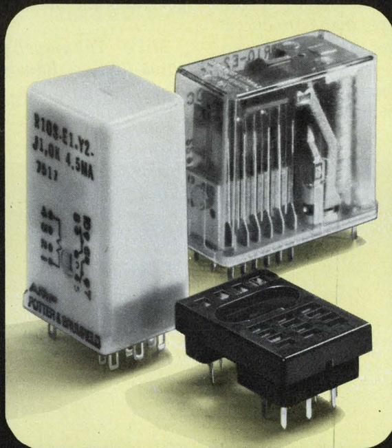
Mechanical life expectancy of the R10 is to 100 million operations—except W contacts, 1 million—and is available with a voltage or current-sensitive coil. It weighs, depending on the number of contacts, from 22 to 40 grams. Pickup ranges from 2.25 to 86 VDC, 5 to 86 VAC, or 0.6 to 45 milliamp with proper power supply.
