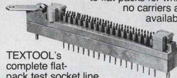
TEXTOOOL's complete flat-pack test socket line now includes units to accept devices with 50, 52, 64, 70, 76, 82 and 96 leads (two and four sided). All sockets feature maximum device protection while insuring consistently good electrical contact. Wiping contacts eliminate "dimpling" or gold removal, and lids are reinforced in the contact area.
