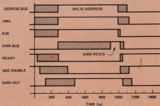
5. ANDing the VMA and R/W signals decodes a valid address in the 16-channel parallel-conversion system for the 6800 microprocessor (a). Address information, the
