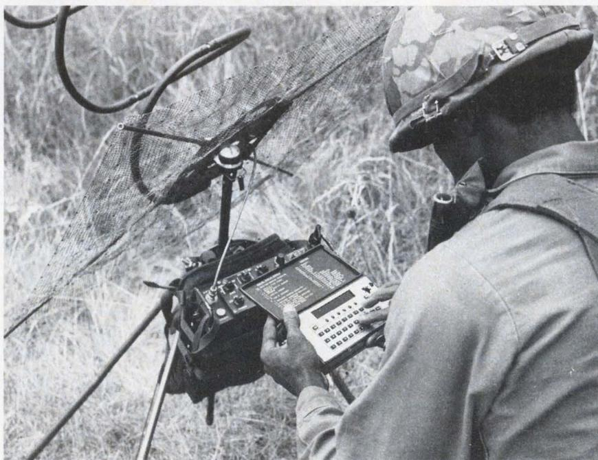
**Using only 35 W of power and a satellite relay, the AN/PSC-1 can communicate with support units as far as 9000 miles away.**
