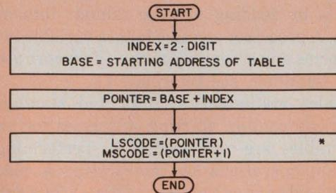
\*The Intel 8080 generally stores 16-bit numbers or addresses with the LSBs first while the Motorola 6800 stores them with the MSBs first. LSCODE and MSCODE are thus reversed in 6800 memory.
