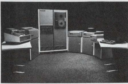
**New medium-scale, multi-use computer system from Harris.** Powerful VULCAN Virtual Memory Operating System supports more than 50 terminals simultaneously. Greater I/O throughput. MOS Memory with error correction. Powerful micro processor based CPU. Operates with ANSI 74 COBOL, FORGO, SNOBOL, FORTRAN, RPG II, extended BASIC. Handles multi-stream batch processing, multi-concurrent RJE's (host and remote). Harris Computer Systems, 1200 Gateway Dr., Ft. Lauderdale, Fl. 33309 (305) 974-1700.
