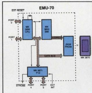
then be copied to AIM-70 for execution. This is a true in-circuit-emulation configuration. Real time execution of the target system code, breakpoint insertion, and single-step operation are a few of the features available with this system.
