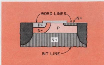
1. The simple cell structure of the I<sup>2</sup>L RAM of Fairchild gives the 4096-bit device two to three times the speed of its MOS RAM competitors.
