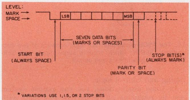
13. In ASCII serial format, the two logic levels are called "mark" and "space" instead of HIGH and LOW. Each character requires 10 to 11 bits.
