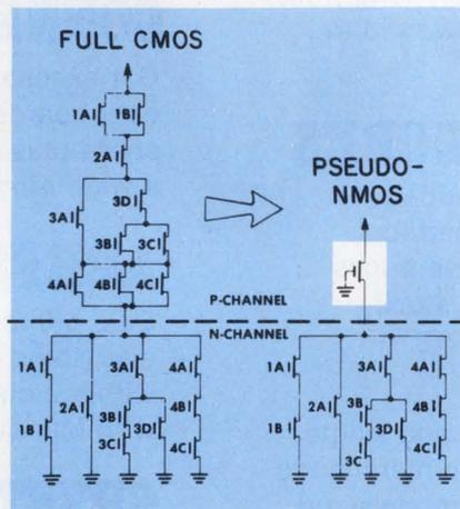
By using a pseudo-NMOS structure instead of normal CMOS design, engineers at Bell Laboratories managed to reduce the complexity and size of the gate logic in their 8-bit CMOS microprocessor.
