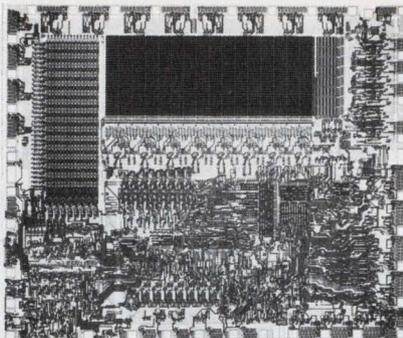
**Containing 1024 bytes of UV PROM and 64 bytes of RAM in addition to a full 8-bit  $\mu$ P on a single chip, the 8748 is the first of a new breed of user-programmable microcomputer circuits pioneered by Intel.**
