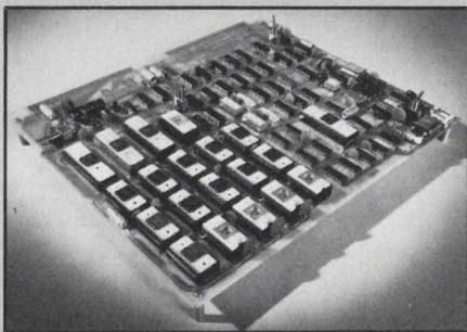
A series of inexpensive microcomputer kits has been designed to meet various needs—from the beginner's to the advanced engineer's. The kits in American Microsystems' EVK series are based on the 6800  $\mu$ P and range in price from \$133 to \$765.
