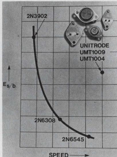
sistance between the shifting conduction site and the base terminal increases. Consequently, when the base is driven from a practical impedance source with a finite resistance, the increasing base resistance reduces the turn-off base drive by 1/2 to 1/4 the initial value and greatly increases fall time.
