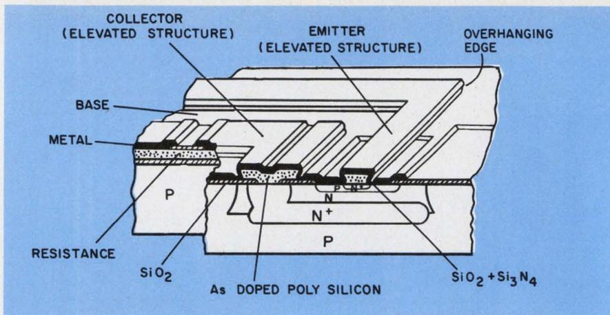
This integrated transistor structure uses the Elevated Electrode IC process developed by Musashino Electrical Communication Laboratory. EEIC achieves ultra-high speeds in part by decreasing junction capacitance.
