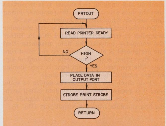
8. PRTOUT is a subroutine for printer-interface logic. After the data are transferred, control is returned to the main program.
