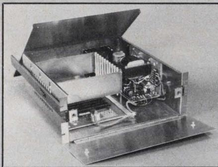
Several Micromodule card cages and a power supply have been added by Motorola to support M6800-based equipment development. Two card cages are available: one with five card slots, the other with 10. Both cages have motherboards that are pin-compatible with all Micromodules and EXORciser modules.
