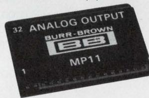
Both the MP10 and MP11 provide  $\pm 10V$  outputs with 8-bit resolution and throughput accuracy better than  $\pm 0.4\%$  of full scale range. With a price of just \$99 (100's), it just doesn't make sense to design your own analog I/O solutions. Send for details today. Write or call Burr-Brown, International Airport Industrial Park, Tucson, Arizona 85734. Phone (602) 294-1431.
