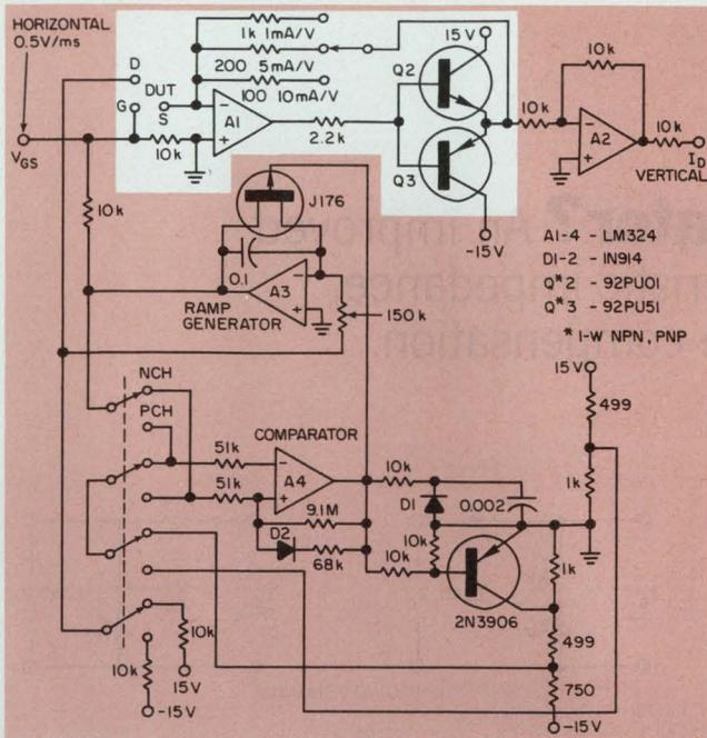
2. Basis of the tracer is a current-to-voltage converter designed around an op amp ( $A_1$ ), one-fourth of a quad. Amplifier  $A_2$  forms a unity-gain inverter, while  $A_3$  and  $A_4$  form the sweep generator. Sweep rate is 0.5 V/ms.
