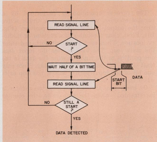
15. To detect a start bit reliably, the signal is monitored twice. Conversion starts only if the start bit is present at both sampling times.
