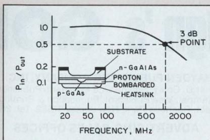
shorter than the electron diffusion length can be used to reduce the electron lifetime further. The time delay due to the diode's space-
