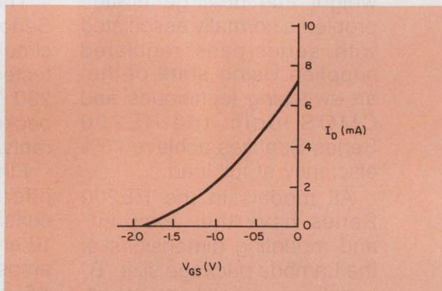
1. Output of the curve tracer is a typical FET transfer curve, like this one for an n-channel unit.
