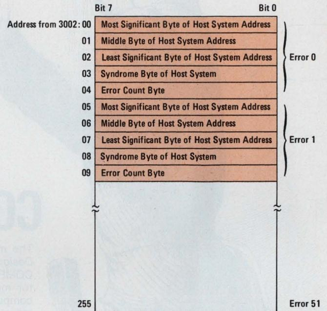
12. The random-access memory needed to hold the log data must be grouped into blocks of five bytes for each error file. Three bytes are needed for the system address, one for the parity and one for the error-count.
