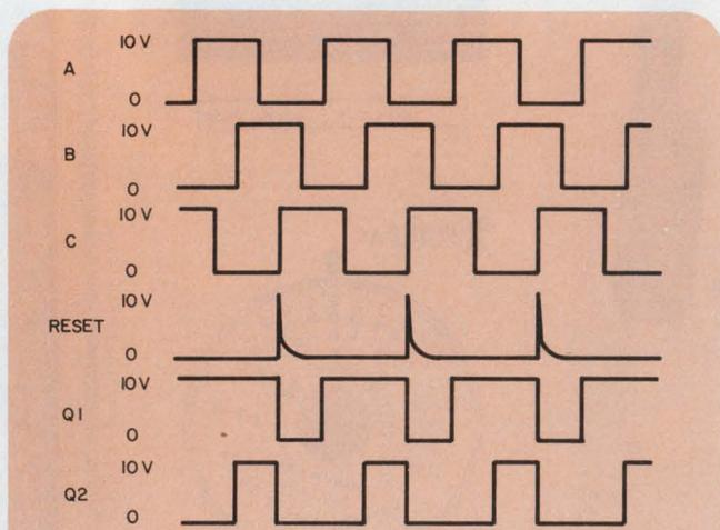
2. Any one of the following correct phase sequences—ABC, BCA or CAB—will produce a train of rectangular pulses at the output  $Q_2$ , in Fig. 1. For incorrect sequences—BAC, ACB or CBA—the output,  $Q_2$ , stays LOW.
