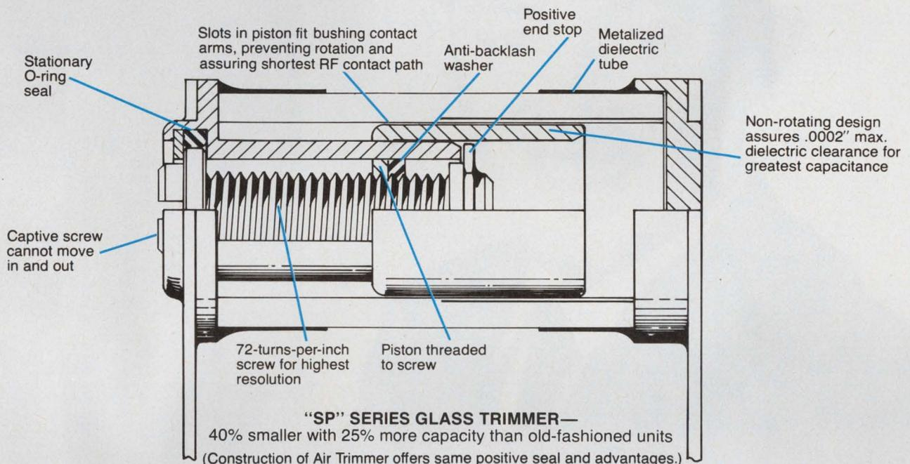
When high Q and stable performance are a *must*, you can't settle for a trimmer capacitor that is "almost right". Only Voltronics, with its unique, patented, non-rotating piston, eliminates the problems of conventional capacitors.
