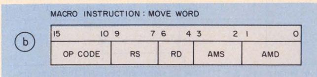
7. By making the microword as long as necessary, every control function you will ever want can be given its own field (a). A macroinstruction word can also be divided into fields (b), which must be decoded further into microinstructions.
