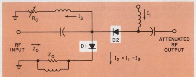
2. A pair of PIN diodes in an L-pad configuration can be used to attenuate rf signals controlled by dc current. Both  $I_1$  and  $I_2$  must be varied appropriately to control attenuation and keep  $Z_0$  constant.
