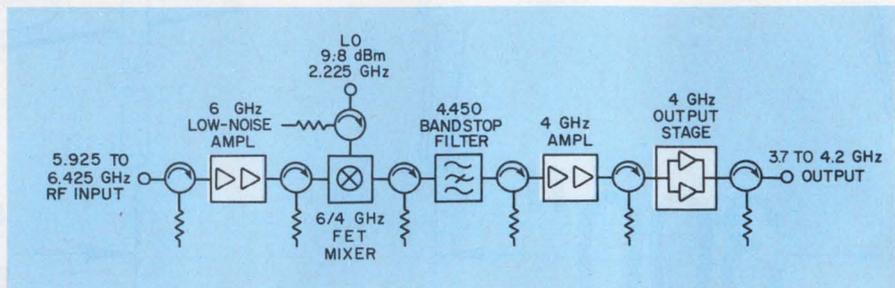
High gain, excellent linearity and low noise figures are provided by gallium-arsenide FETs in this satellite-communications receiver.
