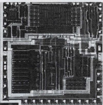
**Duplicating the Nova instruction set, the 9440 microprocessor developed by Fairchild uses I<sup>3</sup>L processing to attain a chip size of only 182 × 189 mils.**
