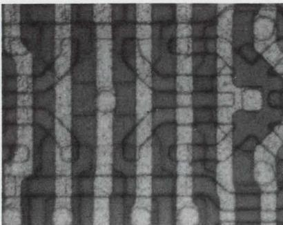
Shrinking the size of a memory cell so that four transistors and two high-impedance resistors are contained in 2.75 mil, Mostek designers have come up with a 4-k static RAM that operates with less than 80 mW.
