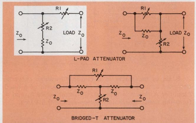
1. L-pad attenuators can provide a constant characteristic impedance,  $Z_0$ , as the attenuation is varied—but only at the input terminals. A bridged-T configuration can keep  $Z_0$  constant at both input and output terminals.
