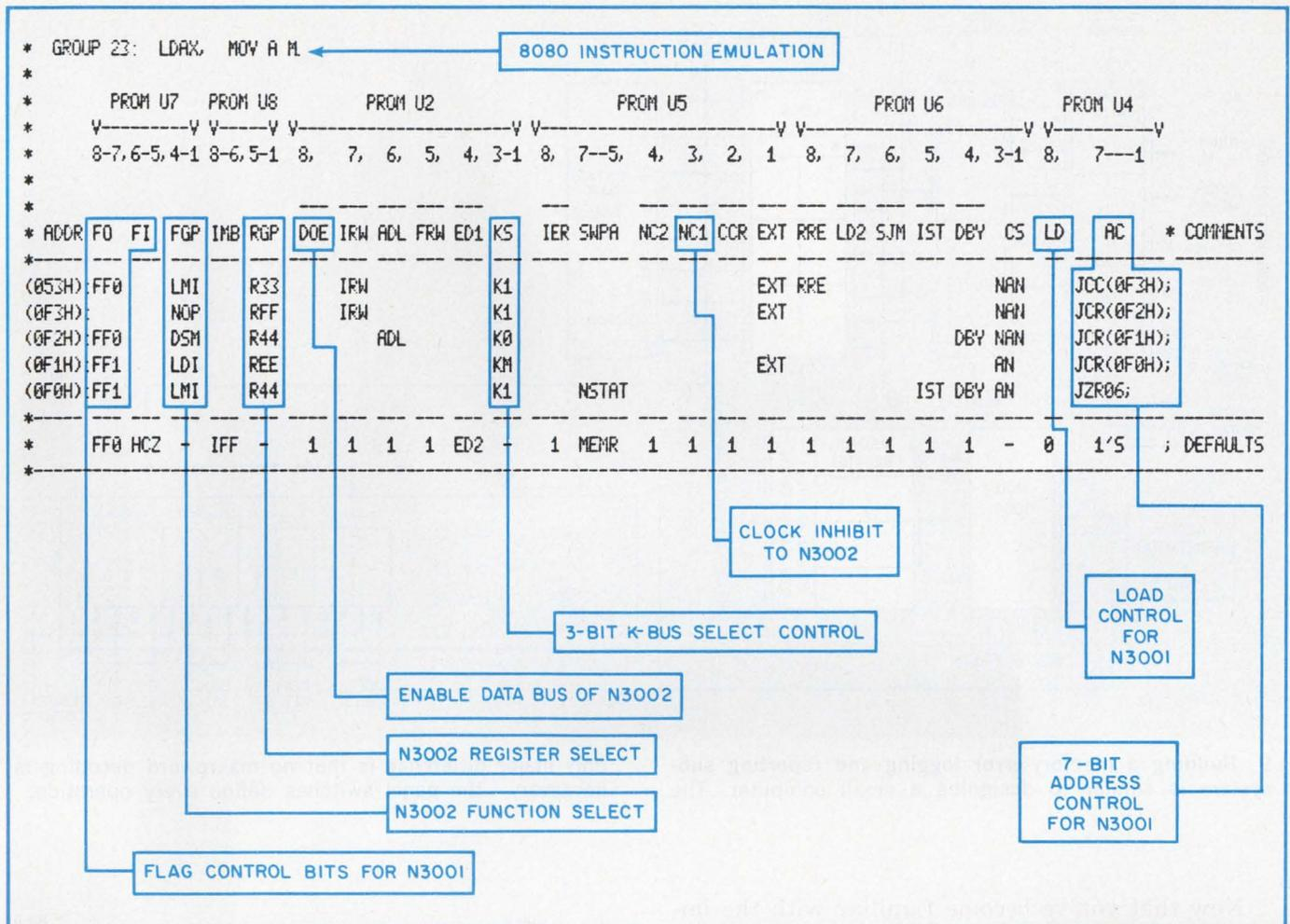
8. Using a high-level Micro Assembler to turn mnemonic microword listings into executable code can cut the time required to develop and assemble microcode. Available
