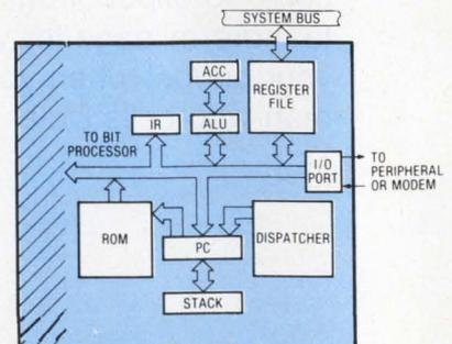
What's better than one  $\mu$ P on a chip? Why two, of course. Combining both a bit and byte-oriented processor on a single chip, Intel has been able to make programmable controllers from the same basic chip.
