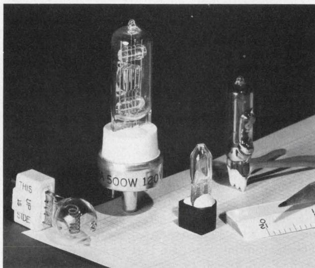
Special, highly stable ceramic-like adhesive can perform satisfactorily up to 2200 C. Here a Sauereisen inorganic cement is used for stable alignment of lamps operating up to 330 C. From left to right: a film projector lamp, a flash bulb and an aircraft warning light. At far right, external leads of mercury switch are sealed.
