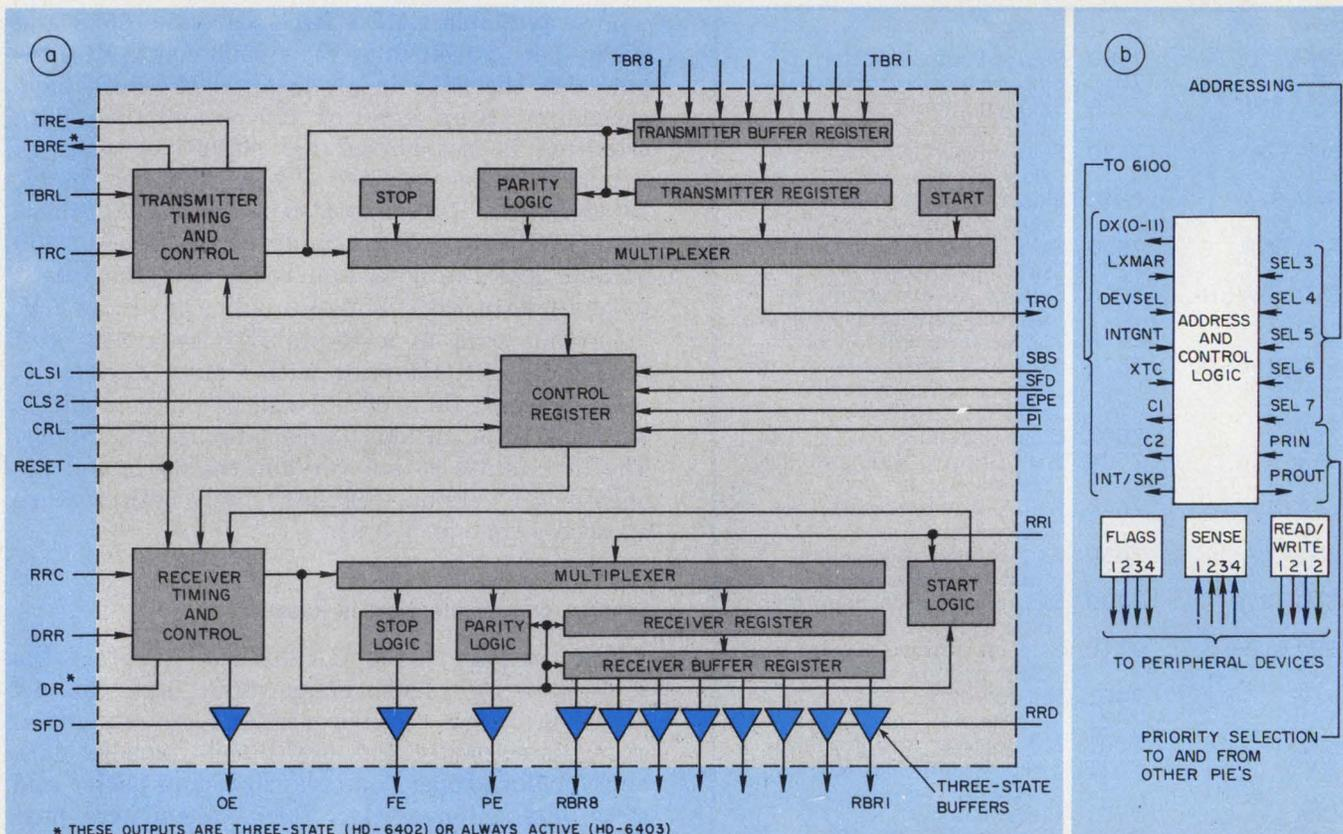
4. Connecting the CMOS UART (a) or the PIE (b) is very straightforward. The UART can operate at clock frequen-
