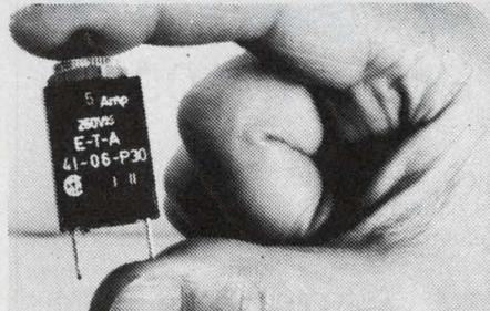
**Overcurrent Protector**, manual reset eliminates fuse replacement. Convenient panel mounting. 19 fractional ratings from 0.1 to 5 amp. Other models up to 400 amp. Trip-free and fool-proof, UL and CSA approved. High quality, low cost \$1.33 ea. in 1000 lots. E-T-A Products Co. of America, 7400 N. Croname Rd., Chicago, Ill. 60648. Tel: (312) 647-8303. Telex: 253780.
