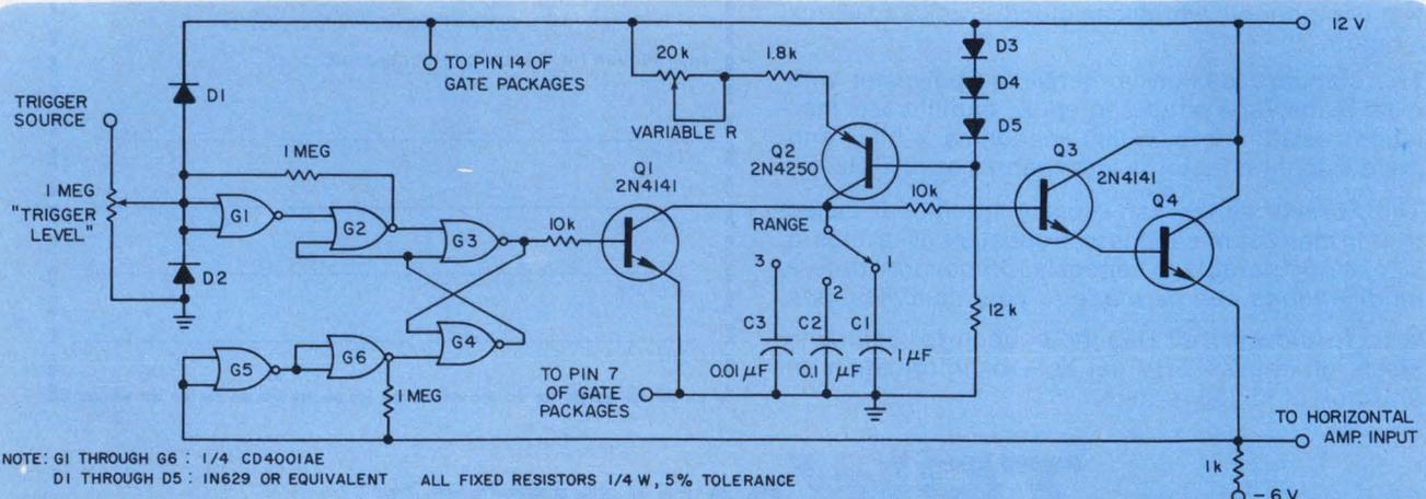
A triggered-sweep capability can be added to old recurring-sweep scopes with this simple trigger-
