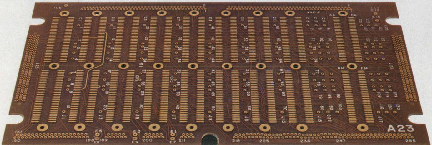
Two major systems — wirewrapping and multilayering — have been used for complex electronic interconnection in the last 15 years. Despite improvements and refinements, each still has inherent disadvantages. That's why Multiwire was created by Photocircuits. It overcomes the disadvantages of wirewrapping and multilayering.
