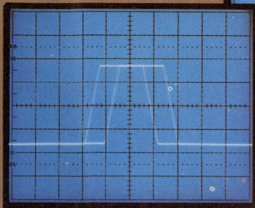
2 Switch to delayed sweep mode and use  $\Delta$  Time dial to superimpose beginning and end of interval.
