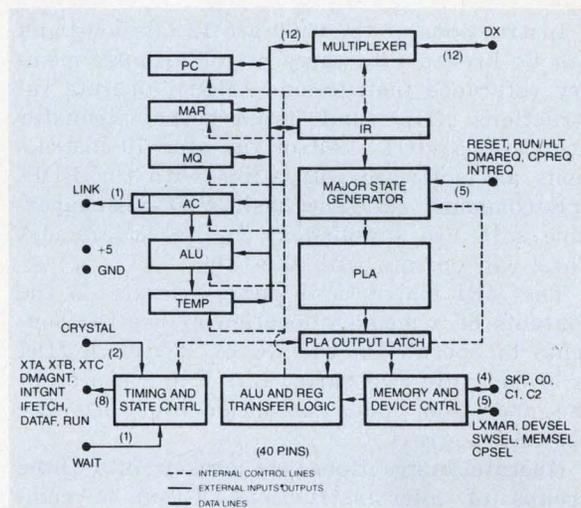
Data and addresses share a common 12-line bus that feeds directly into a 12-bit multiplexer. The multiplexer, in turn, is controlled by the major-state generator and control ROM. All timing and state signals needed by the 6100 are generated by an on-chip clock (only a 4-MHz crystal is required). An internal dividing circuit reduces the clock so that the internal states are 500 ns long.
