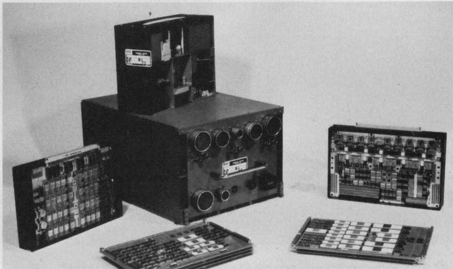
An airborne computer, dubbed the AN/AYK-14, has been developed for the Navy by CDC. The heart of the unit is the AMD 2901 microprocessor.
