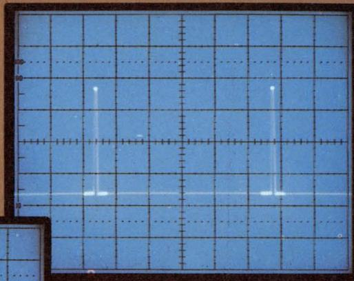
1 Position intensified spots at beginning and end of time interval.
