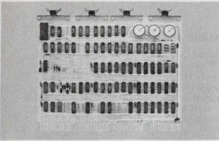
**The TCU-100**, a self-supporting timekeeper for a PDP-11, can give you the time as follows: month and day, hours and minutes, seconds. It can be initialized by simple commands from the computer and features rechargeable battery power for uninterrupted use when the computer is off, plus extensive interrupt capability. Price: \$495. For literature, write or call Digital Pathways, 4151 Middlefield Road, Palo Alto, CA 94306. (415) 493-5544.
