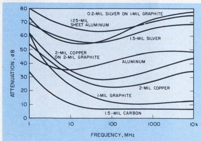
**Shielding effectiveness of conductive coatings** varies with material type and coating thickness. Typical attenuations of Acheson Colloids' formulation on a 0.125-in.-thick polycarbonate sheet are shown.
