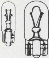
These lamps are ideal for applications such as indicators, markers and general illumination where space is at a premium. Their wedge-based construction makes them easy to insert and remove. They don't require bulky, complicated sockets. And because the filament is always positioned the same in relation to the base, you get consistent illumination from lamp to lamp.
