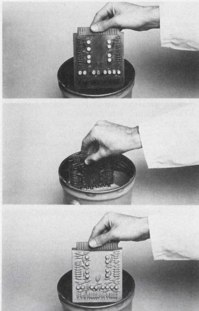
Conformal dielectric coatings protect PC boards and their components against moisture, abrasion and contamination. This Silgan elastomer coating holds components securely.
