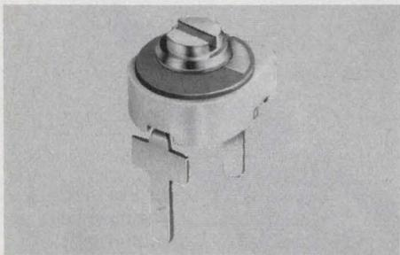
**MINIATURE CERAMIC TRIMMER CAPACITORS** 9371 series of ceramic trimmer capacitors are compact, economical and rugged. They are 50% smaller than other trimmers of this type yet provide high capacitance values. Available in 4 capacitance ranges, 1.5 to 4, 3.0 to 10, 3.5 to 18 and 5.0 to 25 pf with Q's > 300 at 10 MHz. They have an overall diameter of .225" with .215" above board height.
