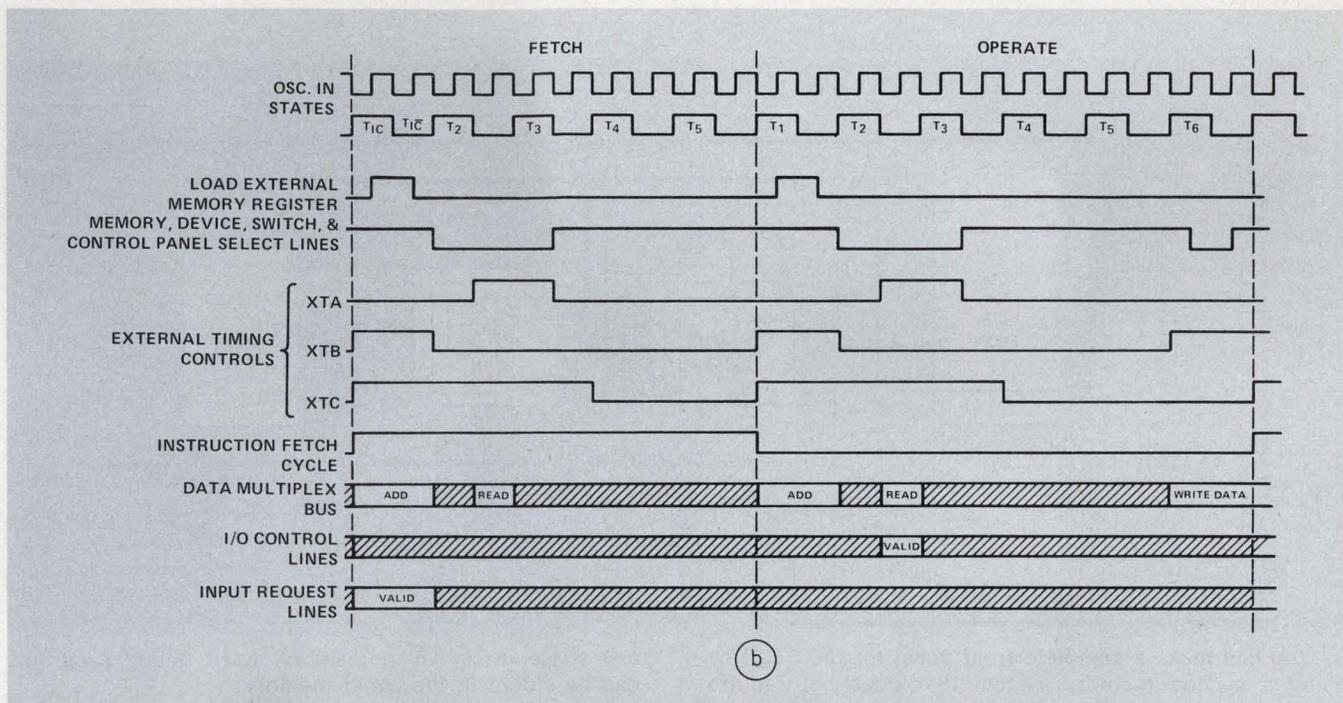
1. By using a shared address and data bus, the pin count of the 6100  $\mu$ P can be kept to 40 (a). Timing
