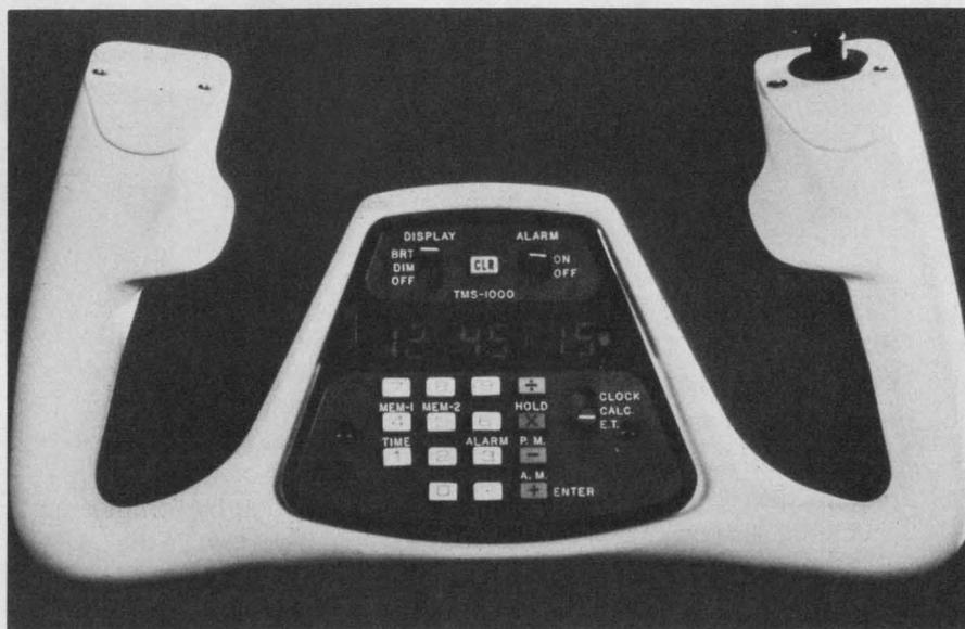
**A two-chip MOS calculator and clock-timer reduces pilot's in-flight workload.** The TMS-1000 by Martin Avionics, requires tight packaging, enhancement of the LED display, and elimination of EMI.
