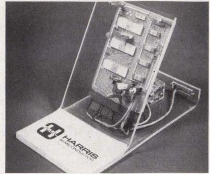
2. Just four circuits are needed to build a minimal operating system—the 6100, a ROM, a RAM and a PIE.
