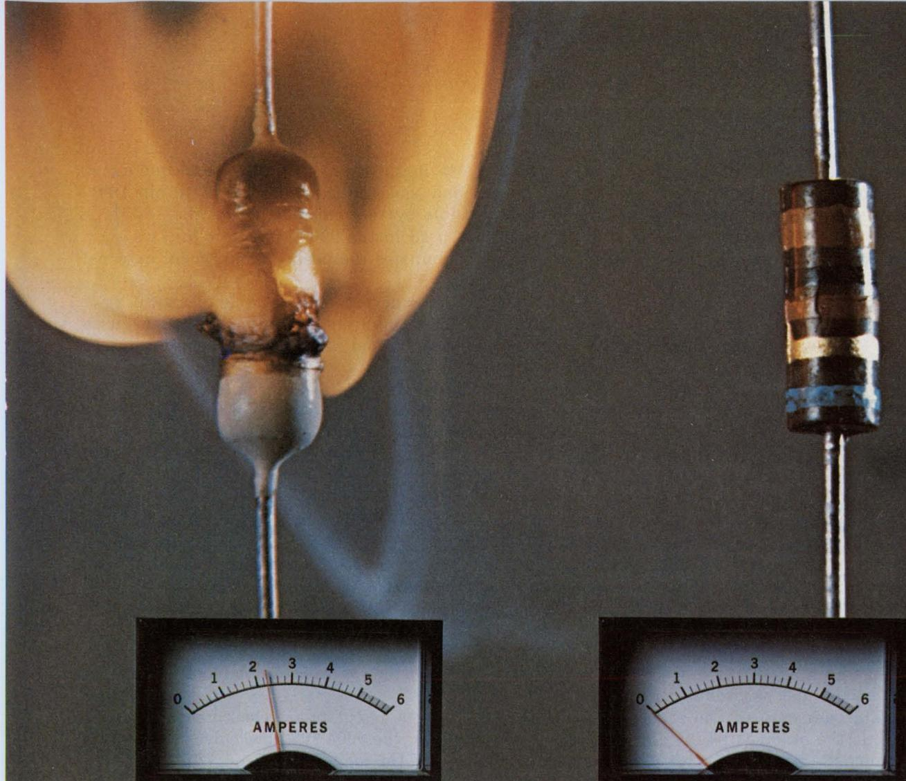
**The failure.** A 16 W overload causes this 1/2 W carbon film resistor to burst into flame. The initial failure mode is a short circuit, causing even more current to be drawn as shown on the meter.
