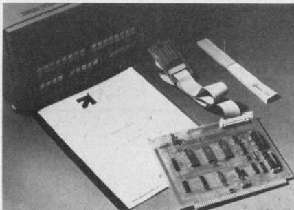
If you have Intel's Intellec 8/Mod 80 development system and you're looking around for a software-controlled EPROM programmer that will work on 2704/2708 devices, the Model 2730 programmer is for you.
