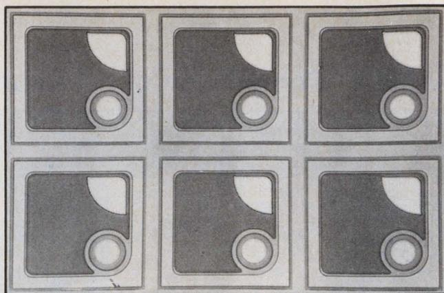
2. These phototransistor chips are Siemens type BP 102. The bright circular spot is the emitter contact, the triangular spot the base and the dark square the photo-sensitive area, which measures 0.6 mm<sup>2</sup>.
