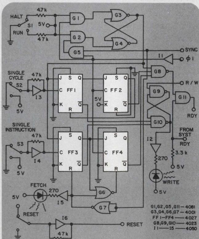
1. To operate a 6502  $\mu P$  in the single-cycle or single-instruction mode, set  $S_1$  to Halt. The  $\mu P$  will then stop at the proper time to allow you to initiate either mode by momentarily pressing either  $S_2$  or  $S_3$ .
