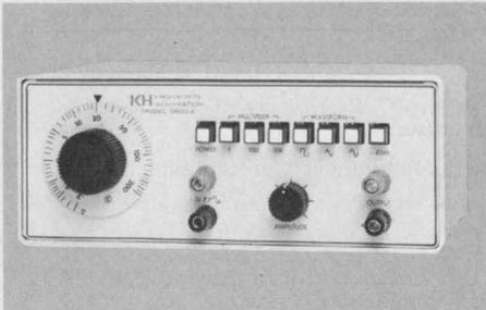
Krohn-Hite Model 5800A function generator, budget priced at \$245, offers sine, square and triangle waveforms over a range of 0.2 Hz to 2 MHz. Distortion is typically less than 0.3%. Simple 1000:1 frequency tuning dial. Pushbutton controls. 50-ohm output adjustable from 5 mv pk-to-pk to 15 volts. Auxiliary 1-volt pk-to-pk square wave output. Stock delivery. KROHN-HITE, AVON INDUST. PARK, AVON, MA 02322
