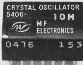
A molded oscillator, on the other hand, has no holes, no open spaces, nothing to hide and nowhere to hide it. Its crystal is hermetically sealed and set in a monolithic block of solid black plastic. There are no spaces for air to penetrate, no room for dirt or moisture to accumulate. Wave soldering can't even deteriorate the unit, so there's no danger of loose pins or joints.
