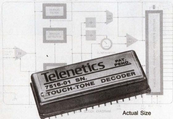
Telenetics' 7516-01 is a complete Touch-Tone Decoder in a 1/2 cubic inch, 32 pin DIP. Telephone Standard 2-of-8 tones are received, processed and decoded into discrete 1-of-16 or BCD (plus strobe) outputs. Input signal ranges -22 to +4 dBm with a balanced, capacitively coupled, 50 K $\Omega$  impedance. Operating voltage range is 8 to 28V dc (single supply); temperature range -30 to 70°C.
