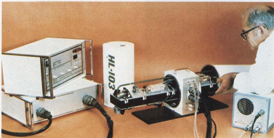
Nd:YAG pulsed laser systems, such as the HL-103 from International Laser Systems, are used in such applications as nondestructive testing and ballistics research.
