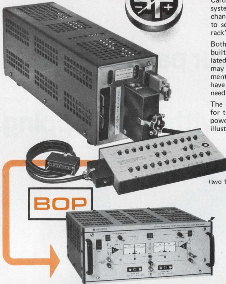
Kepeco's Digital Programmers are composed of individual PC Cards that may be combined as you require to form a control system. The combination to the left provides a 12-bit, 2-range channel for voltage setting, plus an independent 8-bit channel to set a current limit. It is housed in a convenient "quarter-rack" assembly, seen here from the rear.
