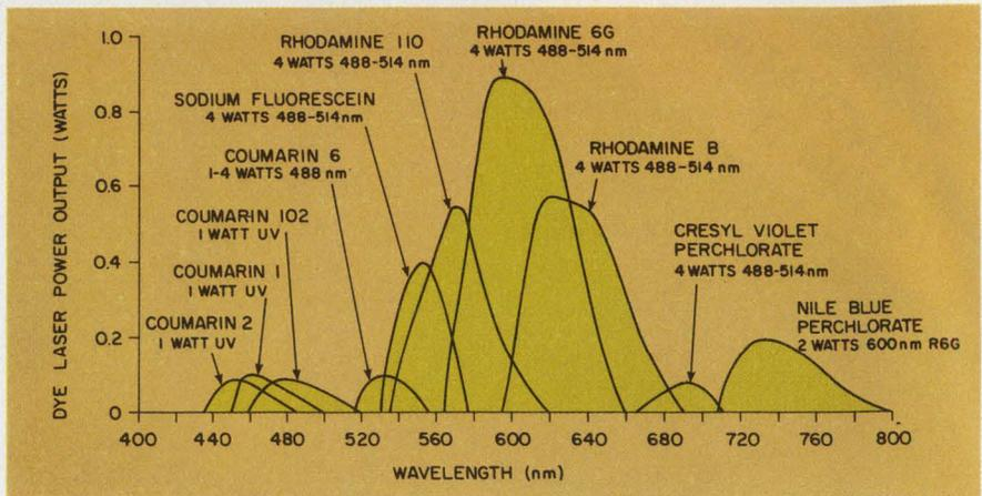
Various dyes can be used to tune the dye laser all the way from 400 to 800 nm. These are some of the typical dyes used. The performance data are for the Spectra-Physics Model 375 high-performance CW dye laser.
