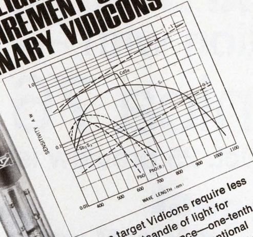
Silicon target Vidicons require less than .01 footcandle of light for effective performance—one-tenth the requirement of conventional antimony trisulfide vidicons. Unsurpassed resolution is another reason for switching to the N747T or N736T Vidicon for surveillance, industrial and educational TV cameras. When you compare the performance, you'll be amazed at the price.
