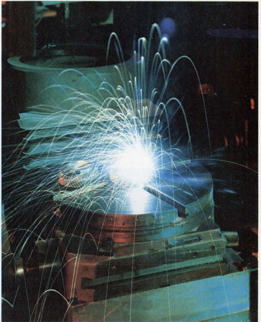
Two gears of an automobile transmission component are welded together by a high-power CO<sub>2</sub> industrial laser from Avco Everett Research Laboratory.
