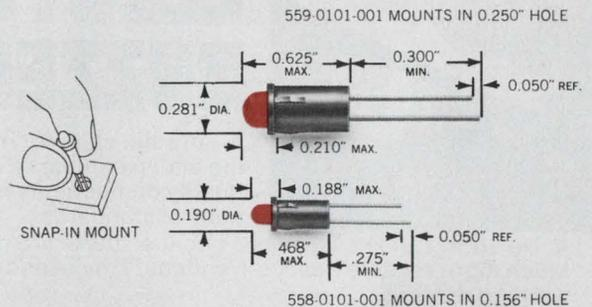
**558 and 559 SERIES** Available in red, green or yellow LEDs, with and without integral current limiting resistors. Snap-in mounting requires no additional hardware. Straight terminals suited for wire-wrapping and/or soldering. Low power requirements—15 to 20mA. In 1000-lot quantities each
