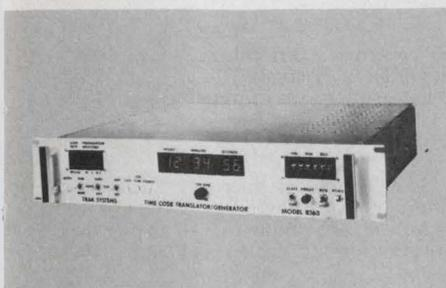
**MODEL 8363 TIME CODE TRANSLATOR/GENERATOR** operates on external 1 MHz standard or optional 1 MHz internal standard. Automatic WWV synchronization included. Time of day on six 0.6-inch planar displays. Code input formats include IRIG A, B, G, NASA 36, XR3, and 2137. Time generation continues with loss of input code. Numerous options and formats available. TRAK Systems, 4722 Eisenhower Blvd., Tampa, FL 33614. 813-884-1411. Telex 52-827.
