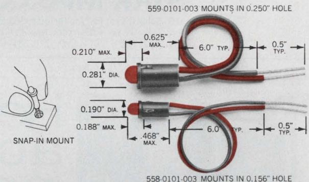
**558 and 559 SERIES** Available with 6" wire leads, these red, green or yellow LEDs are designed for quick positive insertion in 0.031" to 0.062" panels. Compact design allows high density packaging. In 1000-lot quantities each
