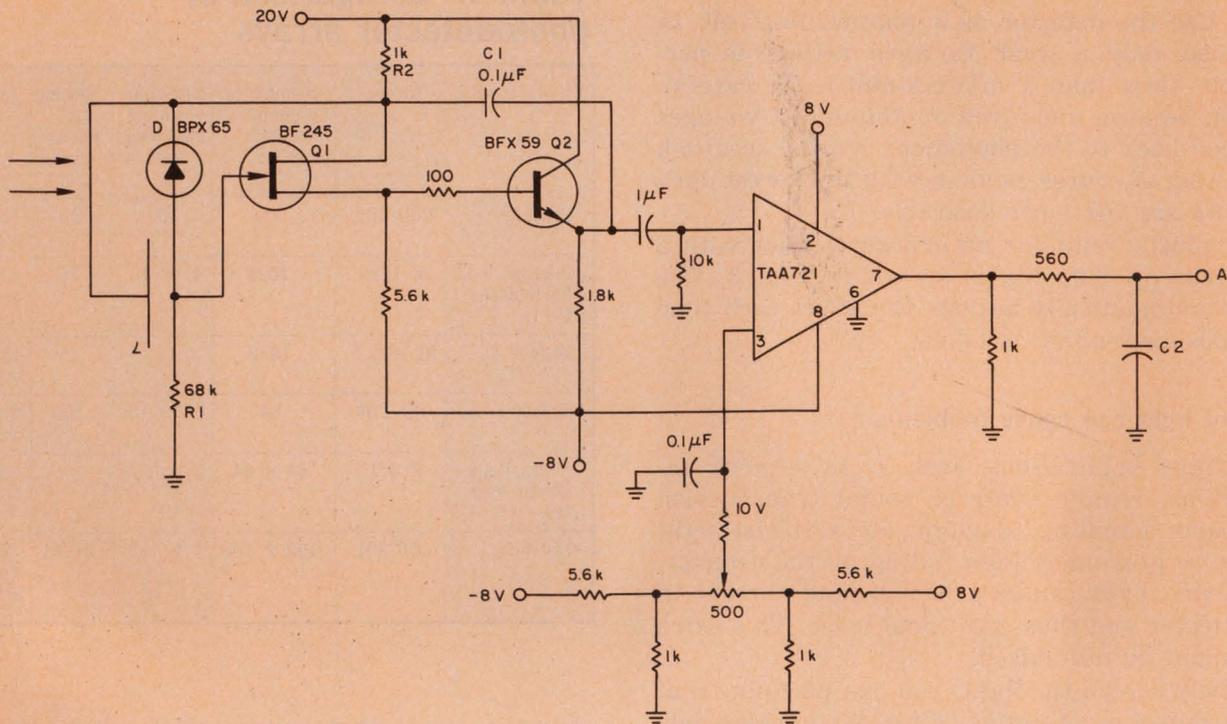
5. For operation at frequencies exceeding 5 MHz, this photodetector circuit uses compensation that is fed back
