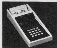
We also make a portable programmer, FPLA programmer and the Romulator.™ The Romulator allows you to emulate/simulate PROM operation — in your circuit — without PROMs. PROM data is easily altered and updated on the Romulator keyboard, all prior to PROM programming.
