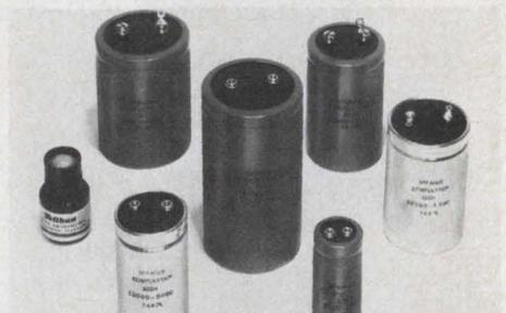
**'LYTIC' CAPACITORS WITH AN OPTION.** Type 32D Compulytic® Aluminum Electrolytic Capacitors, designed for power supply applications, give you the option of securing more capacitance in a given case size with the Type 32DX version or of obtaining lower ESR and higher ripple current capability in Type 32DR. Sprague Electric Co., 347 Marshall St., No. Adams Ma. 01247 (413) 664-4411.
