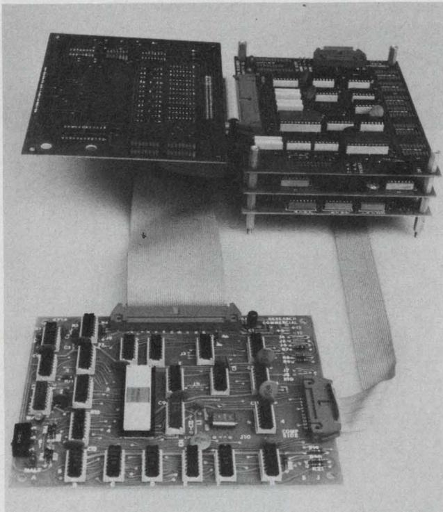
The MIKE-3 system of boards from Martin Research contains  $\mu$ P and clock, keyboard and display, debug, and memory—each on a separate plug-in board that connects with the others (3 boards plus 2 optional).
