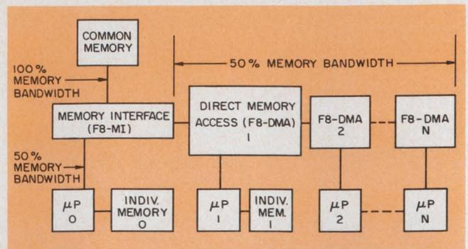
6. A high-speed system may be constructed if individual microprocessors can access common memory through DMA (Direct Memory Access).
