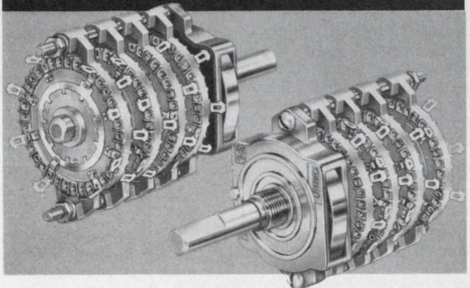
Reduce your design time with this 1½" diameter rotary switch. 8 to 36 positions, depending on detents selected (11 available, from 10° to 45°) allowing thousands of switching variations. Crisp, uniform ball and starwheel Unidex® detent. Double-wiping, self-cleaning, high-pressure contacts. Military types available.
