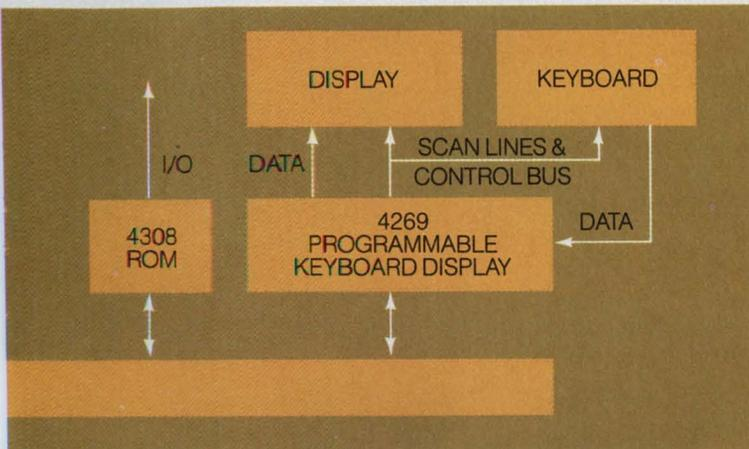
and system memory for display refresh since the necessary memory and control are built in. One 4269 can operate and refresh alphanumeric displays or indicator arrays with up to 32x4 digits, 16x8 characters or any configuration of 128 elements or lights, including a 20-character Burroughs Self-Scan\* Display.
