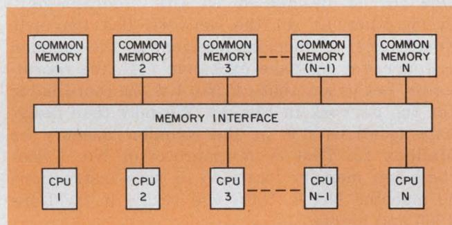
10. Systems that have individual subports of common memory allow fast operation, but require complex memory interface circuitry.
