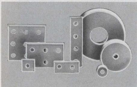
**CIRCLE & MULTI-FEED-THRU CAPACITORS;** available in a wide range of sizes and configurations, with NPO, BX, Z5U and Y5V characteristics. For use as feed-through elements, where volume efficiency of capacitance performance is required. Applications also include filter networks, pulse and logic circuitry, and signal bypass to ground elements in broadband circuits. Available in configurations suited to customer needs. Johanson/Dielectrics, Inc., Box 6456, Burbank, CA 91510 (213) 848-4465.
