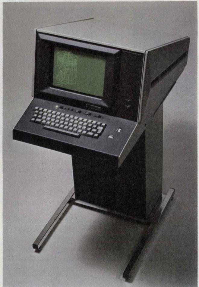
Structural analysis performed on a Tektronix storage-tube terminal provides geometric previews of a section of a diesel-engine piston.
