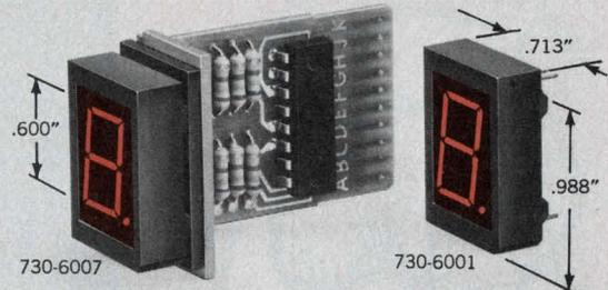
**730 SERIES** A new 0.600" LED character in super bright red, seven-segmented readout . . . low power . . . draws 10mA/segment or less . . . operates with standard IC power supply levels. Very high contrast ratio . . . visible from 40'. Available with or without on-board decoder/driver, plus or minus bar, and with bezel mounting. In 1000-lot quantities each LED
