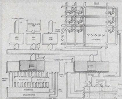
With the availability of two software-programmable devices—the 4269 keyboard/display unit and the 4265 general-purpose I/O unit—users of Intel's MCS-40 family of 4-bit  $\mu$ C systems can reduce the number of components needed to operate an increased number of peripherals. The MCS-40 family is based on the 4004 and 4040  $\mu$ Ps and consists of components that can be used with either  $\mu$ P. All ICs are available from Intel (3065 Bowers Ave., Santa Clara, CA 95051. 408-246-7501).
