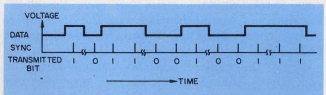
3. A timing diagram illustrates the serial and asynchronous method of transferring data.
