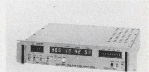
**MODEL 8365 Universal Time Code Generator** has all the features required in a time-code generating instrument. Unit generates all 6 IRIG Codes in DC level-shift form. Modulated output may be ordered with unit or added later by inserting plug-in modules. Unit automatically synchronizes within 2 ms of WWV or within .5 μs of an external standard. Has RFI filtered power supply and provision for 12-volt battery backup. TRAK Systems, 4722Q Eisenhower Blvd., Tampa, FL 33614.
