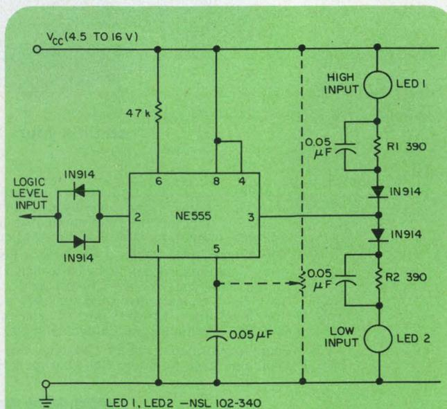
The logic probe can provide accurate level detection if the voltage at pin 5 is adjusted to the desired reference level.
