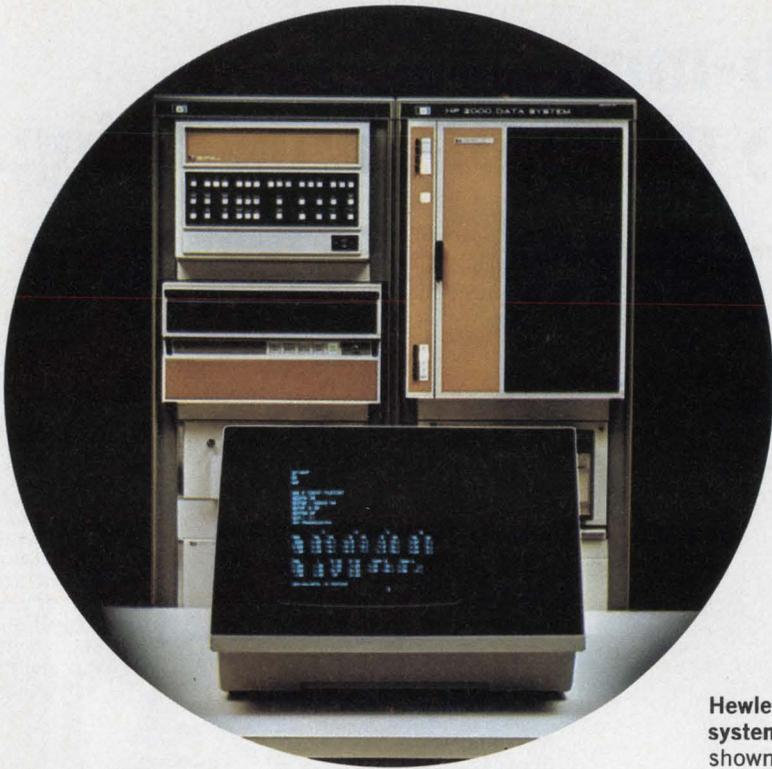
Hewlett-Packard's minicomputer-based scientific data system offers multiterminal, on-line data processing. It is shown with a microwave problem on the screen.
