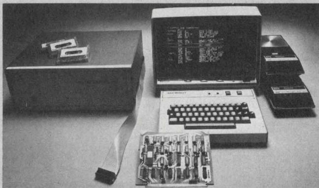
The two most needed microprocessor hardware-development tools, an in-circuit emulator and PROM programmer module, now come on a single plug-in board. Called the M8-40, the board works in conjunction with the Model 8/16 development system from Microkit (2180 Colorado Ave., Santa Monica, CA 90404. 213-828-8539). The combination emulator and programmer costs \$1100, which includes all software and cables.
