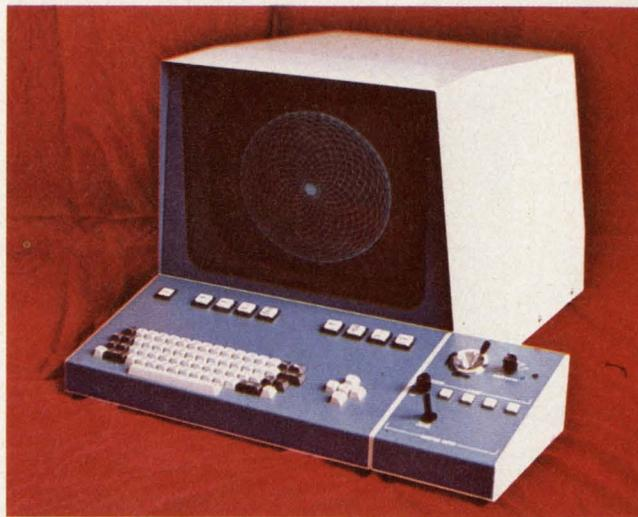
Scan-conversion systems, like this one from Princeton Electronic Products, retain data on a silicon storage tube and use a standard CRT for display.
