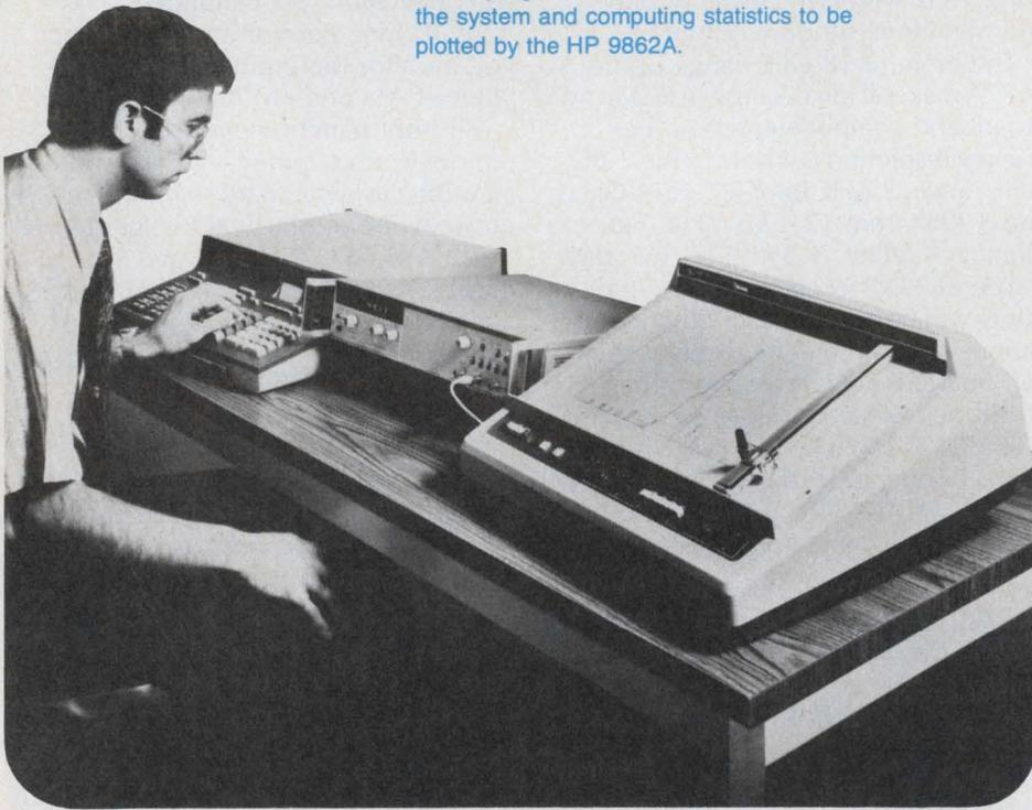
Add Option 041 to the Model 5328A Universal Counter for completely automated operation under computer or calculator control *plus* higher performance time interval measurements.
