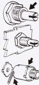
notched tube-steel shell mates with notched end plate. Result? A stronger assembly that takes more torque when installing...with no chance of damage. The leads emerge thru a notch in the steel shell, so they *will not, can not* be sheared by rotation during installation.
