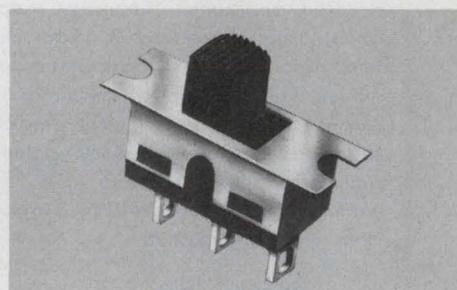
**Model 1101 Slide Switch,** subminiature SPDT in either *Printed Circuit* or *Panel* mount models. Electrical life: 40,000 actuations at full load. Contact rating: 6 amps with resistive load @ 120 VAC or 28 VDC; or 3 amps with resistive load @ 250 VAC. Free engineering sample on request. C&K Components, Inc., 103 Morse St., Watertown, MA 02172 Tel: (617) 926-0800 TWX: 710-327-0460 TELEX: 92 2546
