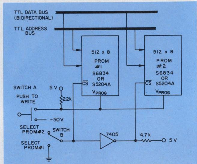
1. Different PROMs can be programmed collectively—a key requirement for board programming. To write (program) data in or read them out, use switch B to select a PROM. For programming, apply address and data, and then depress switch A. For a read operation, simply apply an address; data will then appear on the bus.
