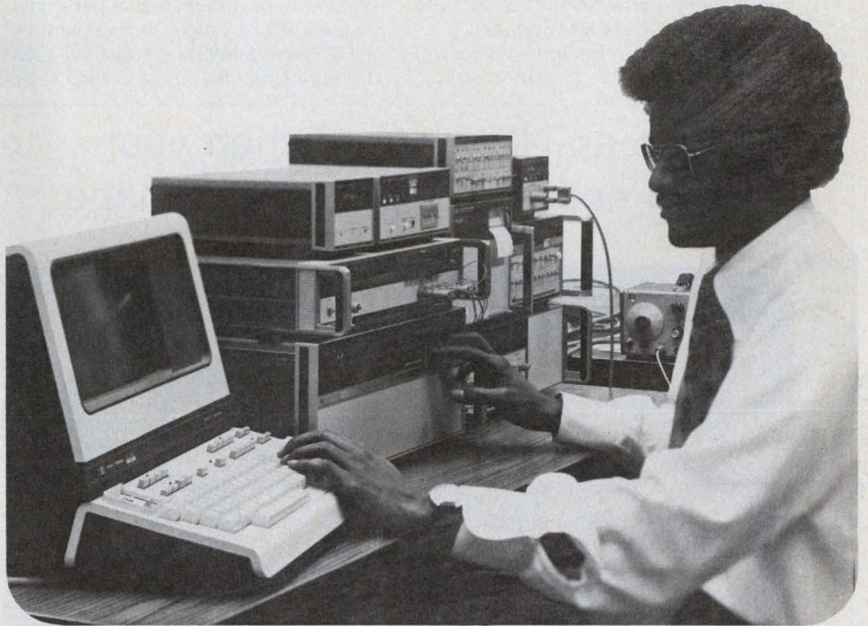
Now, system designers can connect HP-IB instruments, like the DVM, scanner, numeric display, thermal printer, timing generator, counter, and digital-analog converter shown above, to the powerful control, data processing, and storage capabilities of Hewlett-Packard Real-Time Minicomputers.
