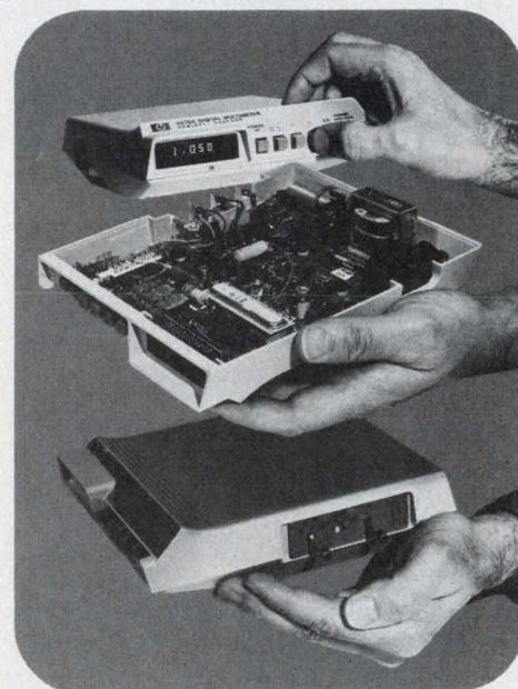
Compact new DMM with advanced circuitry and packaging resulting in high reliability. One circuit board contains all the electronics.
