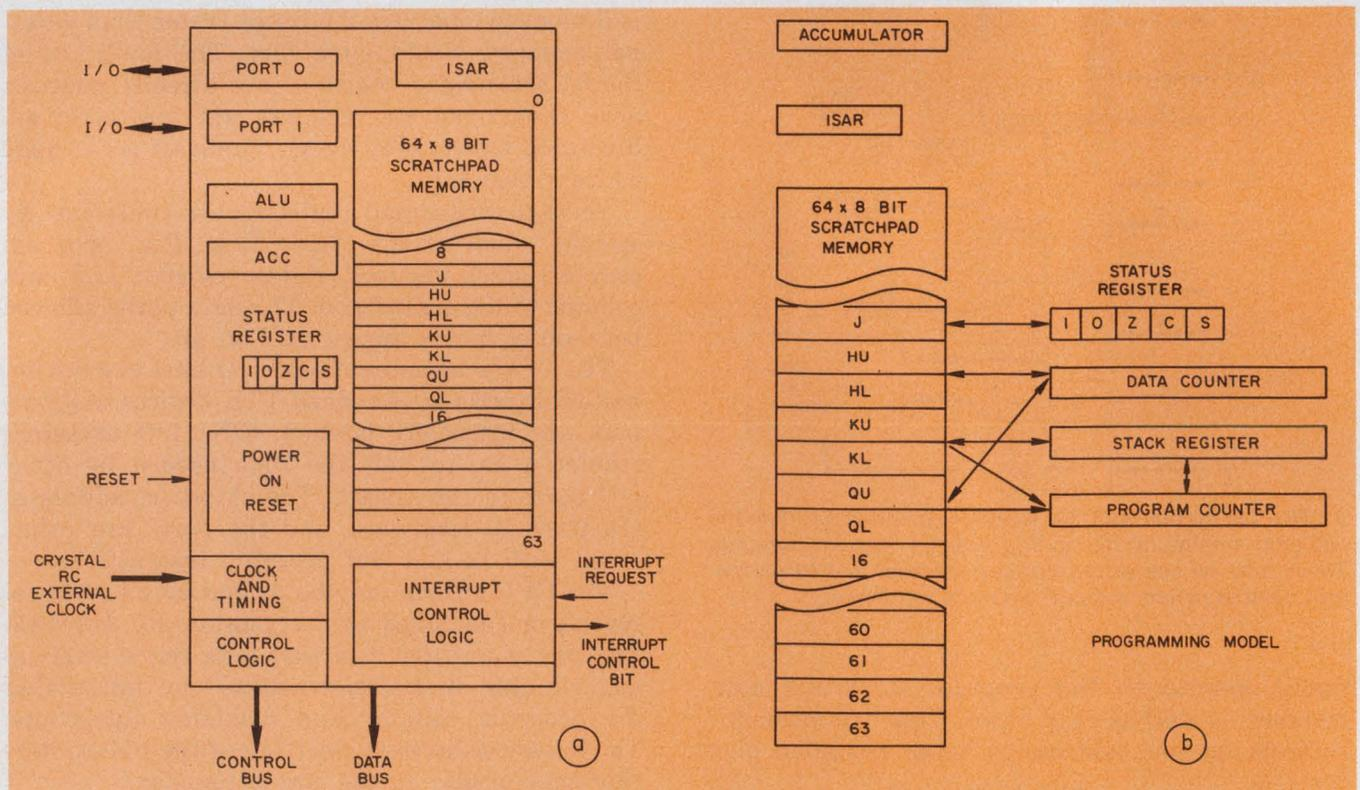
4. The CPU chip contains a 64 x 8-bit RAM, two 8-bit I/O ports and internal clock (a). It also has a power-on reset function and 16 TTL-compatible I/O lines. All 64
