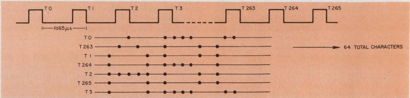
7. RAMs used as display buffers can access the points on a raster-scan display to automatically select 64 columns.
