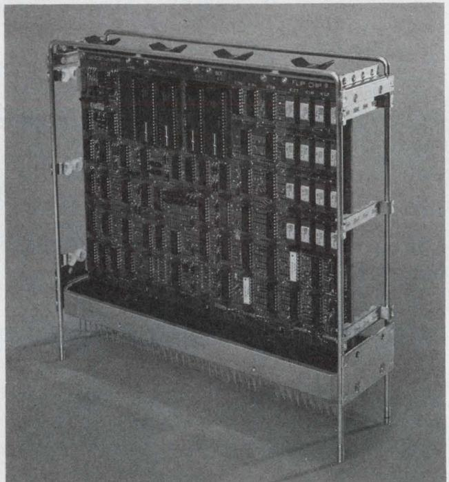
Digital Equipment Corporation's LSI-11 is a 16-bit  $\mu$ C compatible with the firm's PDP-11 line of computers. I/O and additional memory cards are also available.
