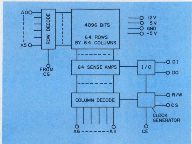
1. A 22-pin dynamic RAM uses a direct approach. Separate address, data, control lines and power pins ensure simple interfacing.
