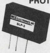
The SLP protectors were expressly designed to protect signal/data/telephone lines from transient overvoltages caused by lightning, heavy machinery, elevator motors, generators, etc. The SLP interfaces between the signal lines and the sensitive circuit to provide a sophisticated blend of high speed (nanoseconds) voltage limiting and brute force protection. The SLP's recover automatically to standby when the need for protection has passed.
