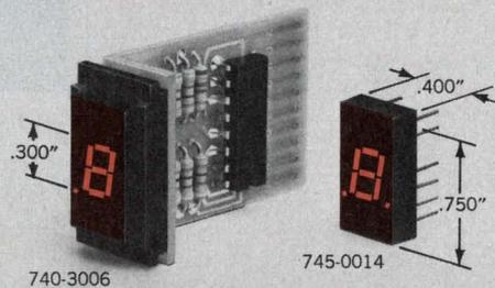
**745 SERIES** A new 0.300" LED character in a very bright red, seven-segmented readout . . . low power requirements. Standard 14-pin DIP . . . available with left and right decimal with  $\pm 1$ , and with and without on-board decoder/driver. Compatible with most TTL and DTL circuits. In 1000-lot quantities each
