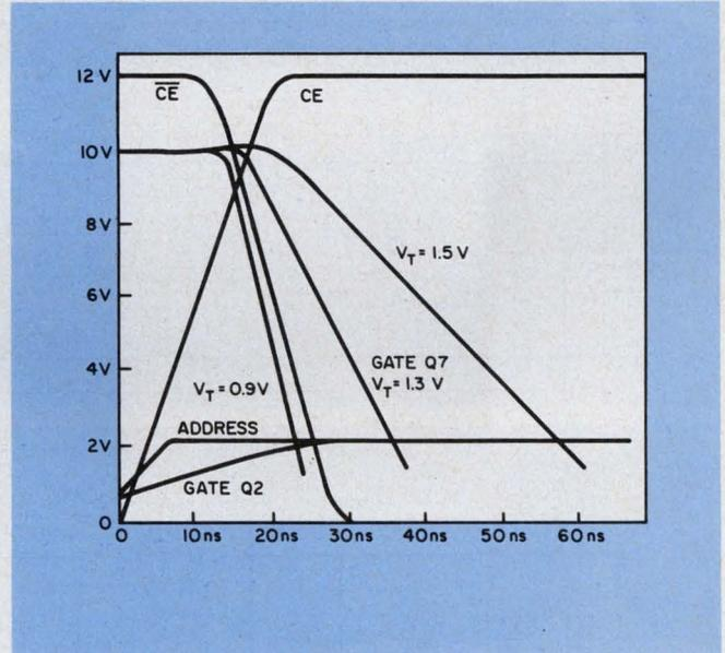
3. RAM input-buffer delay depends on the threshold voltage,  $V_T$ , as shown in these simulated steering waveforms. Speeds can be increased, if unrealistic "TTL-compatibility" specifications are modified.
