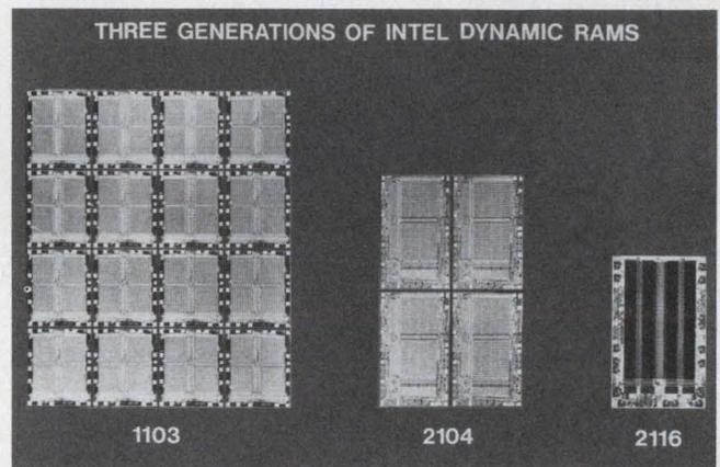
The rapid increase in chip-circuit density over the last few years is illustrated by these Intel RAMs required to produce  $16 \text{ k} \times 1$  storage. The single 16-k chip at right is equivalent to the four chips in the center and 16 chips at the left.
