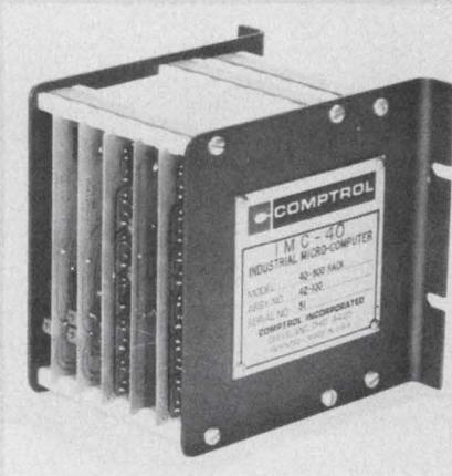
The IMC-40 industrial microcomputer can replace many larger machine and process-control systems. The  $\mu$ C consists of a 4040 CPU and can hold up to an 8-kilobyte control program. Since the I/O circuits use high-noise-immunity logic, the IMC-40 is practically immune to industrial noise.
