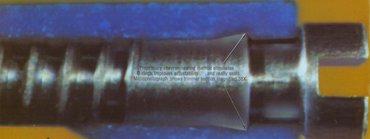
Proprietary chevron-sealing method eliminates O-rings, improves adjustability . . . and really seals. Microphotograph shows trimmer section magnified 38X.
