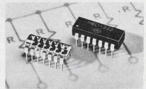
**DUAL-IN-LINE, RESISTOR NETWORKS** for such typical applications as pull-up and pull-down networks or line terminators. • 7 or 13 resistors, 14 pin • 8 or 15 resistors, 16 pin • Resistor values: 100 ohm to 10K ohm. • TCR: ±200ppm/°C • Thick film resistor tolerance: ±2%. All are available for off-the-shelf delivery from over 200 Centralab Distributors. For the name of your local Distributor call 414-228-2911.
