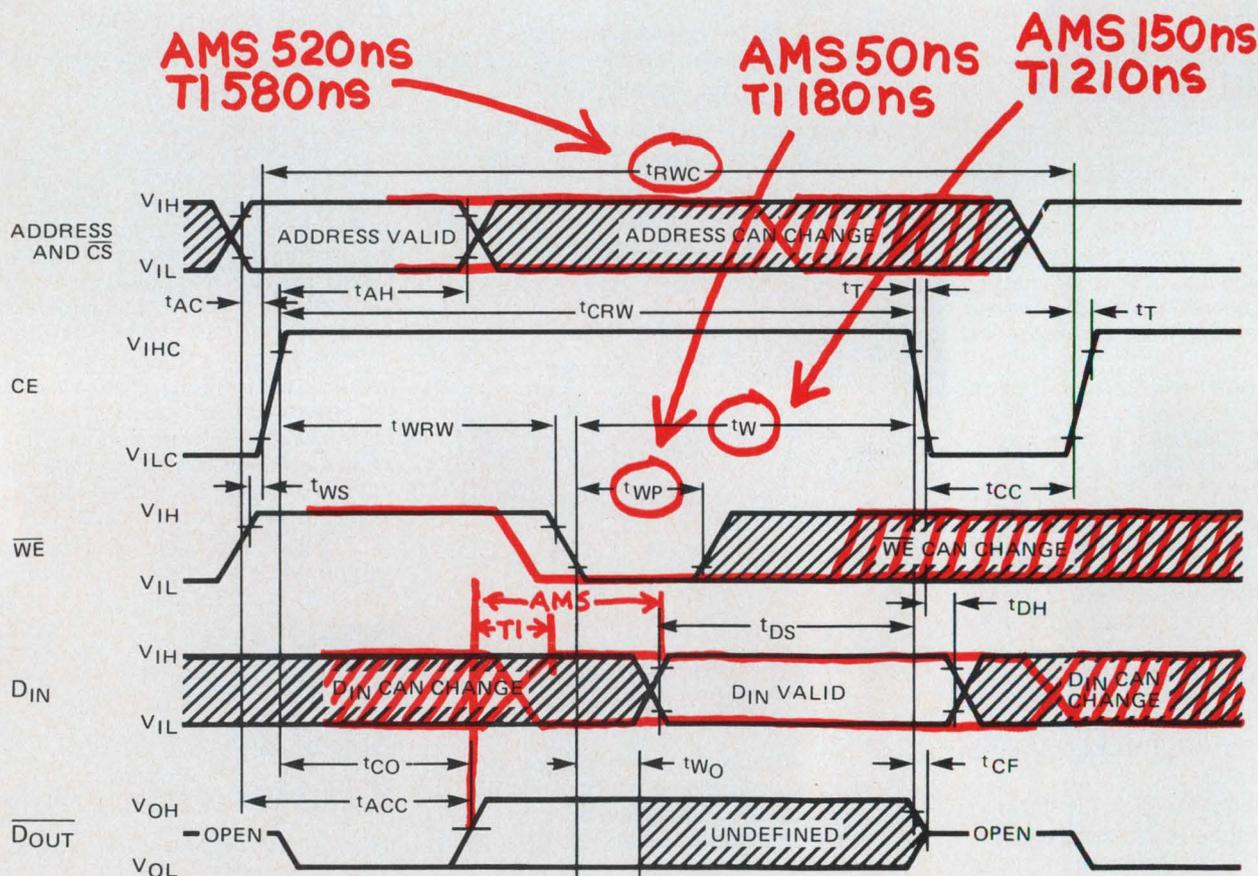
The excessively short system modify time for TI's 4060 stems from the fact that the  $\overline{WE}$  line must go low 60 ns earlier than our 7280. TI's Data In must be stable when  $\overline{WE}$  goes low, while ours only requires that Data In be stable 150 ns prior to CE going low, a clear advantage of 60 ns for the 7280, 80 ns for the 7270.
