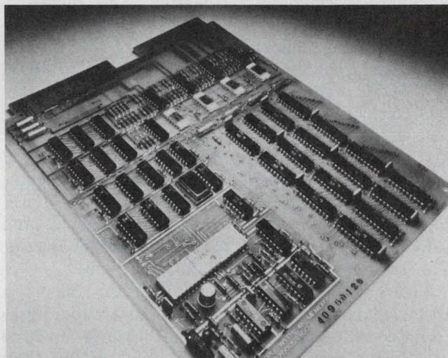
The microNova single-board 16-bit computer from Data General has a 2-bit-wide serial bus and is available with either 2-k or 4-k words of memory.
