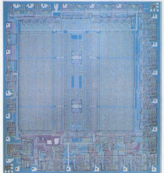
C<sup>2</sup>L, or closed CMOS logic, is used in the RCA CDP1832 512  $\times$  8 memory for small size and high drive capability. Access speeds are between 200 and 400 ns.
