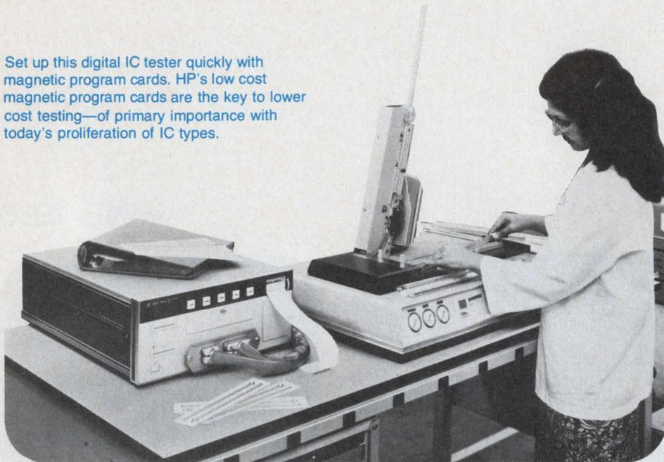
Insert an inexpensive magnetic programming card, and in five seconds this new multi-family Model 5045A digital IC tester is ready for dc parametric and functional testing of digital ICs. It's that simple—absolutely no other set-up or programming is needed. And it'll do some of your RAM and ROM testing too. Programming is so versatile that it can set-up a unique voltage and current level on each pin of the device under test within the limits of  $\pm 200$  mA and 0 to 15V or  $\pm 7.5$ V range.
