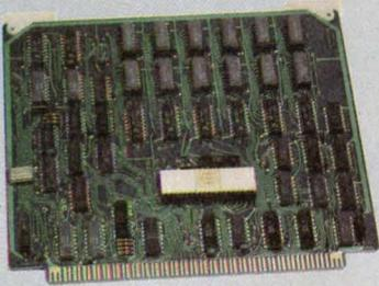
A single chip, N-channel processor arms you with a super-set of 158 instructions that include *all* of the 8080A's 78 instructions with *total* software compatibility. The new instructions include 1, 4, 8 and 16-bit operations. And that means less programming time, less paper and less end costs.
