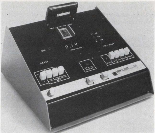
You can test six important op amp parameters with the ESI 1234:  $E_{OS}$ ,  $\pm I_B$ , gain, CMRR and stability. Go/no-go testing is also possible.
