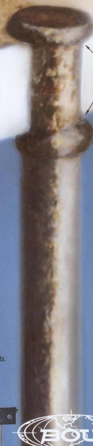
Swage-Bond™ eliminates pin termination failure, provides more reliable tempco. Microphotograph shows trimmer element magnified 20X.
