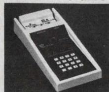
We also make a portable programmer, FPLA programmer and the Romulator.™ The Romulator allows you to emulate/simulate PROM operation - in your circuit - without PROMs. PROM data is easily altered
