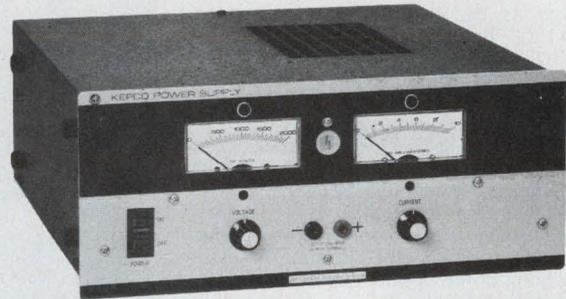
Control voltage with a 10-turn precision panel control (or program like the OPS). Another 10-turn panel control adjusts the output current. LED annunciators signal operation in either voltage mode or current modes. A built-in "uncommitted pre-amplifier" is available for scaling or summing programming inputs. Output is monitored on a pair of 2½" meters.
