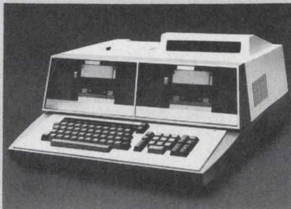
A versatile, remote data terminal has been designed by MSI Data Corp. (340 Fischer Ave., Costa Mesa, CA 92627. 714-549-6000.) Called the Source 7600, the unit uses an 8080  $\mu$ P. The terminal can accept data formatted by the operator and transmit them over a phone line. It can also handle preformatted information such as ordering and inventory data.
