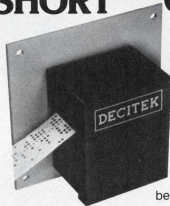
You could spend a lot more for a tape reader and still not get all of SAM'S quality features. SAM clips along at 300 cps, has our sure-footed dual sprocket drive and our state-of-the-art fiber optic light source and photo transistor read head. We can make SAM do all this *and* save you money because we do things differently.
