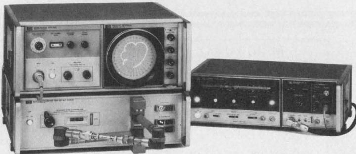
The familiar HP 8410 Network Analyzer now has automatic tuning to track the wide sweeps of the HP 8620A sweeper with its new broadband plug-ins.
