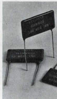
5, 10, 20, 50, 100, 200, 500, 1000, 2000, and 5000 megohm. All in stock. With a voltage coefficient of better than 5 ppm/volt, full-load drift typically less than 0.5% in 1000 hr at 70°C, and 250 ppm TCR or less to 5000 megohm, SLIM-MOX is a little, big performer. For less than a buck.
